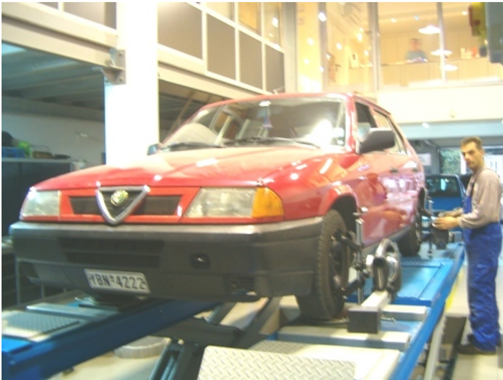
Apostolos hard at work attaching the reflector devices on the left side ...
