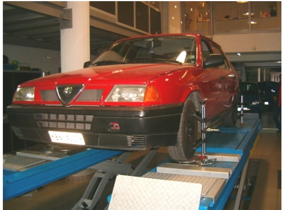
The car sits on the alignment ramp, tyres are carefully inflated at 28 psi and alignment bars are attached to the rim lips on the left side
