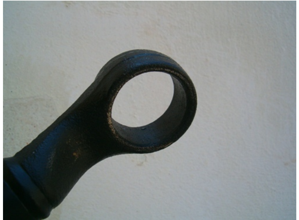
... finally tweaking around with a screwdriver pops the bush out
