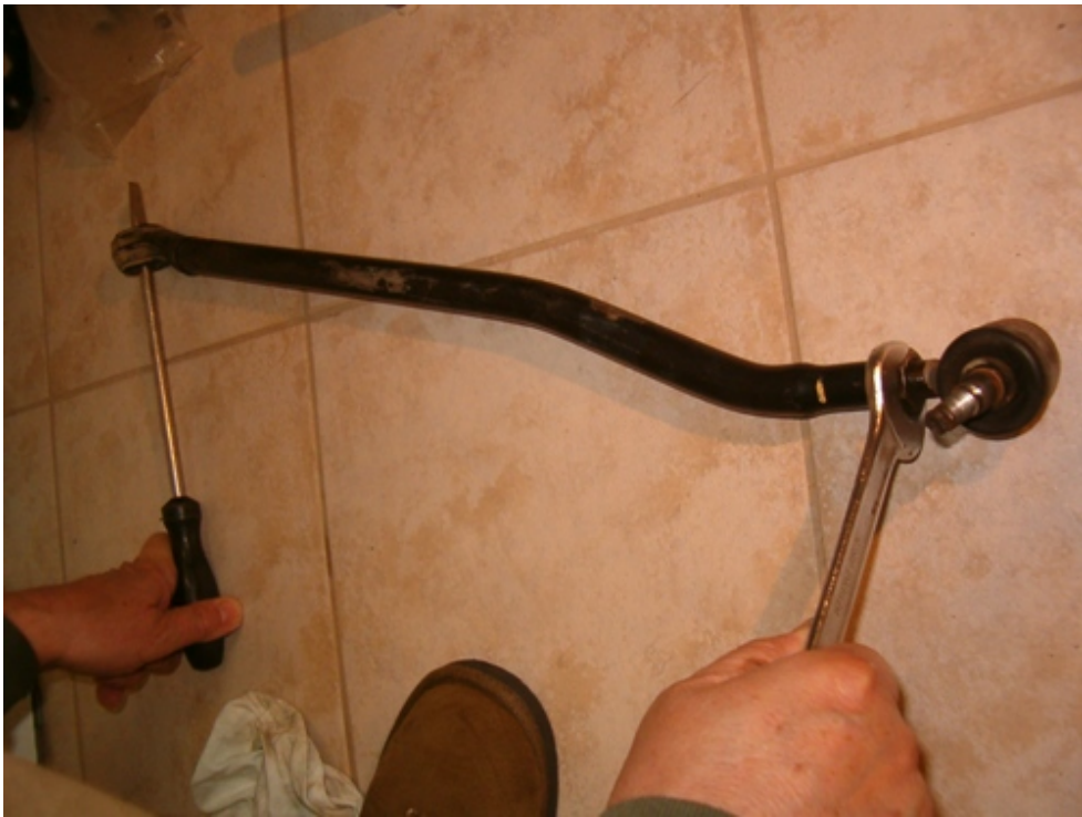
Loosen the ball joint lock nut ...
