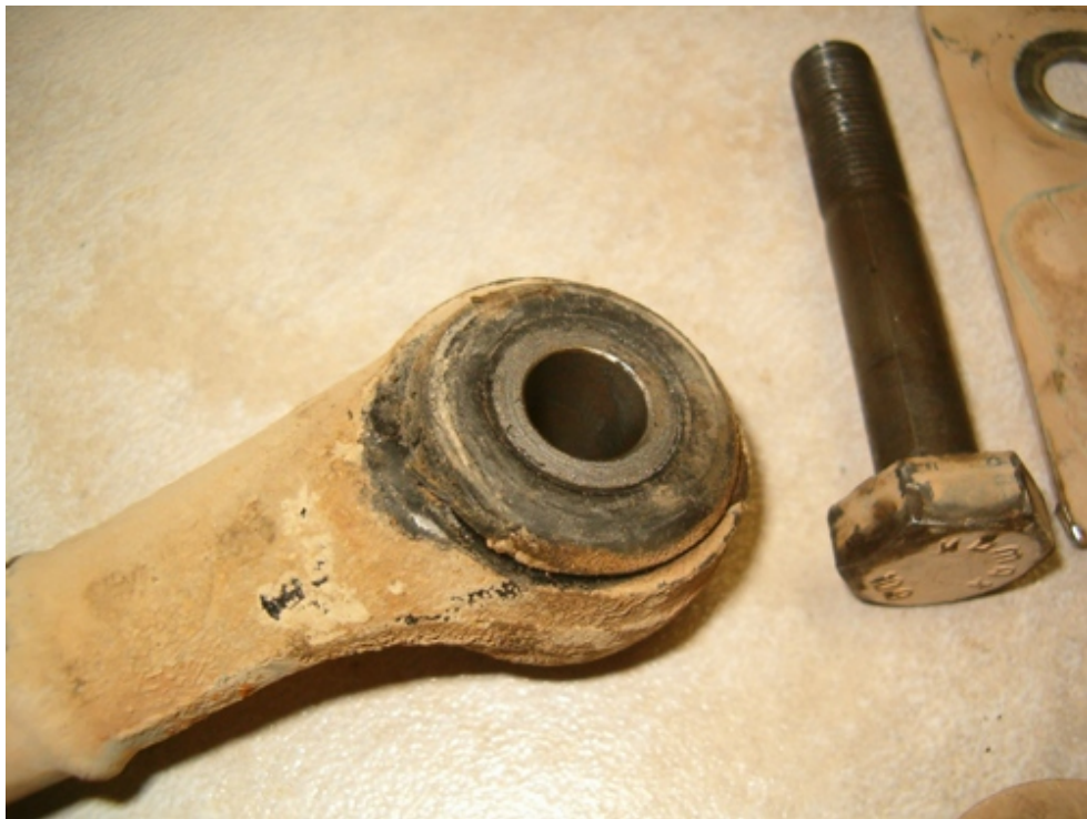
Also a close up of the bush and the 24 mm bolt. Both bushes will be renewed.
