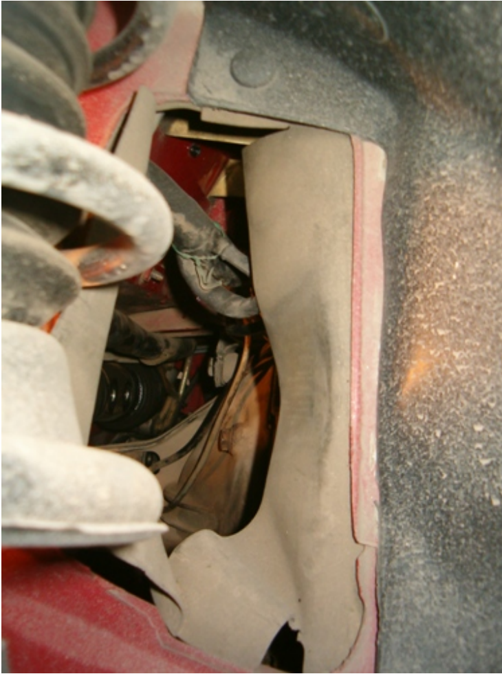
These are the worn out protection pads that will be replaced.
