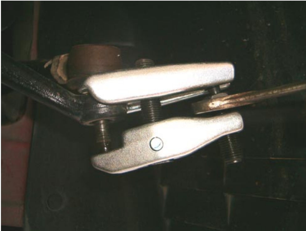
Extract the ball joint with the extractor ...
