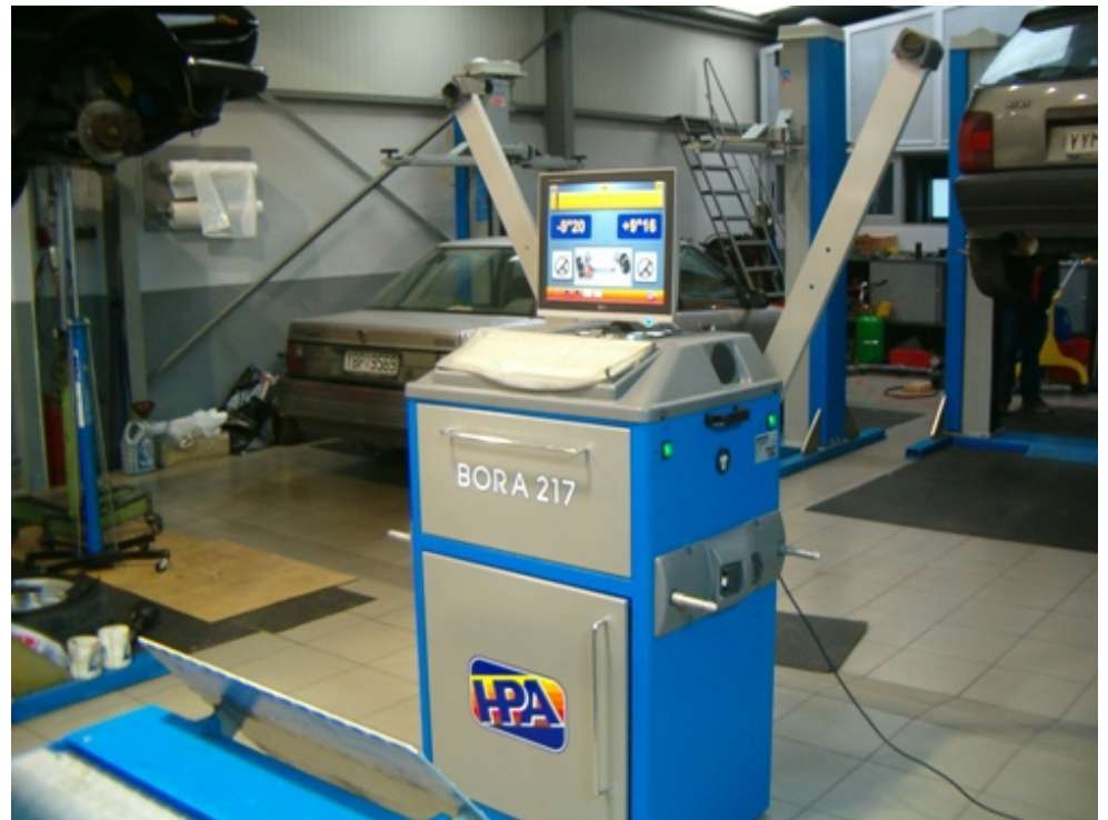
Measurements are displayed on the monitor and adjustments are done to the geometry by the mechanic.
