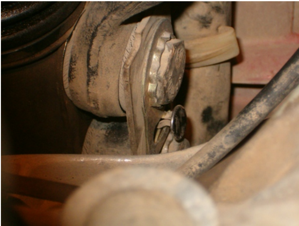
Locate the centre of the steering box and remove the securing pin
