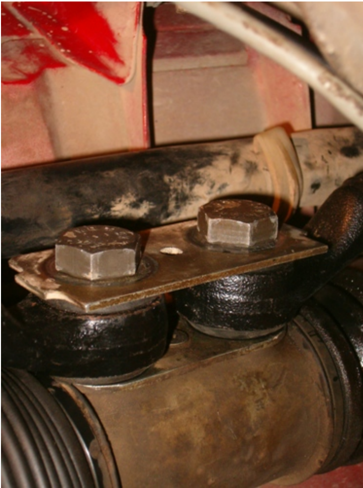
Restore the bars at their position in the steering box along with the relative plate. Torque down the bolts at 39 - 48 Nm
