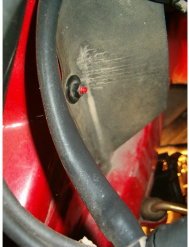
These are the worn out protection pads that will be replaced.
