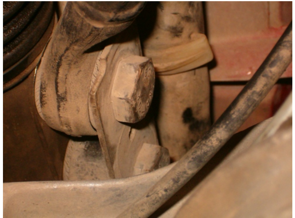
Head bolts (24 mm) are exposed and slackened.
