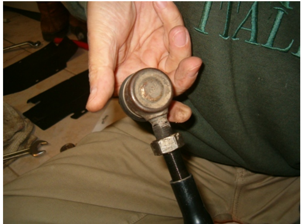
... and remove ball joint.
