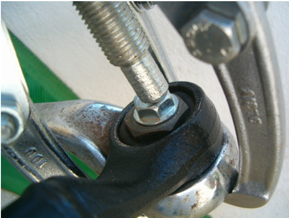
Here you can see a DIY patent when the home garage misses a hydraulic press. Puller pushes the bush and the bar is supported by a 36 mm wrench ...
