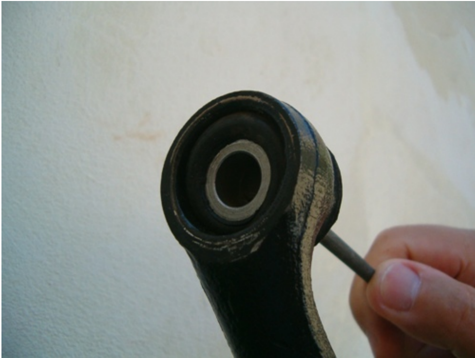
... finally tweaking around with a screwdriver pops the bush out
