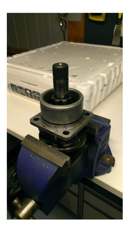
Here you can see the thread which was cut on the tube to screw on to the locking ring and the machined threaded rod to press on to the end of the mini axle
