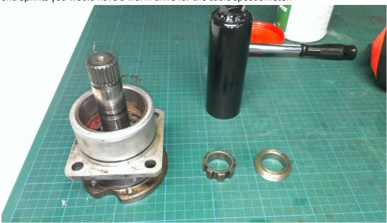
Once the rings are removed you will need to push out the axle from the carrier. This can be done using a press or a jaw puller. As this does not require much force it can be clamped on the alloy carrier (a 2 jaw puller would be preferable here)
