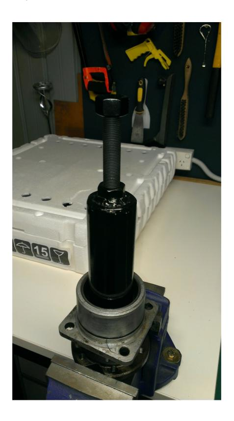
Here you can see the threaded lock ring and the phonic wheel that comes off too. The phonic wheel is used for the speedometer signal for the Alfa 33s, where as for the Sud's and Sprints you would have a worm drive for the cable speedometer.
