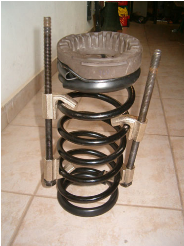
Spring along with the thrust ring in place ready to be fitted on the vehicle. Notice the thickness of the thrust ring.
