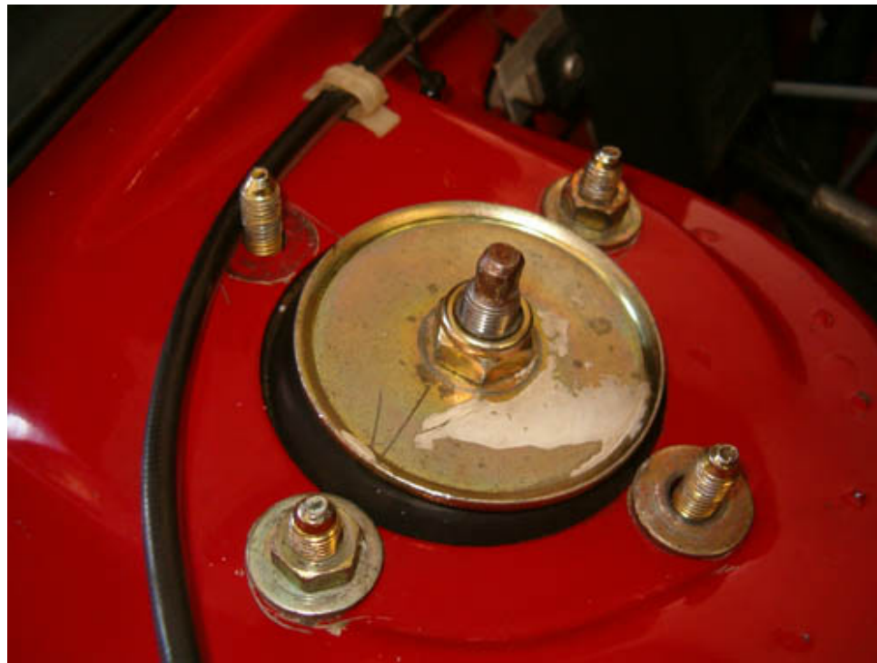
Temporarily keep the strut in place with two nuts
