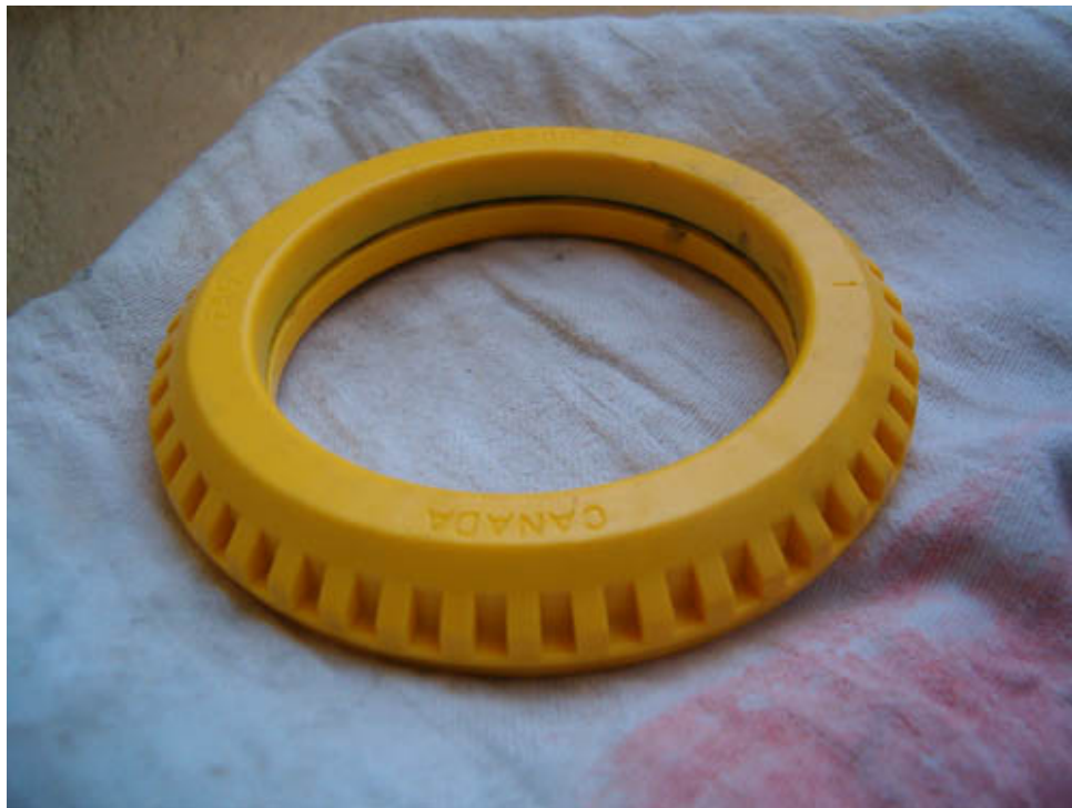
This is the notorious strut pan bearing that is prone to wear. Actually this bearing holds the weight of the front part of the car plus the tension of the suspension.
