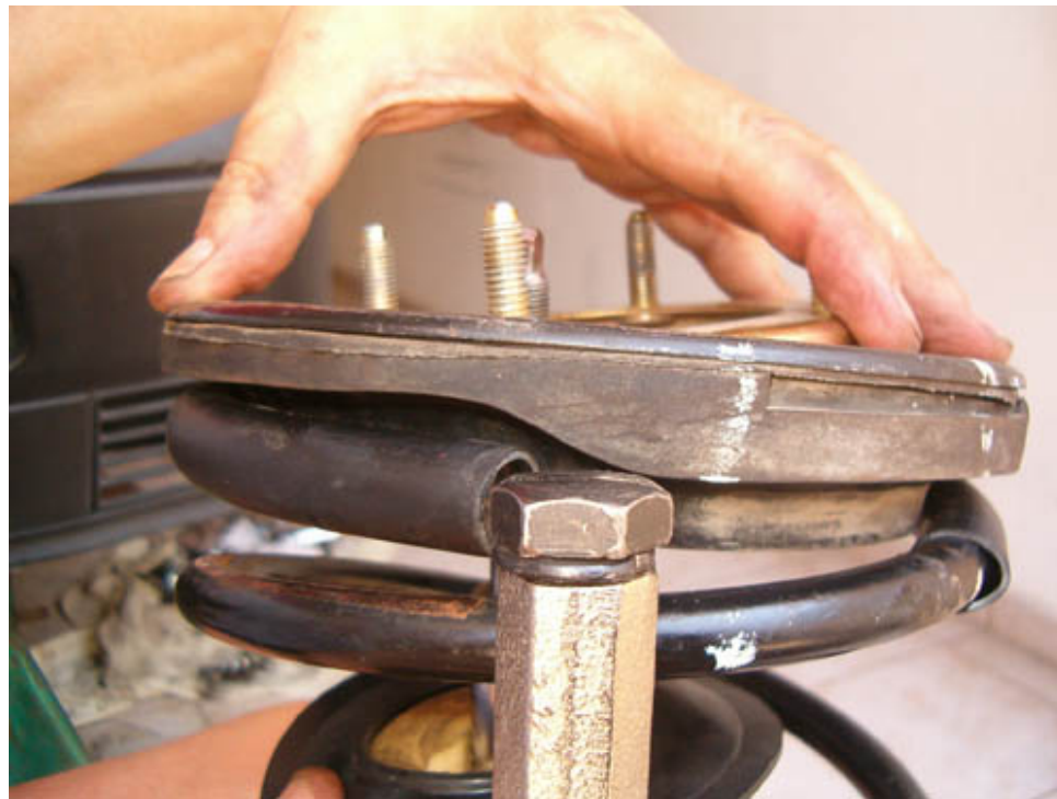
Be sure to align the notch of the retainer to the spring edge
