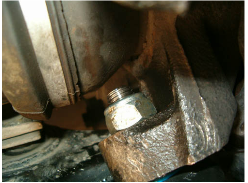
... be sure to fully tighten the nut securing trailing-link to hub
