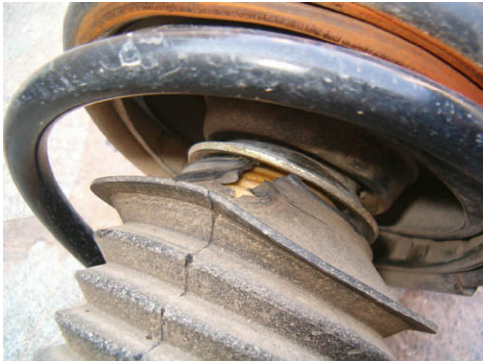
rubber boot is completely shot
