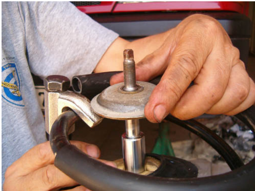
Install lower washer; this is where the upper part of the rubber boot is kept in place
