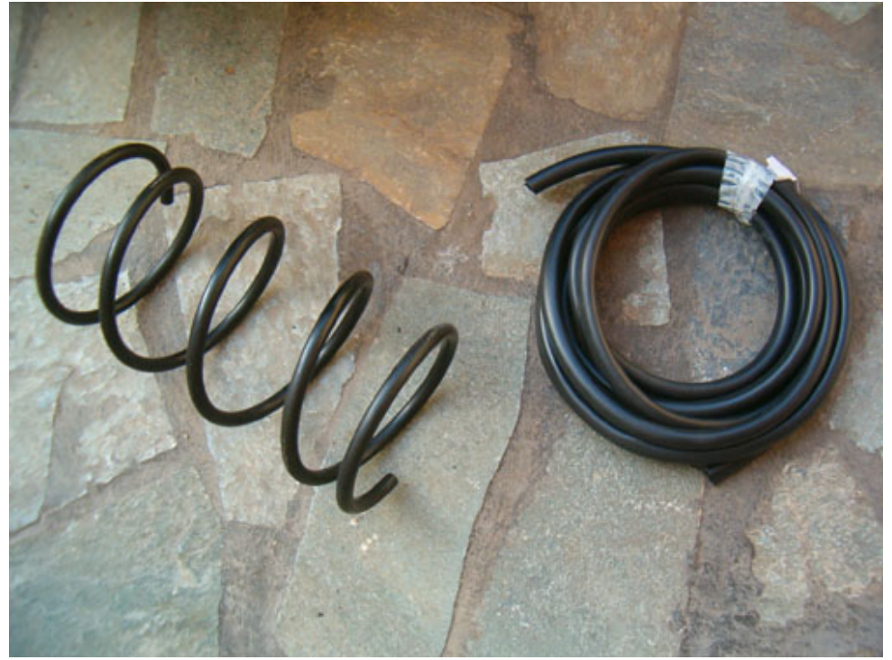
Be sure to install new rubber hose only at the first 180 degrees (1st circle) of the spring
