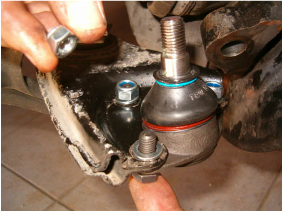
You can install it just reversing the order of removal ...
