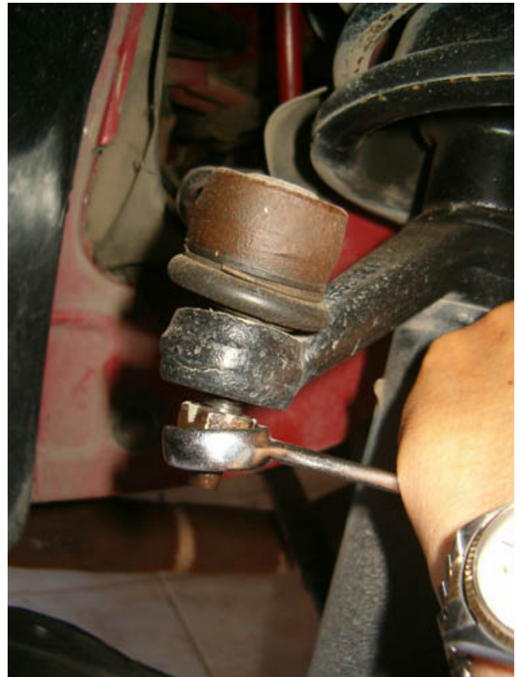
Loosen the four bolts attaching strut to hub and remove nut securing strut to ball joint (17mm key)
