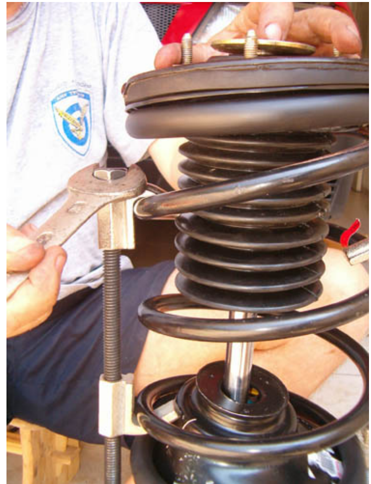
Finally, loosen the spring compressors in order to install strut on vehicle.
