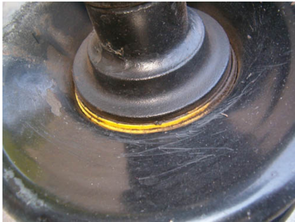
strut pan bearing doesn't look that bad ...
