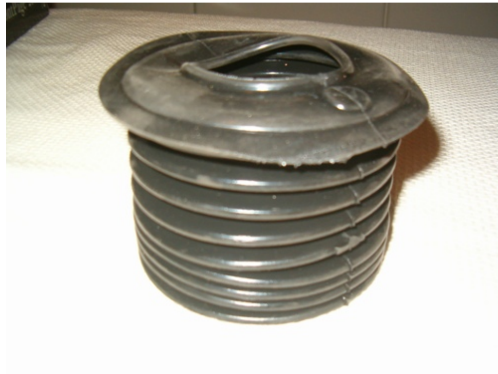
Not much to say about the boots of the strut. These boots, strut pan bearings and lower spring plates are common parts with the Alfa 164.
