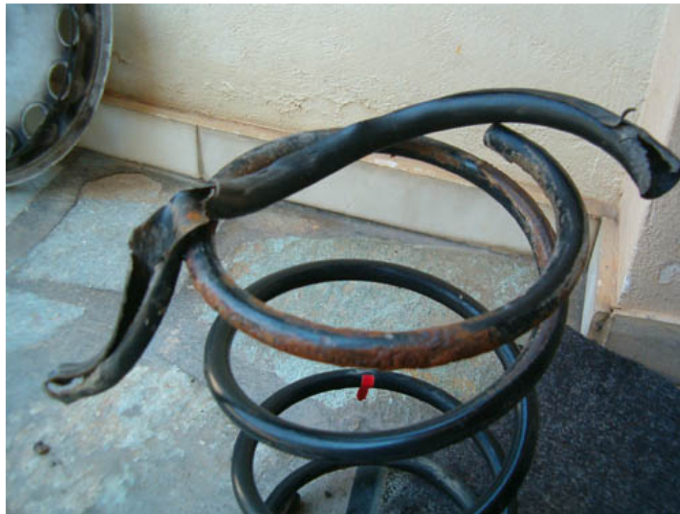
See the extend of corrosion on front springs and the wear on the rubber hose ...
