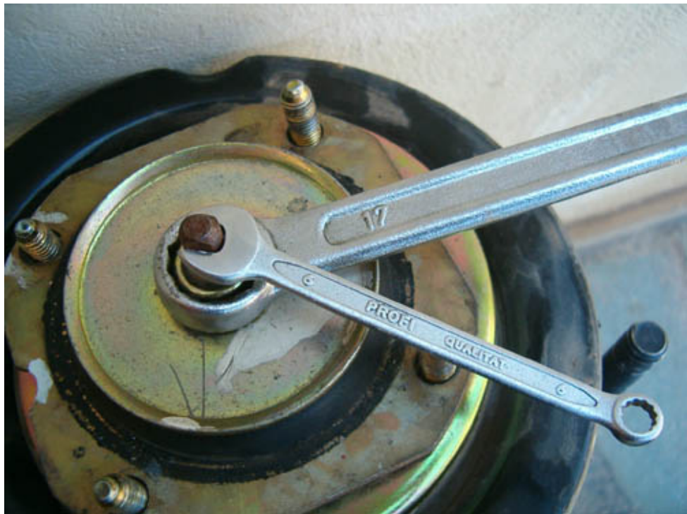
Use a 6 mm key to keep the strut still and with a 17mm undo the nut securing strut to top mount
