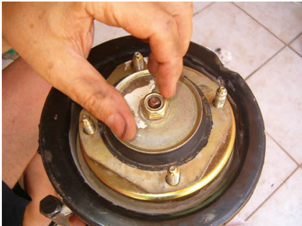
Bolt in the nut only a few turns. You can fully tighten it when on car.
