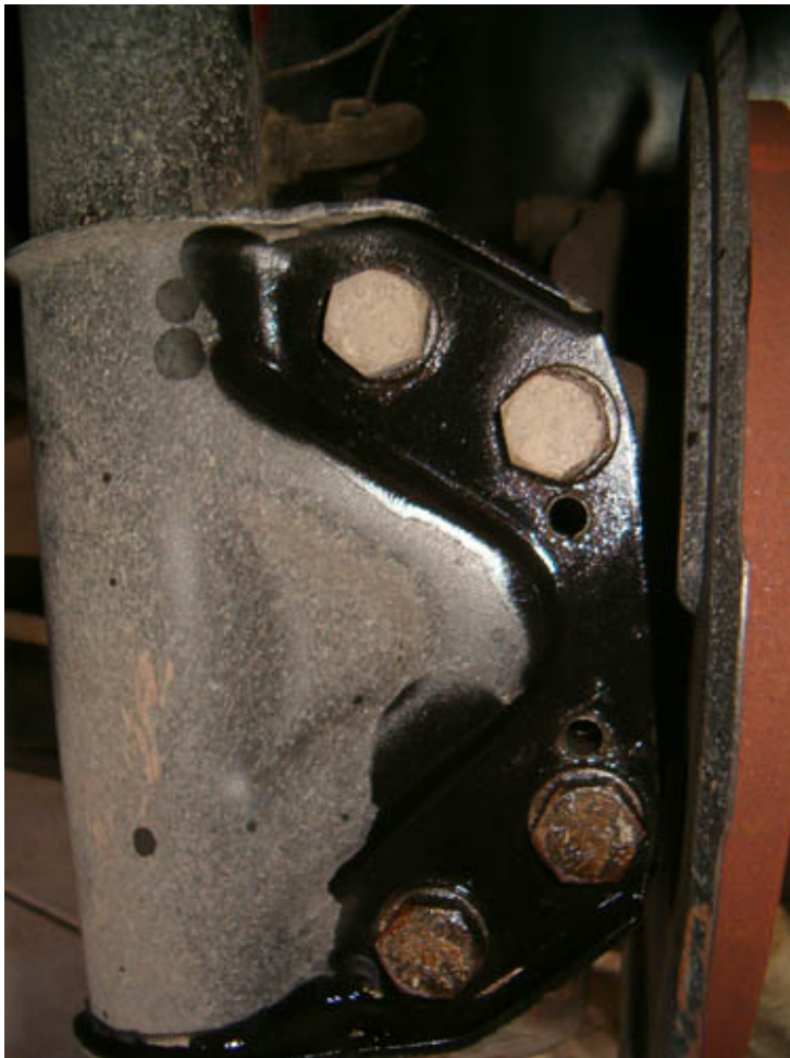
Loosen the four bolts attaching strut to hub and remove nut securing strut to ball joint (17mm key)
