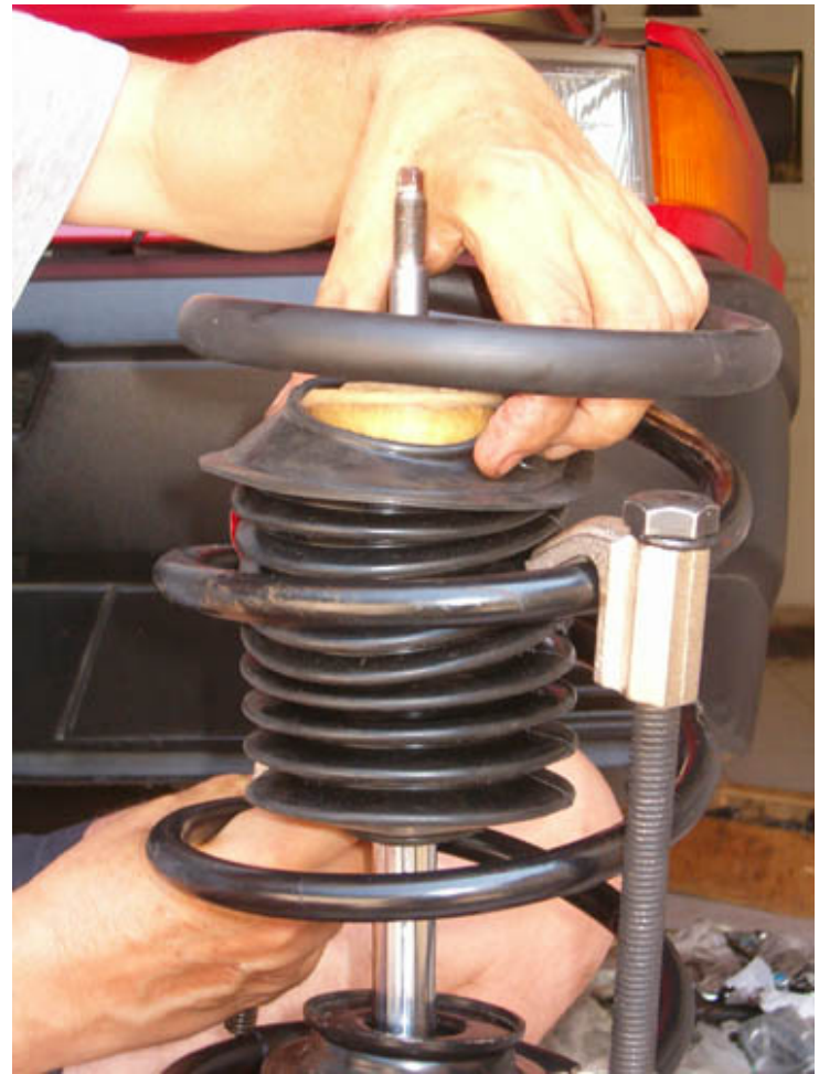
and rubber boot goes inside the rubber bumper.
