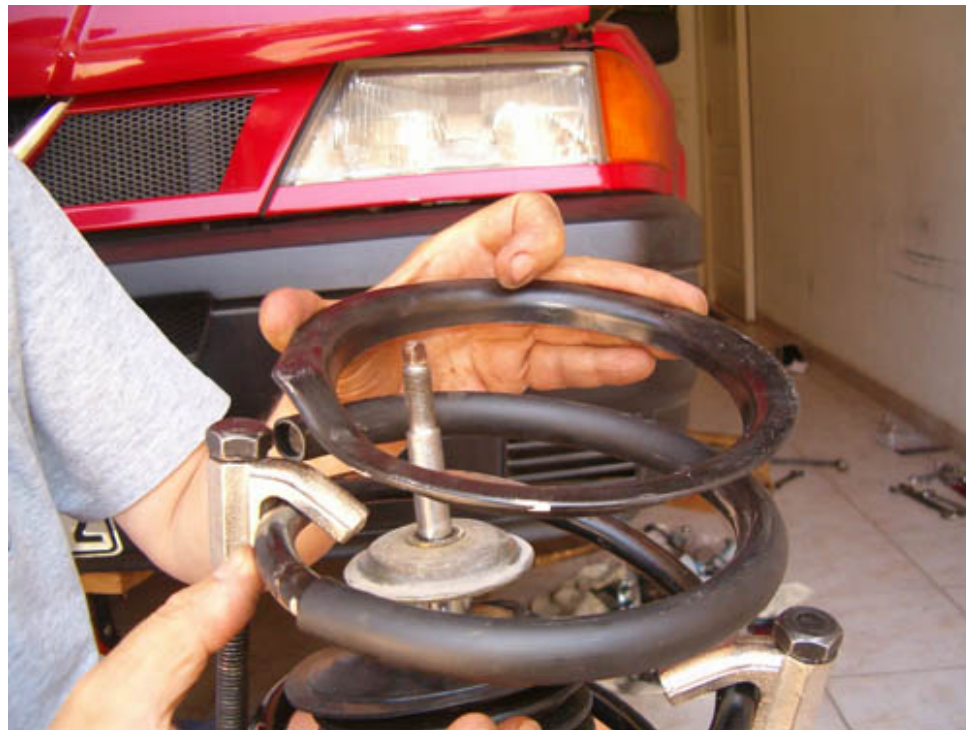
proceed installation of lower retainer ...
