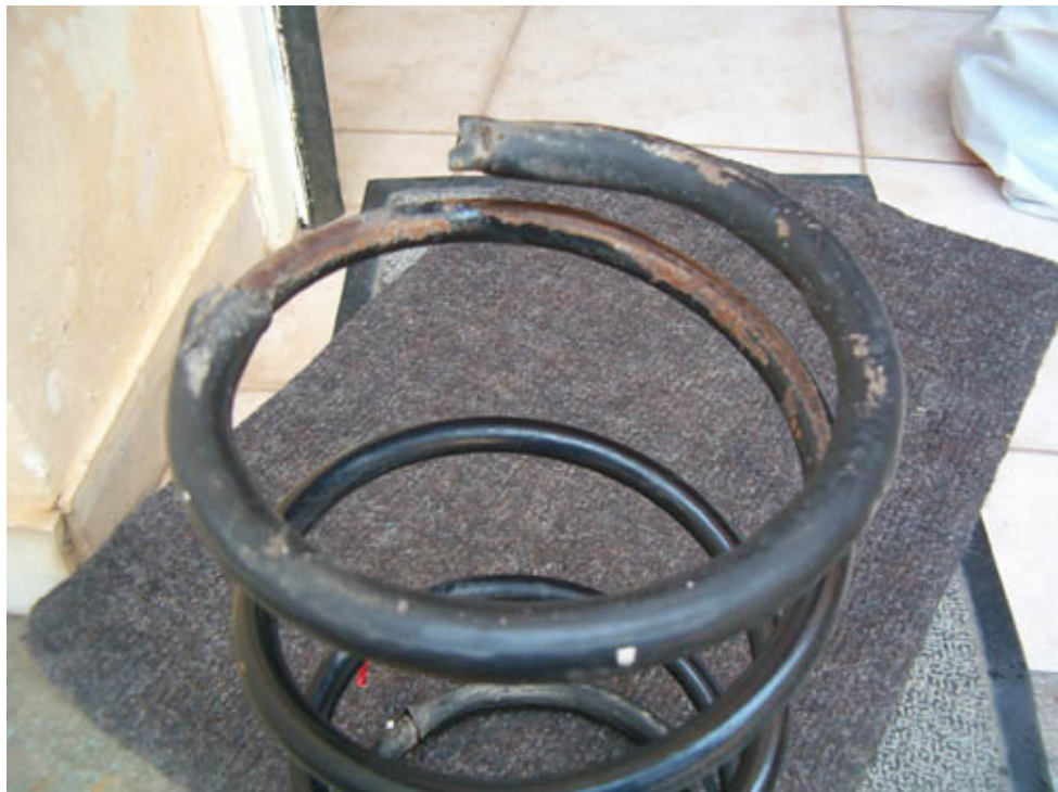
See the extend of corrosion on front springs and the wear on the rubber hose ...
