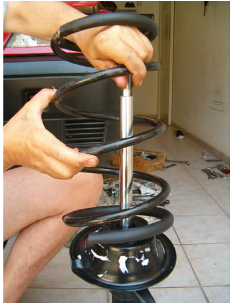
... next install spring
