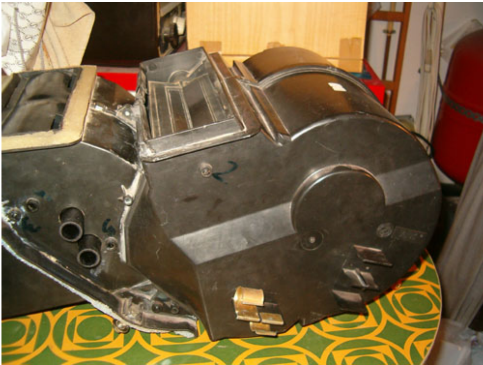
Restore the blower motor covers ...
