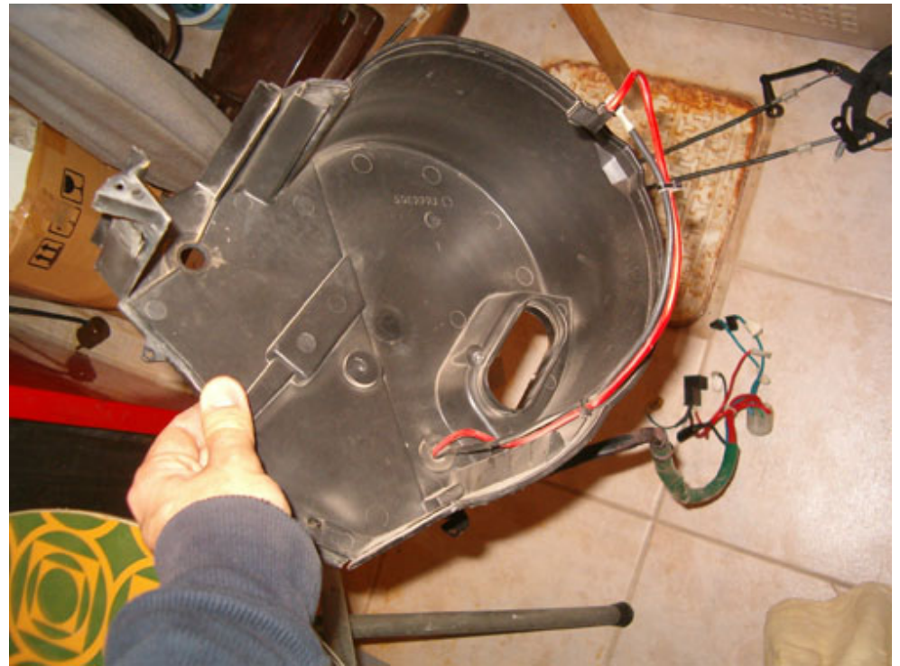
... and wiring harness along with the cover extracted.
