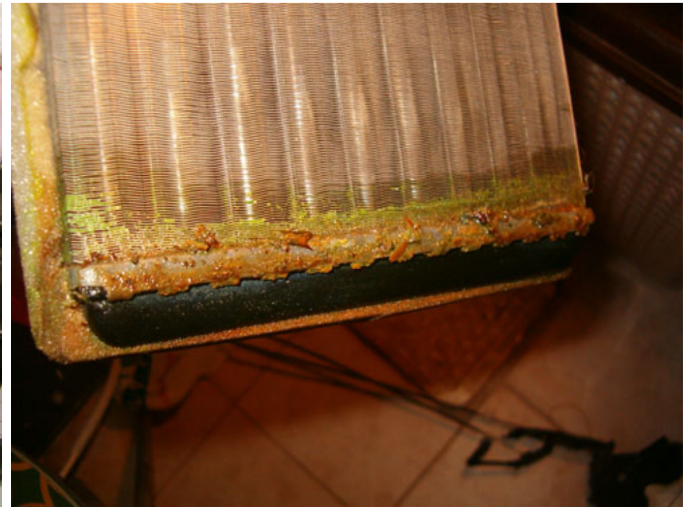
Here the problem is revealed. A fully leaking heater core ...
