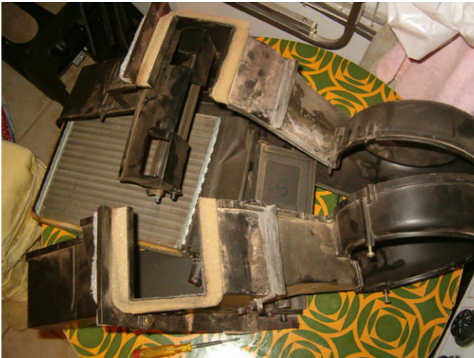
Heater assembly is finally taken apart.
