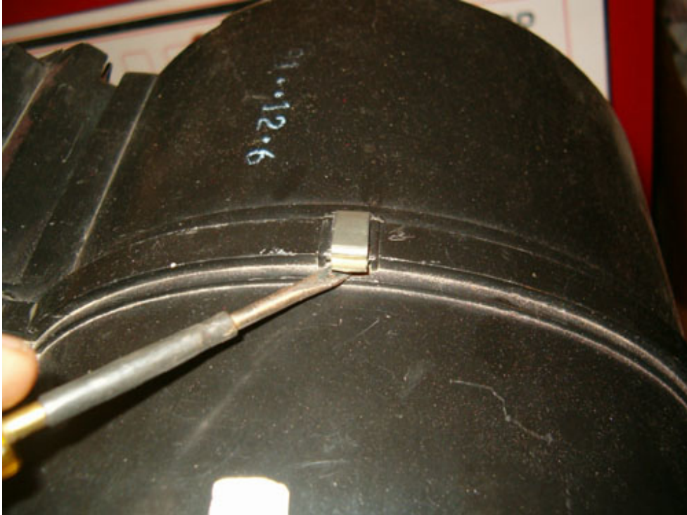
Now that the heater is on the bench let's move on dismantling it. Release locking seals ...
