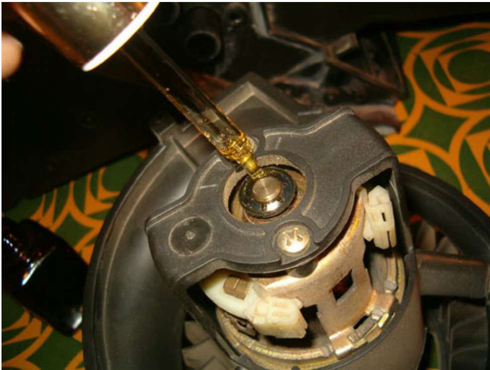
Why not lubricating the motor ...
