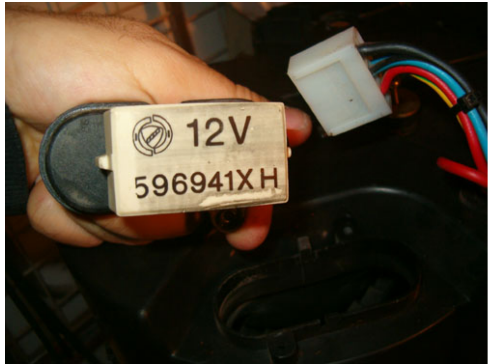
Carefully extract blower motor resistor. This device ensures three motor speeds at your blower - be extremely careful as it is ceramic and breaks easily. In case your blower motor lacks of three speeds, then it is high time you replaced the resistor.
