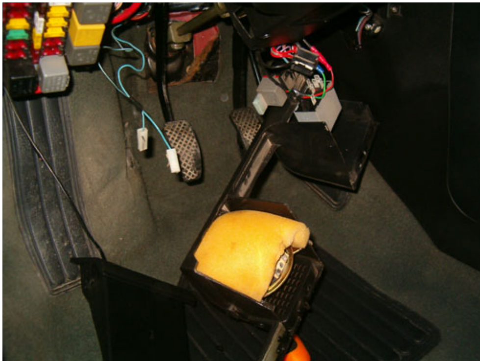
Disconnect speaker leads and the door locking mechanism connector ...
