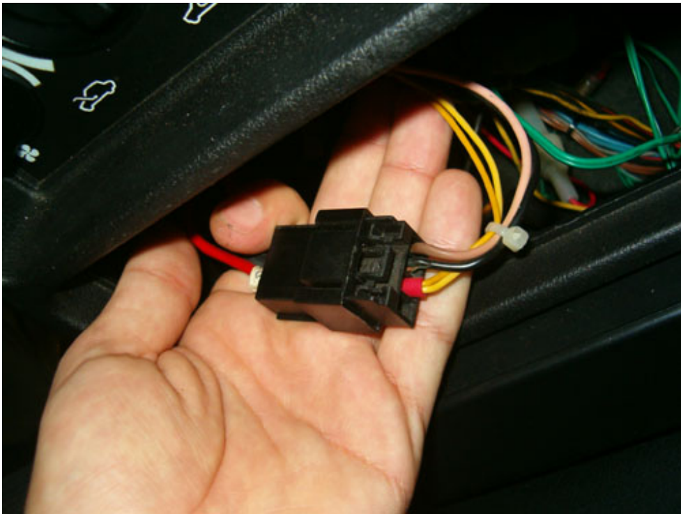
... and heater power supply connector.
