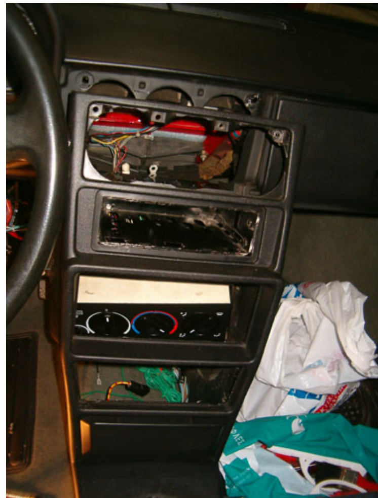
Having disconnected the cigar lighter and ashtray lights slide carefully the console until it is out
