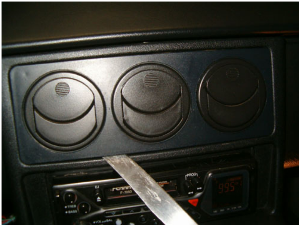
Use a blade to remove the fascia panel. Take it easy as this breaks easily!
