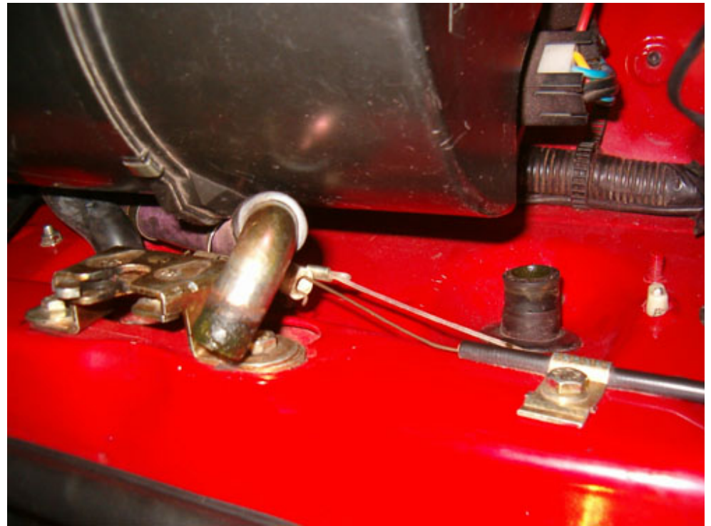
Notice the outlet piping disconnected and barely seen under the hood latch the inlet piping of the heater core.
