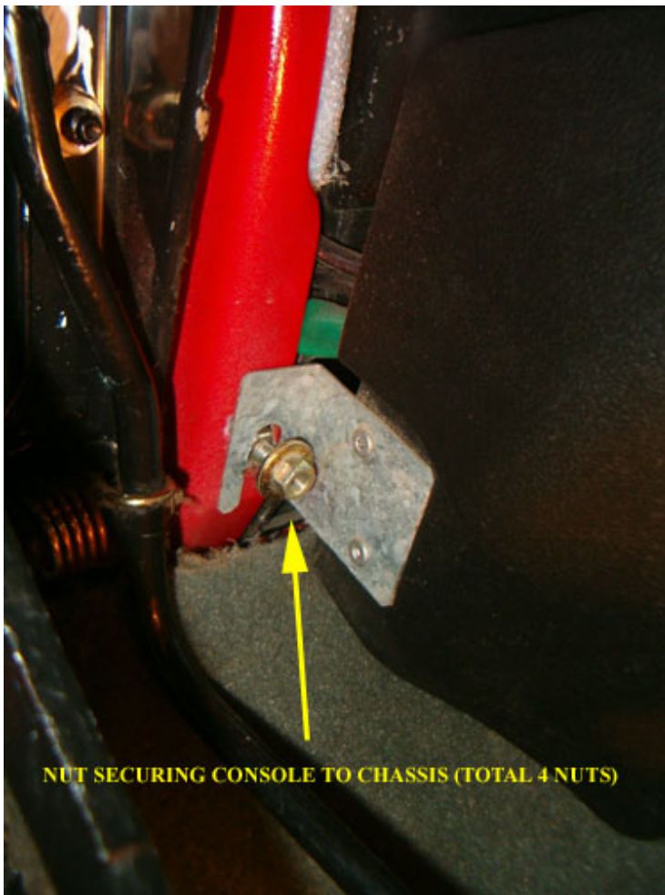
Finally undo the four nuts securing console to chassis (2 per side)
