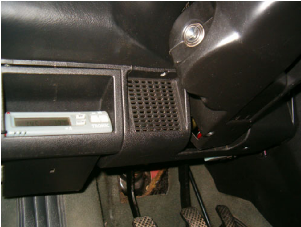
Move on removing the speaker assembly both sides
