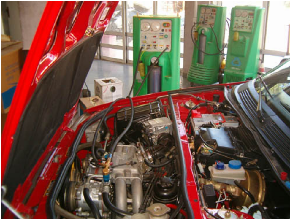
Charging hoses are attached to the compressor ...
