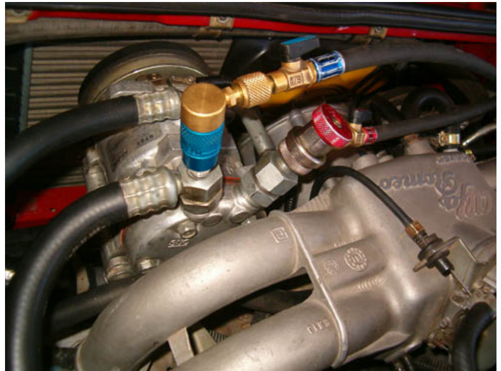
Charging hoses are attached to the compressor ...
