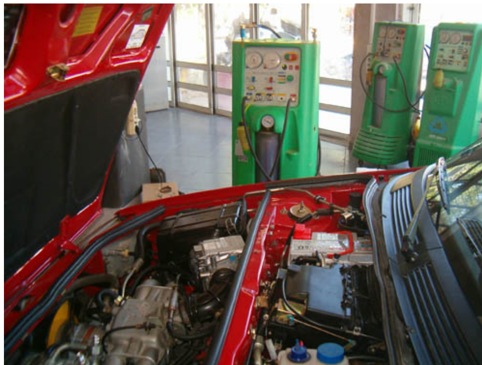
Vacuum/charging machine next to the car ready to do its job.
