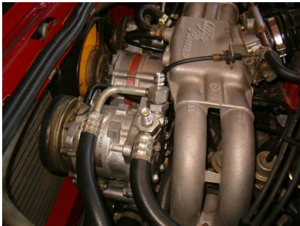
R134a service valves adaptors have been installed on top of R12 valves
