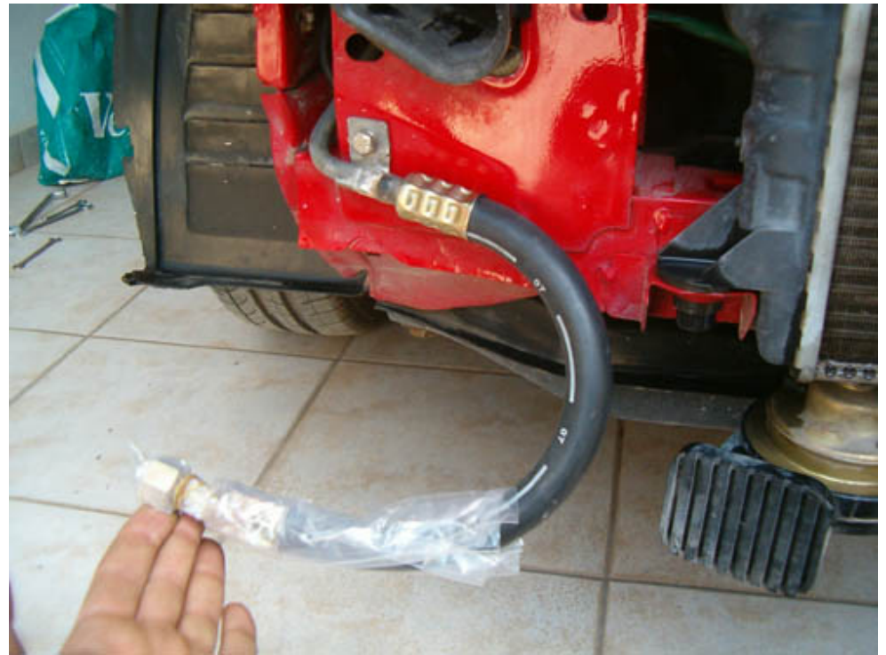
The end shown will attach on the condenser.
