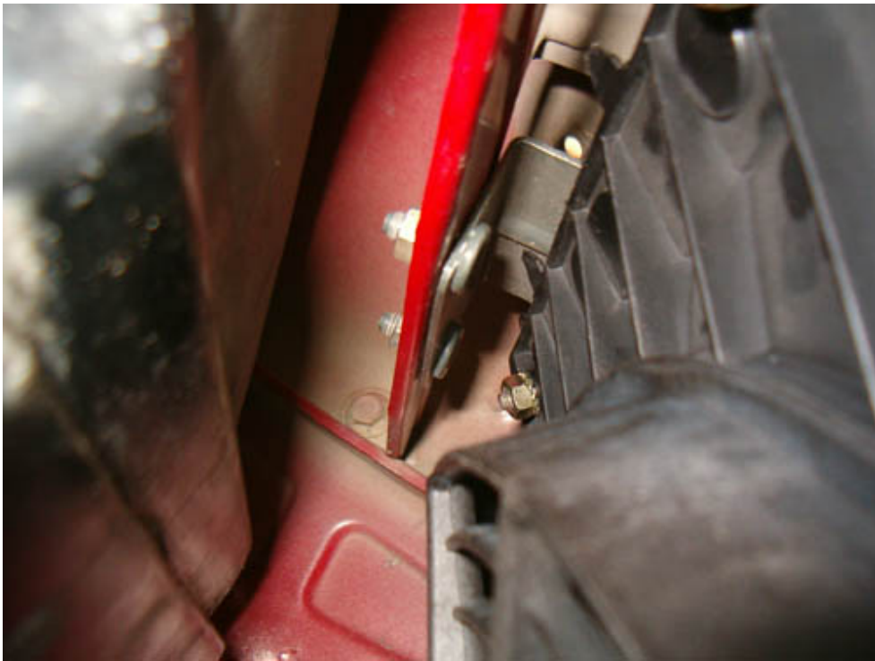
... and the third one is on the rear of the condenser.
