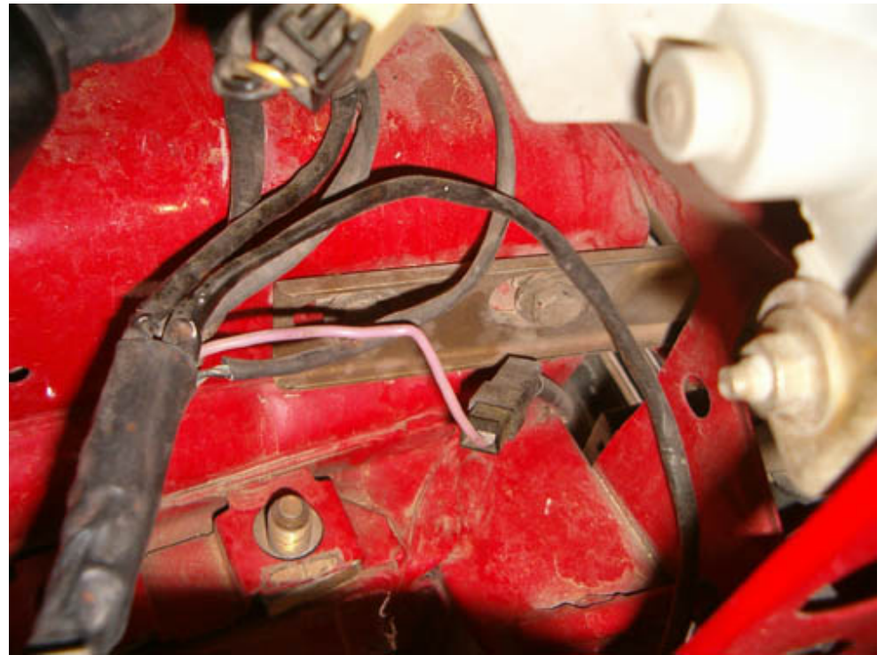
The bumper is required to be remove. Undo the two 13mm nuts of the bumper rail under the headlight (both sides).
