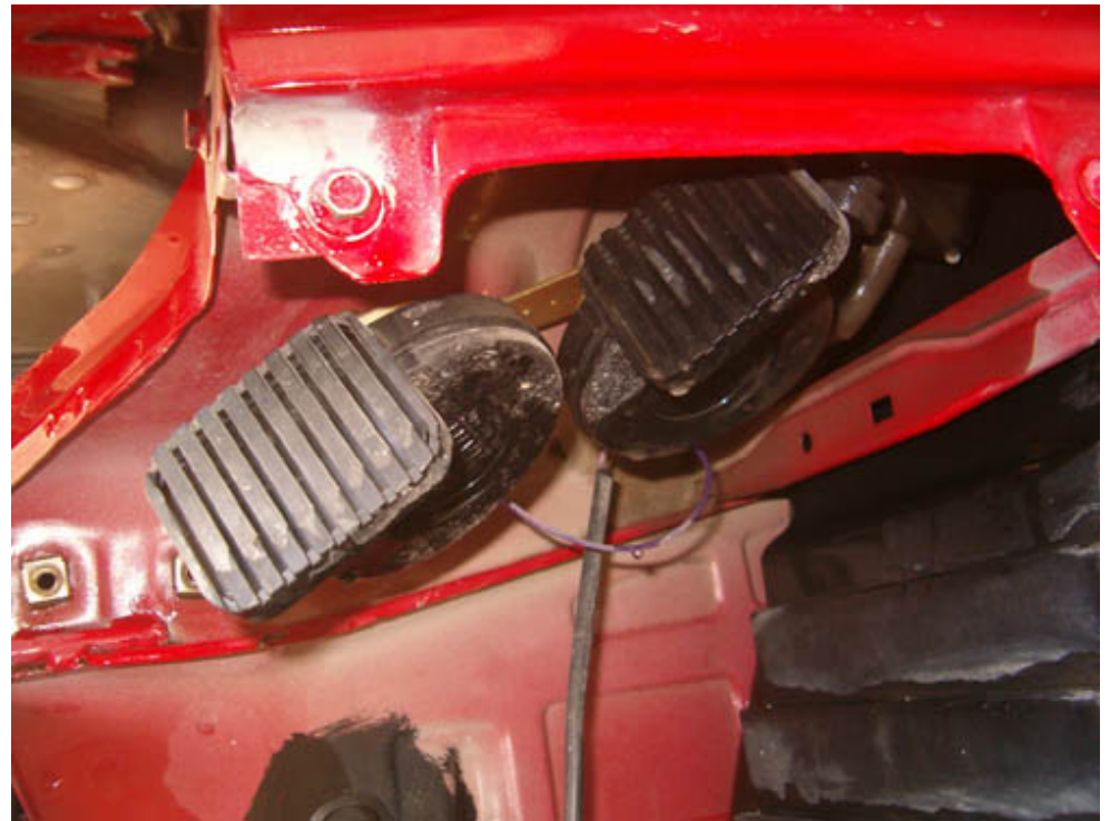
We will remove the horns since the space will be occupied by the condenser.
