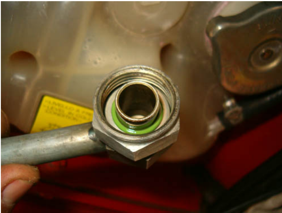
This is the part of the hose that bolts on the compressor port. Again use new O-ring coated with refrigerant oil...
