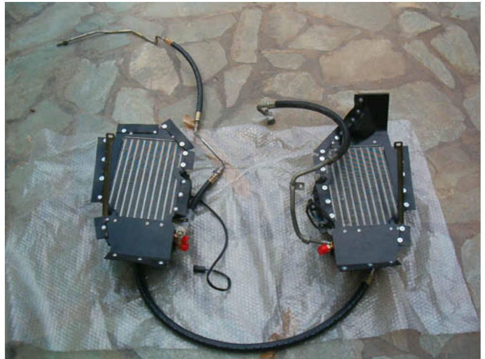
Let's now go to the second round of the installation dealing with the condensers.
