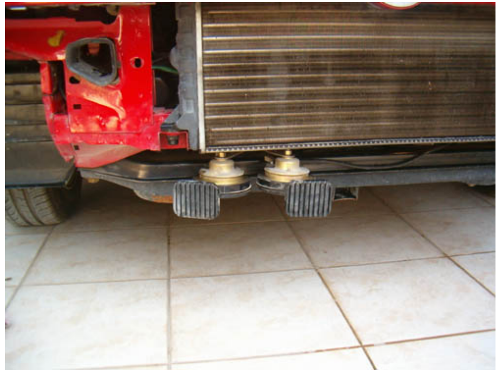
Horns are on their new position. You can use the original wiring since its length reaches the new location with no problem.
