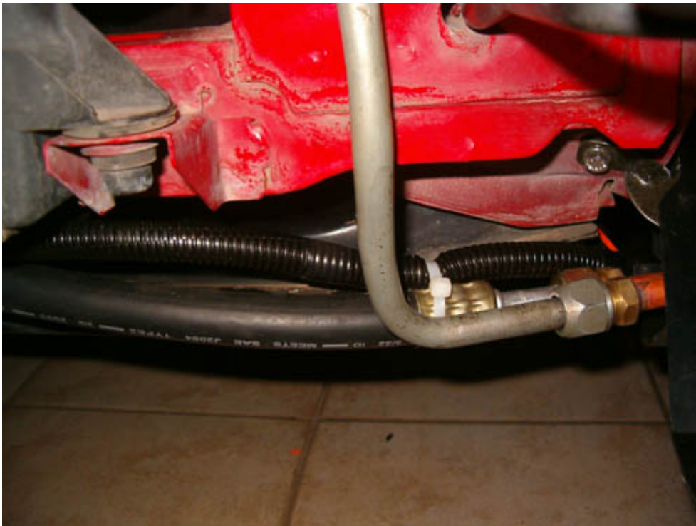
Wiring passes along with the Freon hose ...
