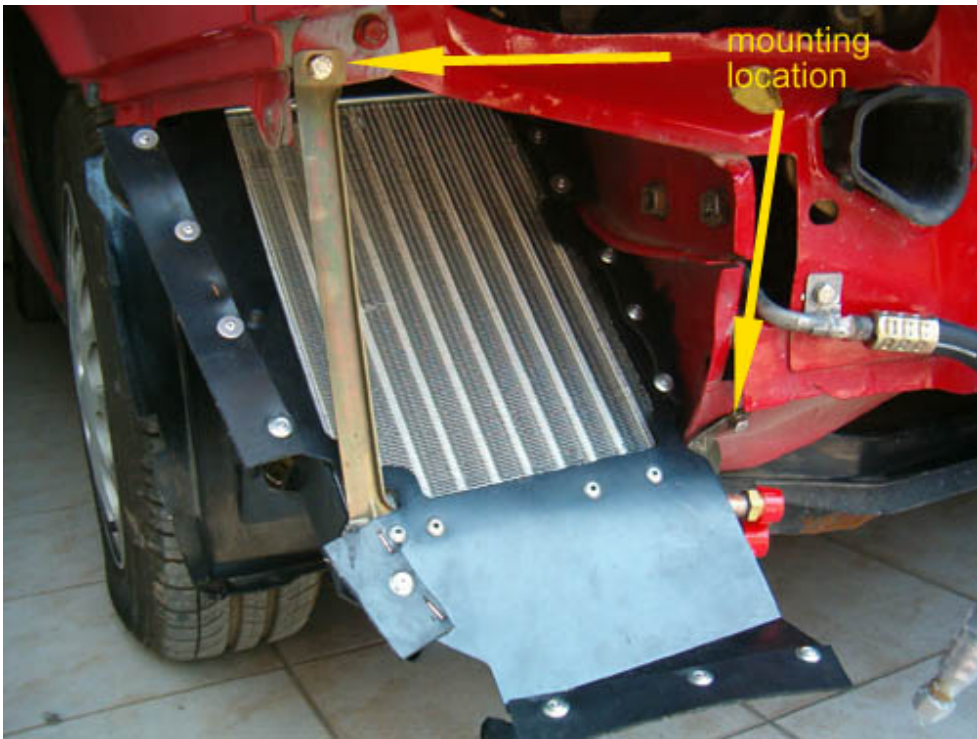
Condensers are now installed. These have three mounting locations; two are shown above ....
