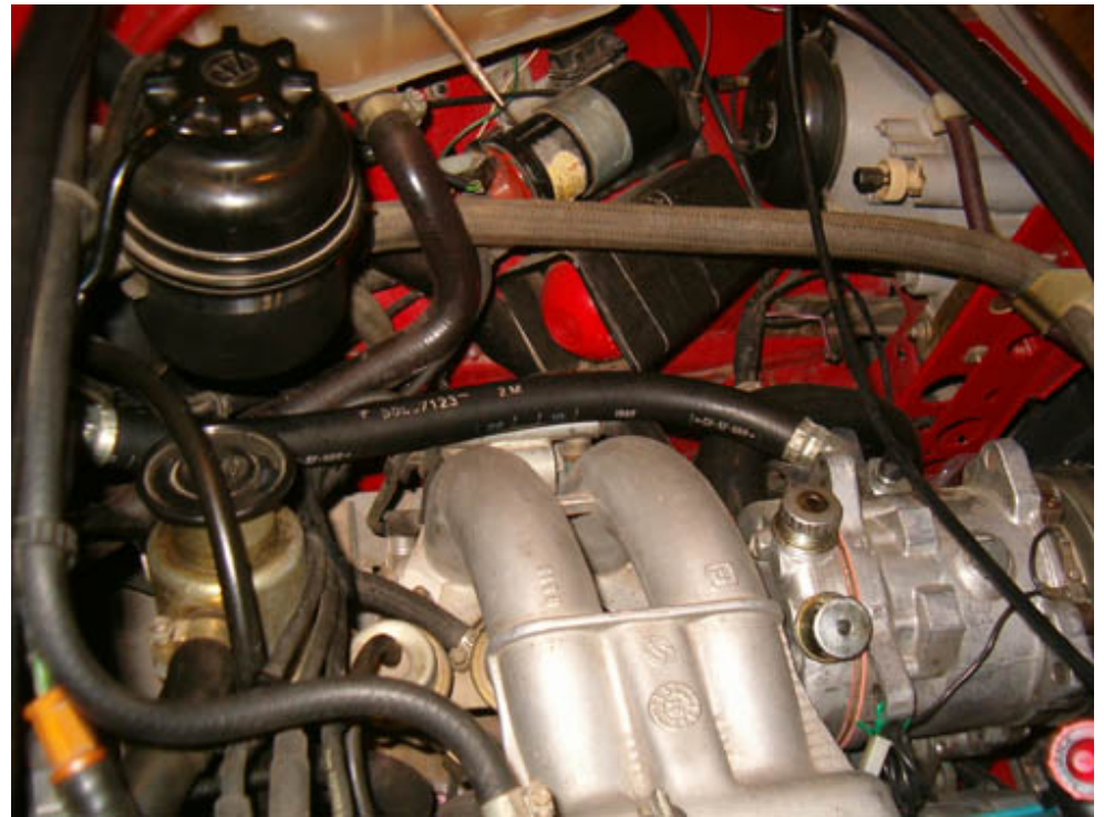
The end of the hose will bolt on the S (suction) port of the compressor
