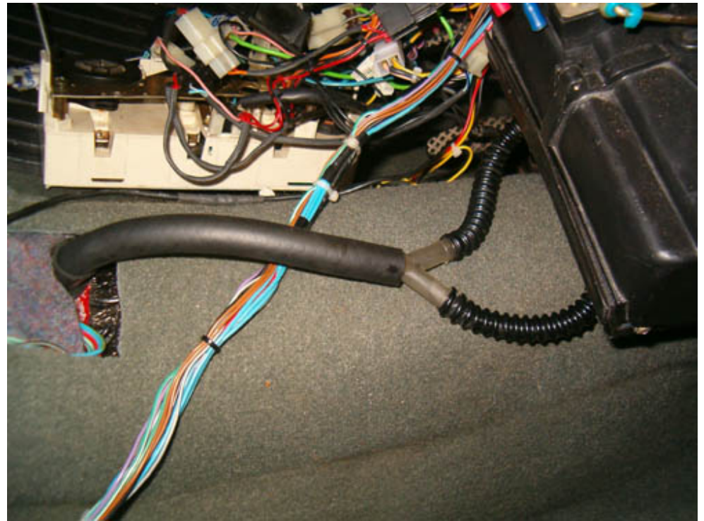
Drain plug is in place and connected to the evaporator.
