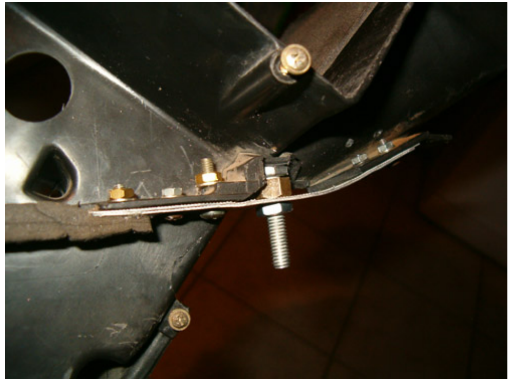
One of the four support points of the unit broke during removal from the donor car, so I had to fabricate one...
