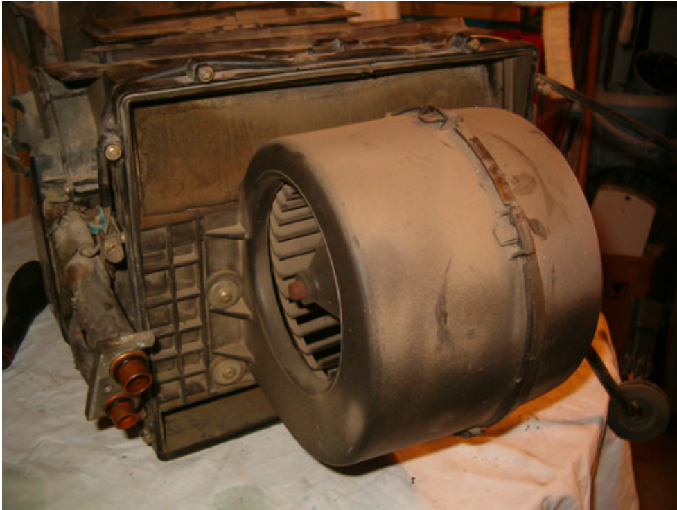
Blower motor exposed ...
