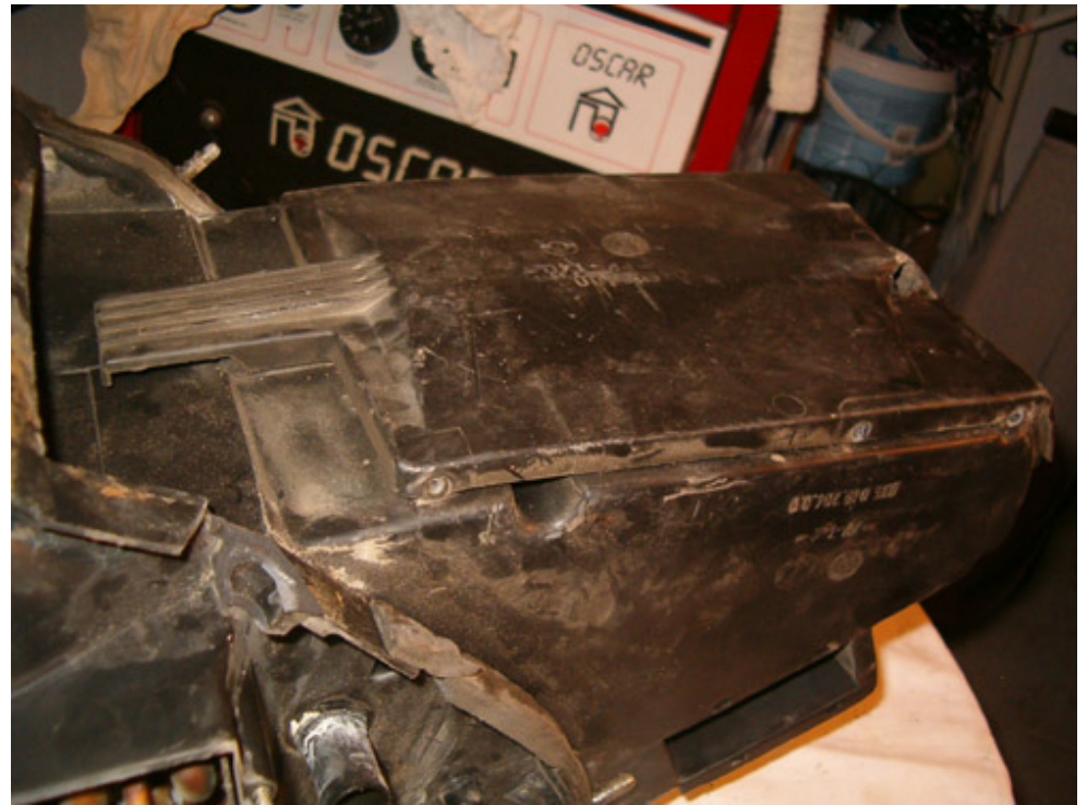
Remove lower plate. This is actually the drain plate of the evaporator
