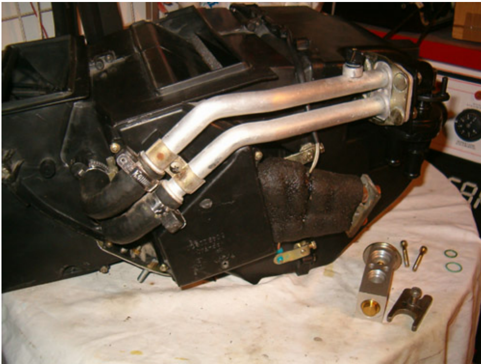
Heater matrix pipes are in place and new expansion valve is installed along with new O-rings all intended for use with R134a.
