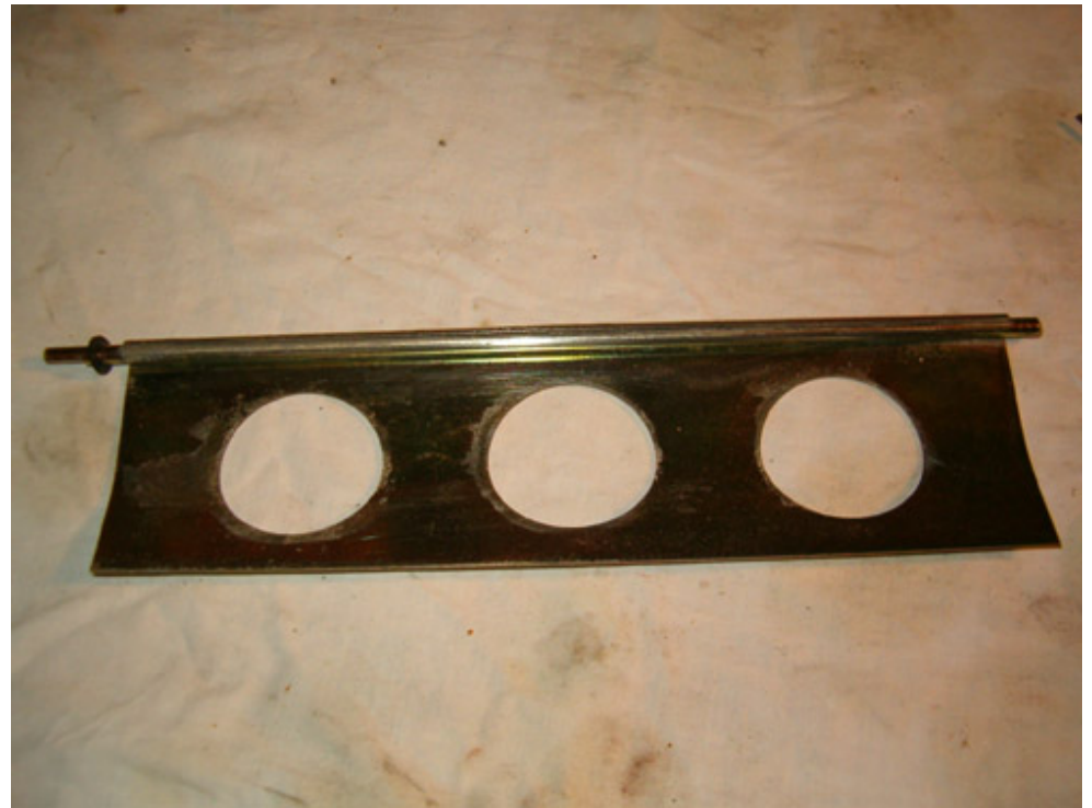
Air direction flap after cleaning. Be sure to remove every trace of old glue.
