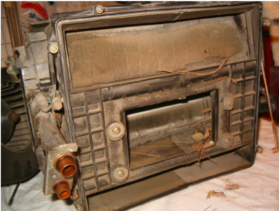
Notice the interior/exterior air circulation flaps. The foam material is collapsing!
