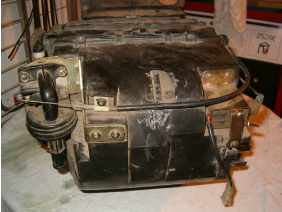
Front view. Notice the big opening and the broken lever of the coolant cut off switch.
