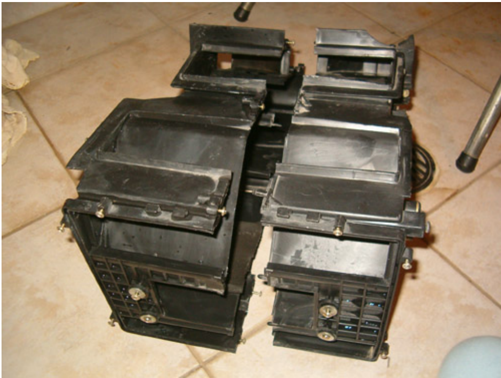
Evaporator half covers after thorough cleaning...
