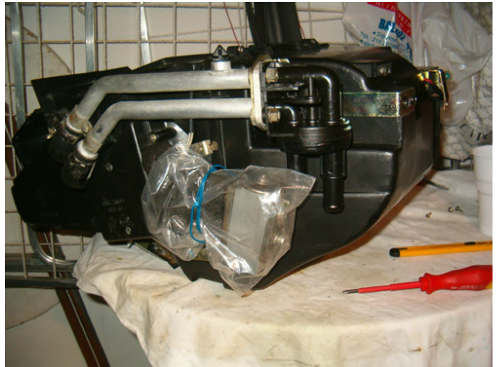
Cover the expansion valve since it should be free of dirt or dust in order to function correctly.
