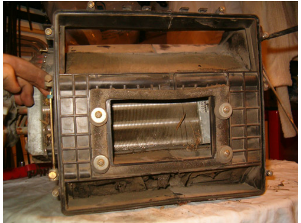
Notice the interior/exterior air circulation flaps. The foam material is collapsing!
