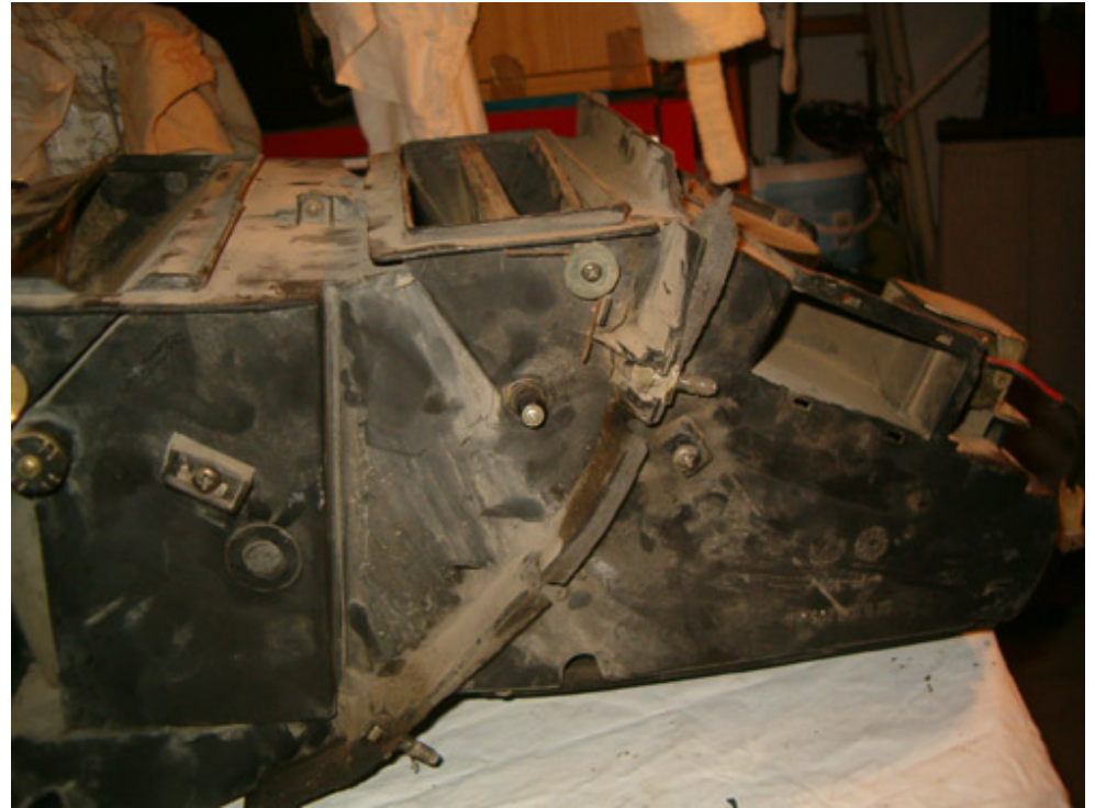
Side views showing servo motor regulating interior/exterior air circulation, blower motor resistor, power connectors, air flow direction ducts.
