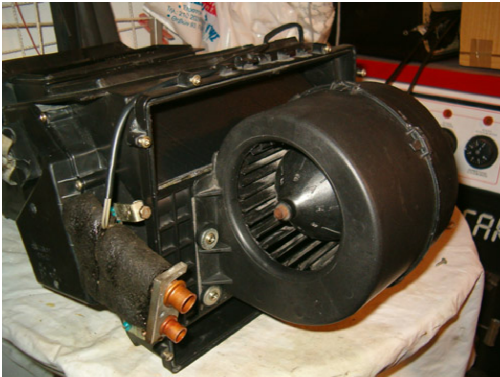
Blower motor is in place.
