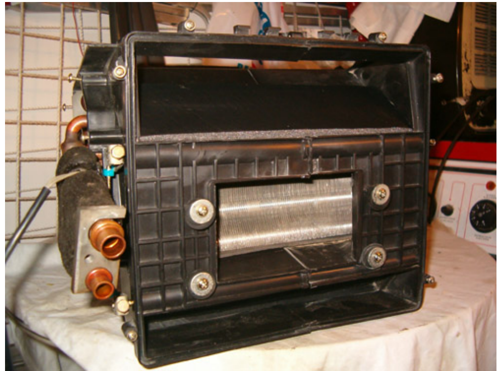
Front part showing evaporator, air flow flaps, and evaporator pipes
