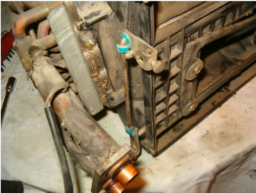
Don't forget to remove the servo motor actuating rod for the interior/exterior air circulation flaps
