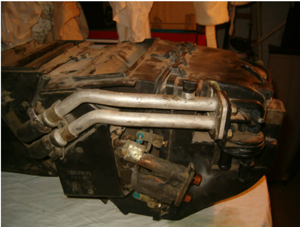
Side view showing A/C and heater piping. Upper pipes are for the heater matrix and lower pipes are for the A/C evaporator.
