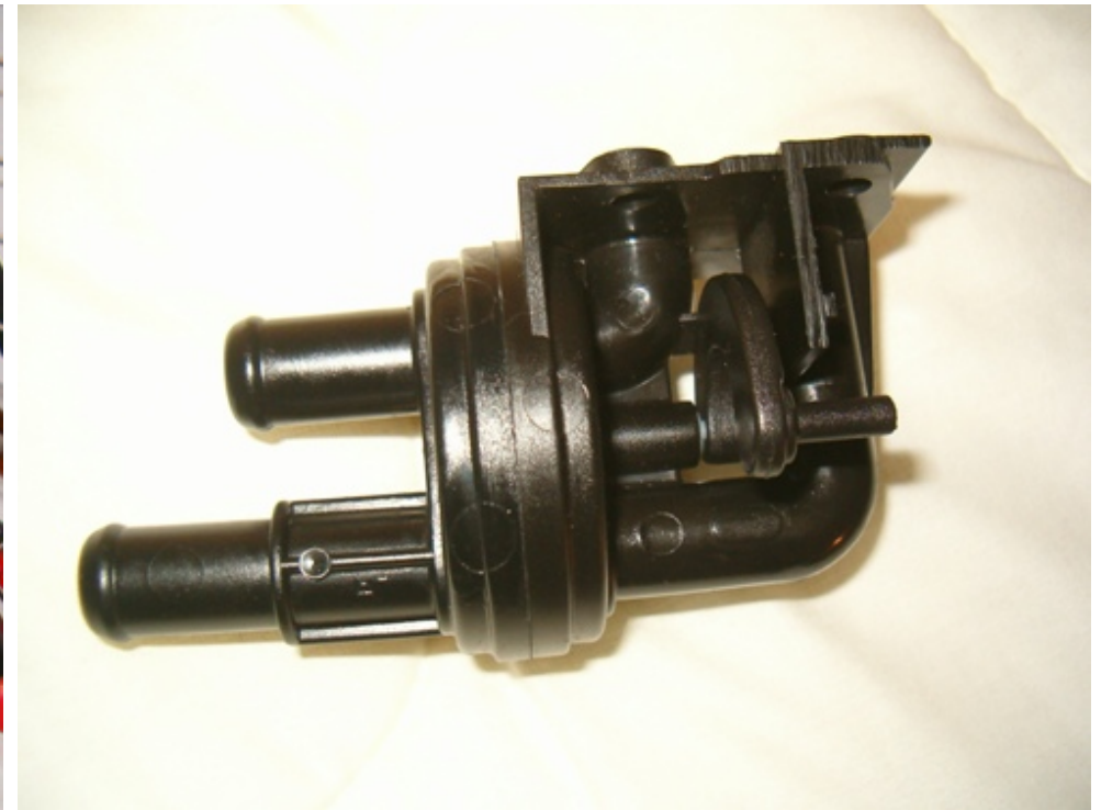
New coolant cut off switch
