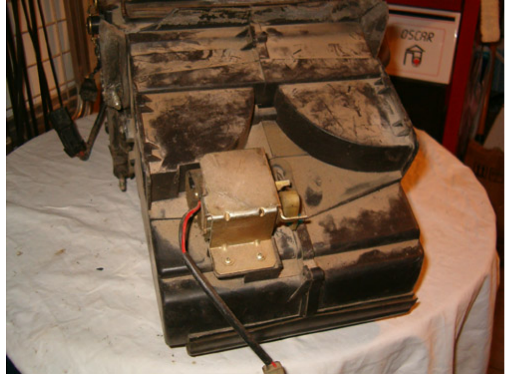
Rear view showing hot/cold air servo motor and air flow direction ducts (feet)
