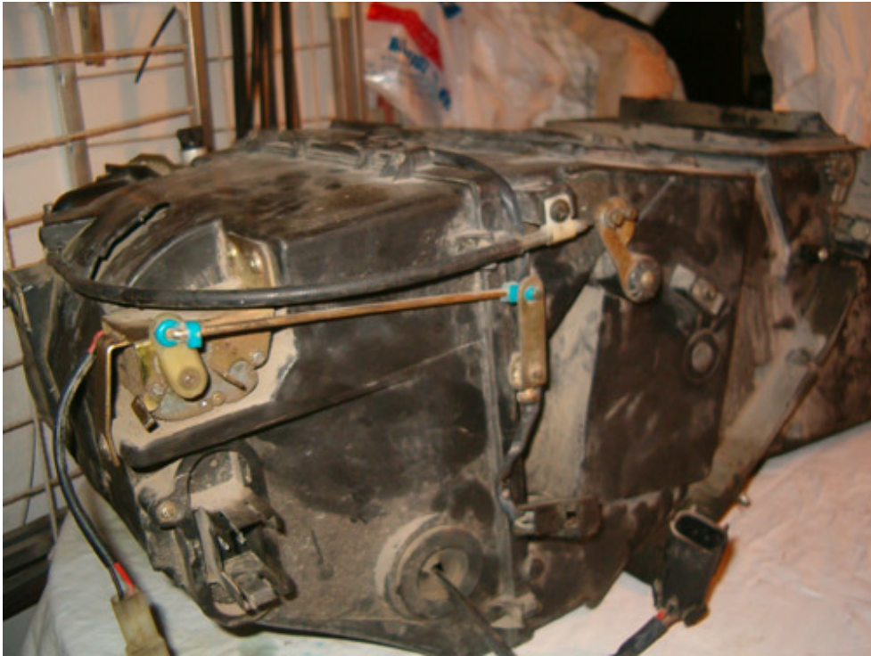
Side views showing servo motor regulating interior/exterior air circulation, blower motor resistor, power connectors, air flow direction ducts.
