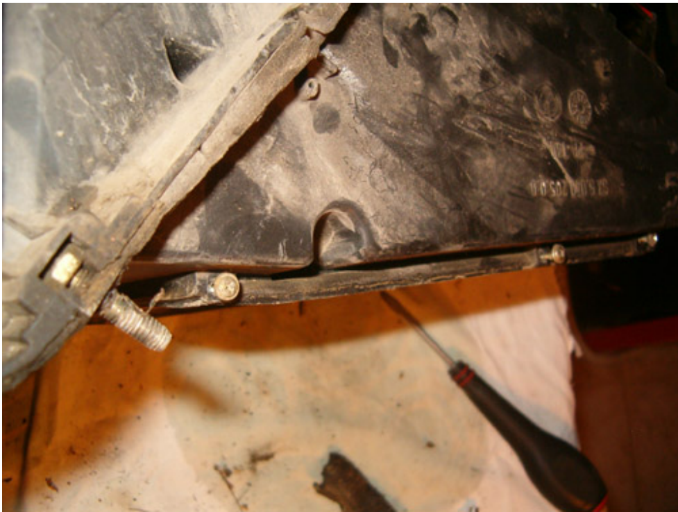
Remove lower plate. This is actually the drain plate of the evaporator
