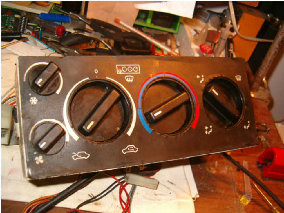
Here is the control panel as taken out of the donor car. The fascia will surely need a good cleaning
