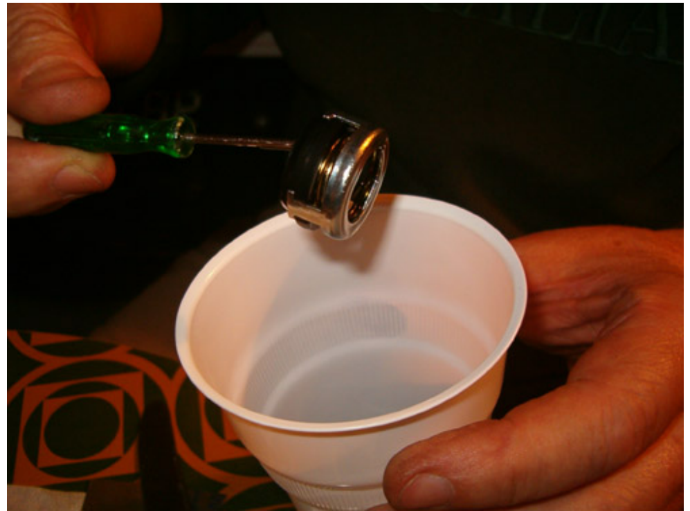
Be sure to dip both parts into clean ester oil
