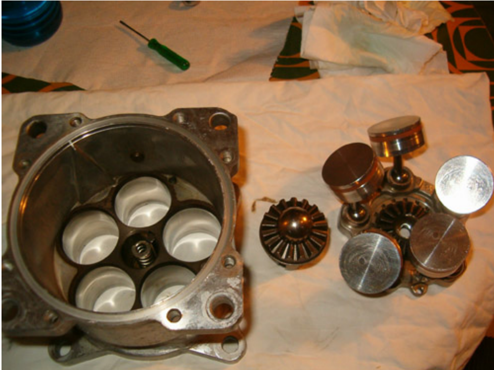
left to right: compressor body, piston shaft, piston assembly
