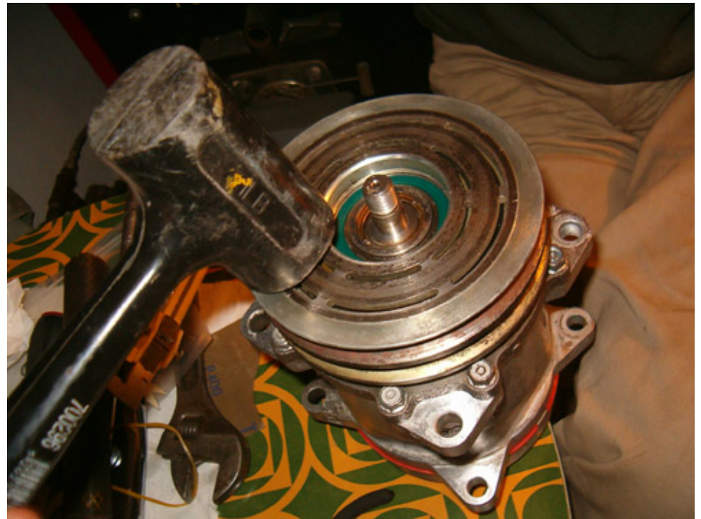
Punch the pulley with the rubber hammer in order to fit in place ...
