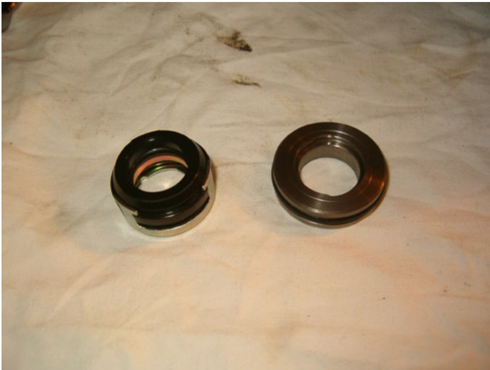
New shaft protective seal (left) and lip seal with O-ring (right)
