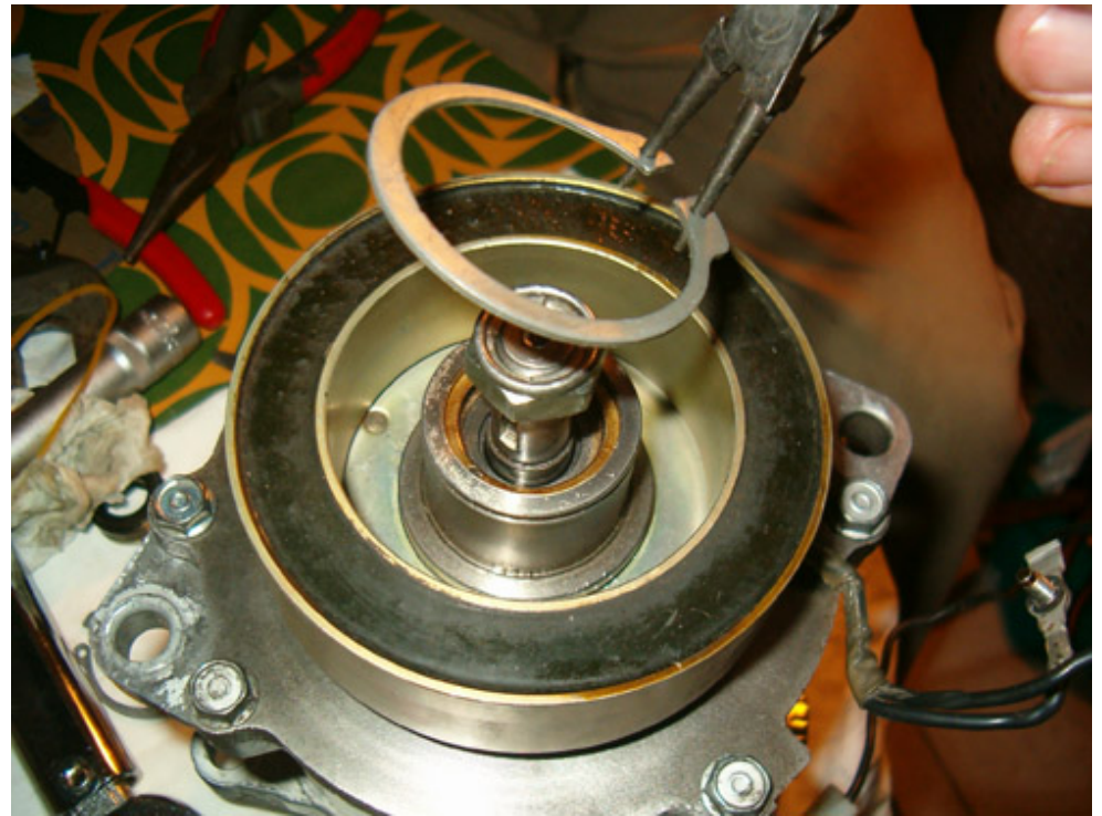
Mount the electromagnetic coupling with the respective lock ring ...
