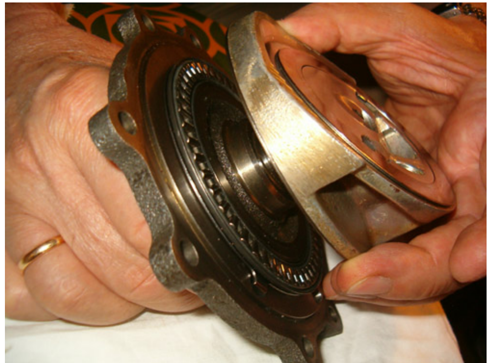
Insert shaft into front part body. Be careful not to miss the bearing
