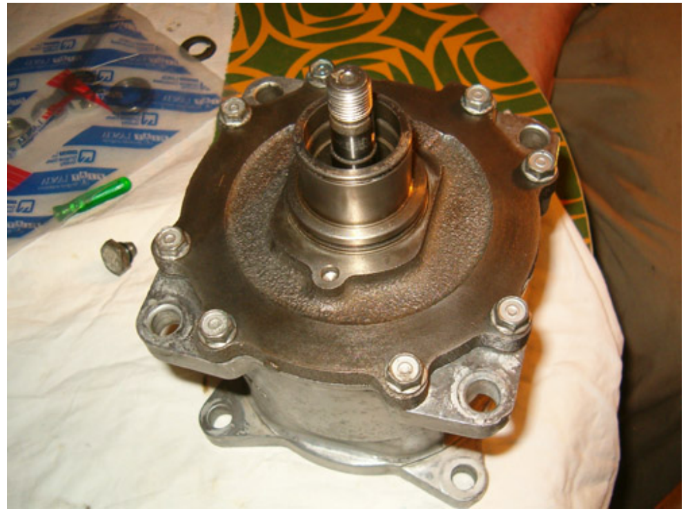
Gradually tighten the screws in cross order
