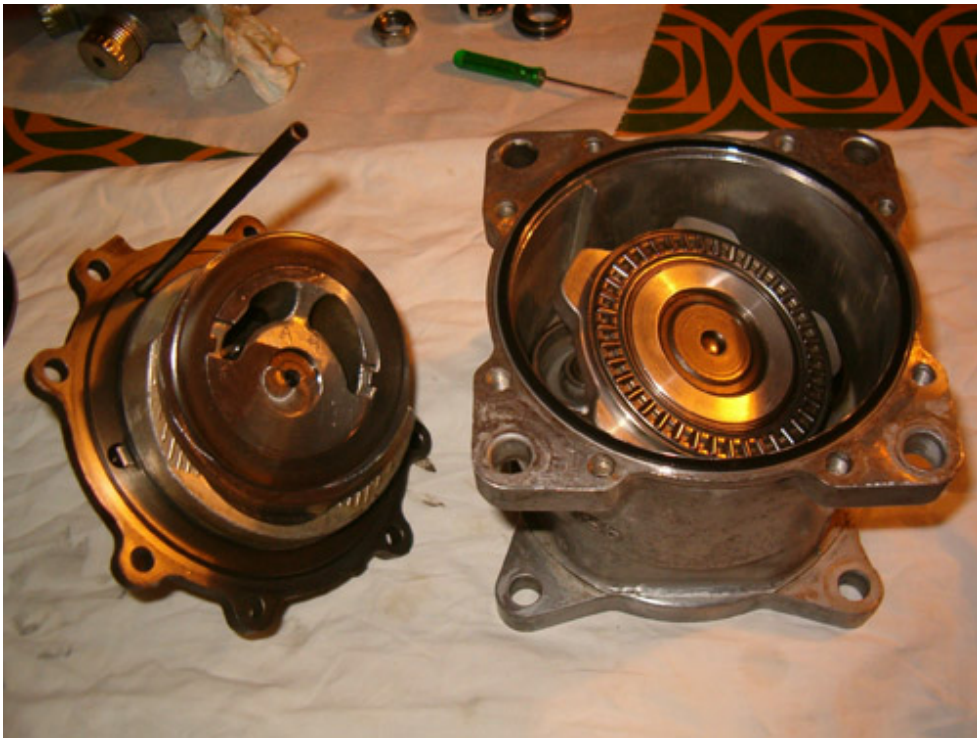
Install new gasket on compressor body and apply some drops of clean refrigerant oil in the groove
