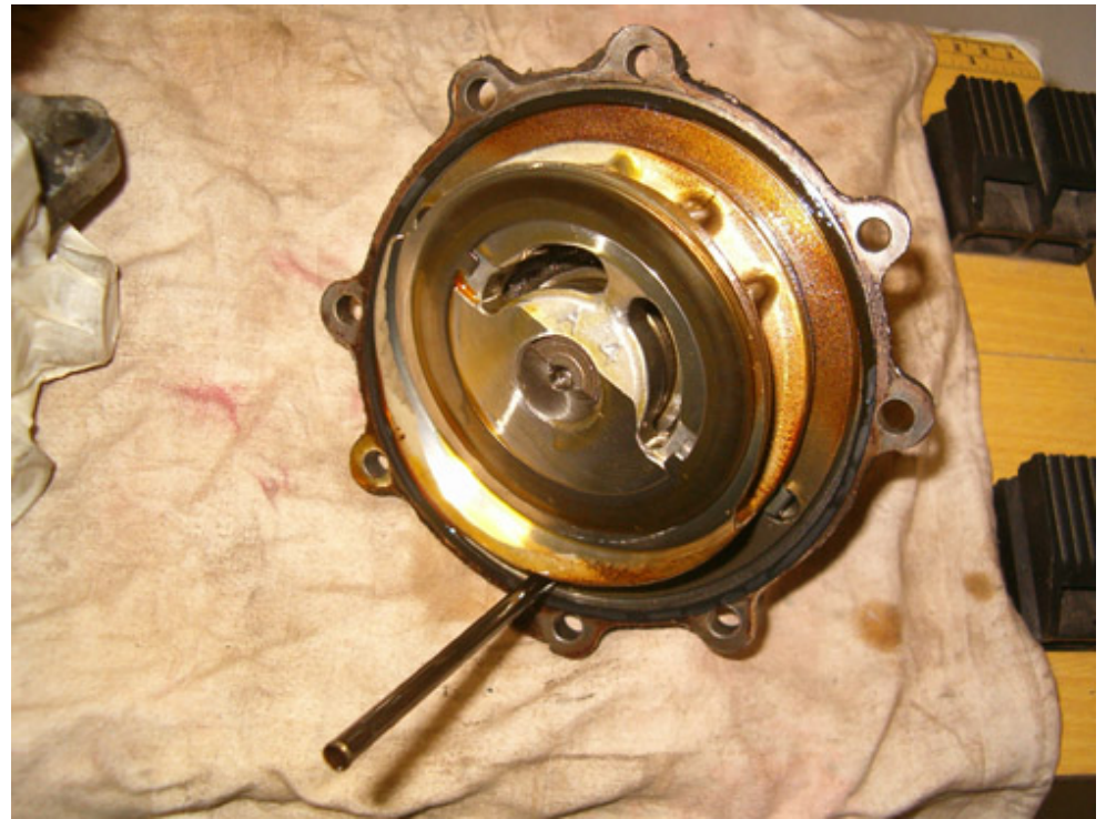
Compressor front part, also slanted. Notice the rod on the bottom; this is intended as an alignment guide to the compressor body.
