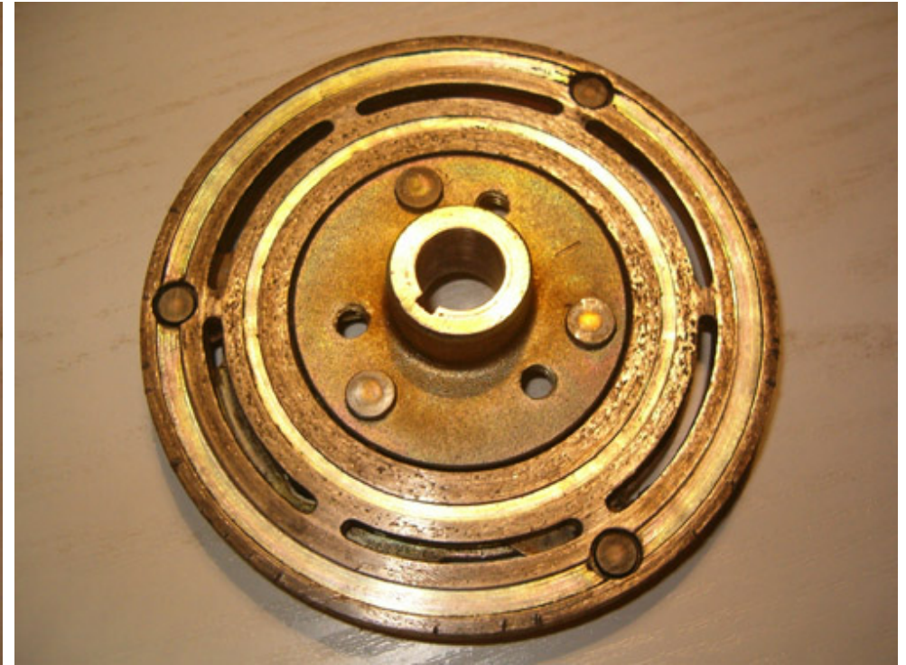
Compressor shaft plate cleaned out (front and back view)
