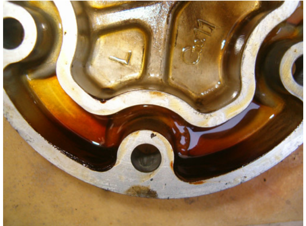
... and clean out oil residue using alcohol (never use petroleum based solvent)
