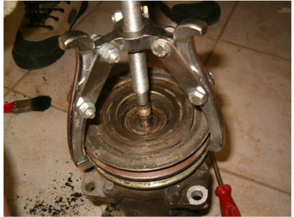
Using the puller lift out belt pulley.
