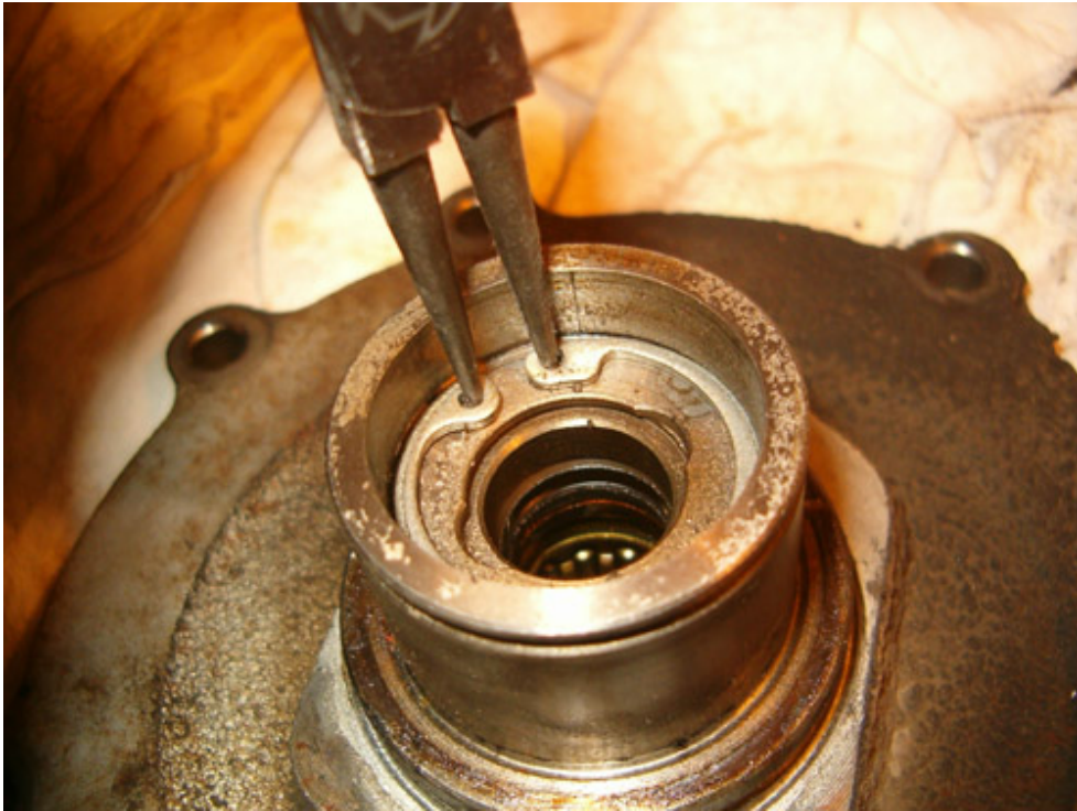
Using expanding pliers remove lock ring ...
