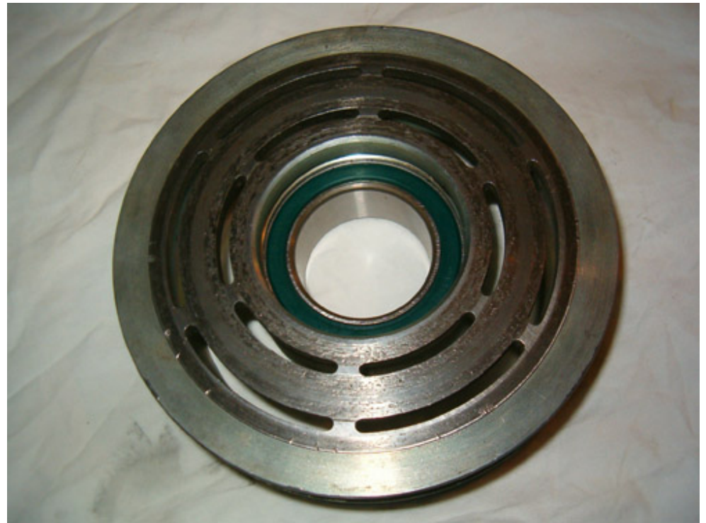
Compressor pulley fitted with new bearing since the old one had excess play and wobble (front and back view)
