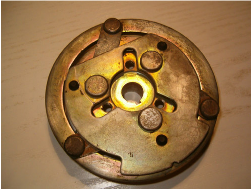
Compressor shaft plate cleaned out (front and back view)
