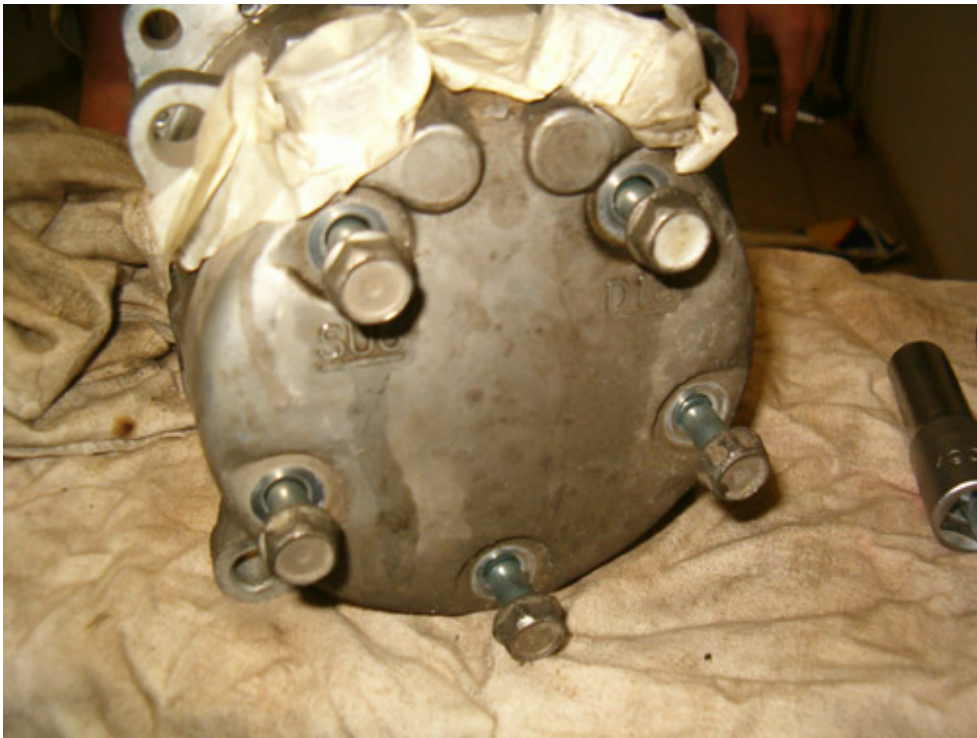
Let's now remove compressor cylinder head (13 mm key is required)
