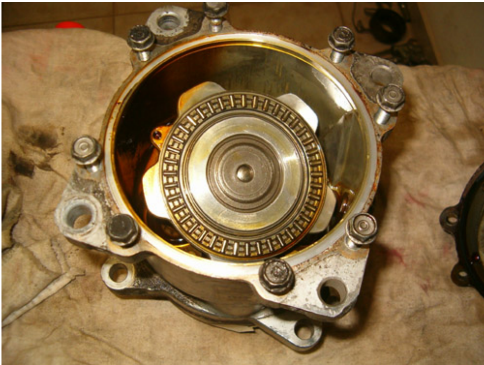
This is the first thing you see when you remove compressor front part. Notice that the piston assembly is slanted. This is so because the pistons are operating one at a time.
