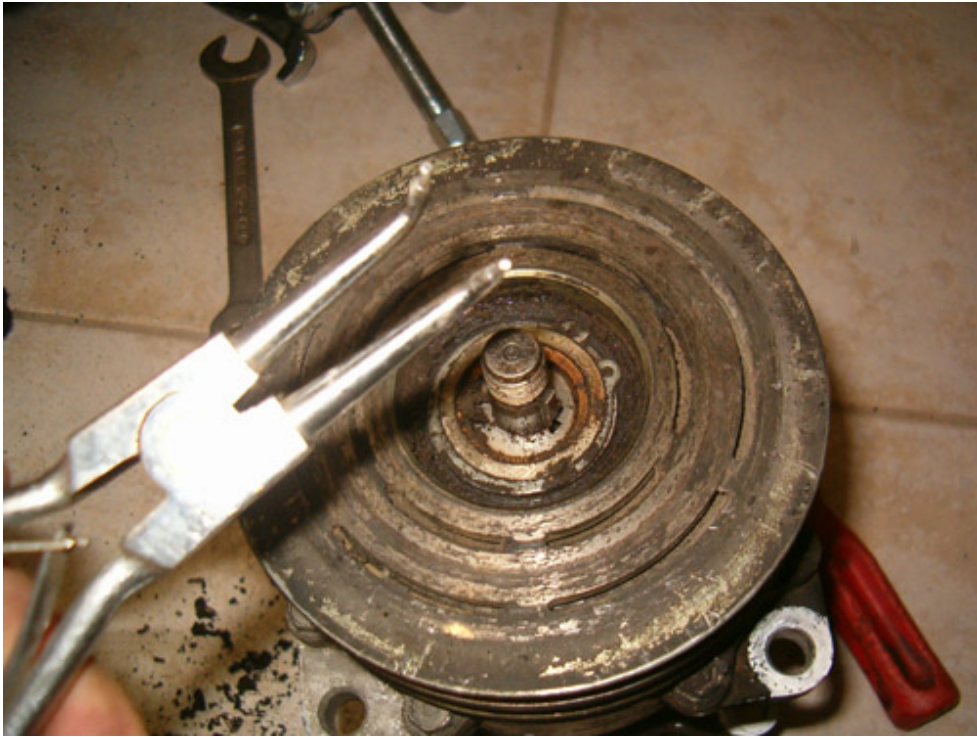
An expanding pliers will help you remove the lock ring securing belt pulley to body.
