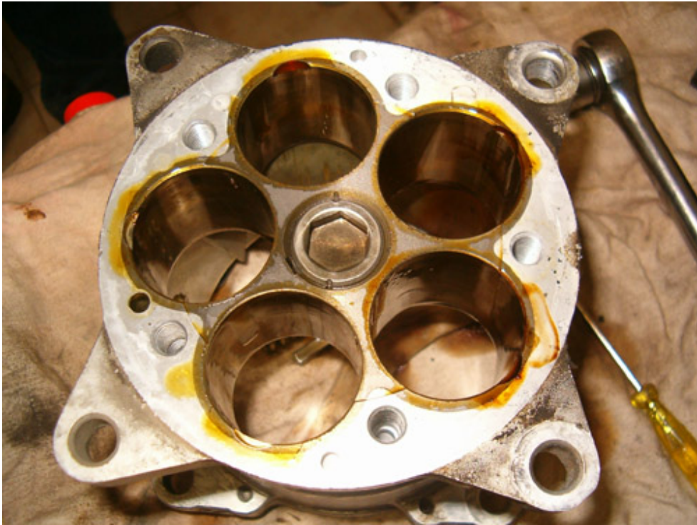
Back view of compressor body.
