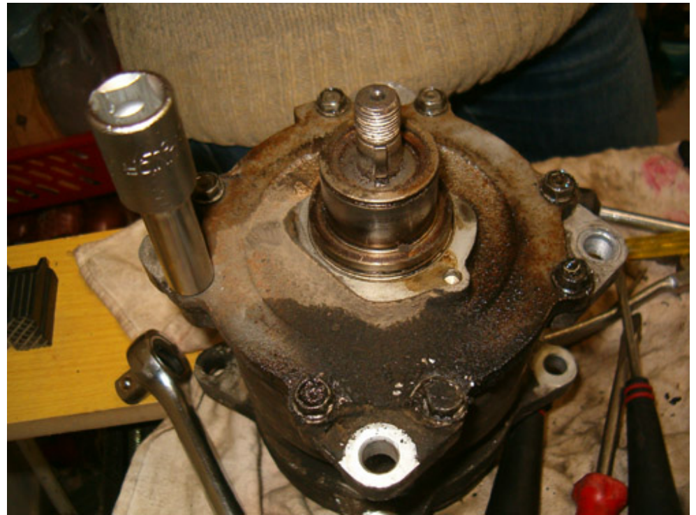
Using a 10 mm key remove the compressor front part
