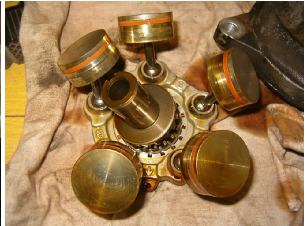
Piston assembly. Notice the yellowish color on each piston; these are traces of refrigerant oil which has come in contact with atmospheric air. This reaction leads to an awful thick residue.
