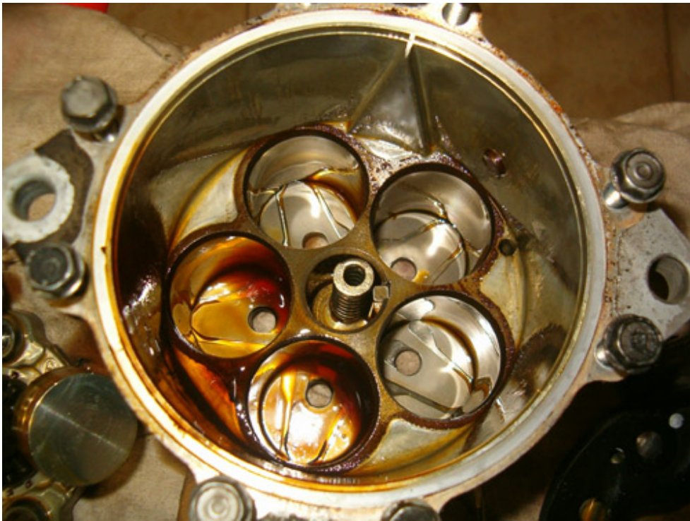
Compressor body as seen with piston assembly removed
