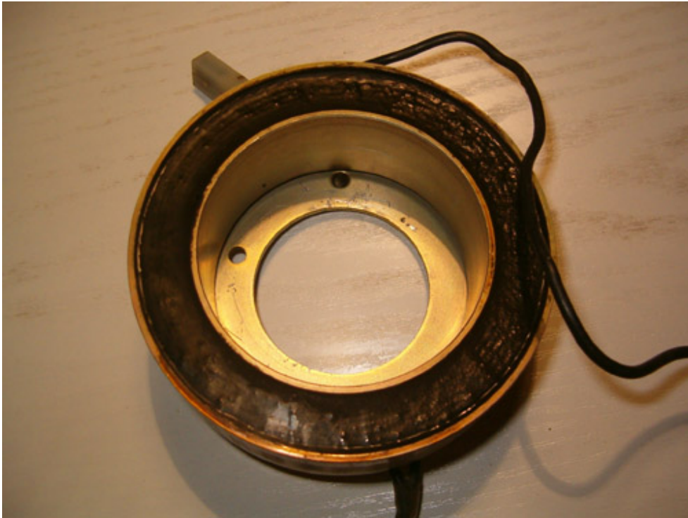
Here you can see the electromagnetic clutch which actually triggers compressor operation (front and back view)
