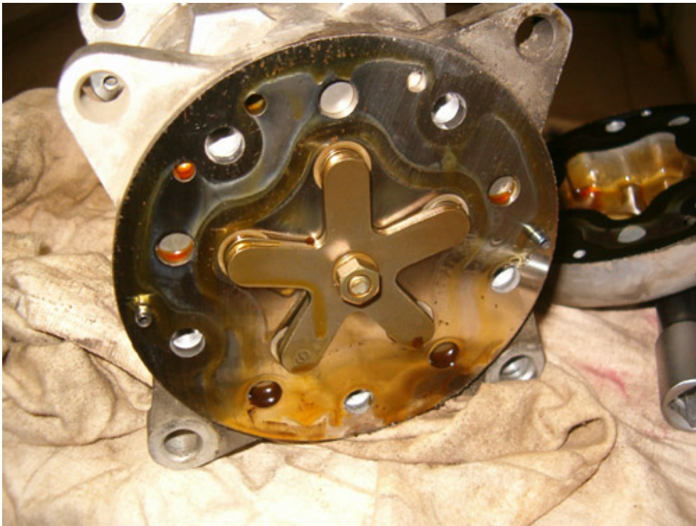
Here is the valve plate assembly
