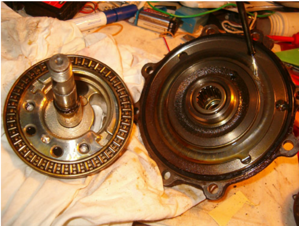
Shaft on the left complete with bearing, front part body on the right.
