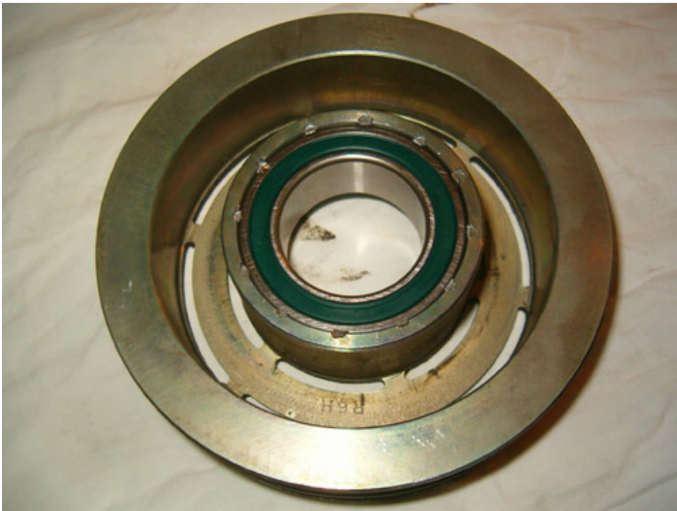
Compressor pulley fitted with new bearing since the old one had excess play and wobble (front and back view)
