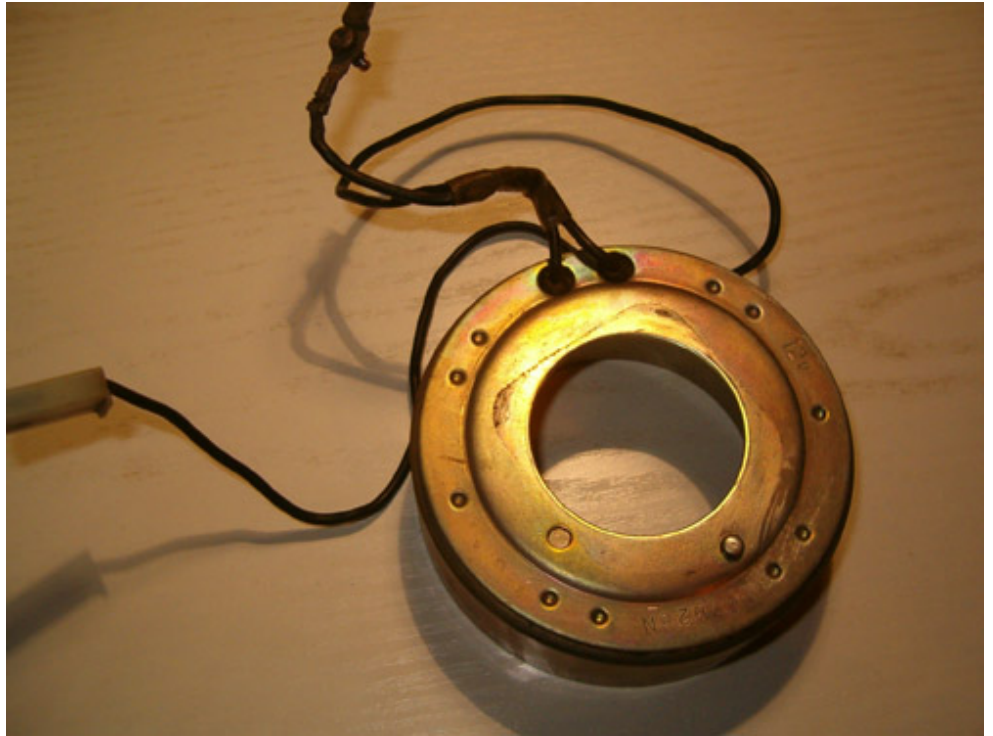
Here you can see the electromagnetic clutch which actually triggers compressor operation (front and back view)
