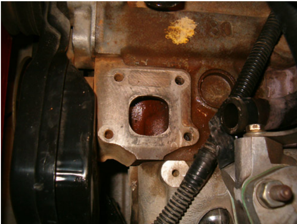
Using a blade scrapper clean up the area where the O-ring will sit upon
