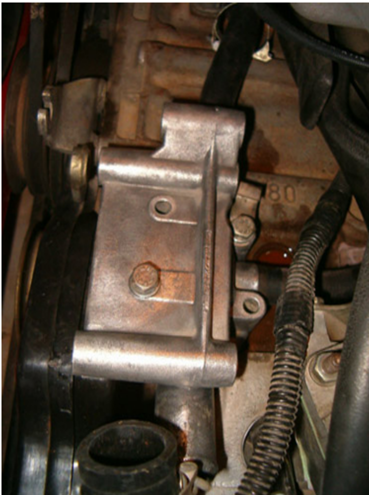
Install bracket on engine block and tighten the screws in cross order.
