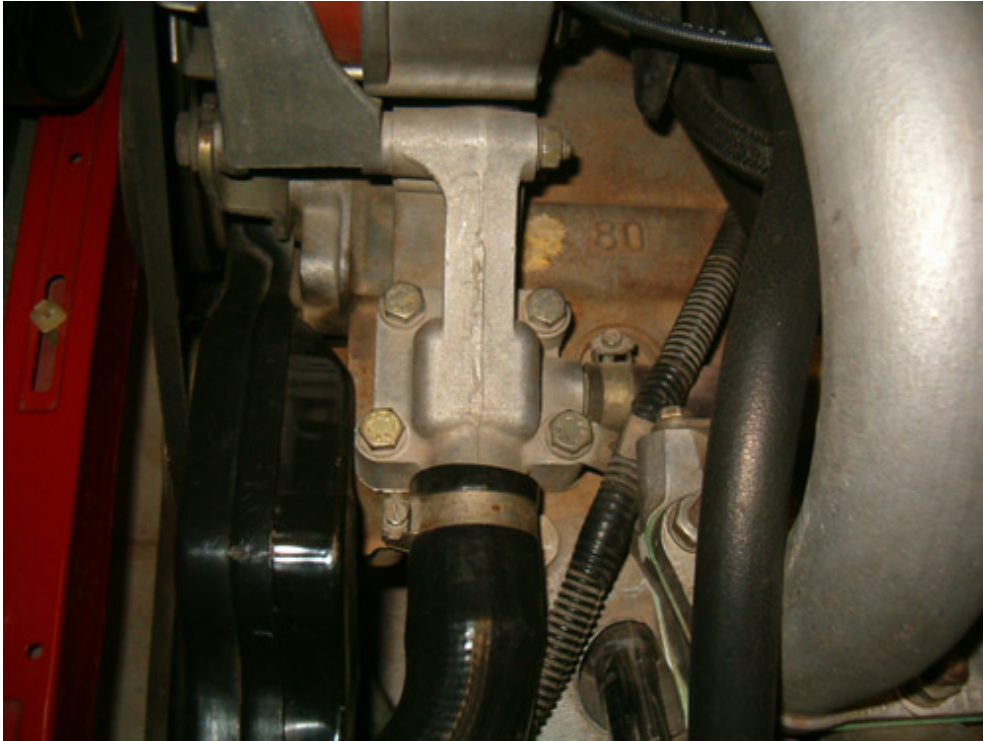
Standard union found on non A/C equipped cars
