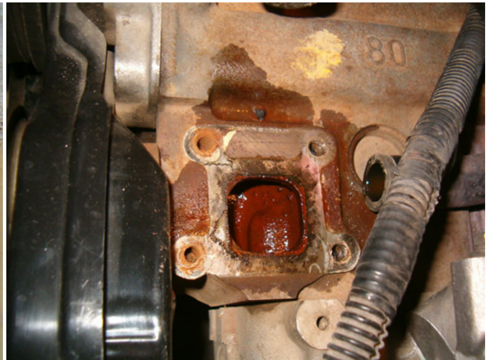
Traces of the rectangular gasket on engine block.
