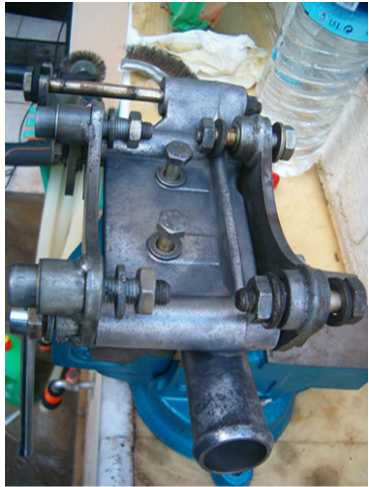
Back in shiny color after wire brushing ... almost like new!
