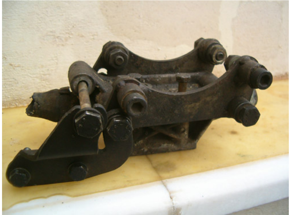
Bracket as taken out as a whole part from the donor car
