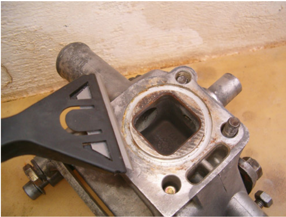
and remove residual dirt with the blade scrapper
