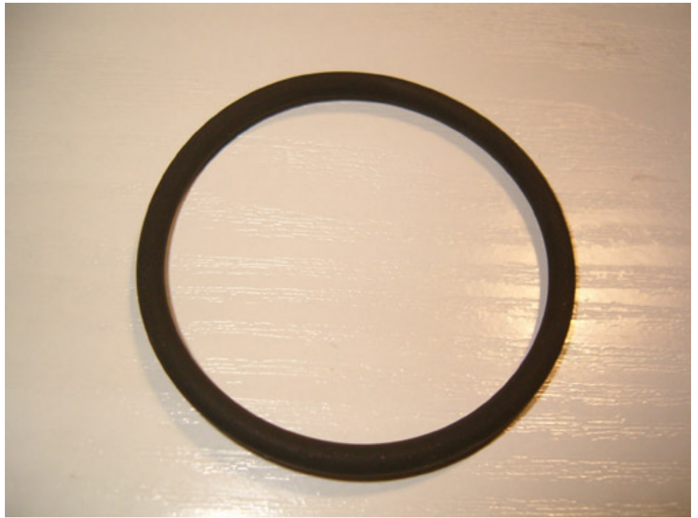
Use new O-ring (part number 14464381) for the bracket.
