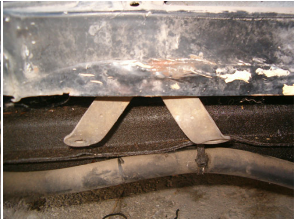
Horns bracket. A very important element since the horns will be moved to the front cross rail.
