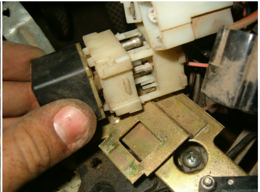
blower motor relay...
