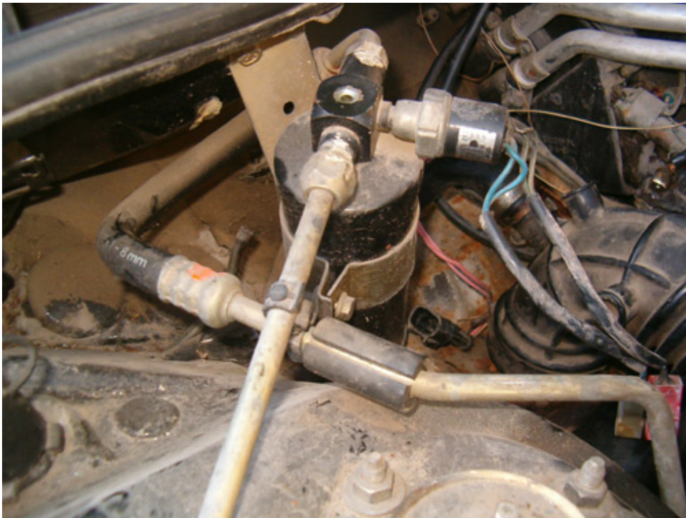
Drier filter and Trinary pressure valve demonstrated
