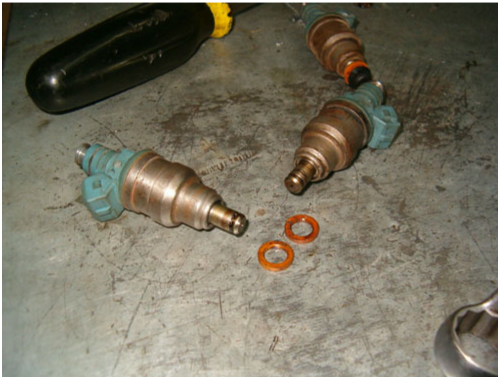
The tips are just plastic hat looking elements which are pressure fitted and it is advisable to discard them and install new ones.
