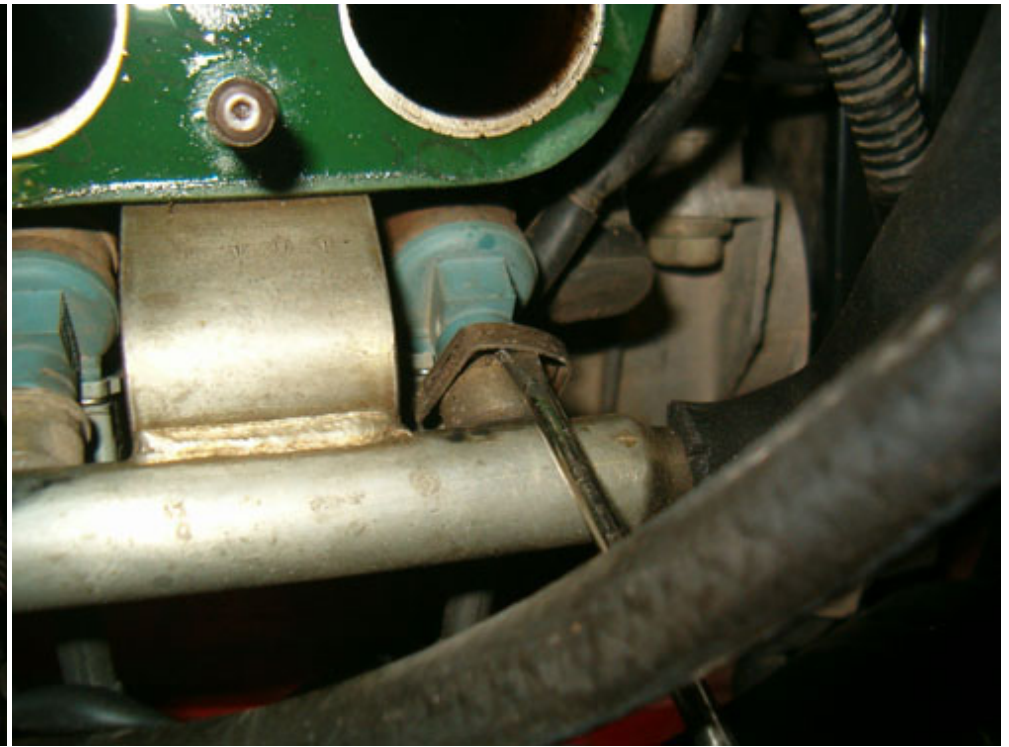
Using a flat screwdriver remove the clip securing injector to fuel rail
