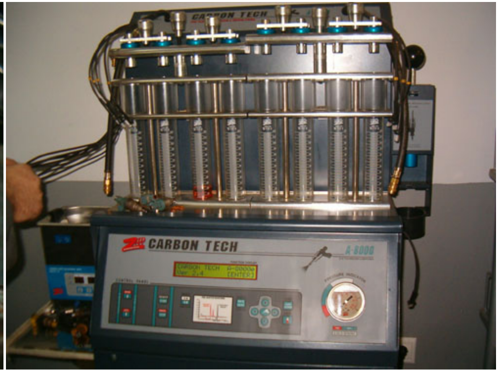
This is the injector cleaning device. It uses the supersonic method to remove combustion particles and debris from the internals of the injector.
