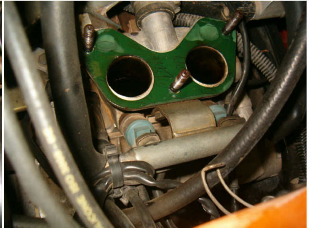
Now you have plenty of room to work on the fuel rail and injectors
