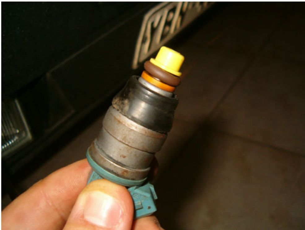
Here you see the already cleaned injector along with its new tip and O-ring.
