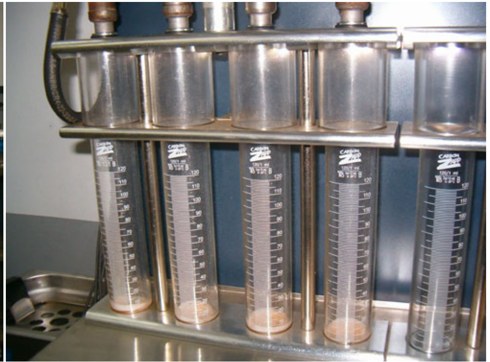
These test tubes are scaled and the prerequisite for the injectors to pass the test is that all four should yield the same volume of fluid.
