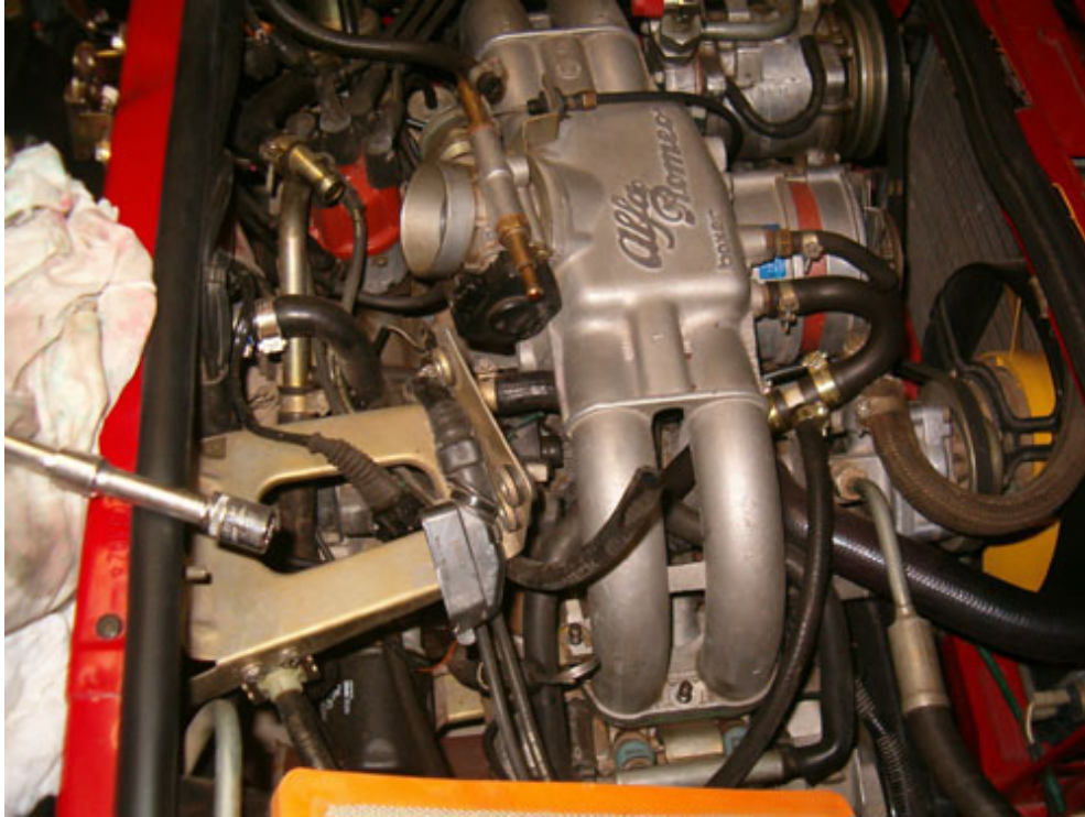
Remove ECU, corrugated sleeve and respective coolant hoses
