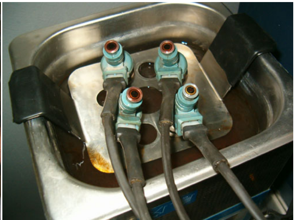
...and submerges the injector tips in the cleaning solvent.
