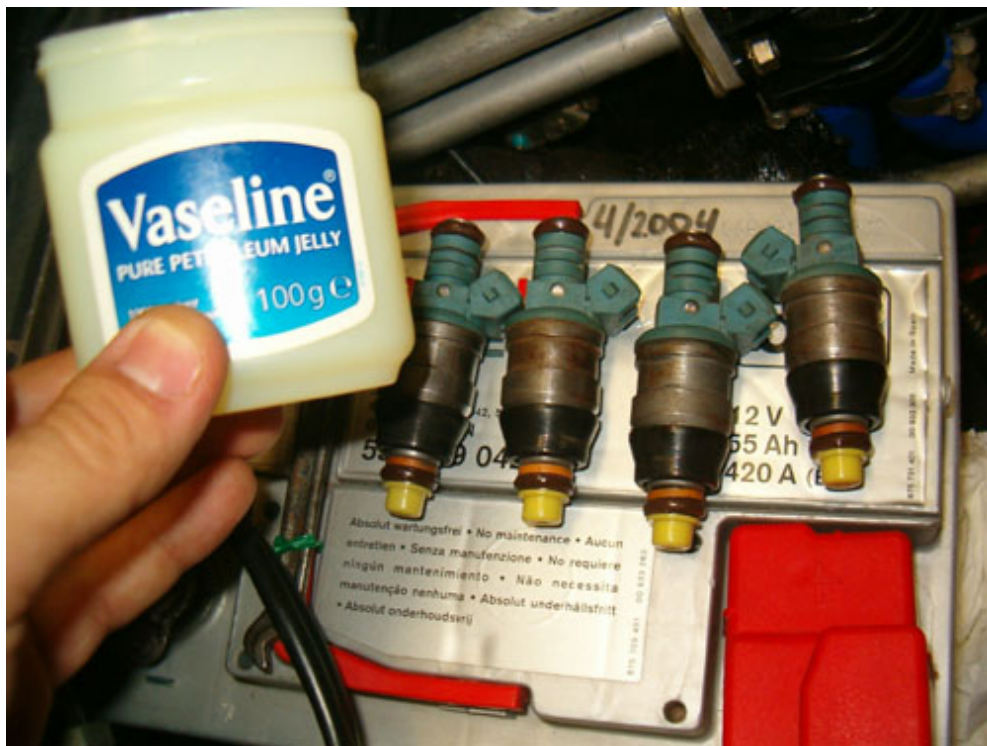
... and use vaseline at the O-rings. It will ease your life during installation.
