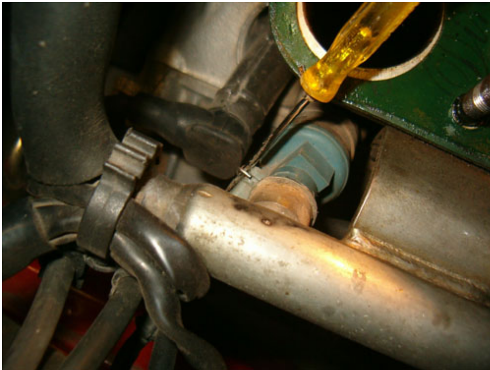
Using a small flat screwdriver remove the metal clasp in order to separate injector from socket
