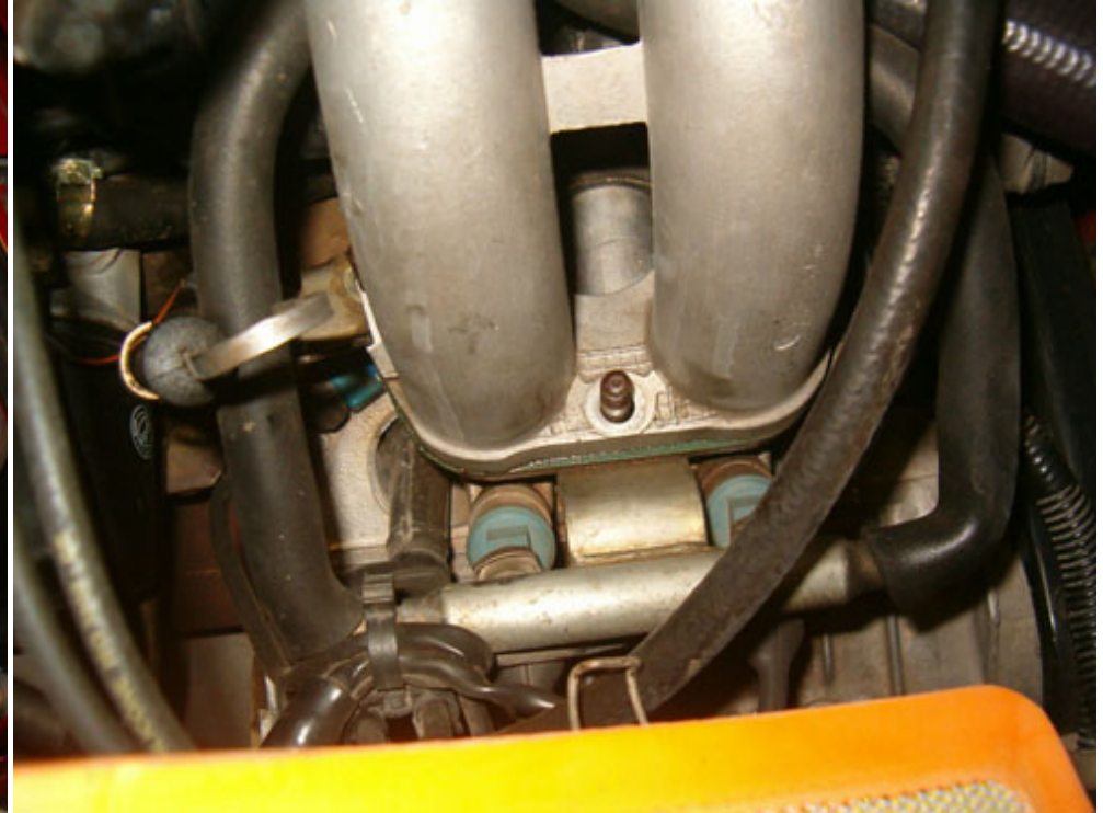
Undo three nuts securing plenum to intake manifold for the right side ...
