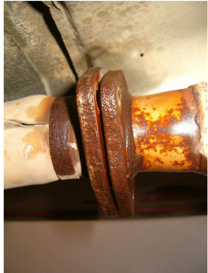
... undone the tree screws keeping together catalyst and exhaust manifold. Note the high rust deposits on the connection and the screws.
