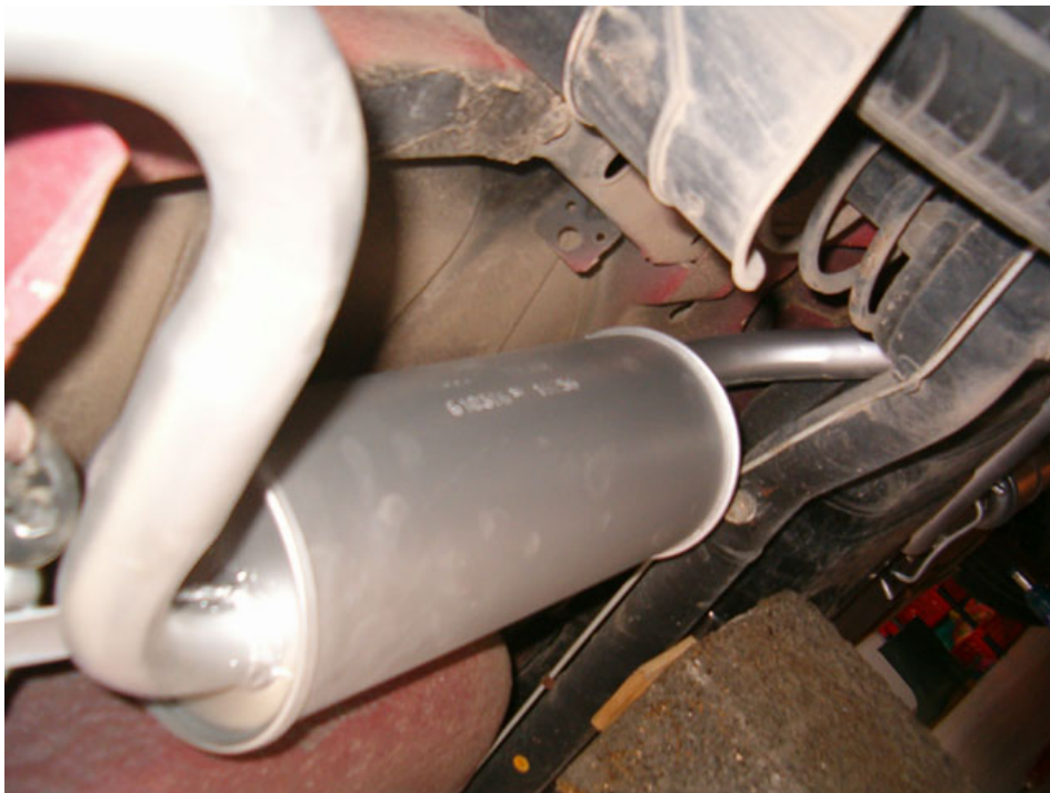
Rear silencer is now installed
