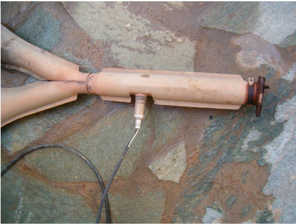
a close-up of the lambda sensor portion of the exhaust ...
