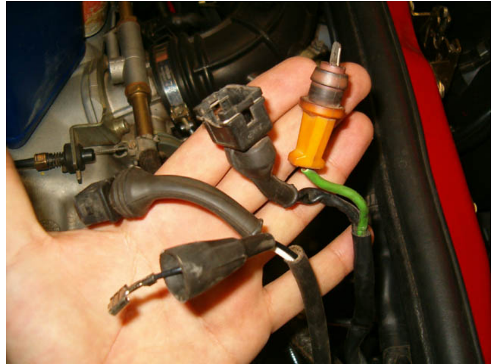
and then disconnect lambda sensor wiring.
