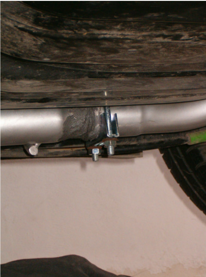
The pipes are now connected and kept in place with the clamp
