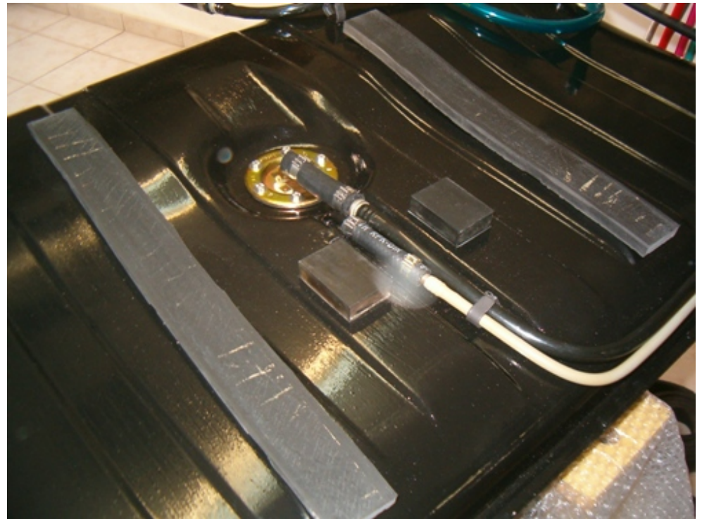
This is the final look of the tank upper side. Two long rubber strips and two smaller ones preventing the fuel lines from touching the floor. Also the blueish hose seen on the right of the tank is the fuel relief hose intended to remove air from the tank during refuelling.
