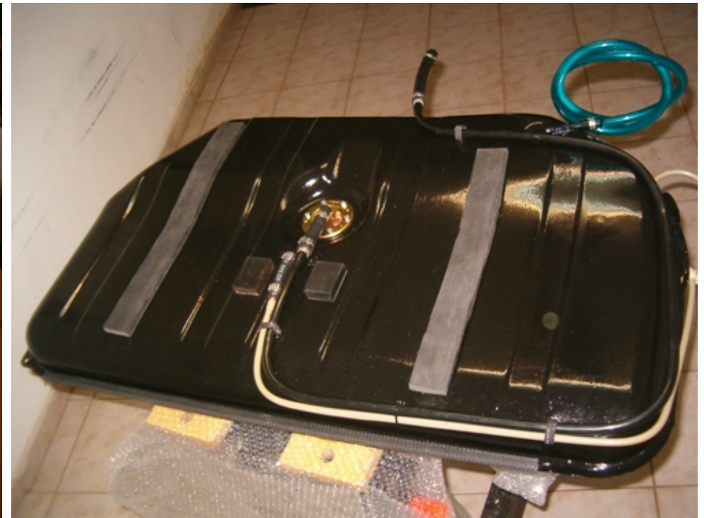
Tank is now ready for installation. It will be a bolt on job by removing the temporary one and installing this one directly.
