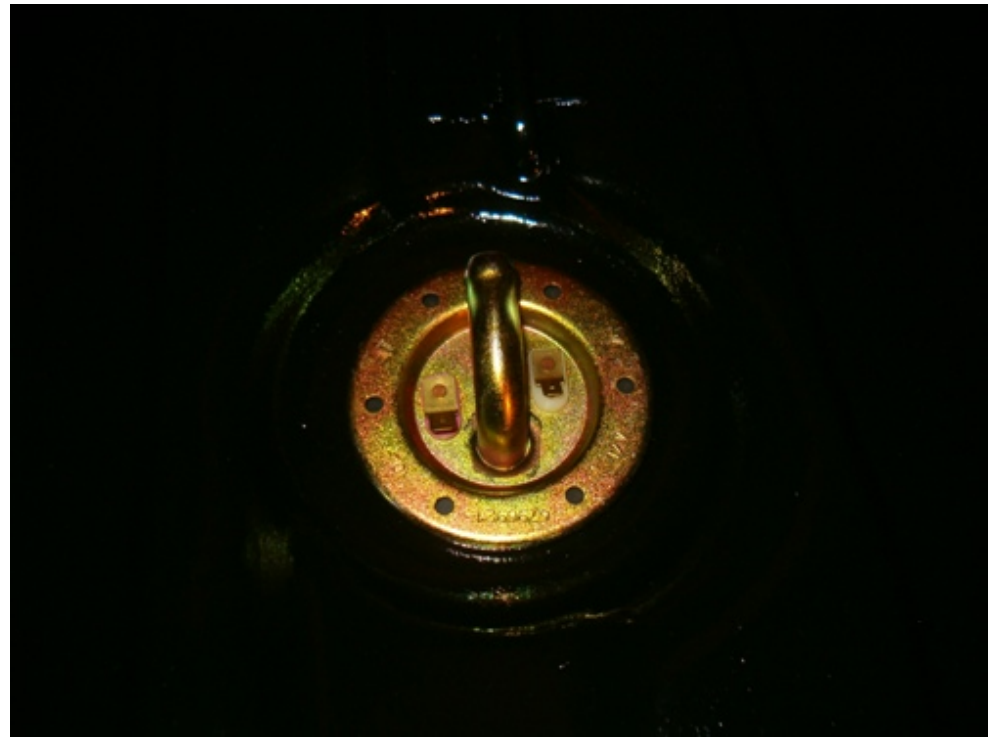
and finally position the sender unit to the correct place.
