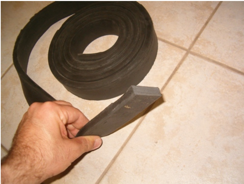
Rubber stripe like in the photo above needs to be installed on the tank upper side. This is the surface that is placed against the floor.
