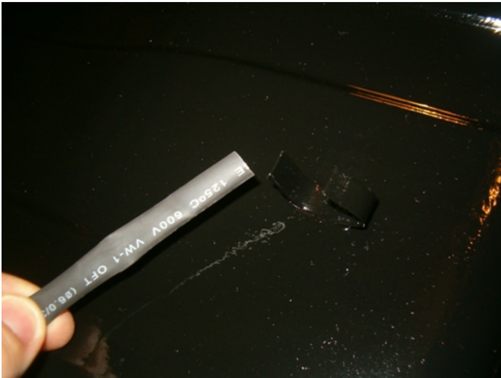
Use a shrink tube so that the the metal keepers do not ruin the fuel lines
