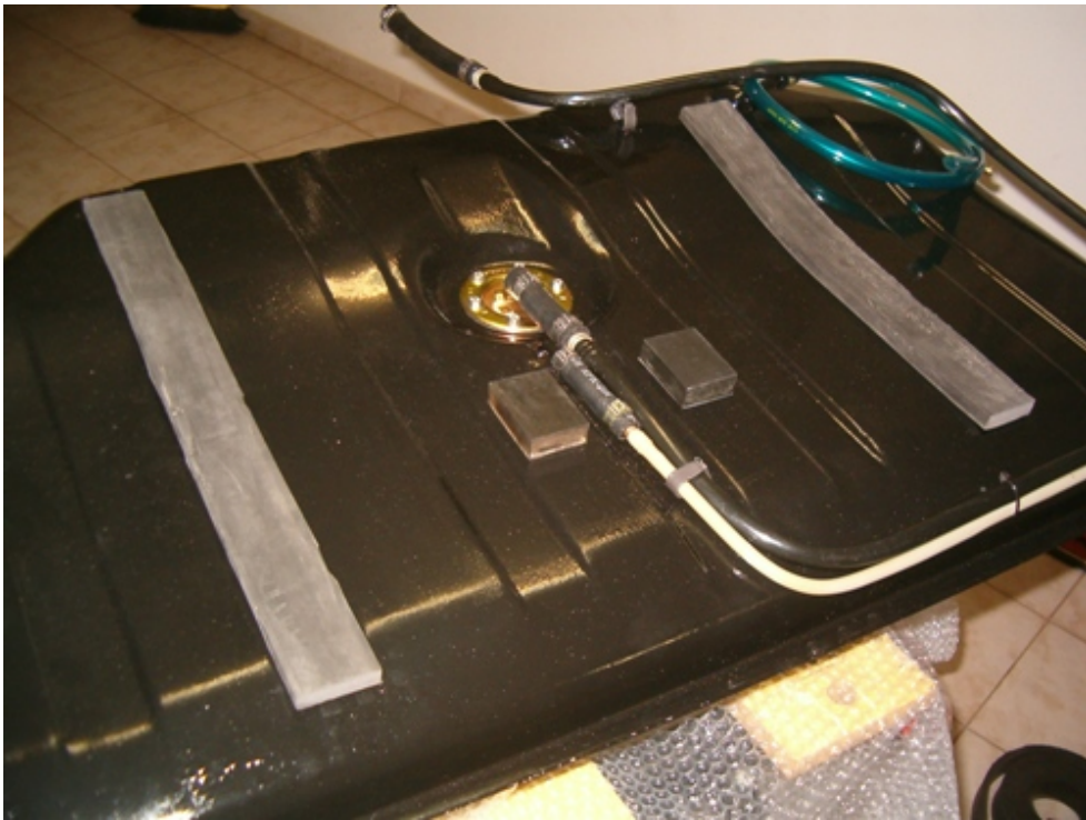
This is the final look of the tank upper side. Two long rubber strips and two smaller ones preventing the fuel lines from touching the floor. Also the blueish hose seen on the right of the tank is the fuel relief hose intended to remove air from the tank during refuelling.
