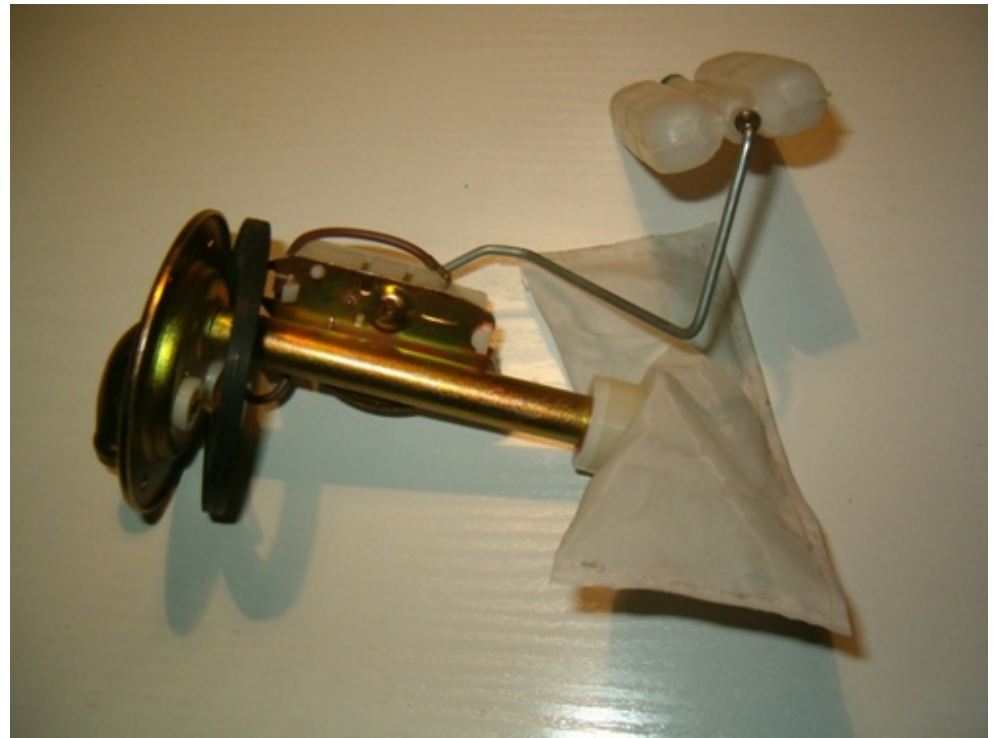
I was lucky to find in Italian eBay a new fuel sending unit. These items have become extinct many years ago.
