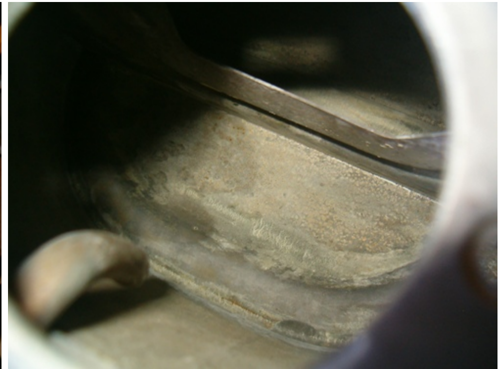
With the aid of a high pressure air blower and a hair drier the tank is now completely dry and ready to accept tank sealer.
