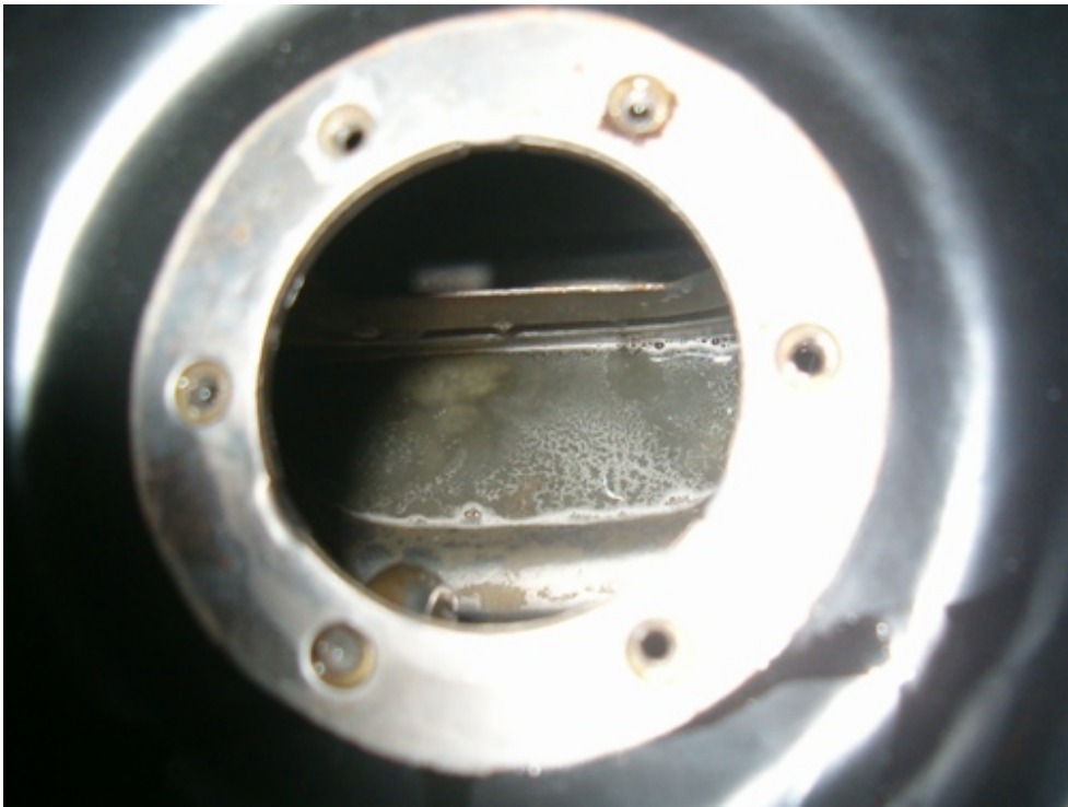
Metal Ready has turned from blue to clear and it will soon take a brown color meaning rust is eaten away.
