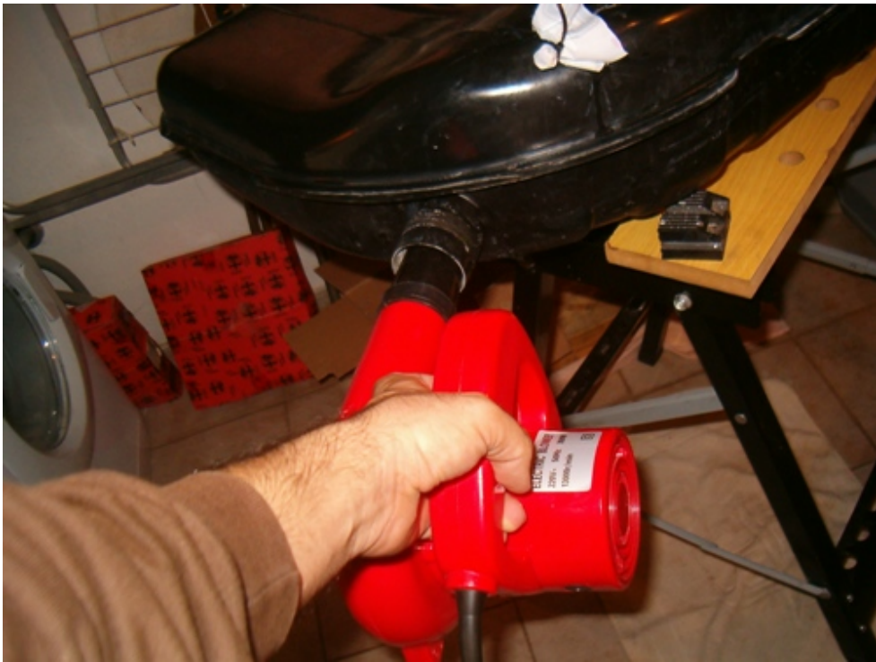
With the aid of a high pressure air blower and a hair drier the tank is now completely dry and ready to accept tank sealer.
