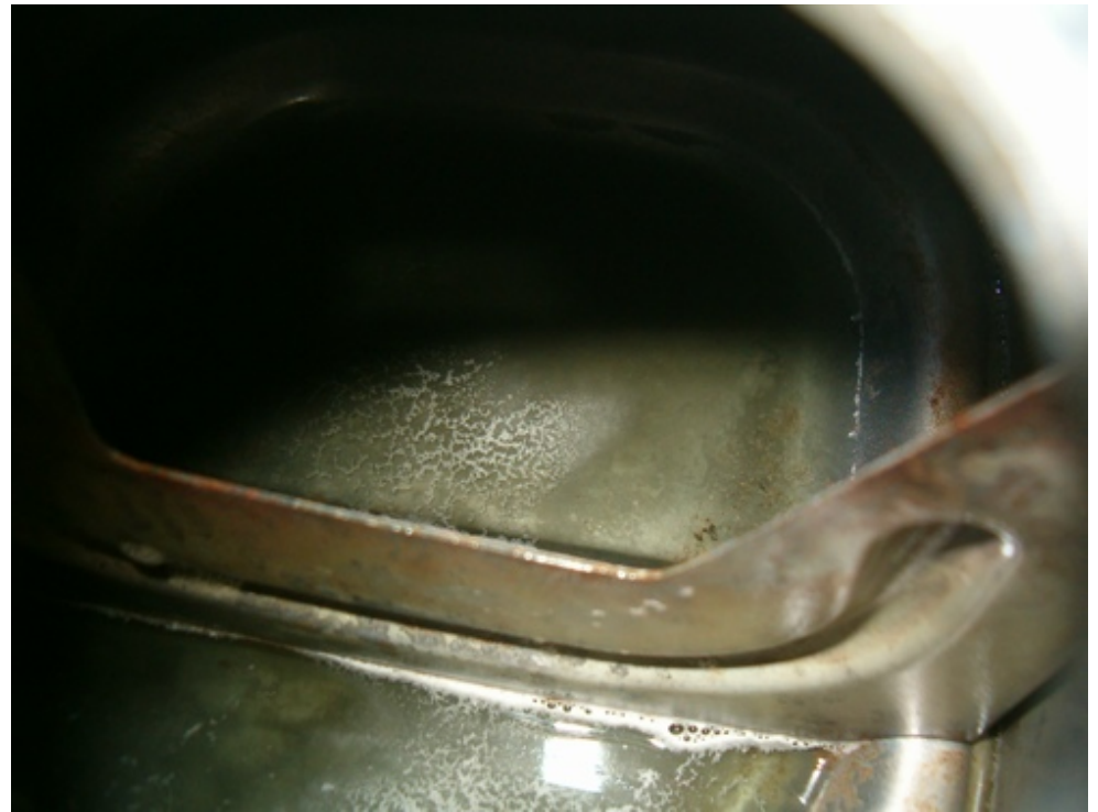
Metal Ready has turned from blue to clear and it will soon take a brown color meaning rust is eaten away.
