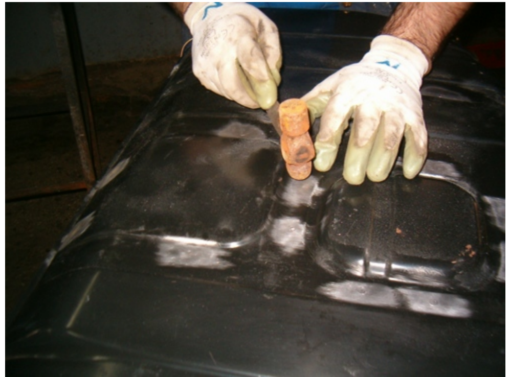
Using the rounded end of the hammer the welds are flattened, so as patches are level
