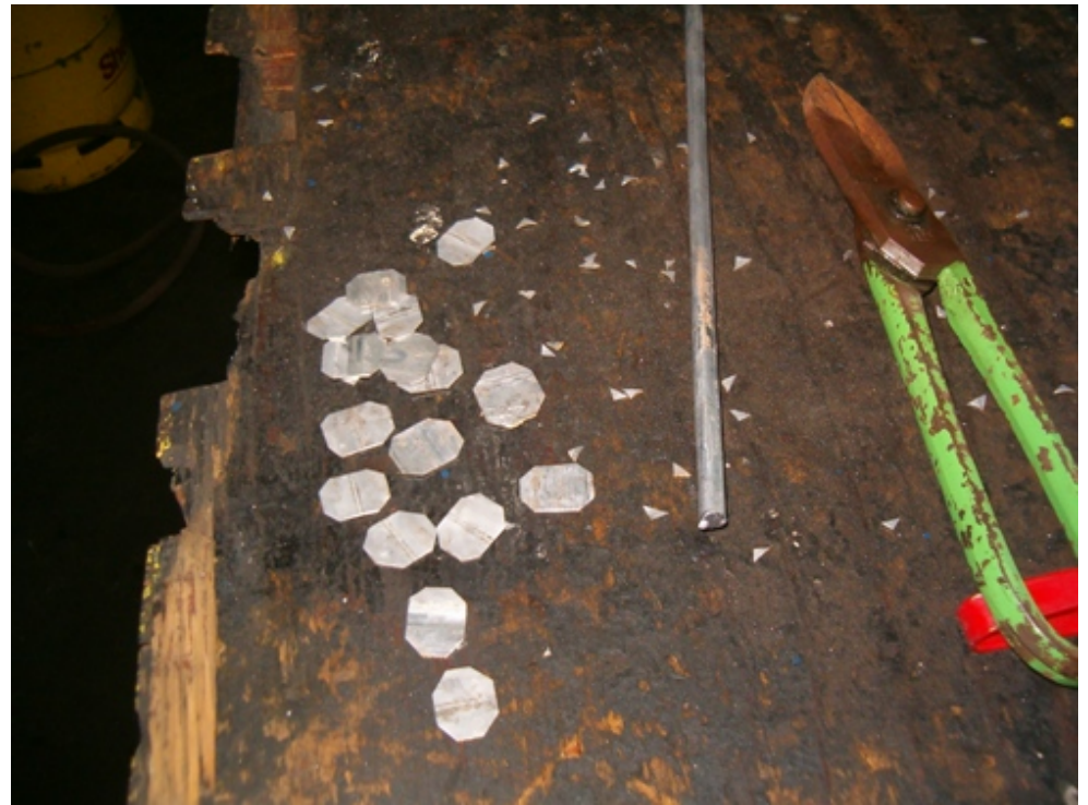
The patches are almost ready in round shape. The material used is brass in thin leafs.
