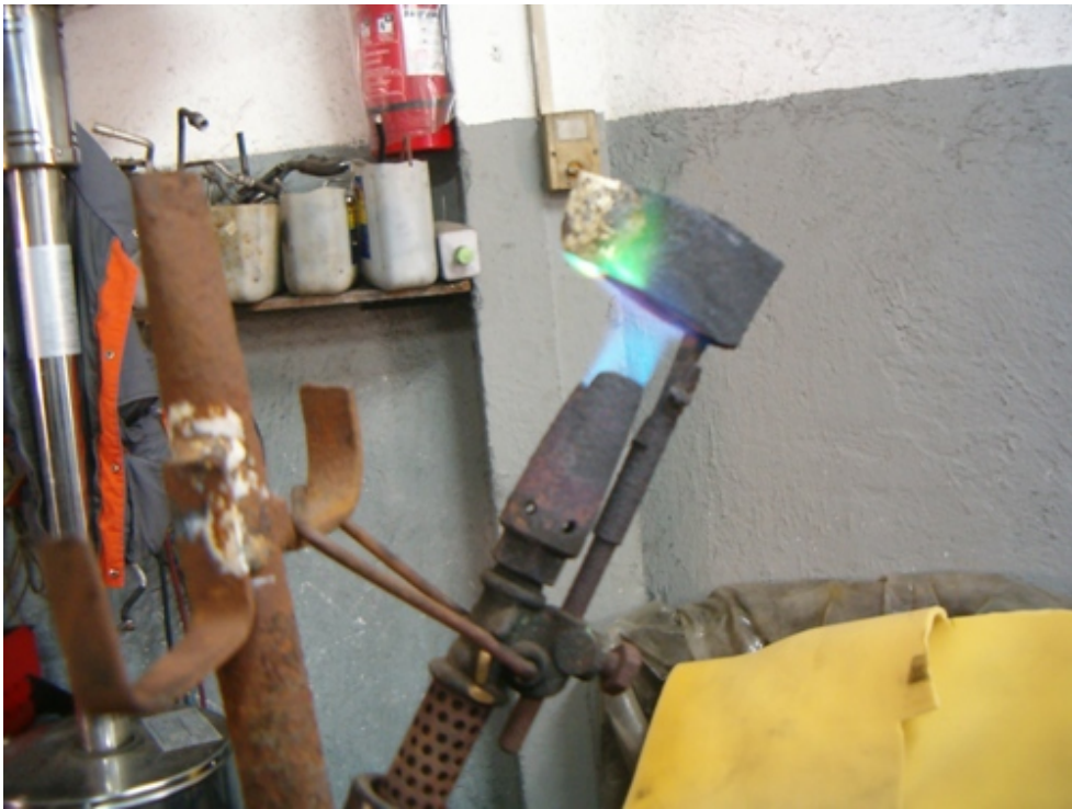
Here is the soldering iron prepared for action. It is not an electrical iron but a liquid gas one as here we want rapid heating of the iron that an electrical one can't provide.
