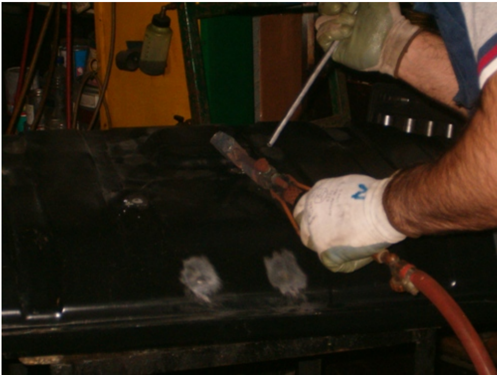
and the first layer of solder is applied to the tank welds
