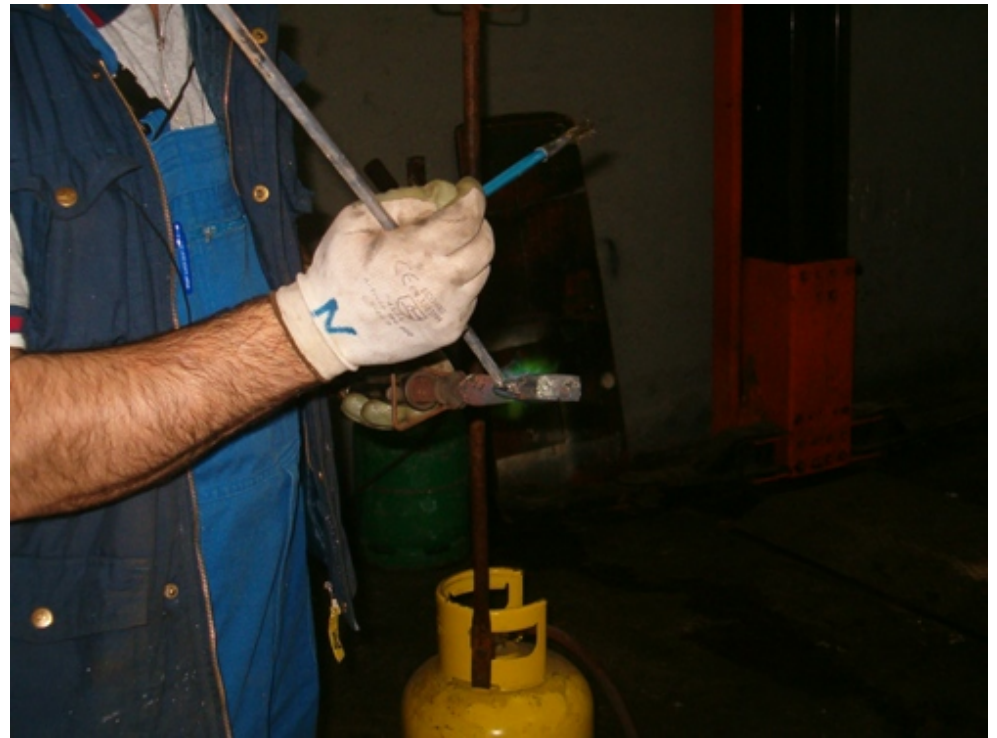
Sodler is being applied on the hot iron
