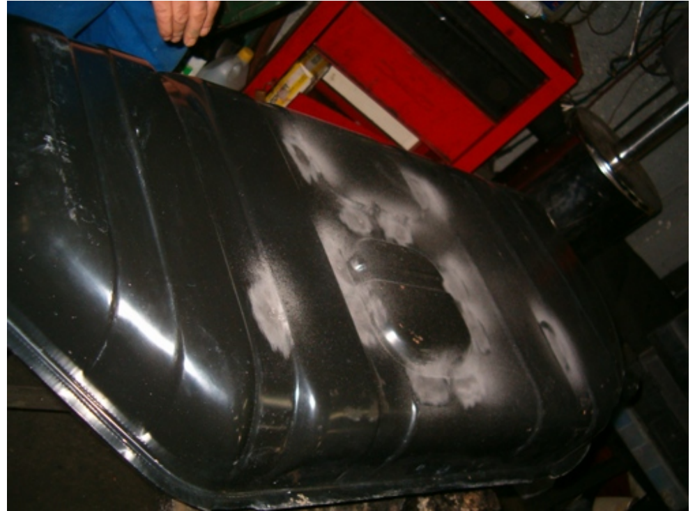
Nearly all welds are now exposed to bare metal
