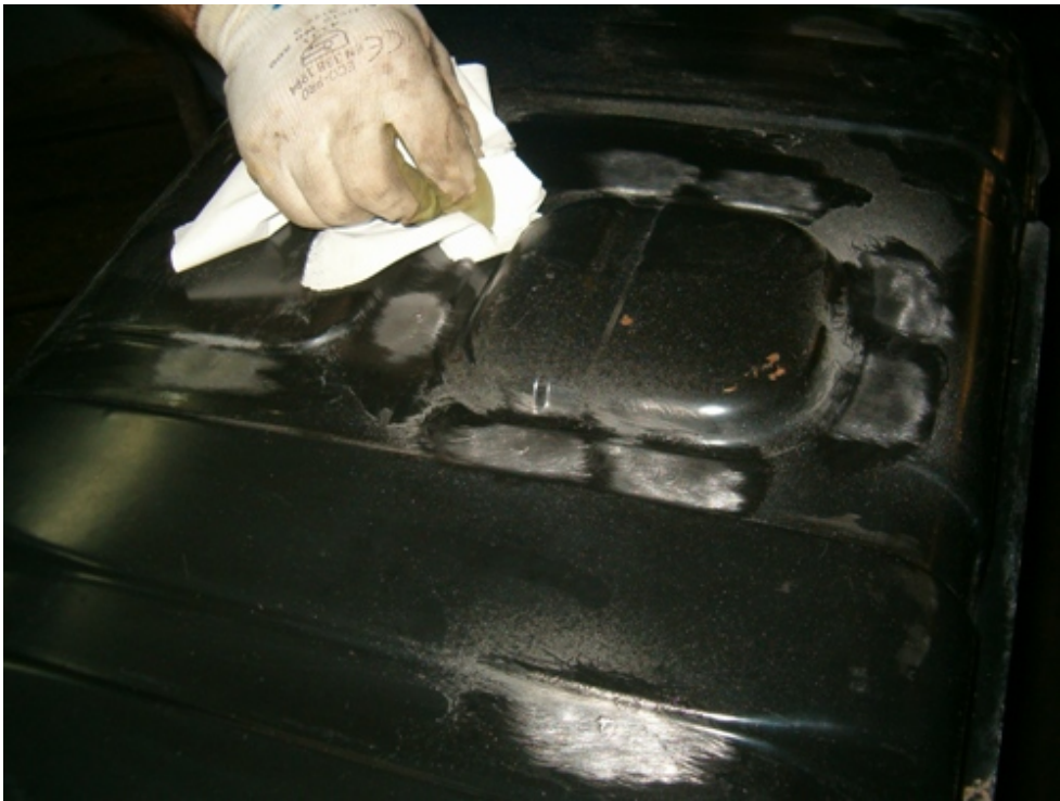
Metal surface is now cleaned with thinner in order to ensure proper bonding
