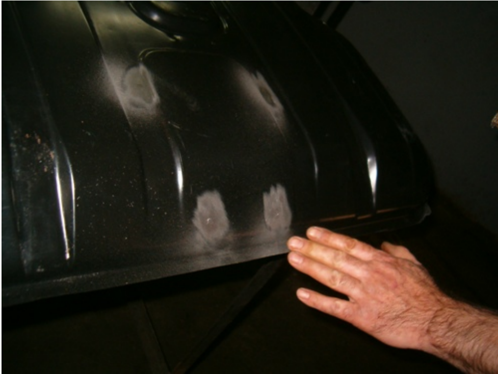
Nearly all welds are now exposed to bare metal
