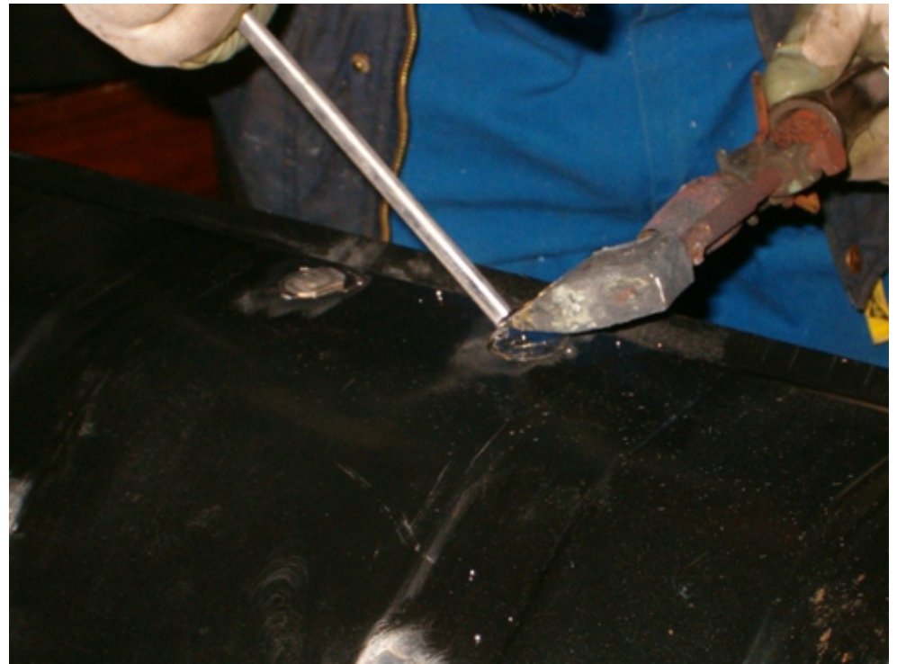
and the first layer of solder is applied to the tank welds
