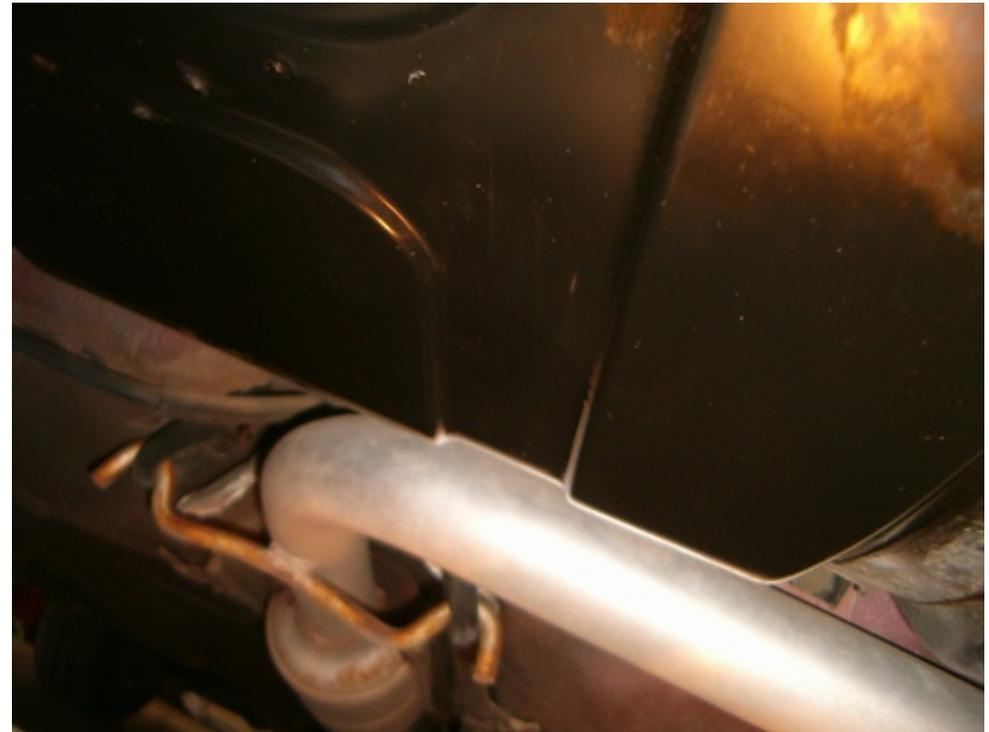
Not clearly seen but this is the part of the tank where the leak is located; it comes off a spot weld.
