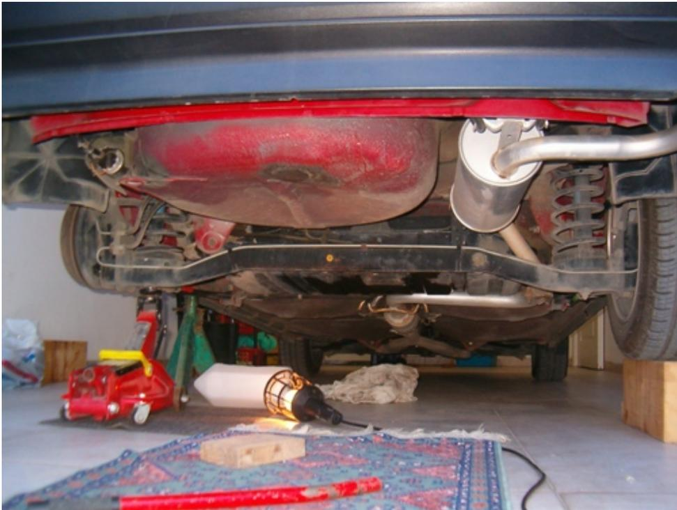
Raise the rear of the car in order to get as much clearance as possible. I used a stand at the left jacking point and a piece of wood under the right side wheel; this way I feel safe under the car.
