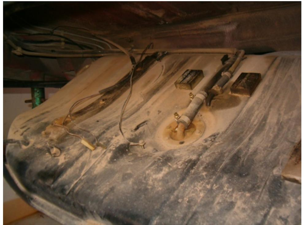
A couple of close ups show the fuel sender unit along with the fuel supply/return lines. Quite nasty is the earth lead that must be removed along with a fuel sender unit bolt. For sure I will find a better solution of attaching the earth lead to the chassis once I restore the tank
