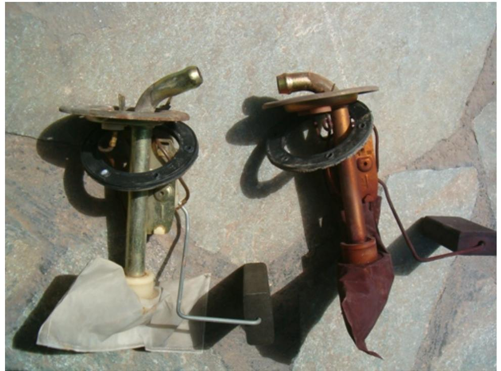
There are a couple of differences between the two tanks as far as the fuel sender unit is concerned. The original tank has the sender unit facing forward (front of car) whereas the replacement tank has the sender unit facing backwards.
