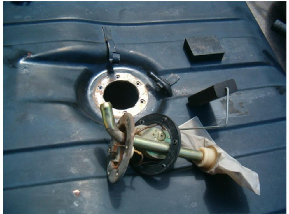
The same principle is applied to the pipe routing. As you can see in the photos above, the original tank (left photo) has the fuel return pipe facing forward (front of car) whereas the replacement tank (right photo) has the return pipe facing backward (rear of car). This is of no major concern as the return pipe will be routed using a flexible 8mm fuel line.
