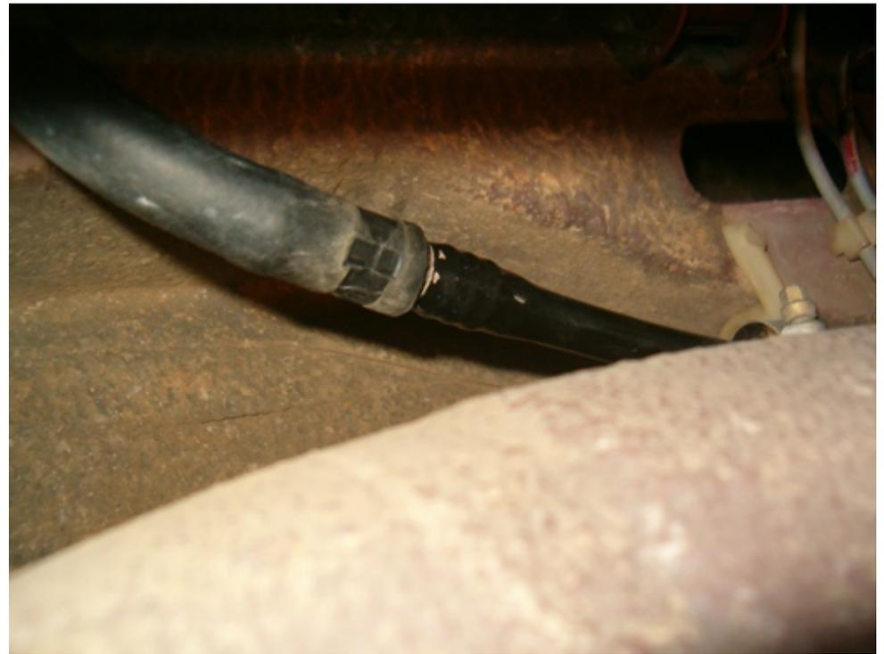
Then undo the clip on the fuel hose that sits just behind the spare wheel well.
