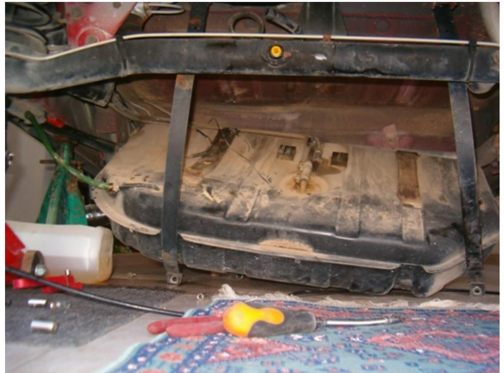
Once the strap bolts are removed the tank easily drops as shown on the photos
