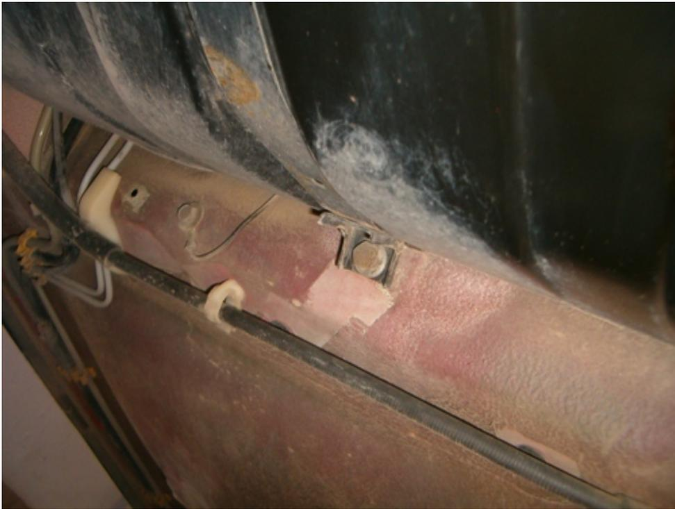
We must remove the two strap bolts which actually hold the tank in place...
