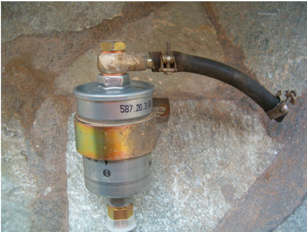
and pay attention so that the support bracket is parallel to the fuel hose.
