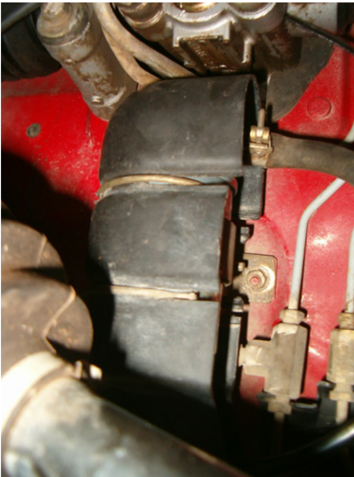
Finally restore the filter cover ensuring that the clips wrap around the filter body.
