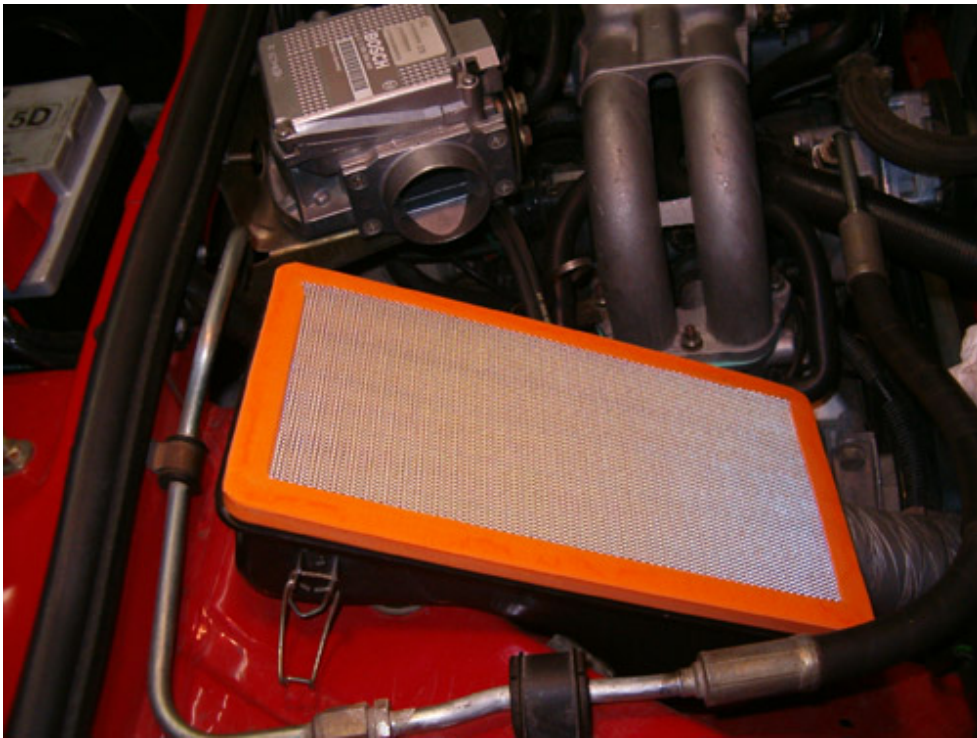
Install the new air filter ...
