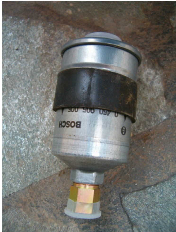
Install the rubber band around the new filter
