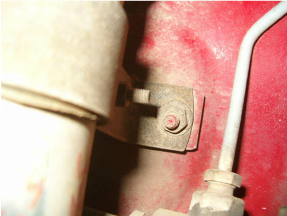
Time to remove the bracket from the chassis so as to remove the filter; it is a 10 mm nut.
