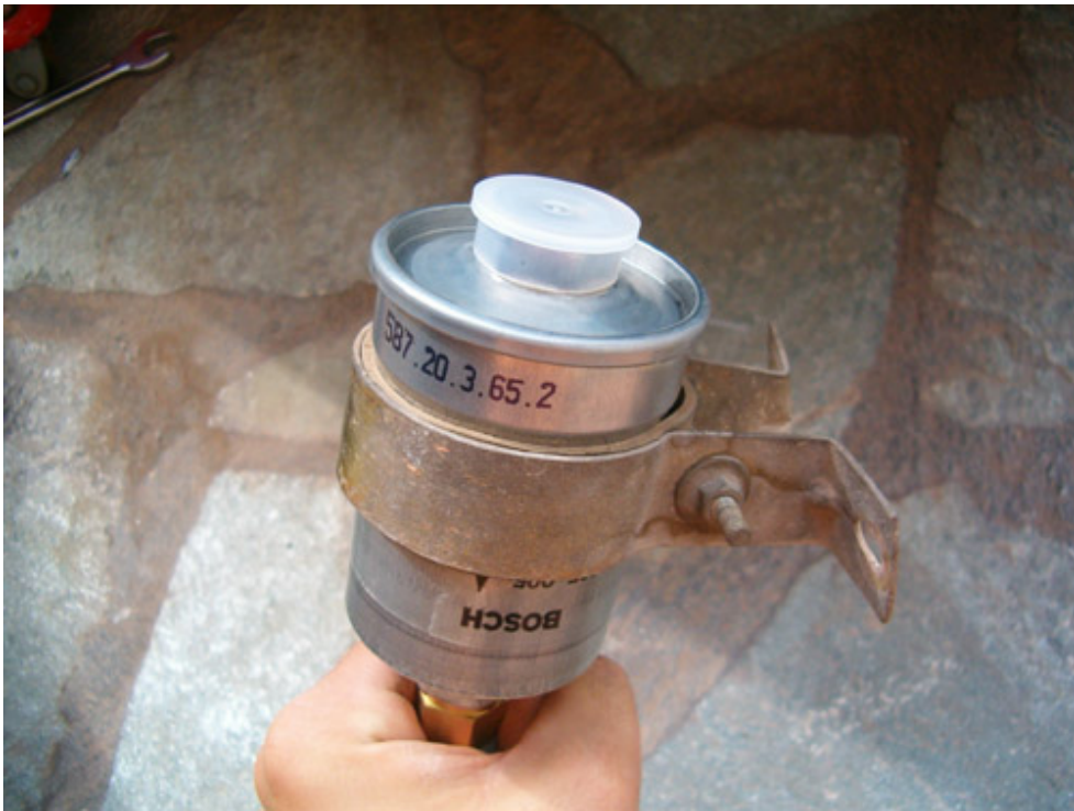
and proceed installing the filter to the bracket; tighten the nut you see in the middle.
