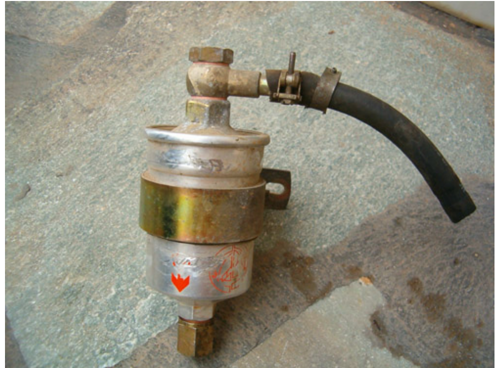
Filter is out of the car along with the inlet fuel flexible hose.
