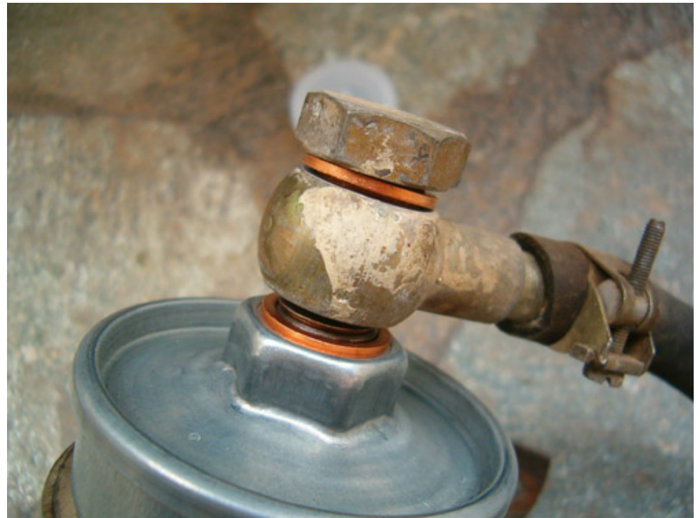
Install the new washers to the upper connection of the filter ...
