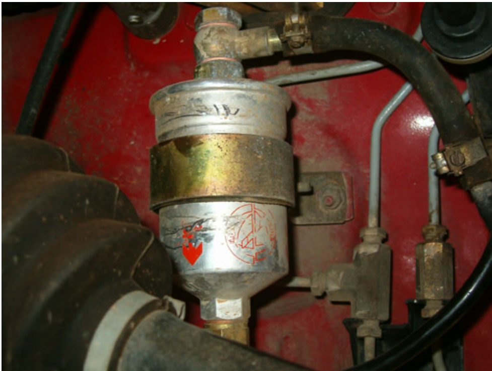
Fuel filter without cover demonstrated
