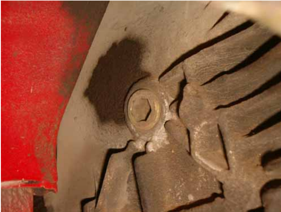
this is the transmission oil filler plug; use the 12 mm Allen key to remove it
