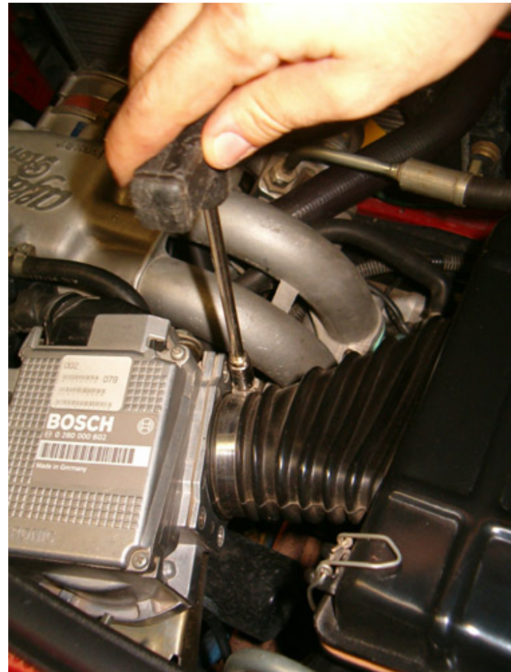
It is time to undo the air filter box clamp ...
