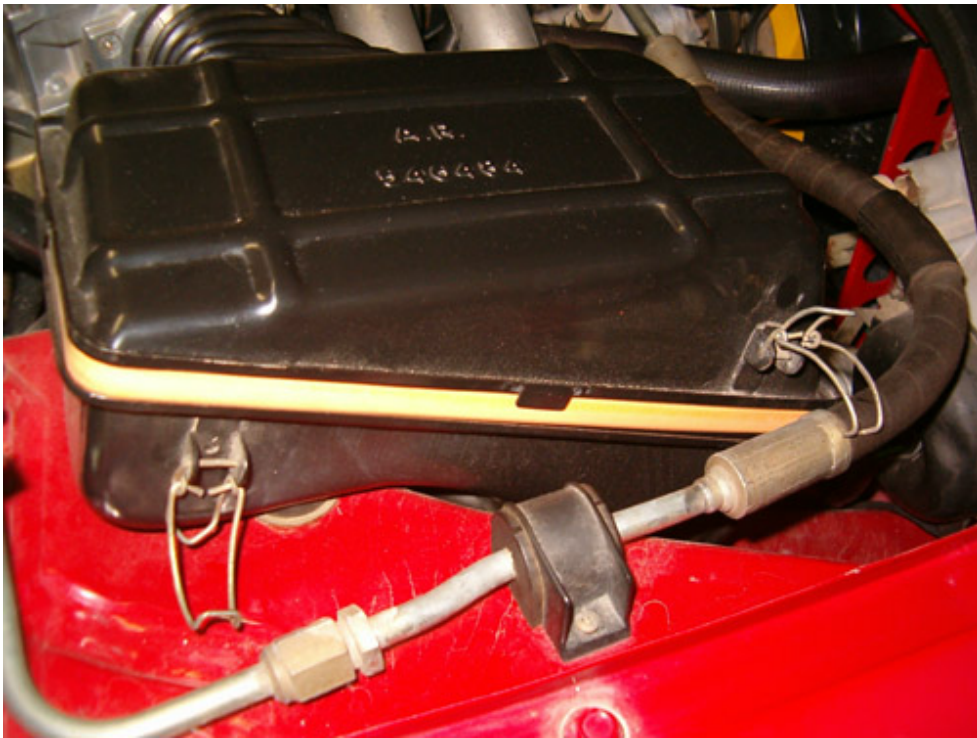
... and the four clamps holding the cover of the air filter box.
