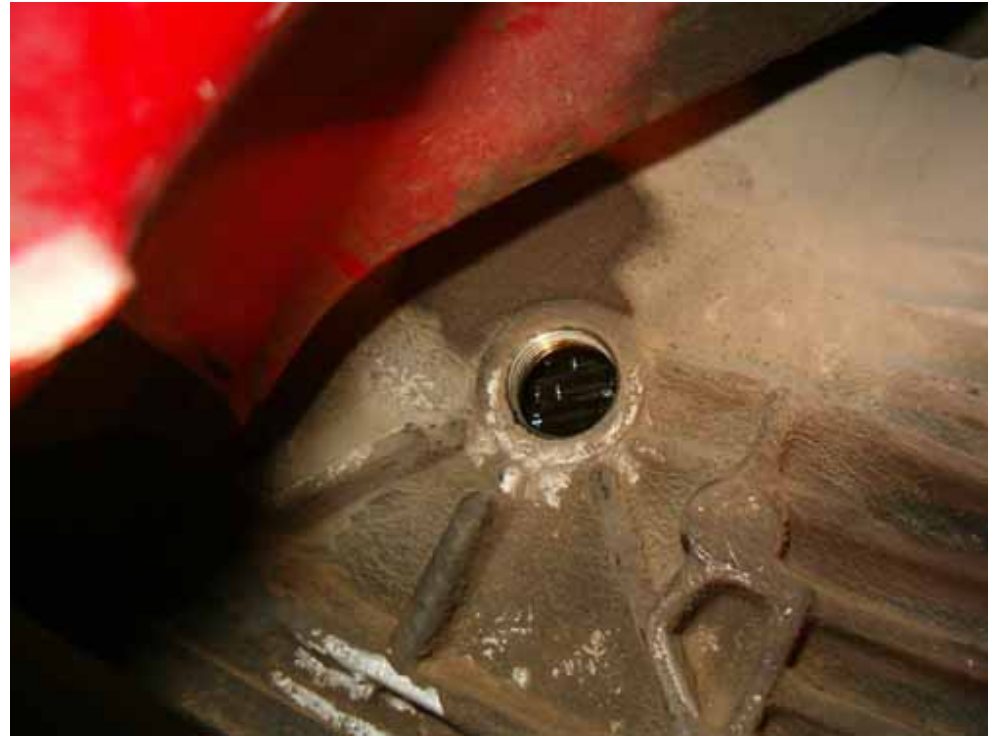
this is the transmission oil filler plug; use the 12 mm Allen key to remove it
