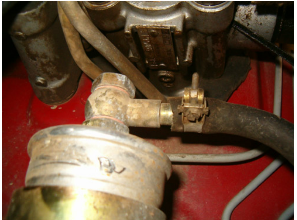
Now that the way is clear, notice the upper connection (fuel inlet) ...
