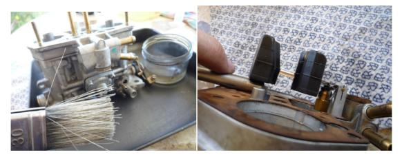
Float level adjustment and acceleration pump calibration was performed.
