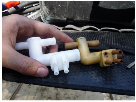
Another example is the water union above the water pump. It was likely a piece of rust...even though this was the special version for tha A/C equipped engines...but Thanassis supplied the used part (perfect condition, thanks Thanassis). Although the part dimensions were slightly different, I could still manage to install it properly:
