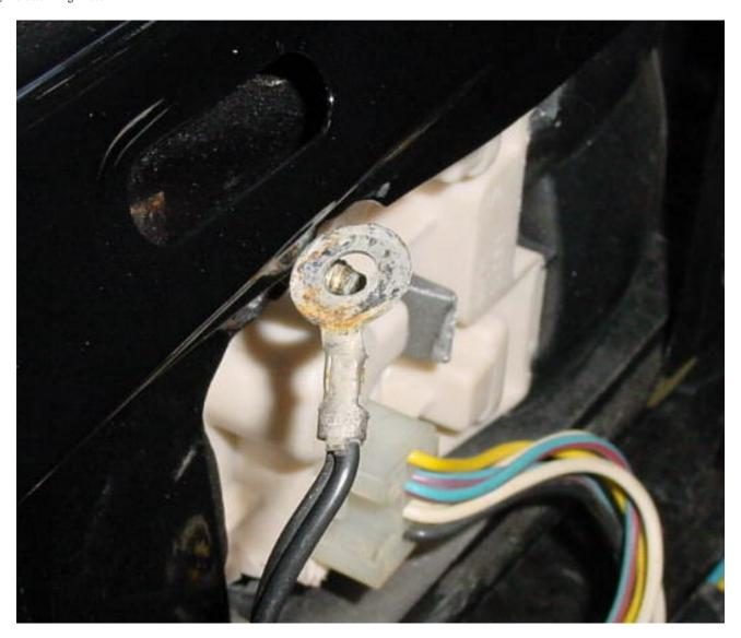
This ring terminal will be under one of the bolts holding the tail lights to the body. I think there's one per side of the car. It grounds the light circuits to the car body, and **it shouldn't look all crusty like the one in this picture!** Clean the terminal and the area of the car body it touches using sandpaper, CRC, electrical contact cleaner or whatever seems appropriate.
