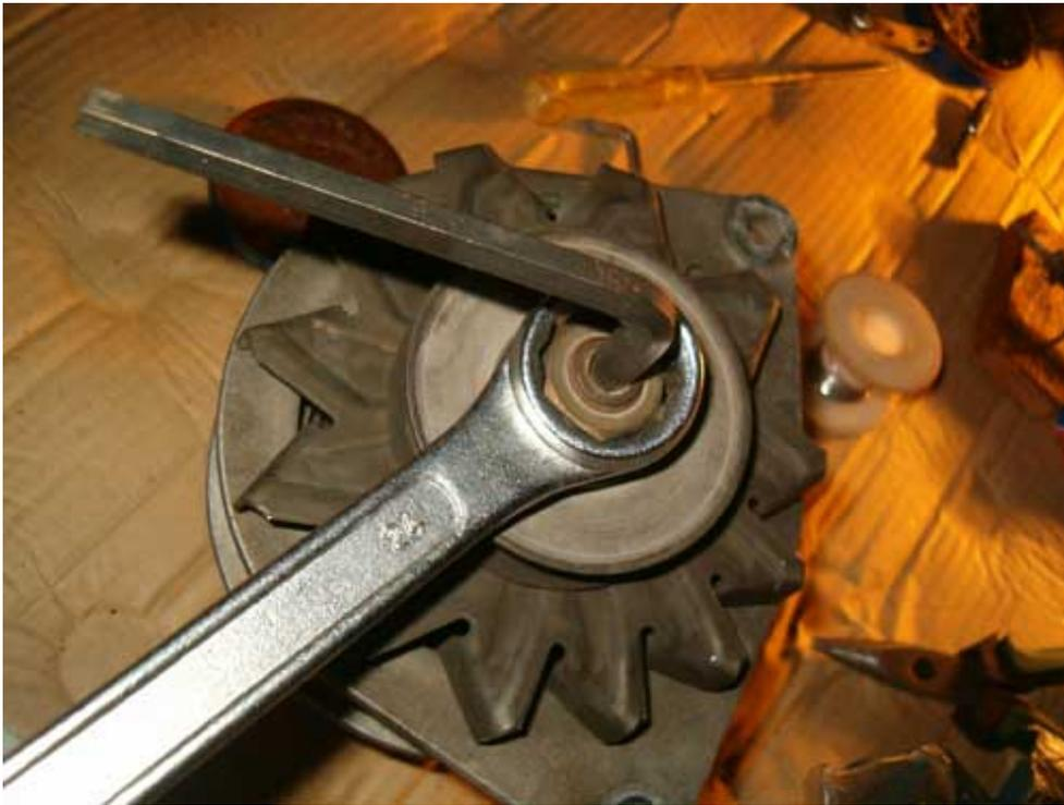
Using the 24 mm wrench and the 10 mm allen key, remove pulley and fan of the alternator. Do not mix the order of the washers under the nut and fan.
