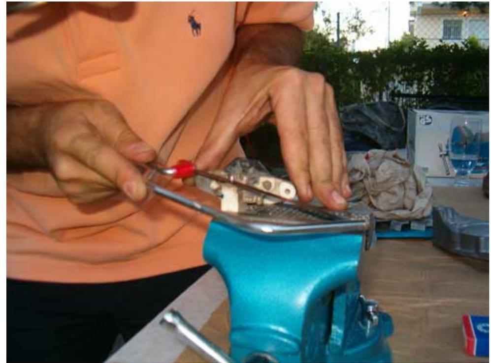
It is now time to replace the regulator brushes. Place the regulator in the vice and with a metal saw, cut the ends of the brushes extruding. It is then much easier to unsolder the brushes.
