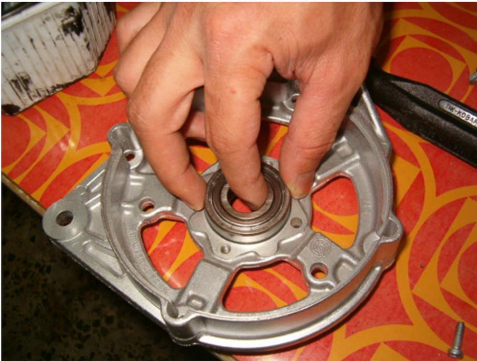
Let's now install the front bearing (SKF 6203). Just install it on its place; no need to hit or press it in.
