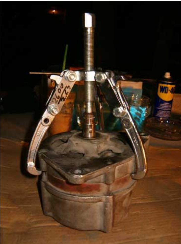
Now using the bearing extractor, pull out the front case of the alternator. Just screw in the vertical bolt and the case will slide out of the rotor
