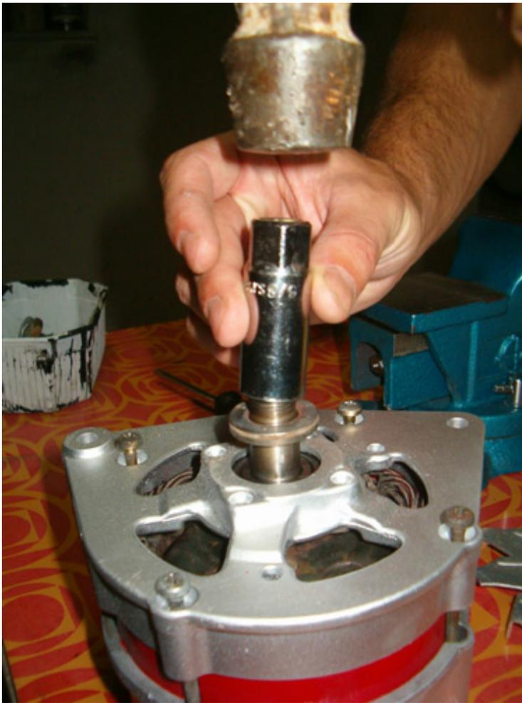
install front cover and with a socket punch in the washer as seen in the photo. Also install and bolt in the four long screws that actually keep the cases and rectifier bridge together.
