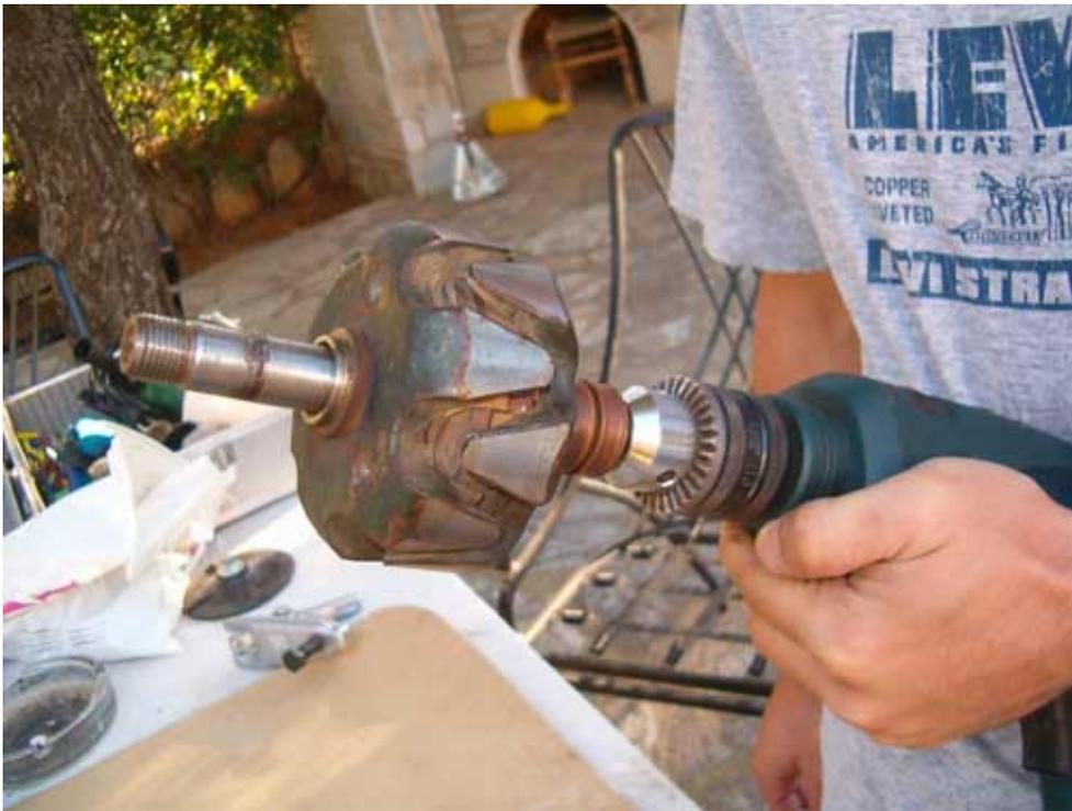
Place the rotor to the drill ...
