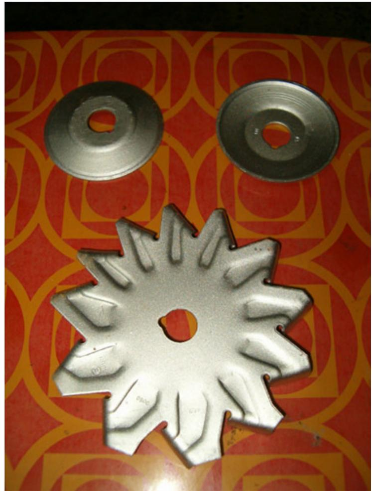
The case, pulley and fan have been painted with high temperature silver enamel paint
