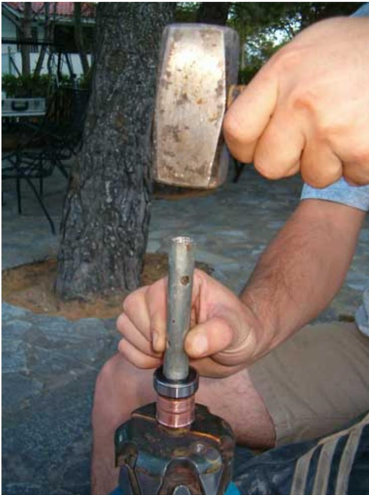
Here is a critical part. Find a socket exactly the size of the bearing inner ring. Place the socket on top and with a hammer punch it steadily making sure to have the bearing sitting vertical to the axis of the rotor. Do not use another way for this installation as hitting the bearing anywhere except its inner ring, it will definitely destroy the inner balls and both rings (inner and outer).
