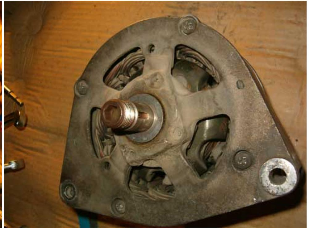
Here is the alternator without pulley and fan. We now need to undo the four bolts on the circumference of the casing. Since these bolts may have never been out, it is pretty likely to ruin their head as they are stuck to the alternator body; do the following trick and you won't miss a single bolt!
