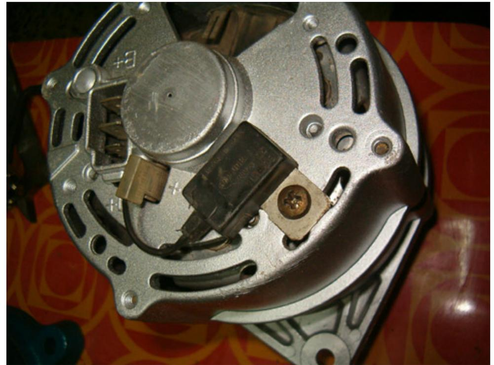
Proceed installing the capacitor which has as purpose to absorb high frequency electrical waves created by current generation. Without this device you could hear in your radio player high pitched sounds which would otherwise escape from the electrical system.
