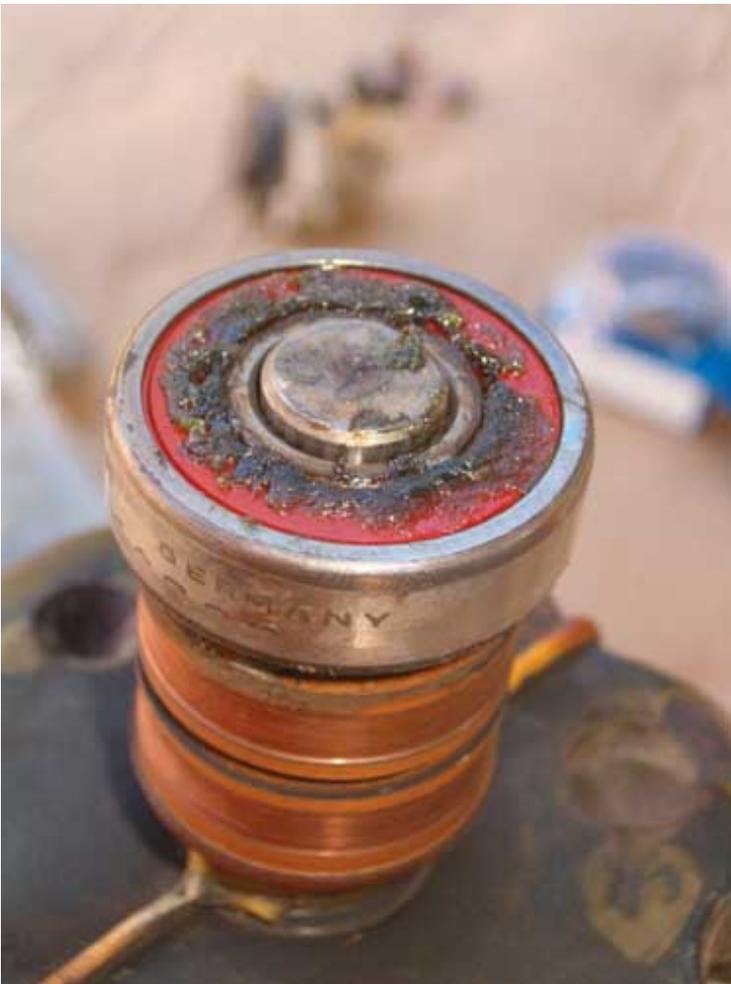
A close -up of the bearing which has lost its grease ... Needless to say that the play of the outer diameter is big enough!
