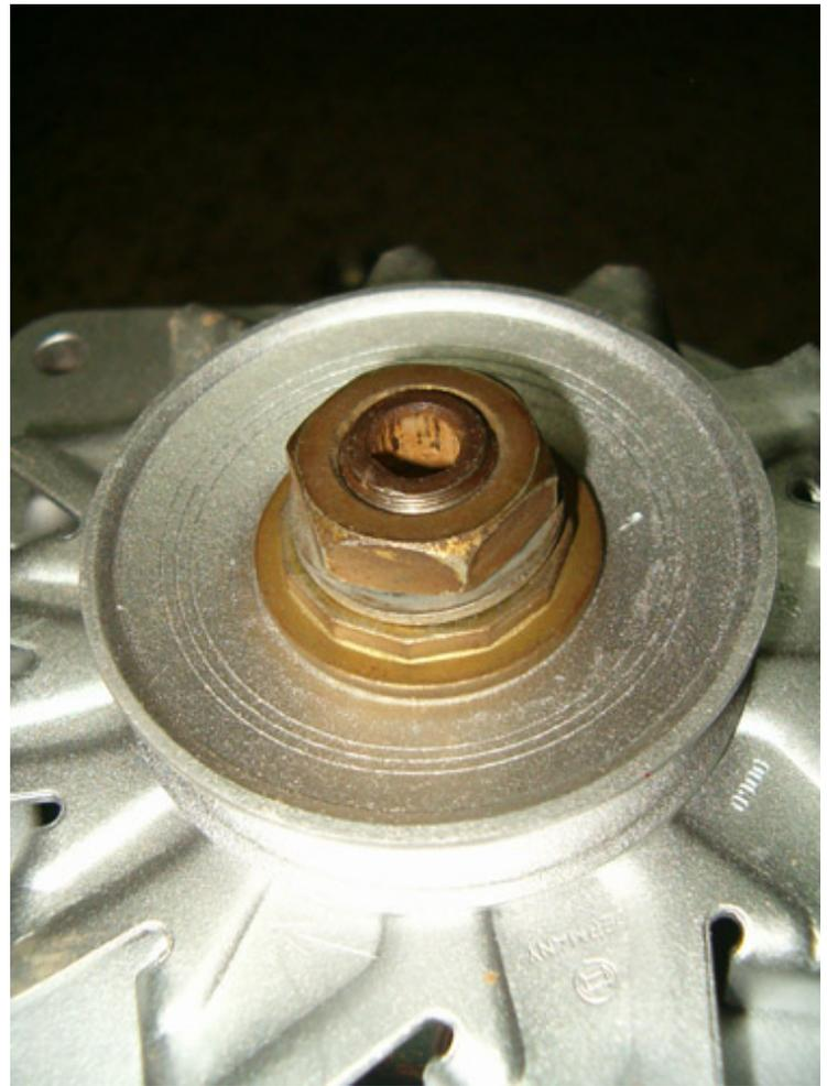
... and finally the two washers and securing nut.
