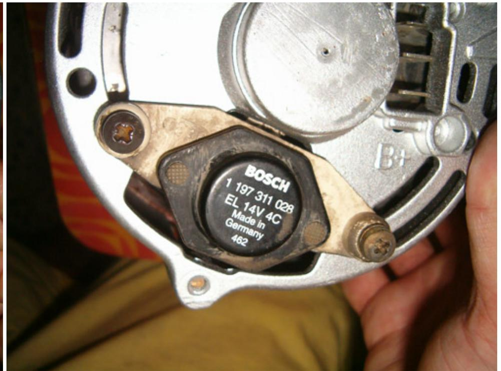
Finally install voltage regulator.
