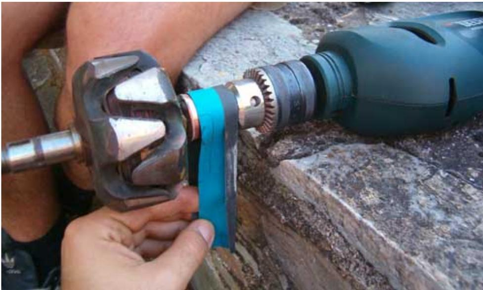
Rotate the drill at low speed and place the sandpaper so that it covers the surface of the slip ring.
