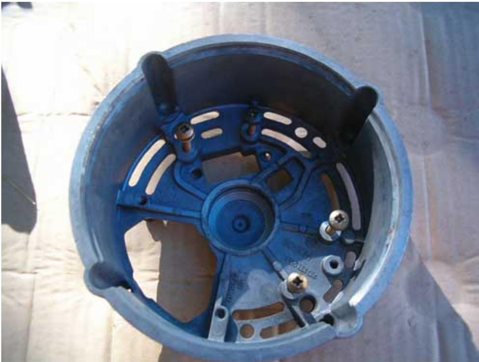
These are the cases of the alternator. Here you can see then cleaned with diesel fuel which eats away dirt.
