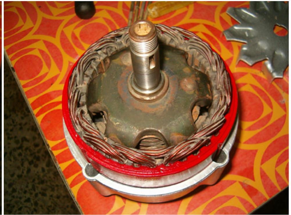
... and press in the rotor to the case.
