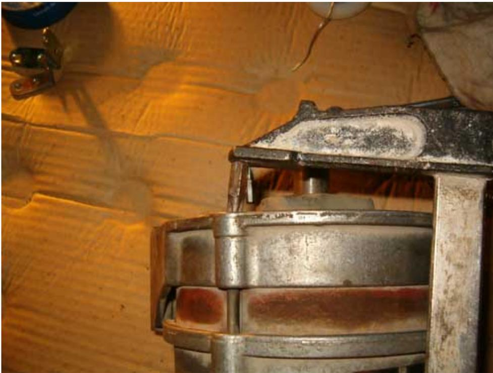
Get hold of a carpenter's brace and a cross screwdriver tip. Make sure that the tip perfectly fits to the screw head.
