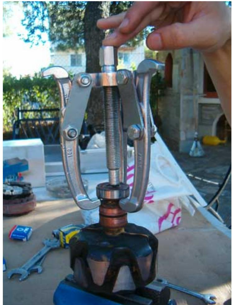
Now we will remove the bearing from the rotor using the extractor. Do not attempt to remove it by using other means !!! You can easily damage the slips rings and you may need to replace the rotor!
