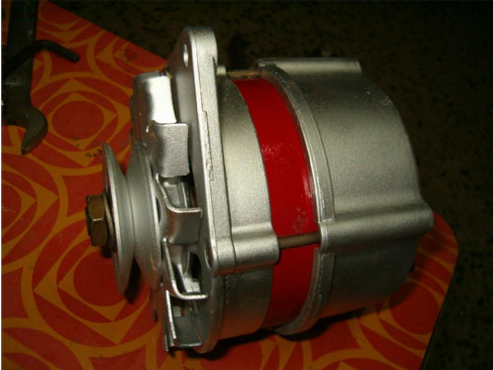
Alternator is now ready for installation to the car. We measured the output of it on idle and it was almost 14 V; on 2,500 rpms it reached 14.3 V. For sure the alternator will last double years as this was a ground - up restoration. Well done!
