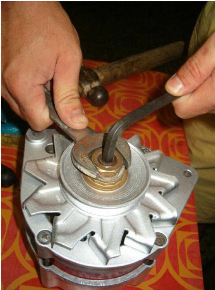
Now fully tighten the nut (24 mm key) with the help of a 10mm allen key
