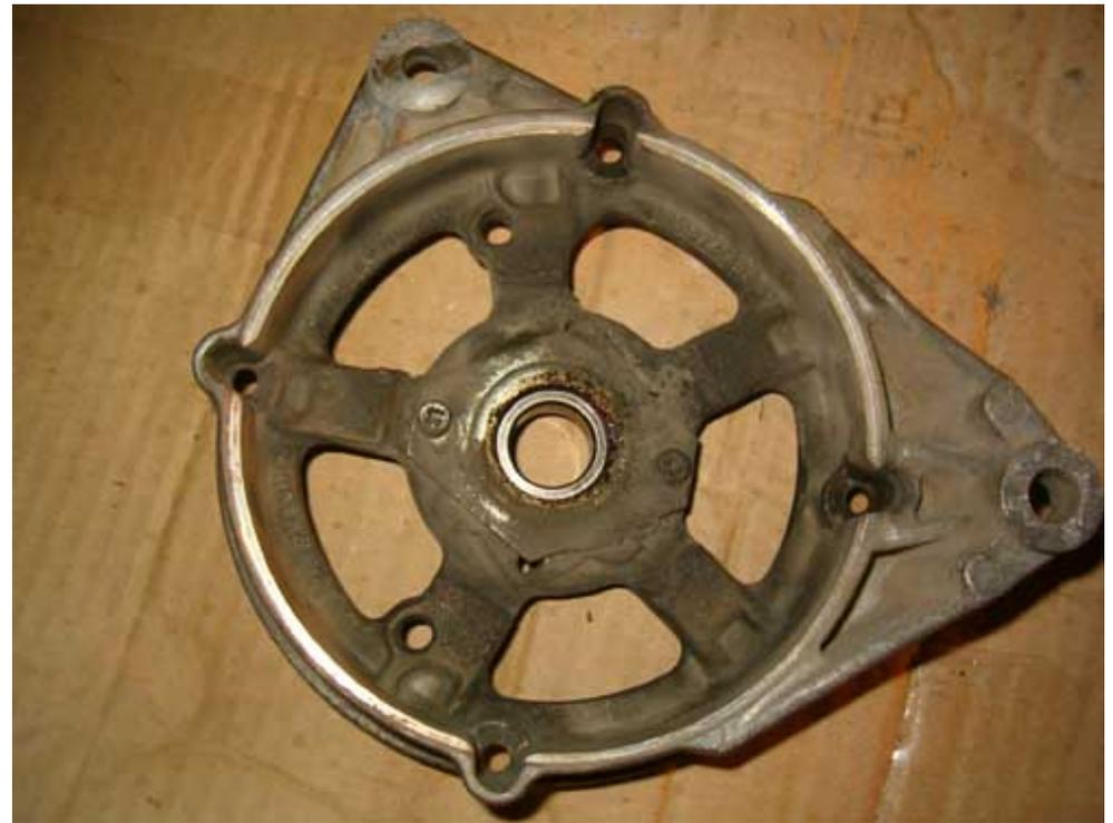
Here is the front case extracted. You can see the front bearing (SKF 6203) in the centre and the two bolts keeping the plate attached to the body.
