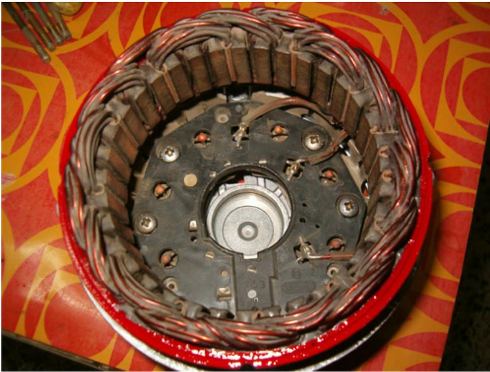
Bolt in the four screws fixing rectifier bridge to case ...
