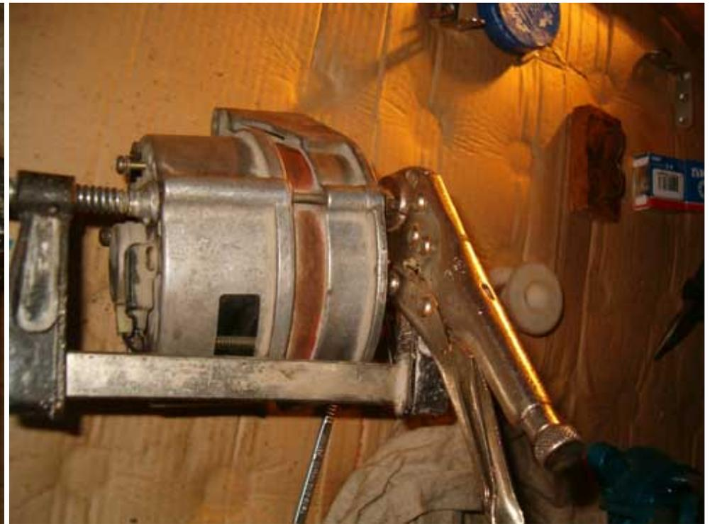
Tighten the brace and using the pliers just unscrew the bolt. It will loosen right away.
