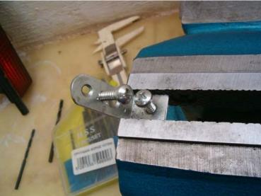
demonstrated are the screws that will be used. The rightmost screw will actually bolt on the window frame and the leftmost will keep in place the lamp plate
