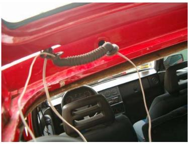
it is now time to pass the lead inside the rubber snorkel and hide it above the headliner
