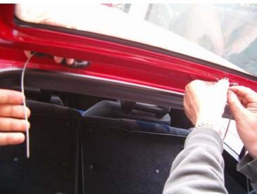
Here you can see the process under which the cable passes inside the window frame. I have used a steel cable that will actually transfer the leads for the light. Steel cable intended for bicycle brakes is perfect.
