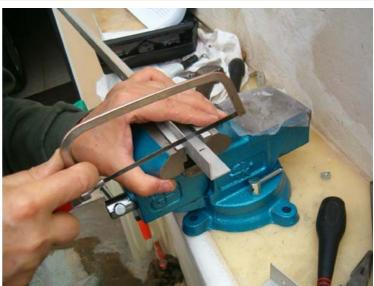
an aluminum piece will help us fabricate two small brackets for the red light. Aluminum is a very nice and handy material to work with; easy cut & easy bent.
