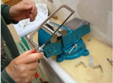
This is the middle of the window frame where the bracket will A vice is a must for such cutting jobs - here the bracket is cut be installed to the measured distance
