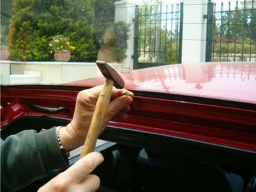
Having measured the centre of the frame, a mark will help punching once or twice will help the drill do a perfect hole; no scores or pitting to the rest of the paintwork
