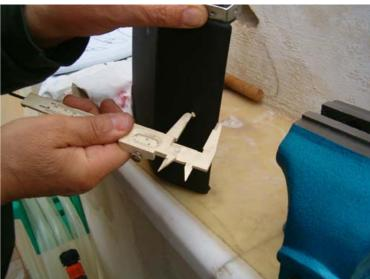
The screw that keeps the plate firm to the window frame will pass through the hole you see in the middle of the plate. We had to fabricate a bracket which would hold the plate; an accurate measuring of the distance between the retaining screw and the edge of the plate had to be performed.
