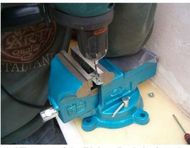
... drilling an extra hole will help us align the bracket to the plate much easier and precisely.
