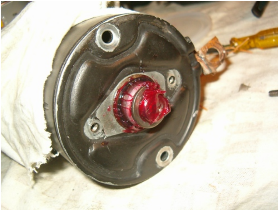
Fit retaining ring, install dust cover and bolt in the new screws
