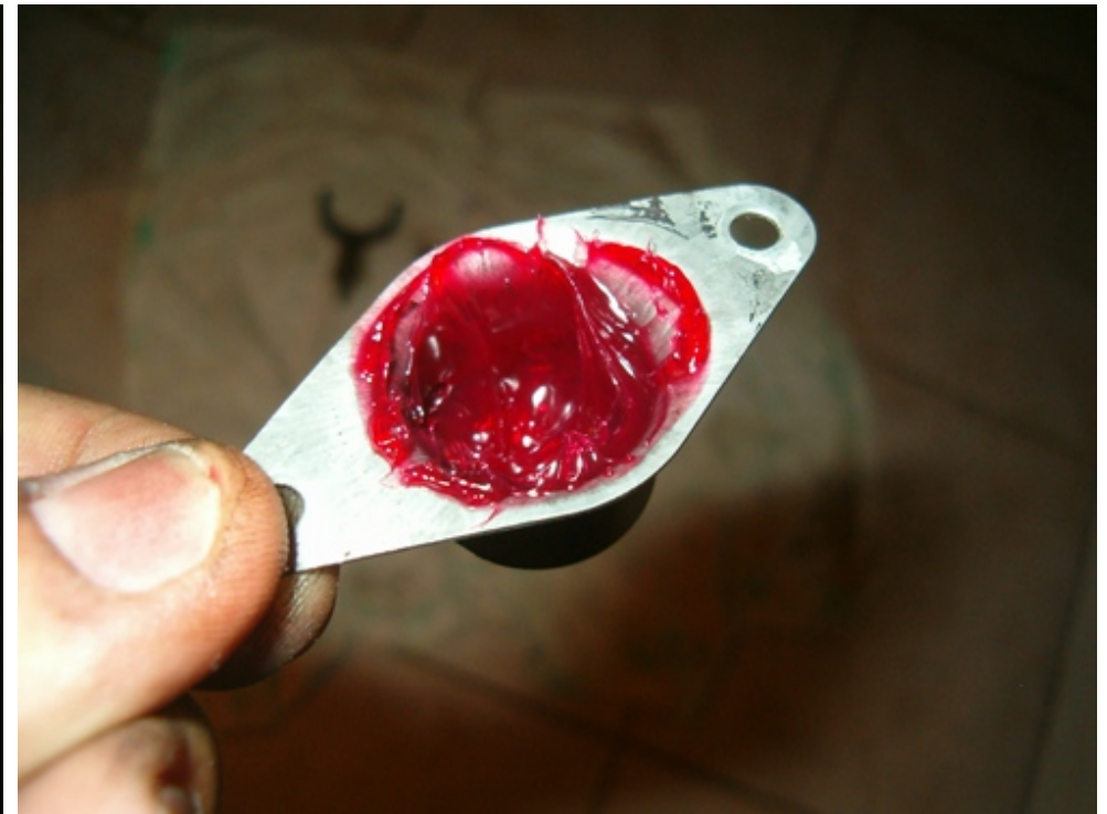
and insert plenty of grease in the dust cover cavity
