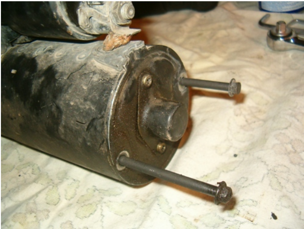
... and then the two long bolts that actually run across the motor body
