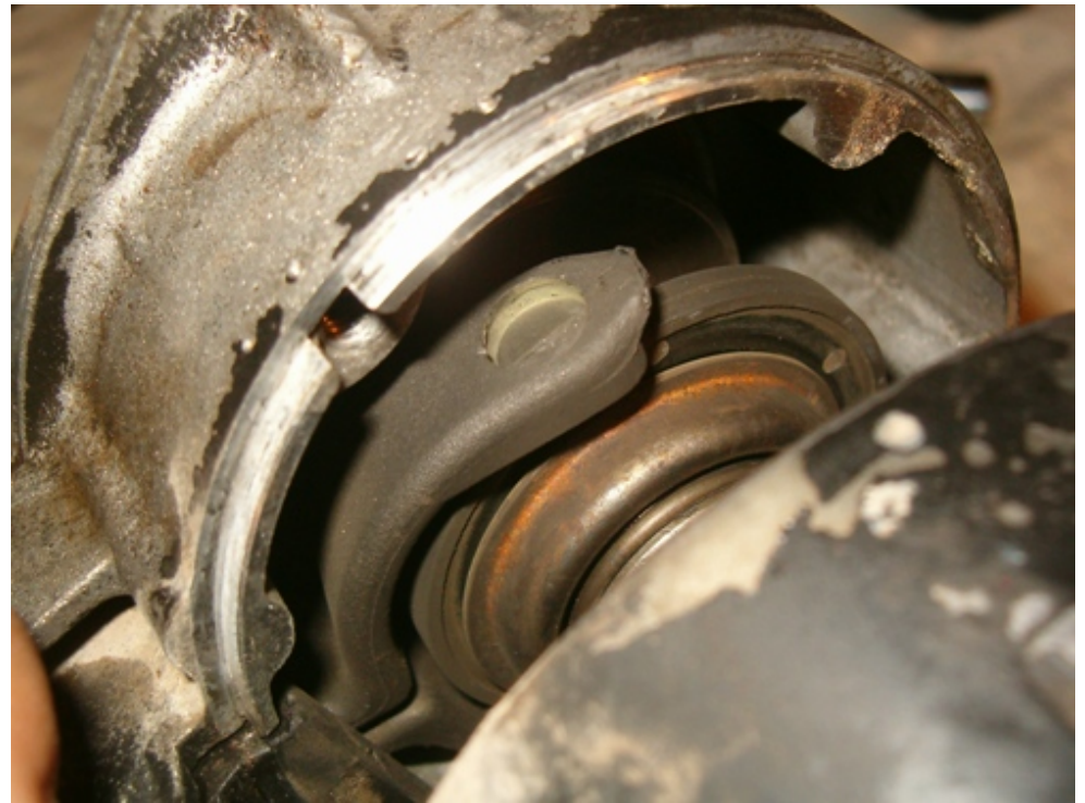
Separate motor body from the drive housing ...
