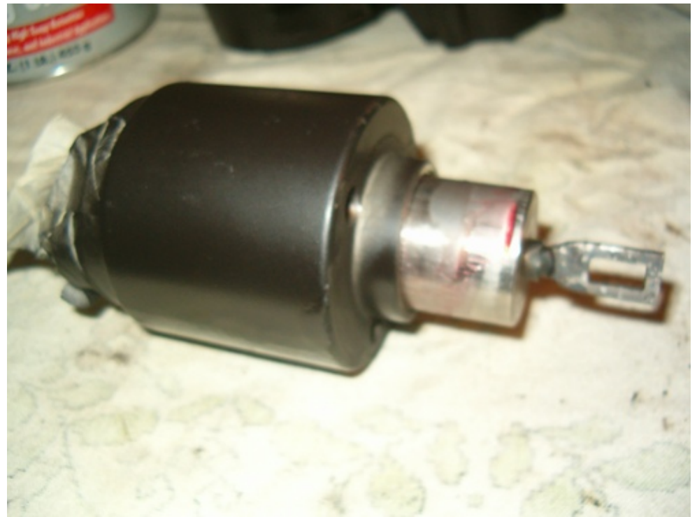
Install piston on solenoid
