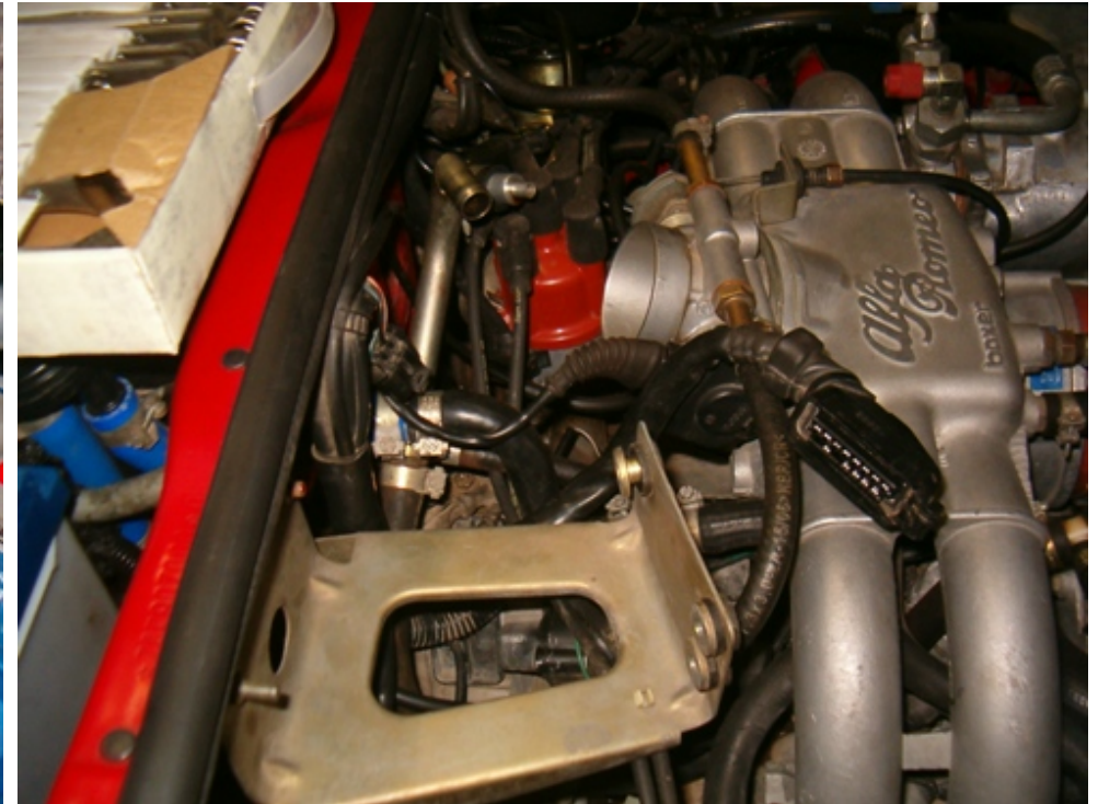
Remove ECU/AFM and intake sleeve in order to free up some space to work on
