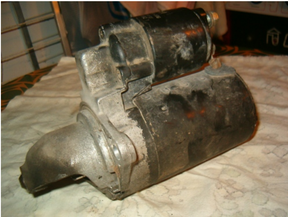
The starter is now off the vehicle and ready to be serviced. It is a high opportunity to have it also painted
