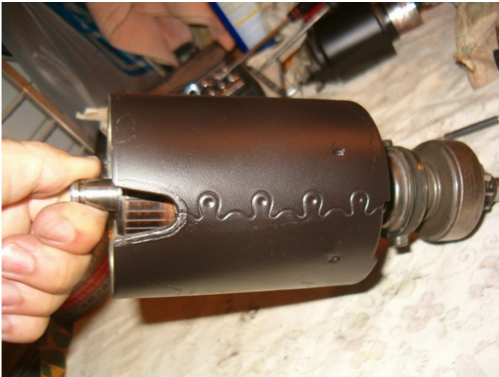
Press in the rotor. Be careful as the magnet force is quite strong ...
