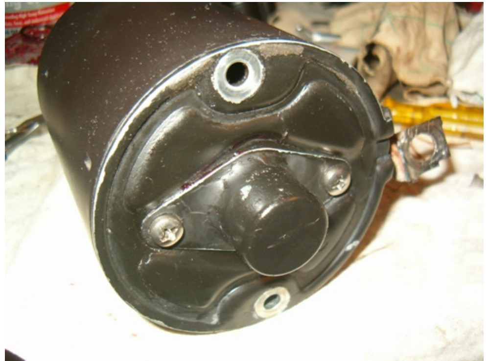
Fit retaining ring, install dust cover and bolt in the new screws
