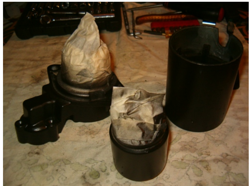
External parts painted with black high temperature paint from a rattle can
