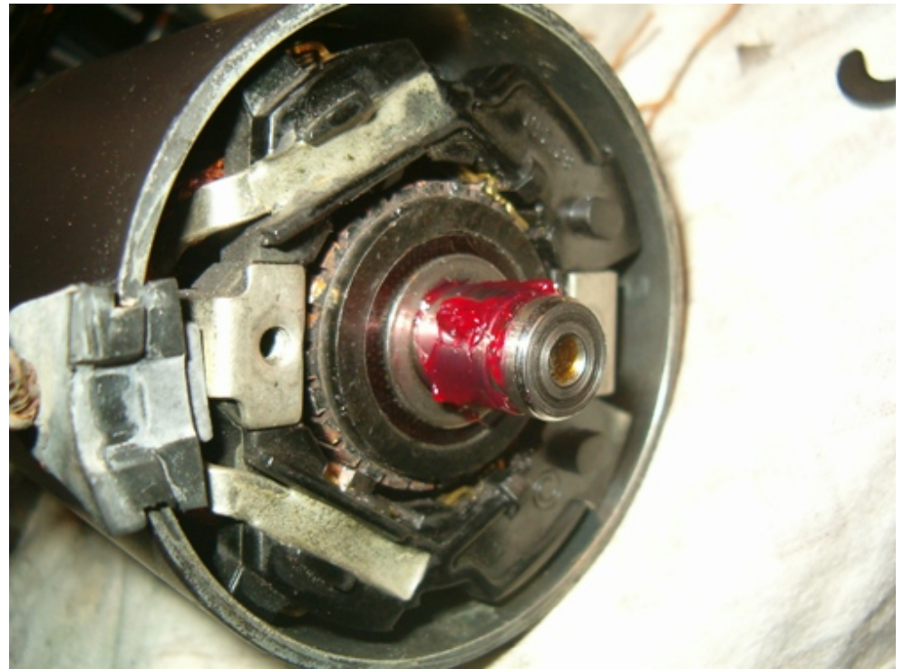
... and lubricate the shaft end and be sure to have the large washer inserted on the shaft end
