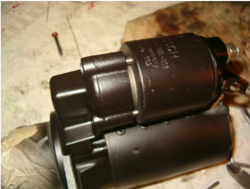
Tighten the solenoid screws in a cross manner little by little as we want the solenoid to sit properly
