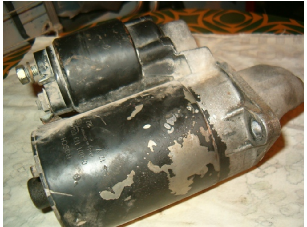
The starter is now off the vehicle and ready to be serviced. It is a high opportunity to have it also painted
