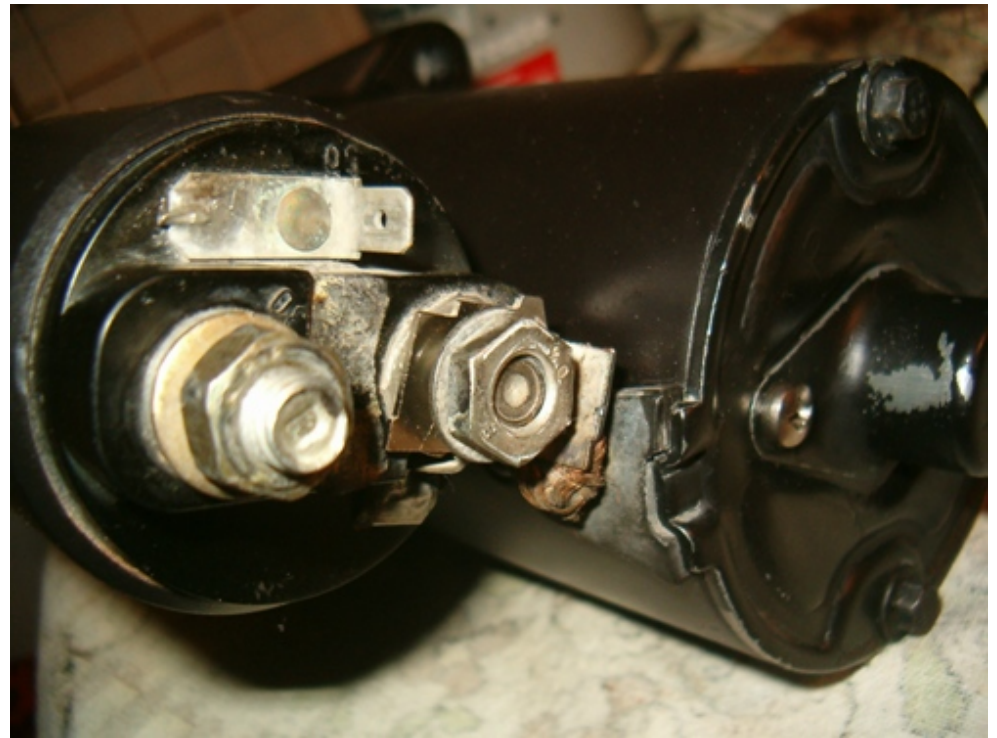
Then fully tighten the positive current strap bolt
