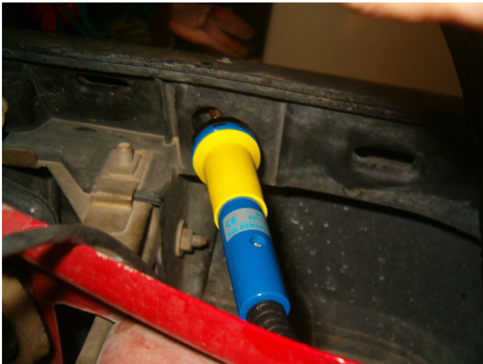
Carefully insert the iron on the opening being careful not to melt the surrounding area
