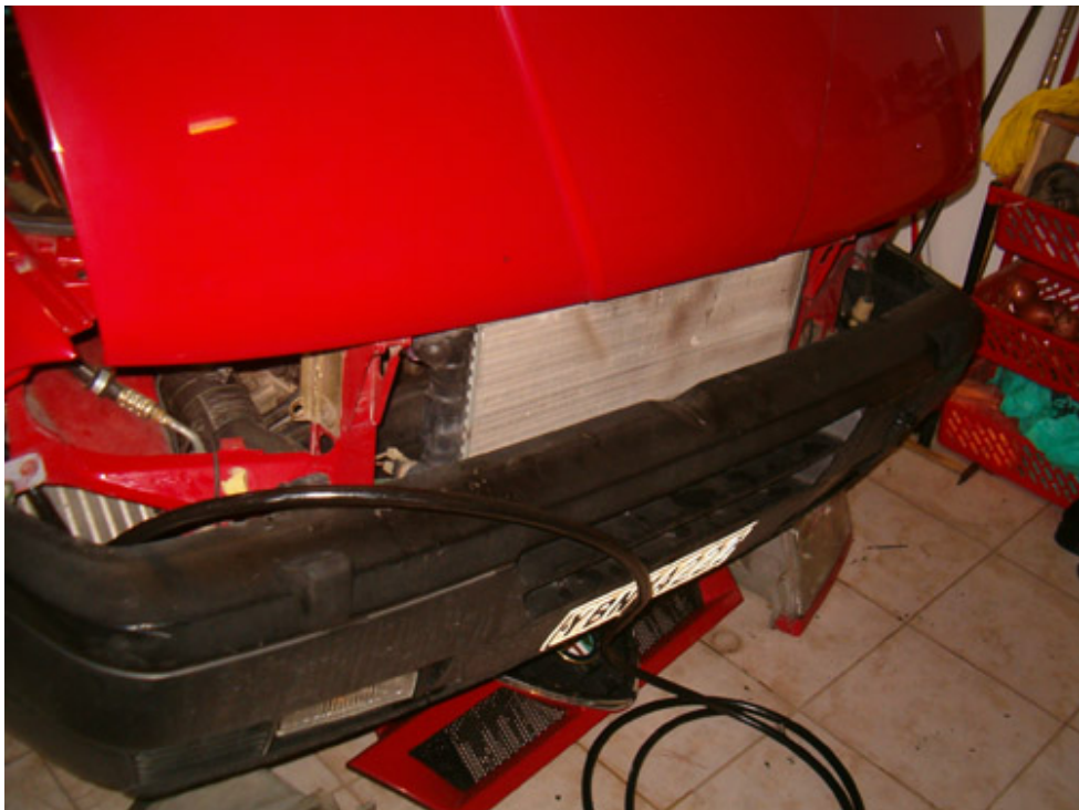
Time to measure the length of the hose and attach it to the headlight washers
