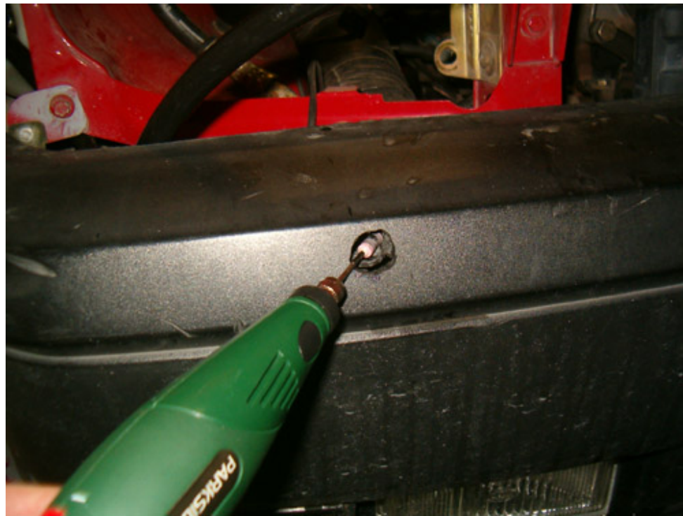
Right after the opening has been created, I used the Dremel tool to machine the plastic and create a round opening.
