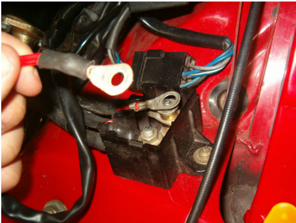
Remove carefully the junction box cover and attach the positive lead of the harness
