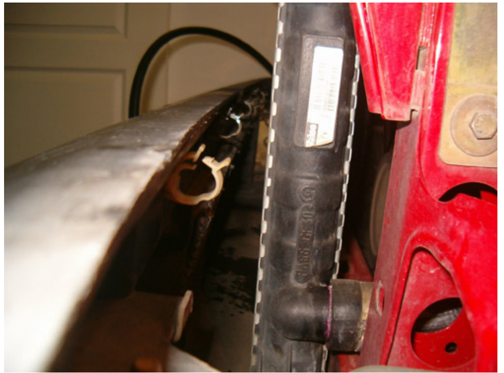
Attach the plastic keepers for the washers hose (6 in total)
