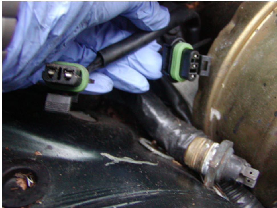
and the respective harness connector on the vehicle main loom. Although the washers kit came off a RHD car, the connector on the LHD version is on the same place (just behind the battery)
