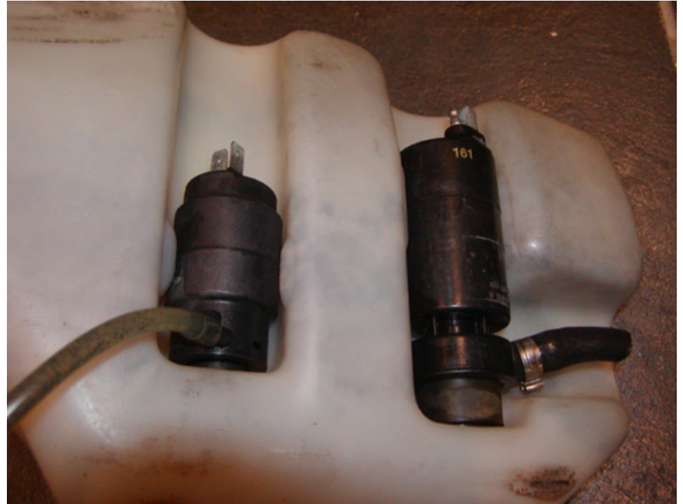
Windscreen washer bottle showing the two pumps. On the left is the windscreen sprinklers pump and on the right is the headlight washers pump; it is almost double size compared to the windscreen one as the cleaning of the headlights is solely depended on the force of the water jet.
