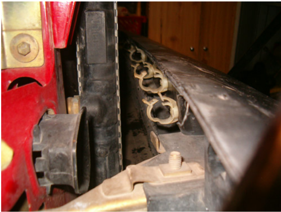
Attach the plastic keepers for the washers hose (6 in total)
