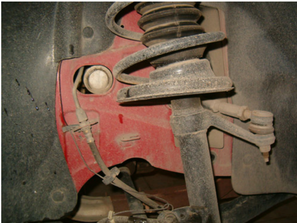
Let's now move lower to remove the plastic wheel arch liner
