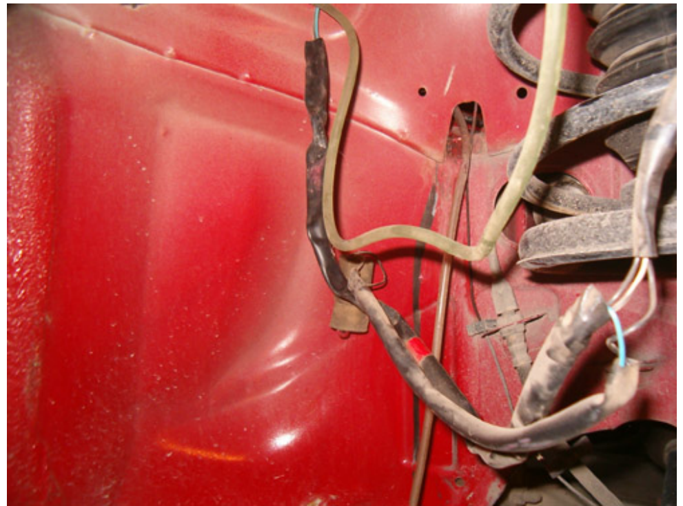
The already existing wiring is now exposed along with the washing fluid supply line
