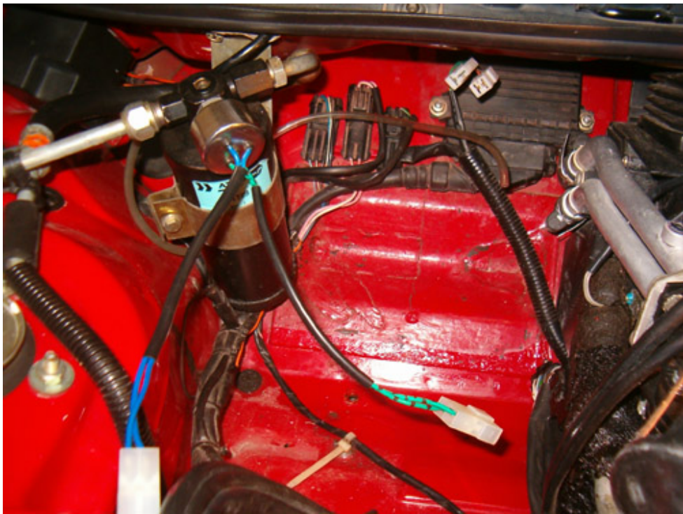
Remove battery along with its support frame.
