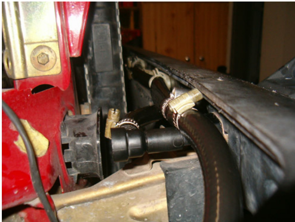
Time to measure the length of the hose and attach it to the headlight washers
