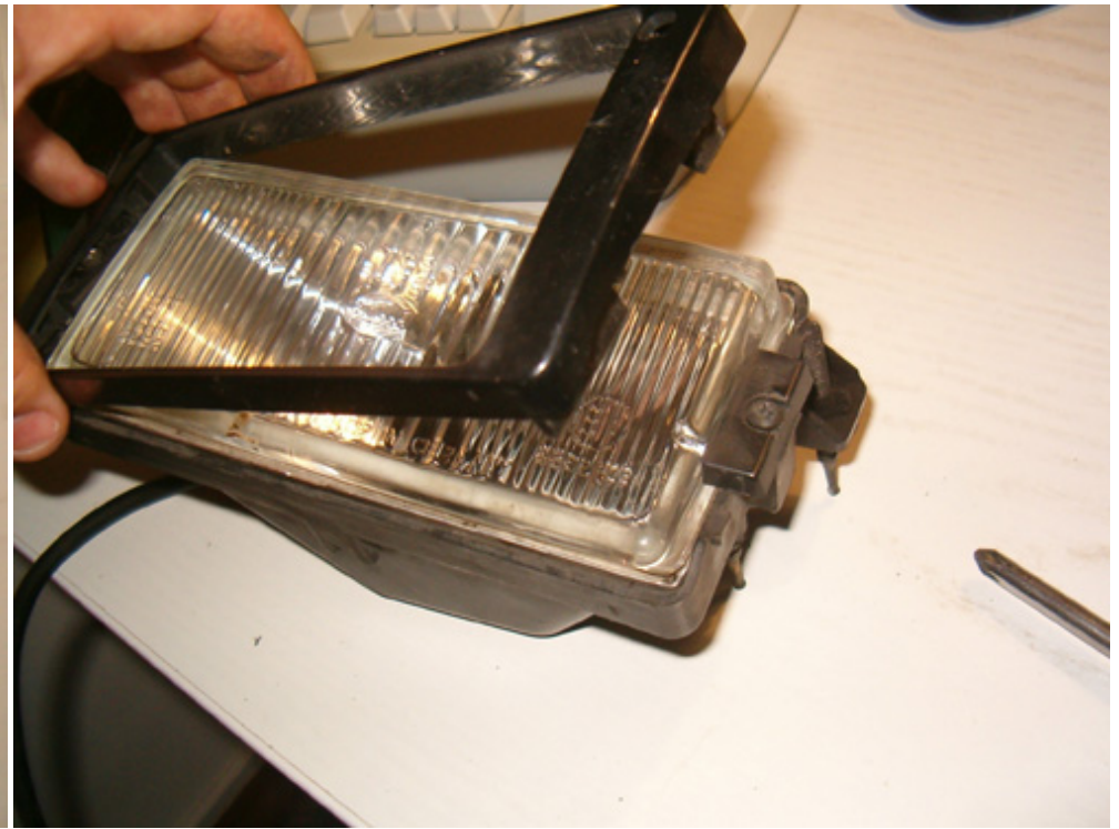
Remove the frame by carefully releasing the plastic clips
