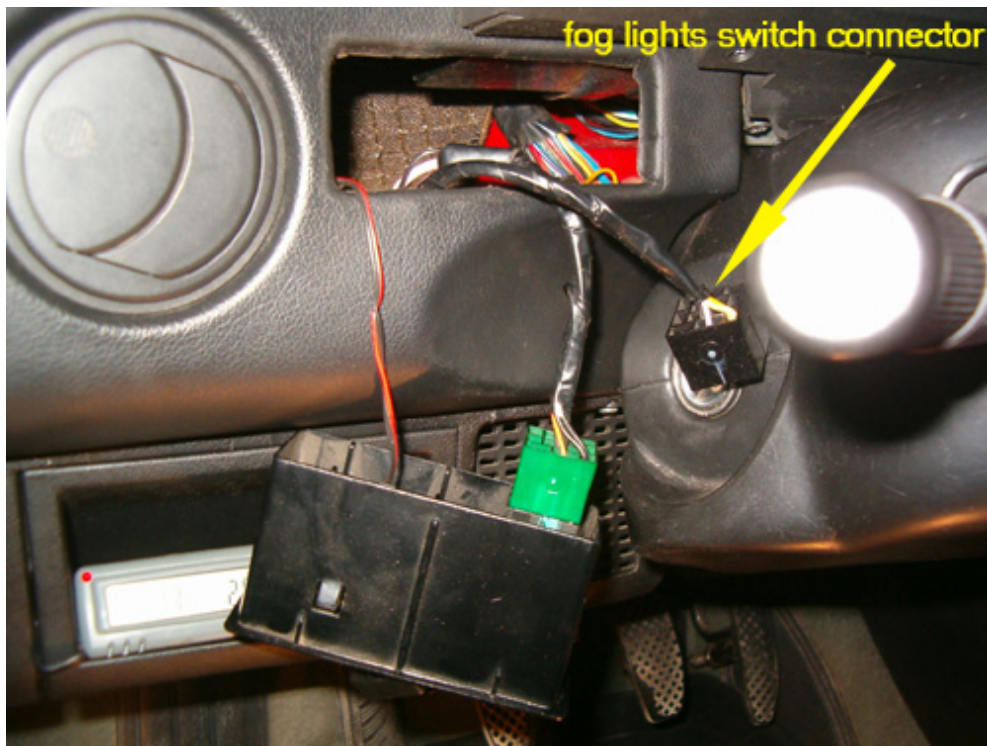
Remove the switches cluster and locate the fog lights wiring connector.
