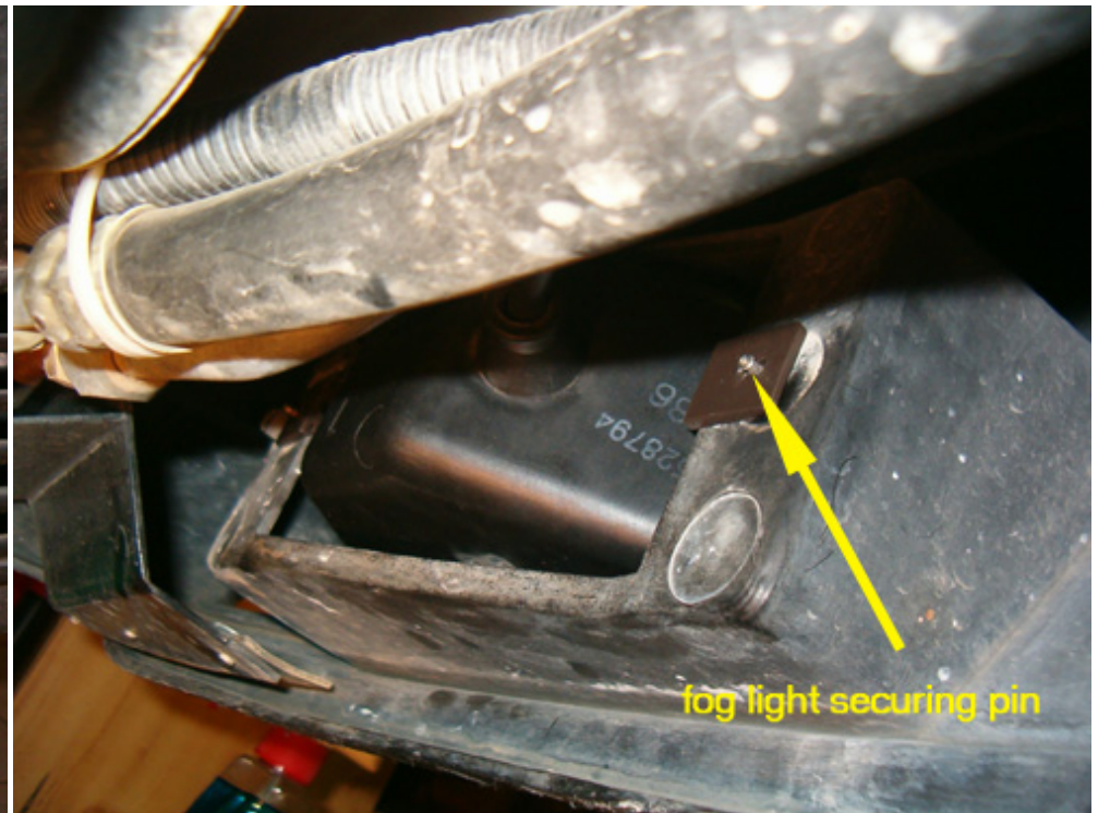
... and light cluster is finally installed for good. In order to be sure that the cluster is firmly attached, make sure that the tip of the pin barely extrudes from the securing clip at all three brackets.
