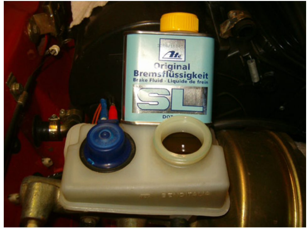
Now top up the brake fluid in the container ...
