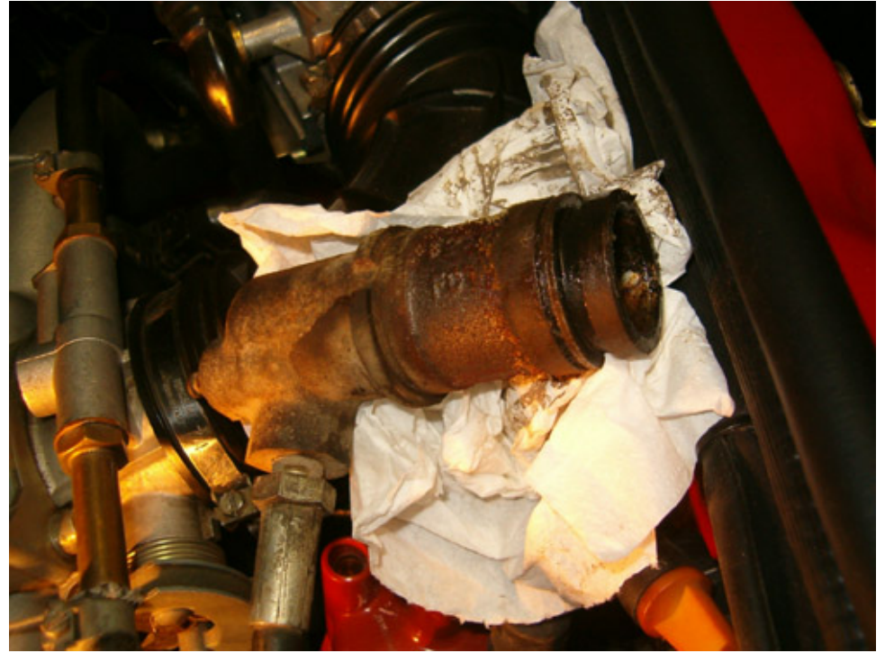
... and clutch cylinder is out at last!
