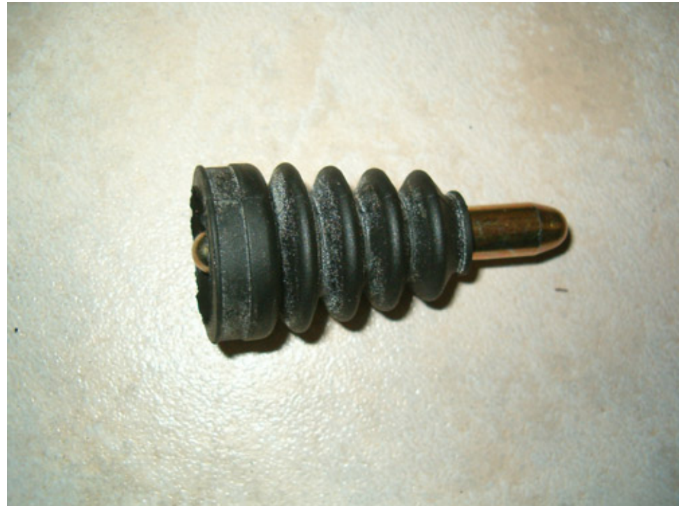
Lets now finish installation by attaching the pin along with the rubber boot.
