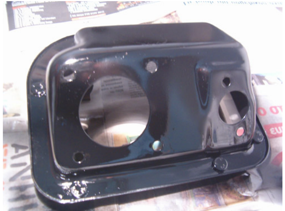
The corrosion has been removed and the pedal shell is now freshly re-sprayed
