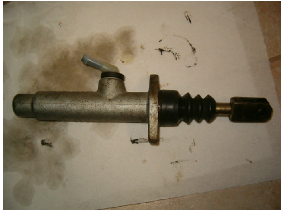
Remove the old clutch master cylinder ...
