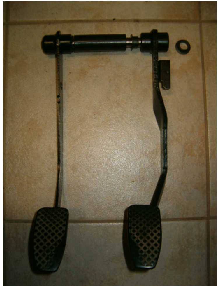
Pedals are now removed and thoroughly cleaned from old grease and residual dirt
