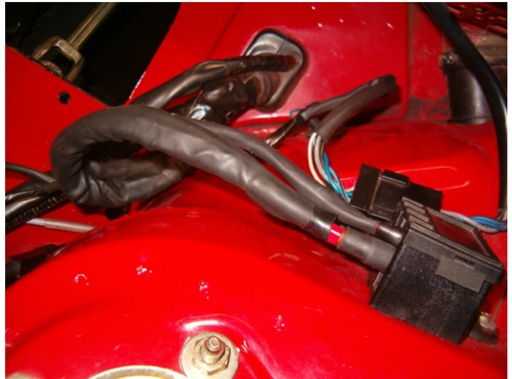
I have used a heat gun to warm up the tubes - this is the final result.
