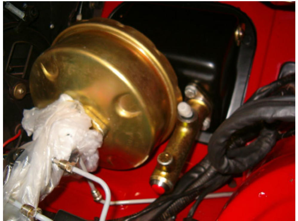
Then install brake servo along with clutch master cylinder
