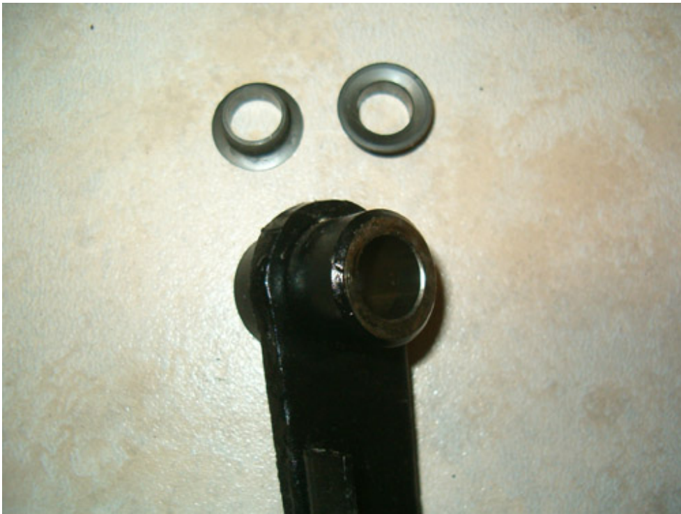
A close up of the pedal shaft and its bushings. Be careful with these bushings as they are plastic and an NLA (No Longer Available) item.
