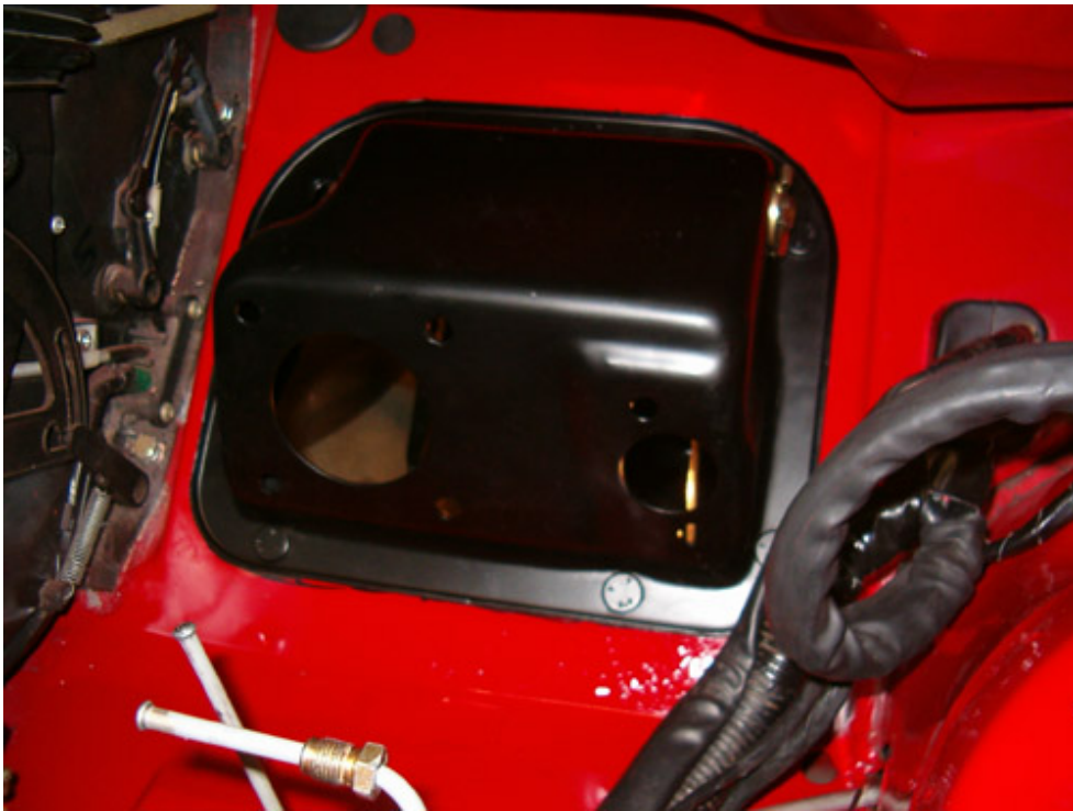
Install the pedal case and fully tighten the 6 retaining nuts in cross order.
