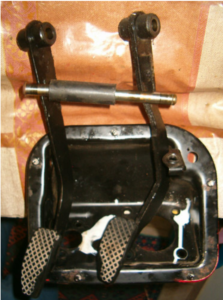
Pedals are now removed and thoroughly cleaned from old grease and residual dirt
