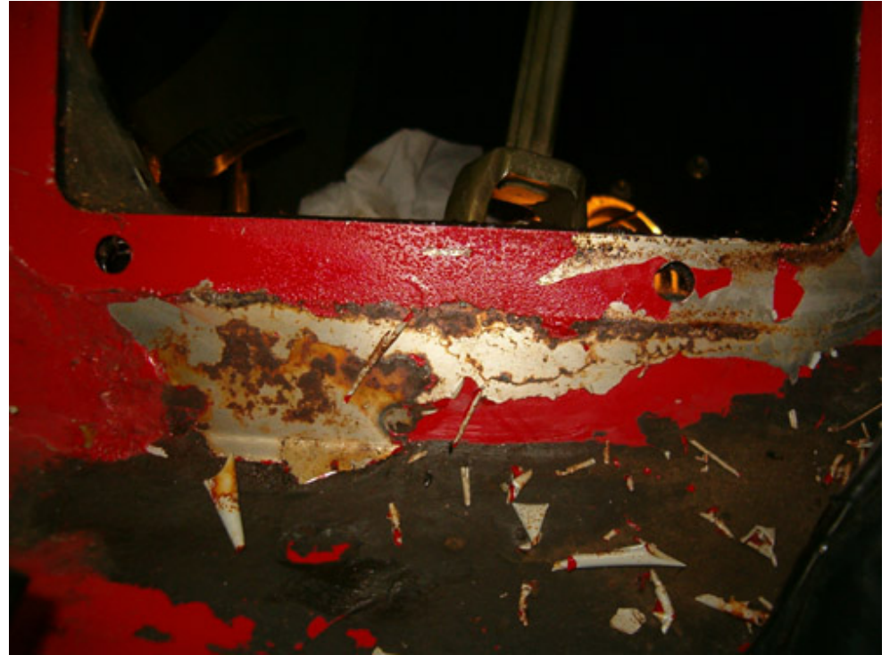
Notice the extend of corrosion... Don't worry this will look like new in a short time!
