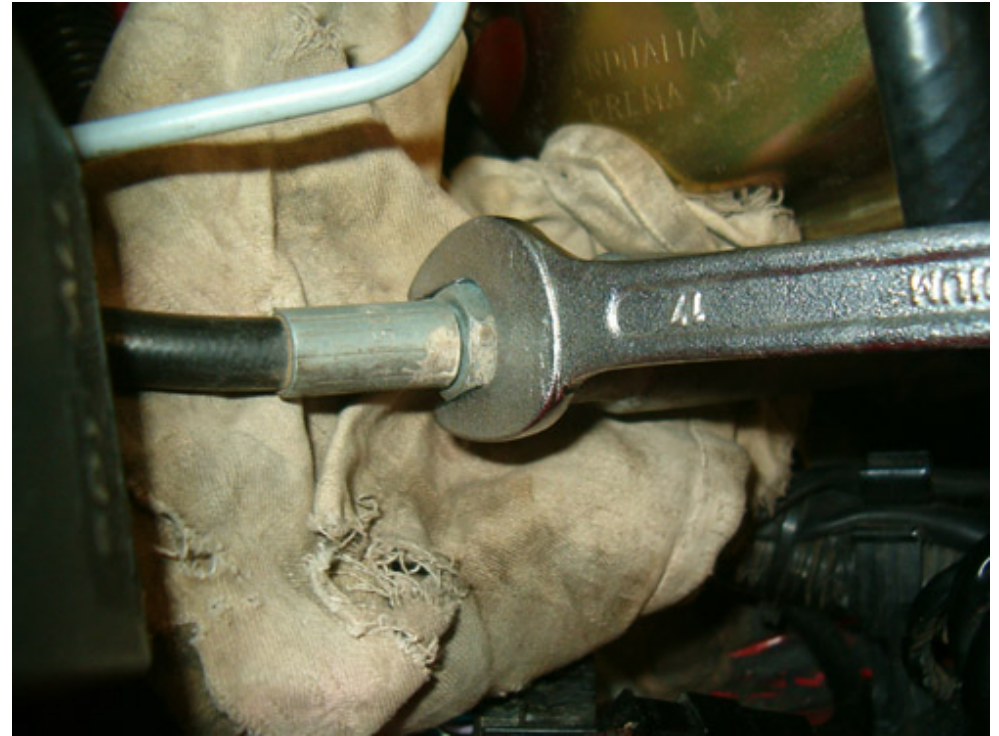
Using a 17mm wrench undo the slave cylinder hose. Be careful and place rags under the cylinder in order to protect the paintwork from brake fluid slippage.
