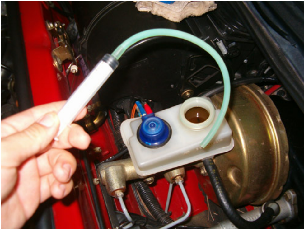
Remove all brake fluid with a syringe
