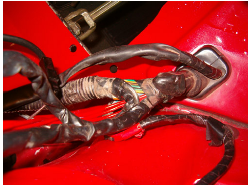
Time to sort the wiring harness a little bit. Be sure to disconnect the battery positive pole.
