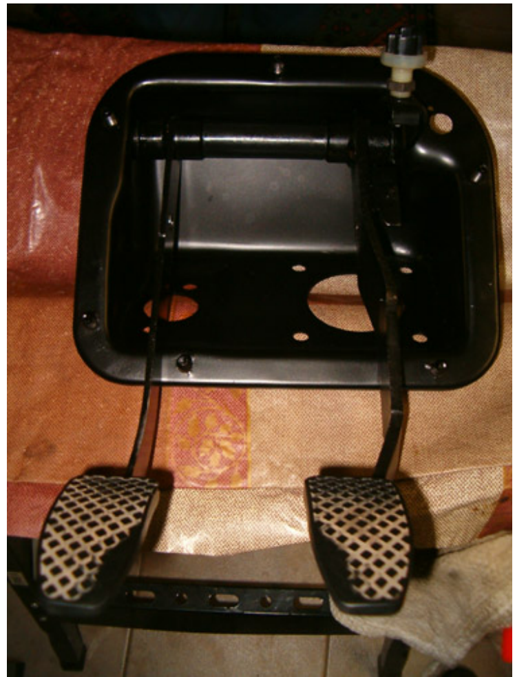
Install middle tube and finally the clutch pedal. Secure the pedals with the lock washer
