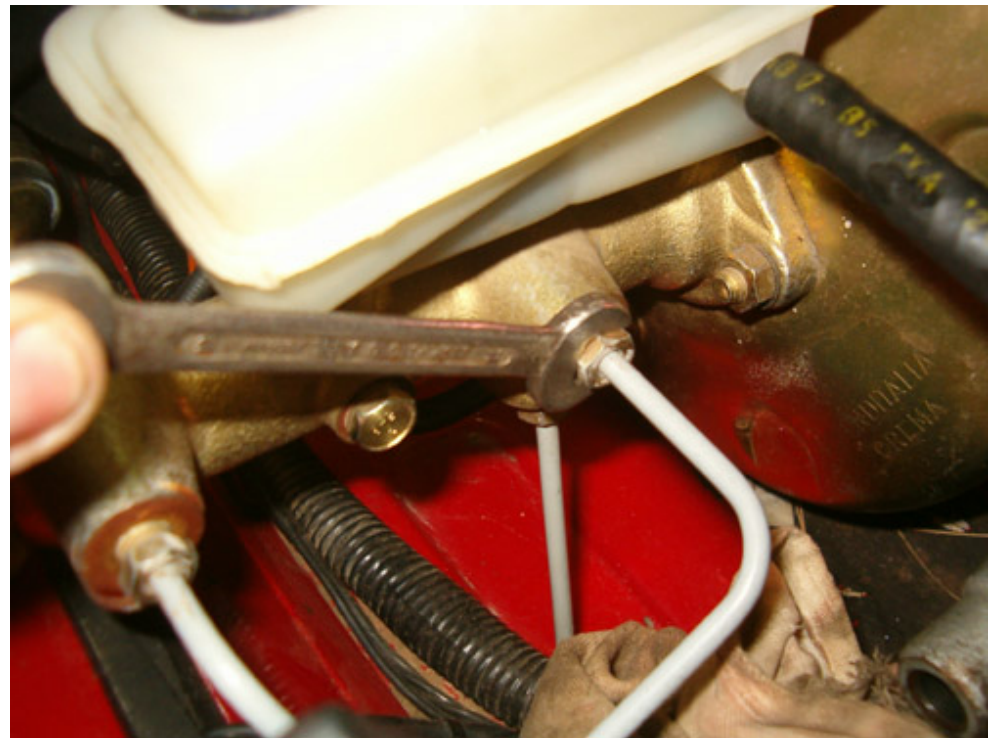
With a 10mm wrench undo the 3 nuts securing brake lines to brake cylinder
