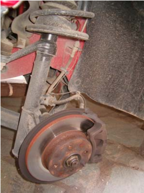
This is how the fenderwell looks without a wheel
