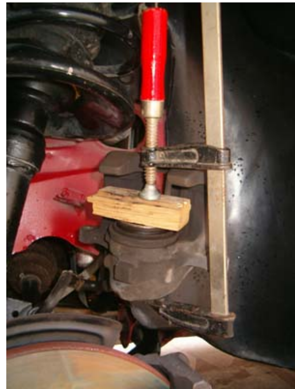
A small piece of wood and a carpenter's brace is perfect
