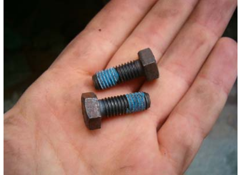
These are the new screws that will bolt on the fixed part of the caliper
