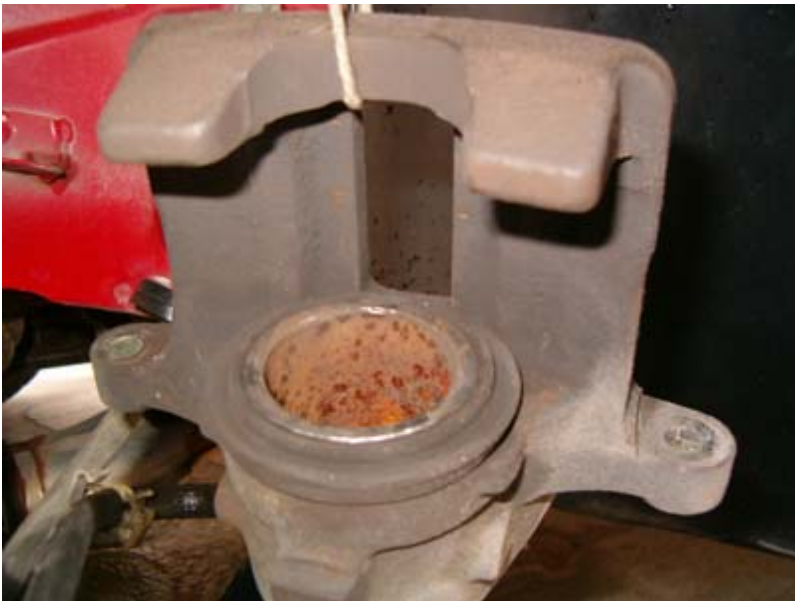
Now we need to do something in order to push inside the brake piston
