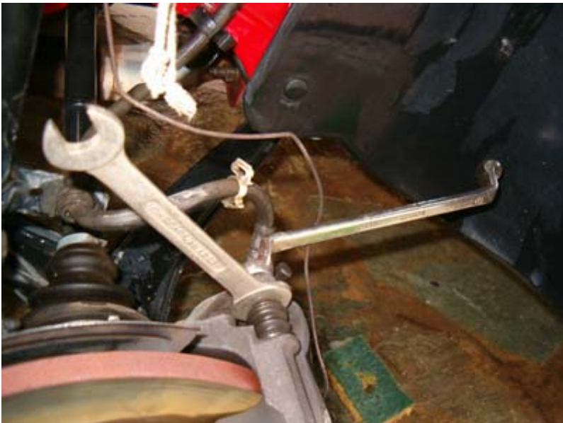
you don't have to remove the clip - simply remove the cable by passing it through
