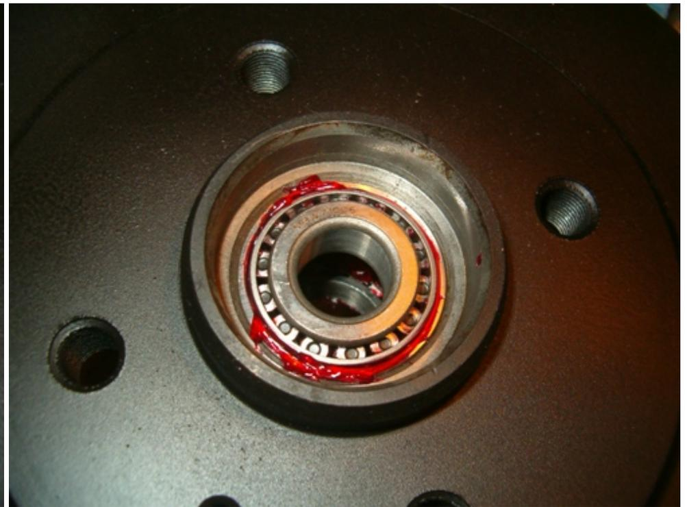
Do the same for the outer bearing. Apply grease in the bearing ring...
