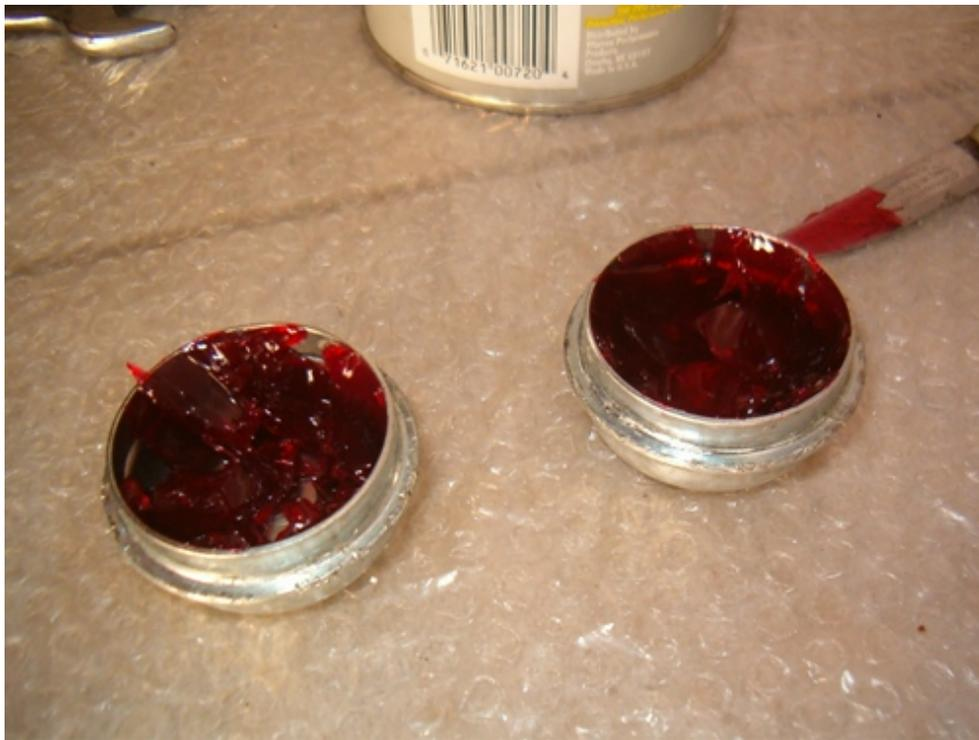
and apply some grease on the axle nut covers
