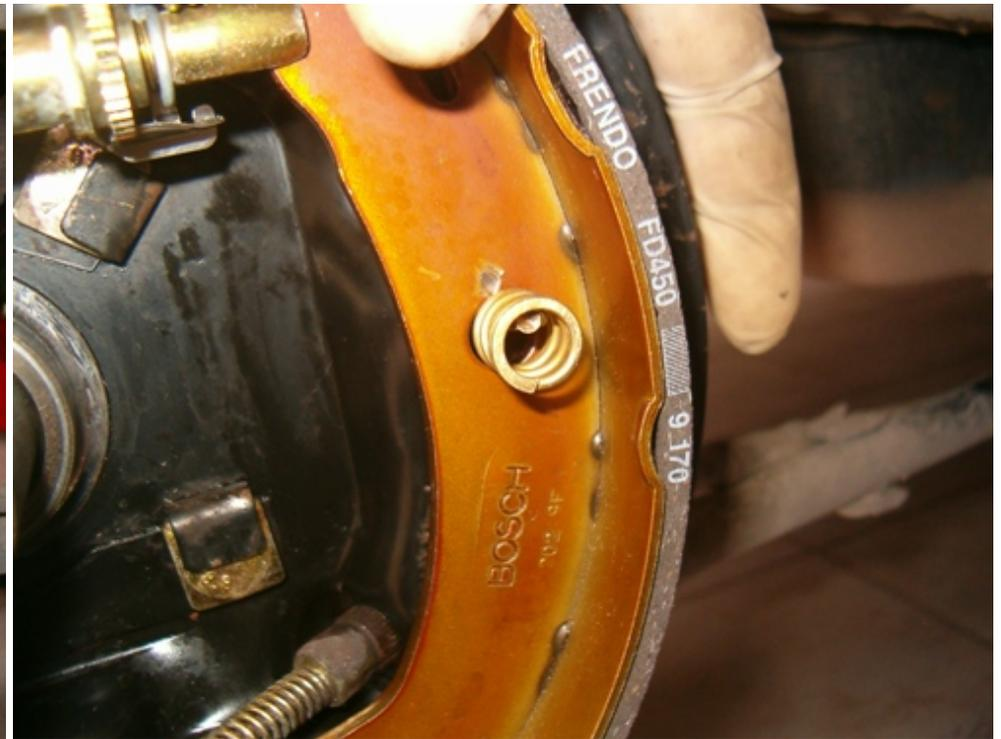
Install pin with direction from the rear cover, install spring....
