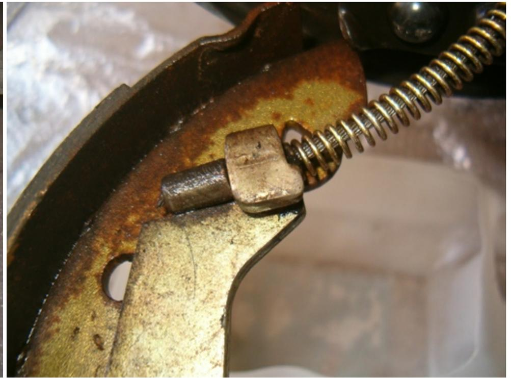
Once out the parking brake cable is exposed. remove it in order to free the jaws.
