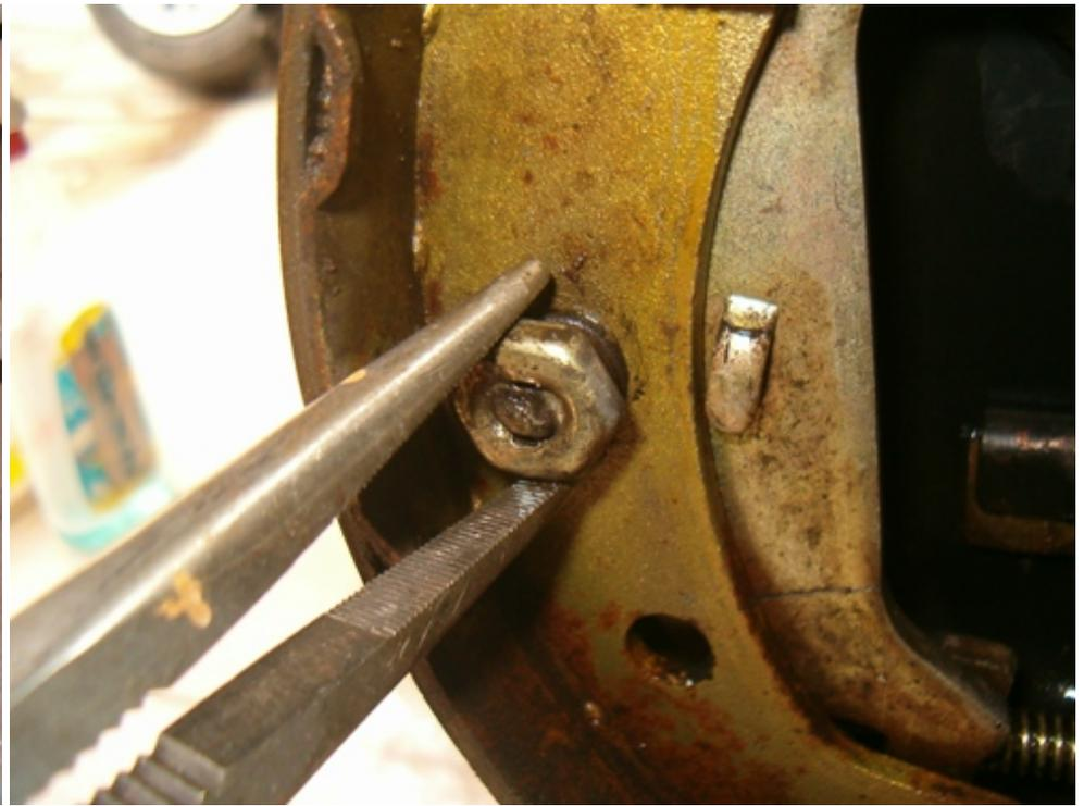
Using a set of pliers remove brake jaws locking nuts. These nuts are used to keep the jaws firmly attached to the drum rear cover.
