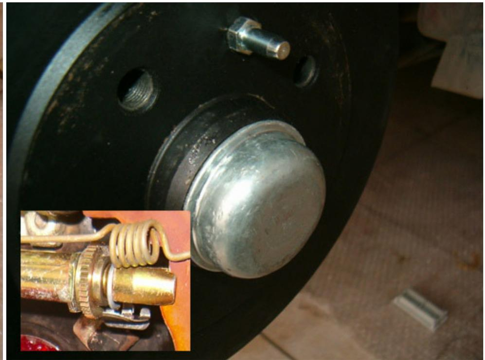
Press the cover in and lets now proceed in adjusting the brake jaws
