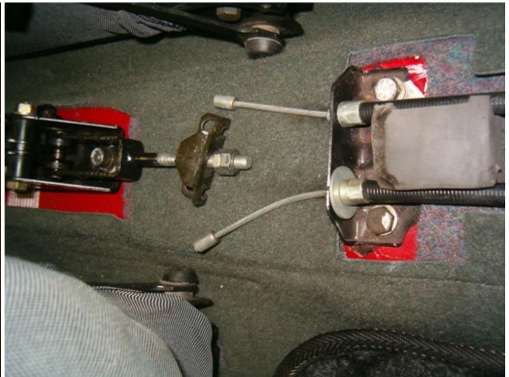
Let's now move on to the rear axle. Remove handbrake trim and fully release the parking brake cables
