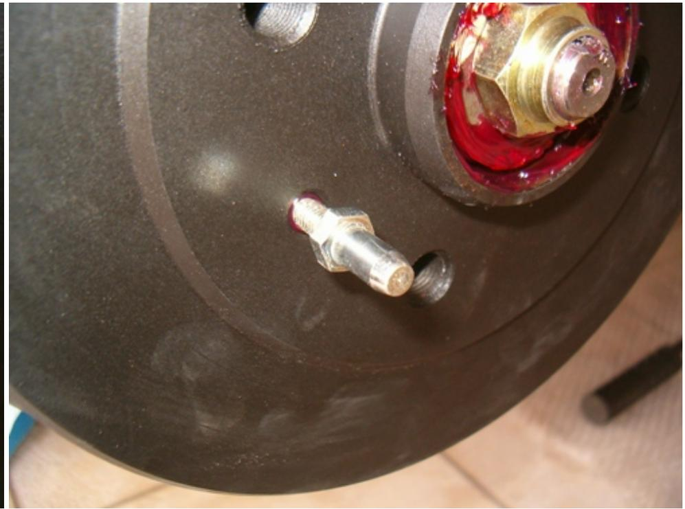
Again apply grease around the axle nut. Tighten the axle nut at the specified torque (25-29 Nm) and in the mean time rotate (CW & CCW) the drum several times in order the bearings seat in their position correctly. Then slightly slacken the nut, hit the axle with a rubber mallet and then punch the nut in order to lock it; be careful so that the nut does not lose its position.
