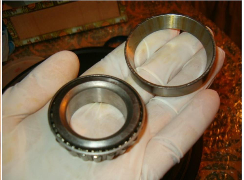
A close-up of the bearing. It consists of the actual bearing and the bearing ring. This ring should be replaced along with the bearing as the inner surface wears out.
