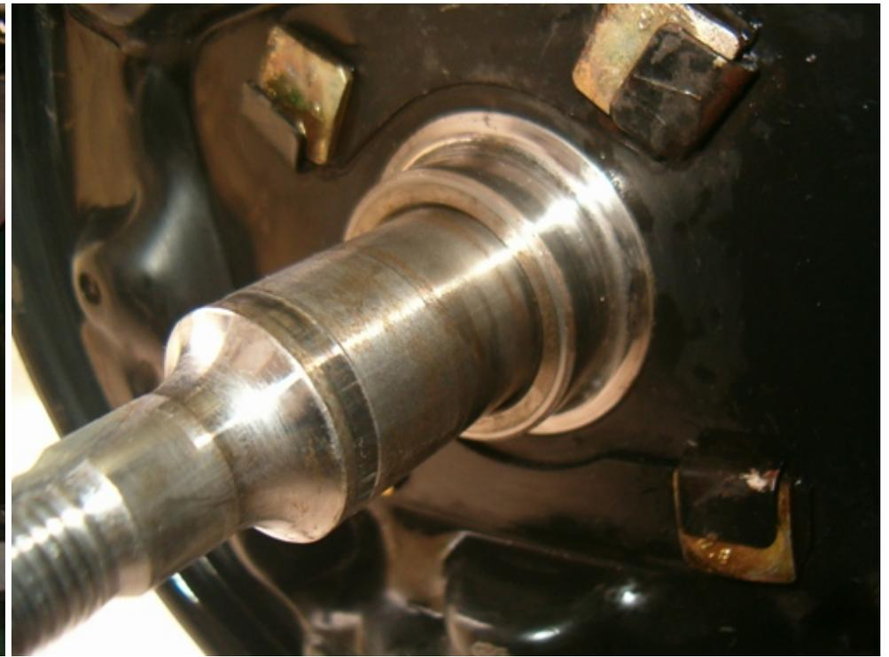
Be sure to have the axle thoroughly cleaned as any trace of dirt may ruin the bearings
