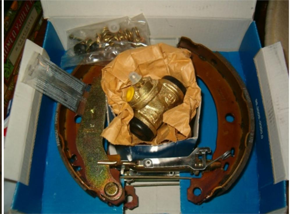
and a complete set of rear jaws. Package includes wheel cylinder, jaws, regulator and new lock rings/springs and pins
