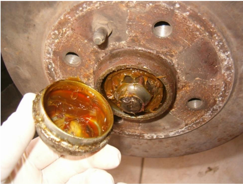
Remove dust cover, axle nut and drum.
