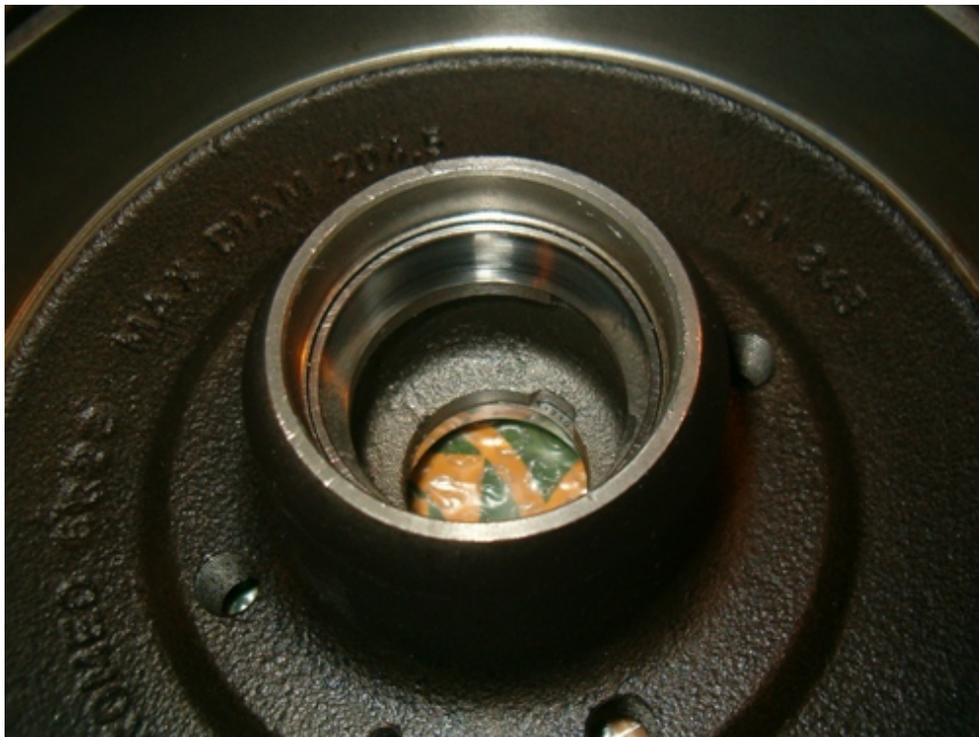
Since I had new drums on my hands, the bearing rings come integrated on the drum, so there was no reason to bother pressing them in. Before applying grease clean the surface with alcohol as it has an oily film from production; oil is used as a rust preventative measure so it is advisable to remove any trace.
