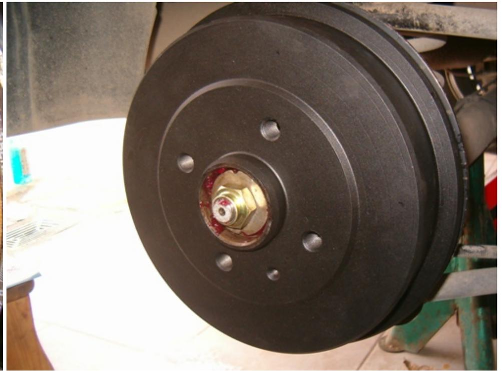
Apply grease to the axle and install drum along with relative washer and axle nut
