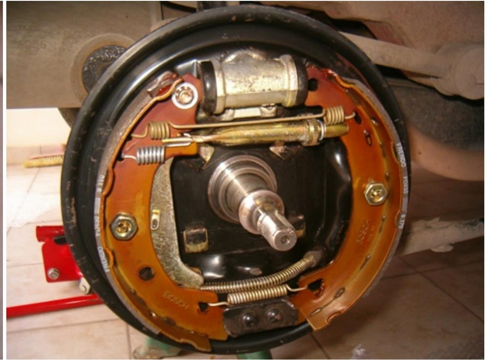
and last but not least the locking ring which keeps the jaws attached to the rear cover
