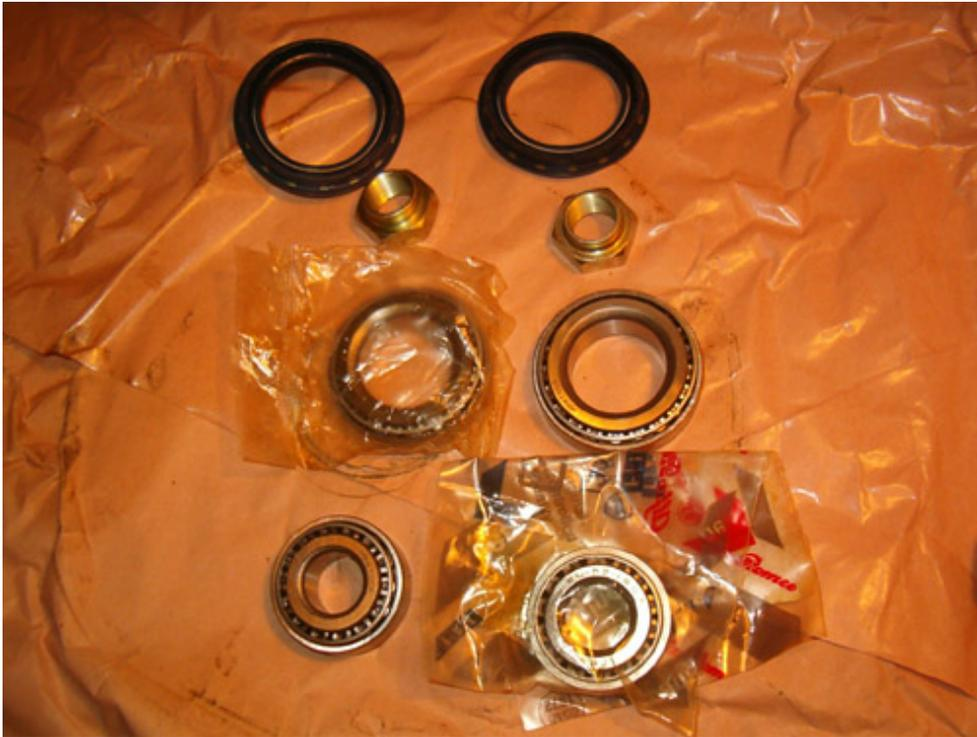
This is the wheel bearing kit consisting of inner and outer bearing, dust seal and axle nut.
