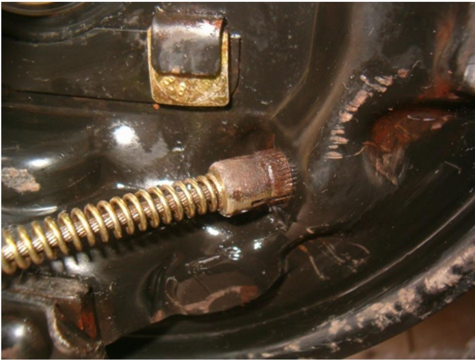
Lubricate the parking brake cable...
