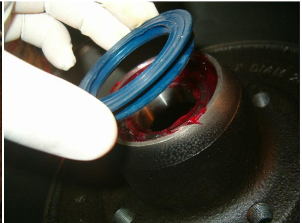
Apply grease and proceed in fitting the dust seal
