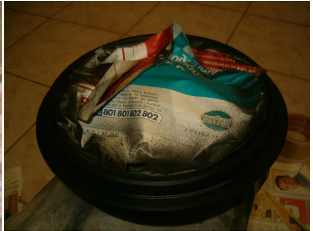
Painted the outside taking care paint does not enter the bearings cavity
