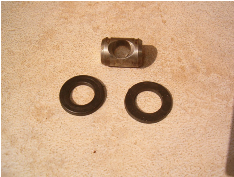
The metal rod you see above is actually the proximity of the spring. Road dirt gets inside the rod and results in metal to metal rubbing hence the funky sound.
