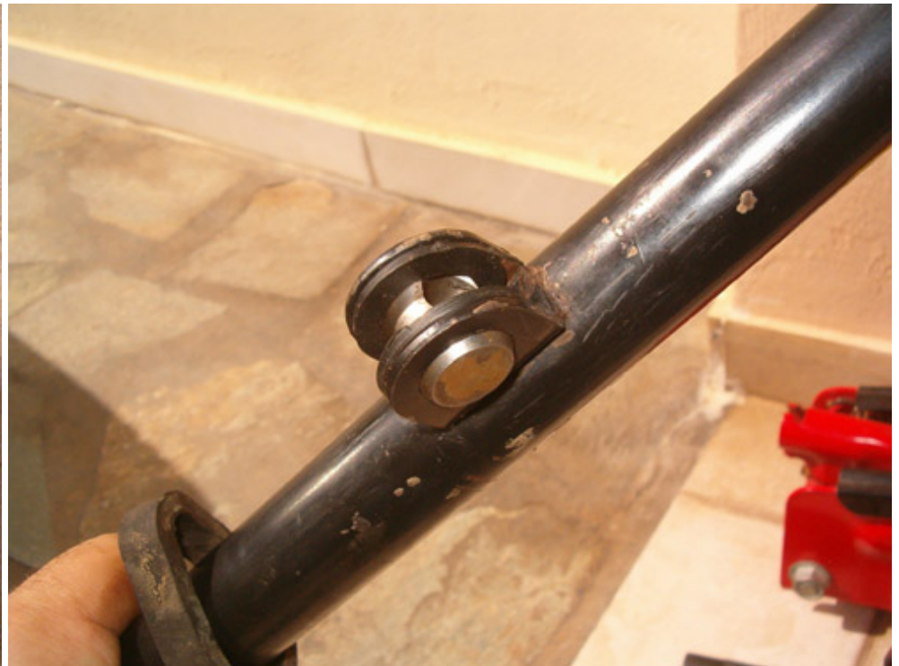
I have used new rubber pads which will keep the spring seated correctly.
