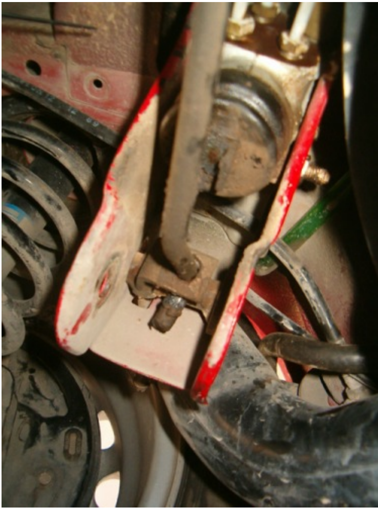
Once the Panhard bar is out of the way the adjustment hook is seen on the end of the spring.
