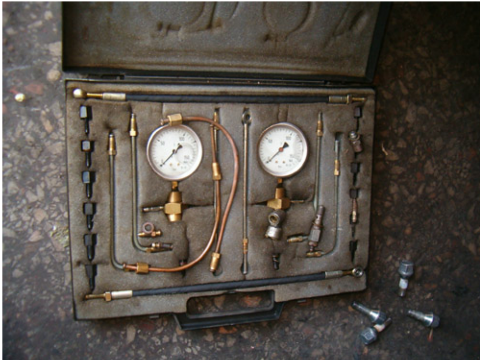
Here you can see the special gauges that measure brake force. It comprises of all the proper gear to check every single part of the brake hydraulics.
