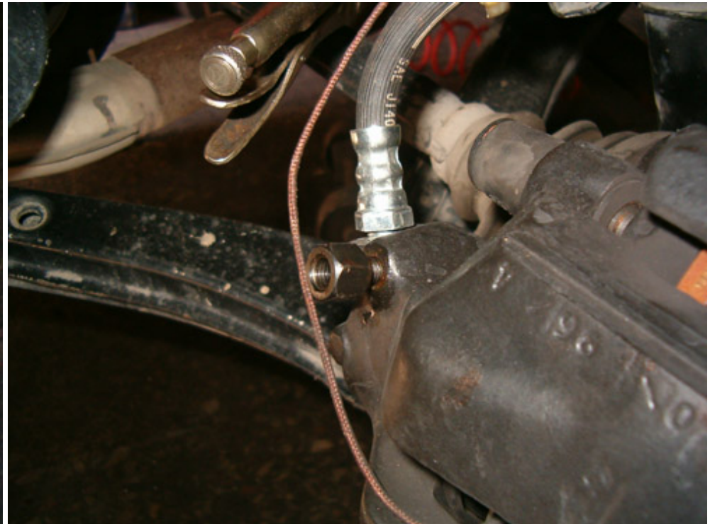
The bleeding nipple has been removed and an adaptor has been placed where the gauge will be attached
