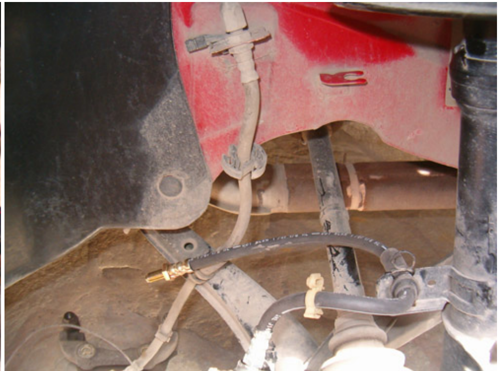
Install spring attaching hose to strut and all the relative plastic holders
