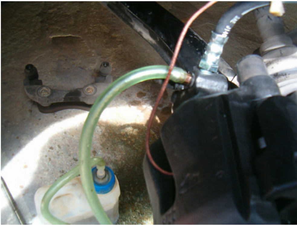
Then bleed the caliper until clean fluid free of air bubbles come out.
