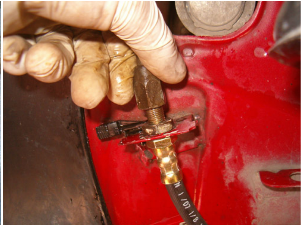
Proceed attaching brake pipe union to brake hose and fully tighten it.
