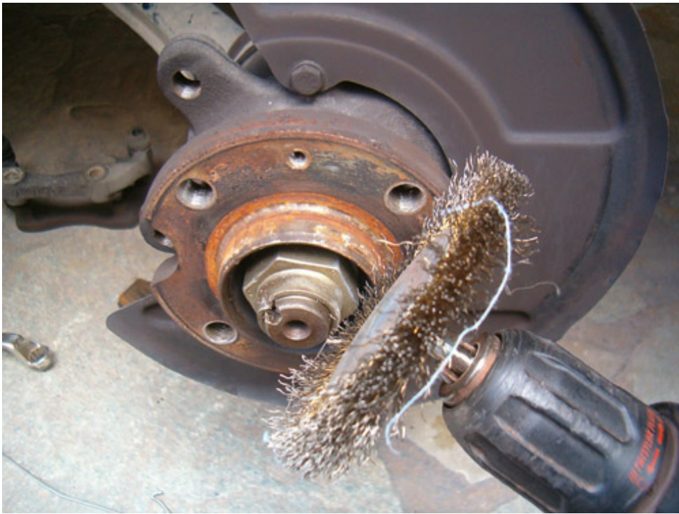
Here you can see the wheel hub; I have chosen to remove loose rust using the wire brush and applying a layer of oil to prevent rust
