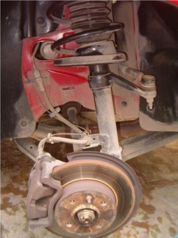
Here you can see the original setup; solid disks with Bendix/Girling calipers
