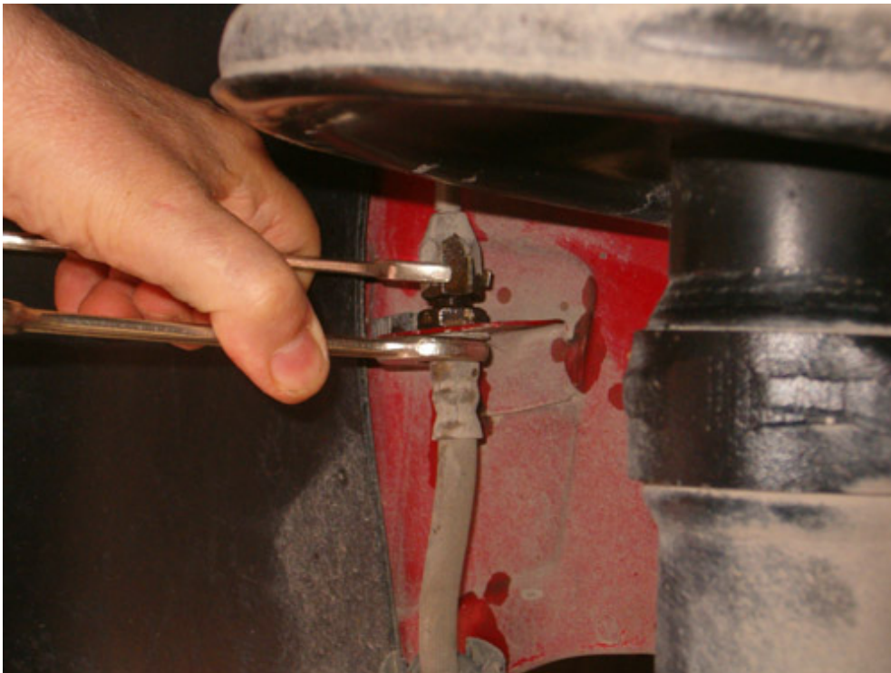
and then undo the brake pipe union to brake hose
