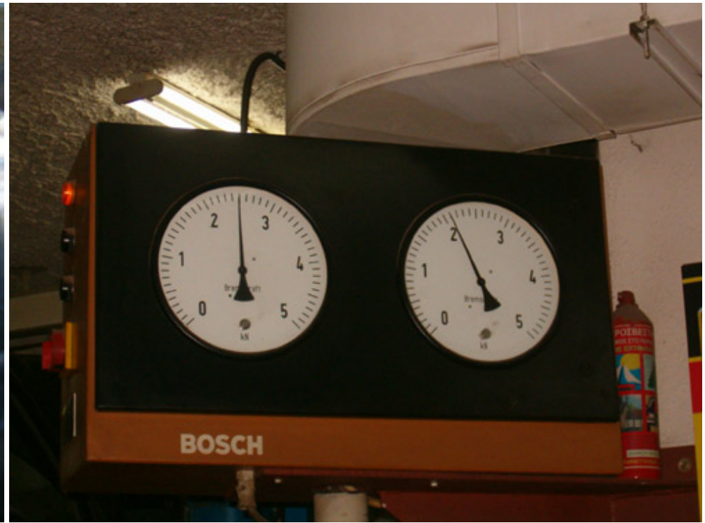
After some hundreds of Kms letting the brake pads/disk bed in I felt that the brakes still drag... This is the proof as the right wheel is ~400N less than the left one.
