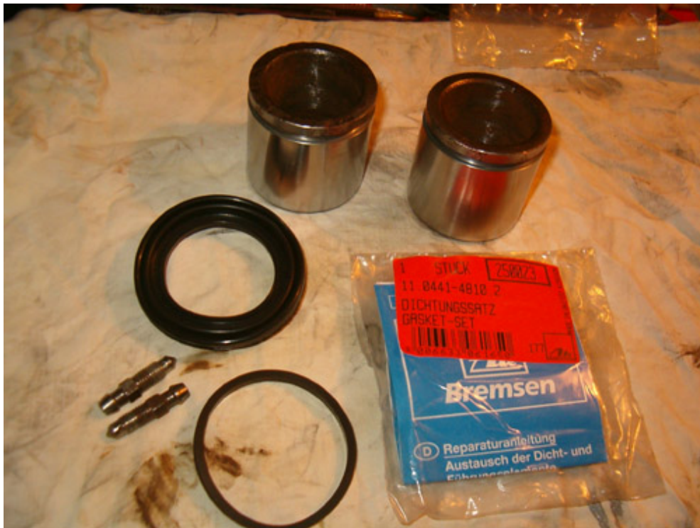
Here is the repair kit; ATE 0441-4810 is the part number for the Alfa 33 16V calipers
