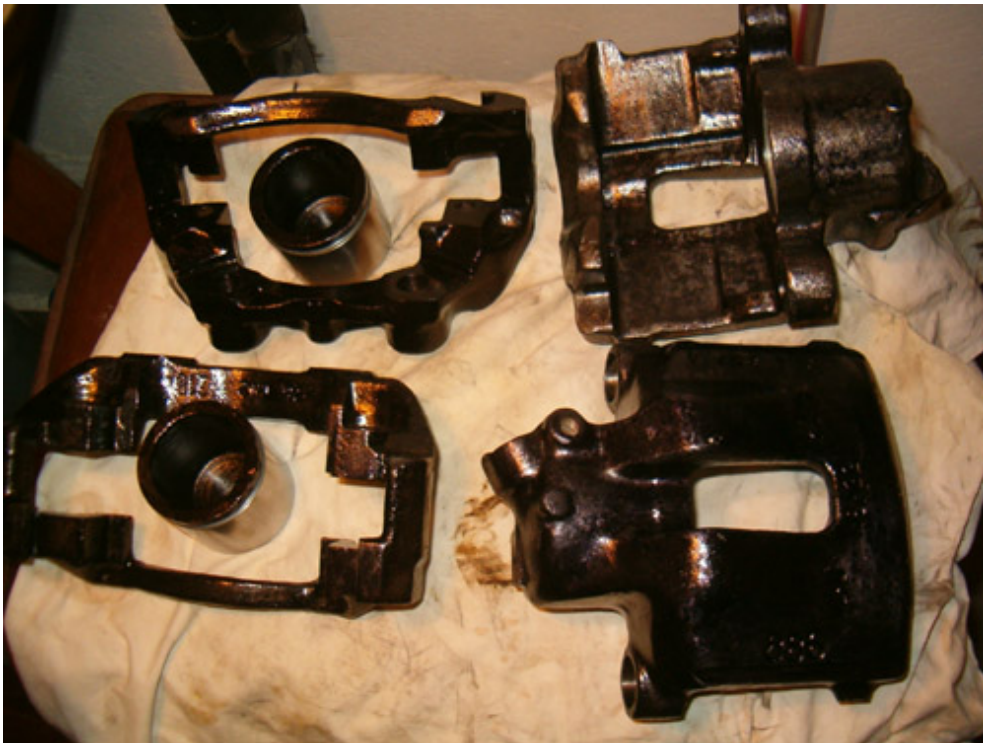
All parts are now treated with rust inhibitor
