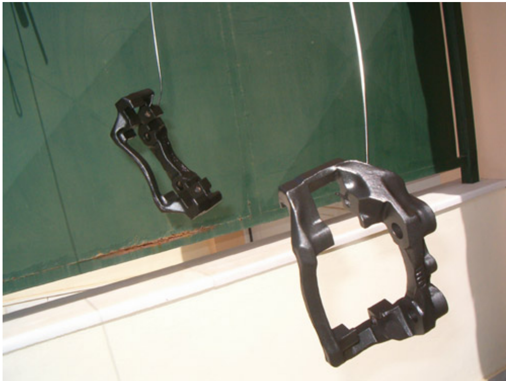
Caliper brackets painted along with the piston internals
