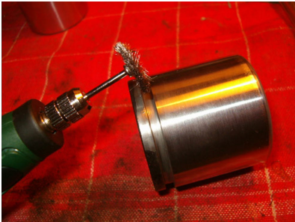
Using the small wire brush on the Dremel tool, I have removed any leftover traces of foreign material
