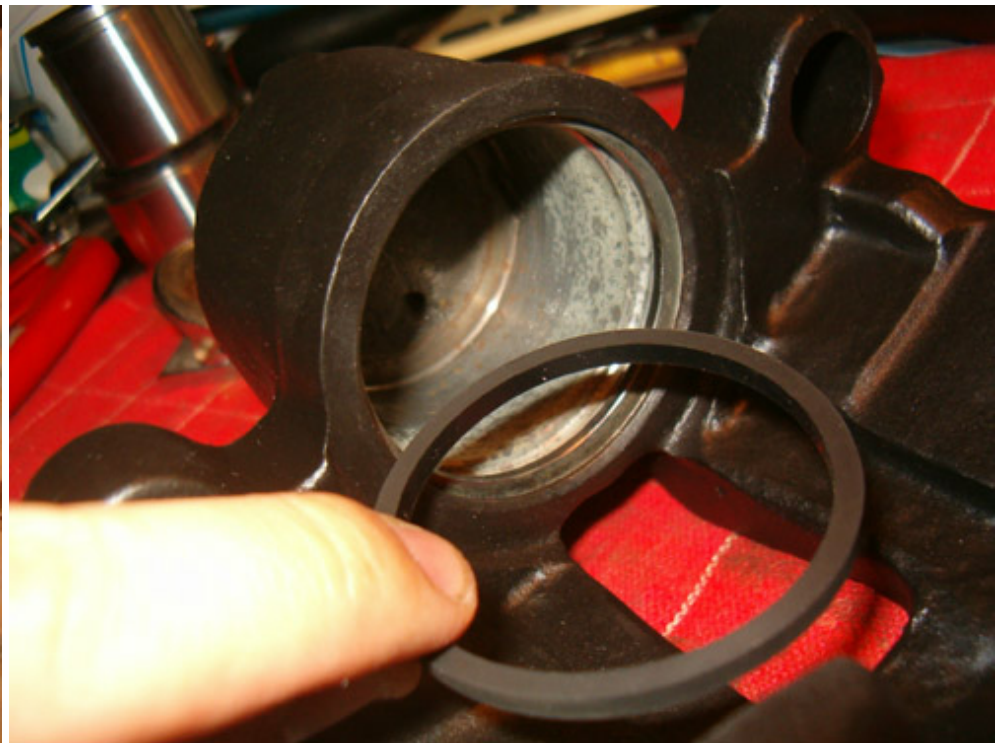
Install the piston seal on the cylinder
