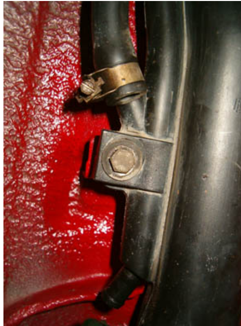
Don't forget the fuel vapor hose (upper and lower).
