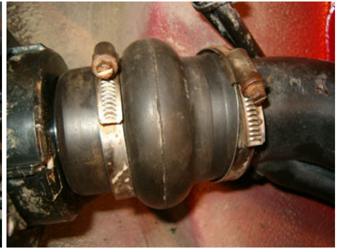
... and finally install the fuel cap boot in its final position.
