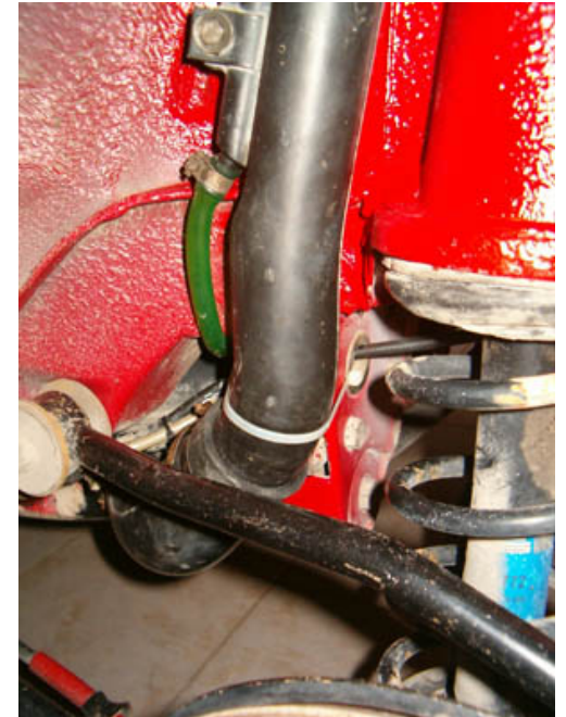
What remains is to keep the tube firm at its lower part. A long cable tie will do the job as shown in the picture; this is the way the factory had done; I have not deviated from any step.
