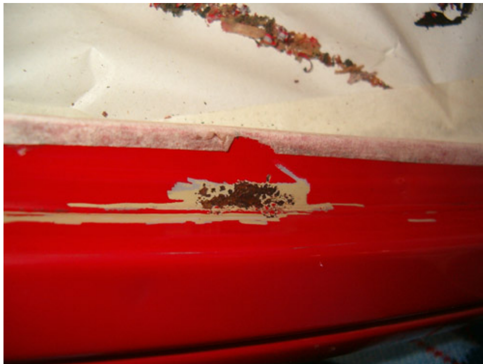
Another rust spot on the A-pillar post
