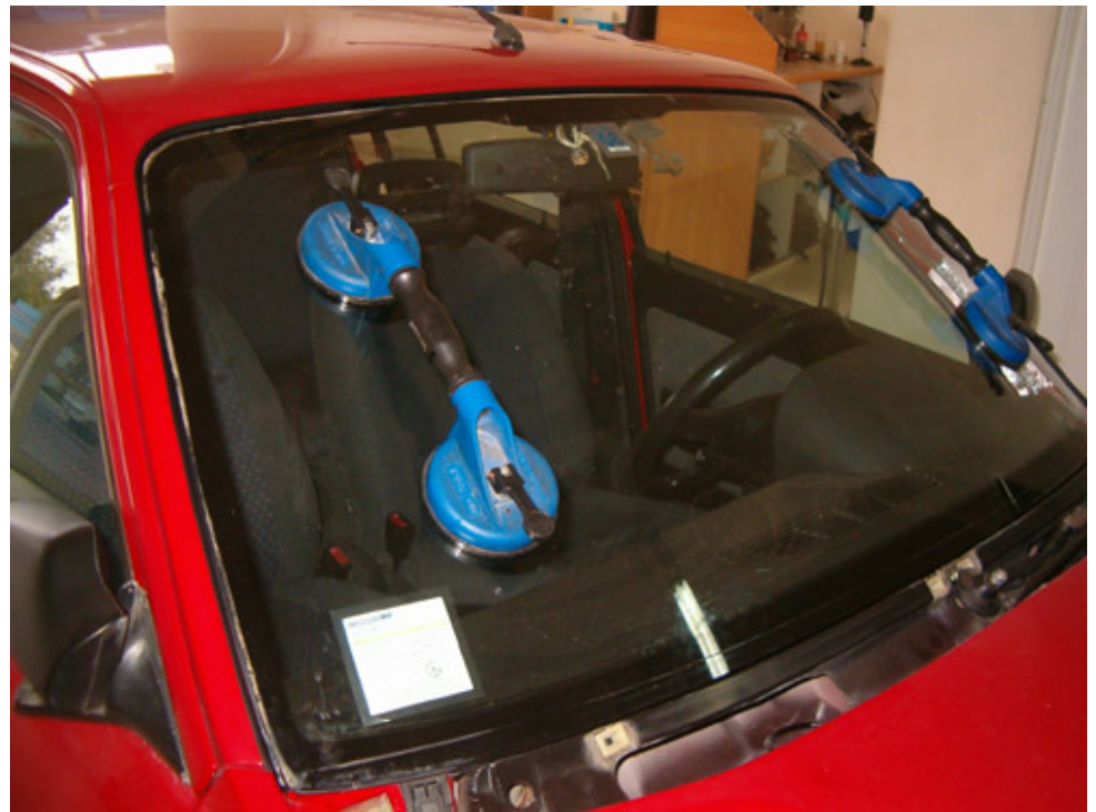
The windscreen gaps around the frame are now adjusted and the plastic stops on the bottom of the frame are locking the final position of the windscreen
