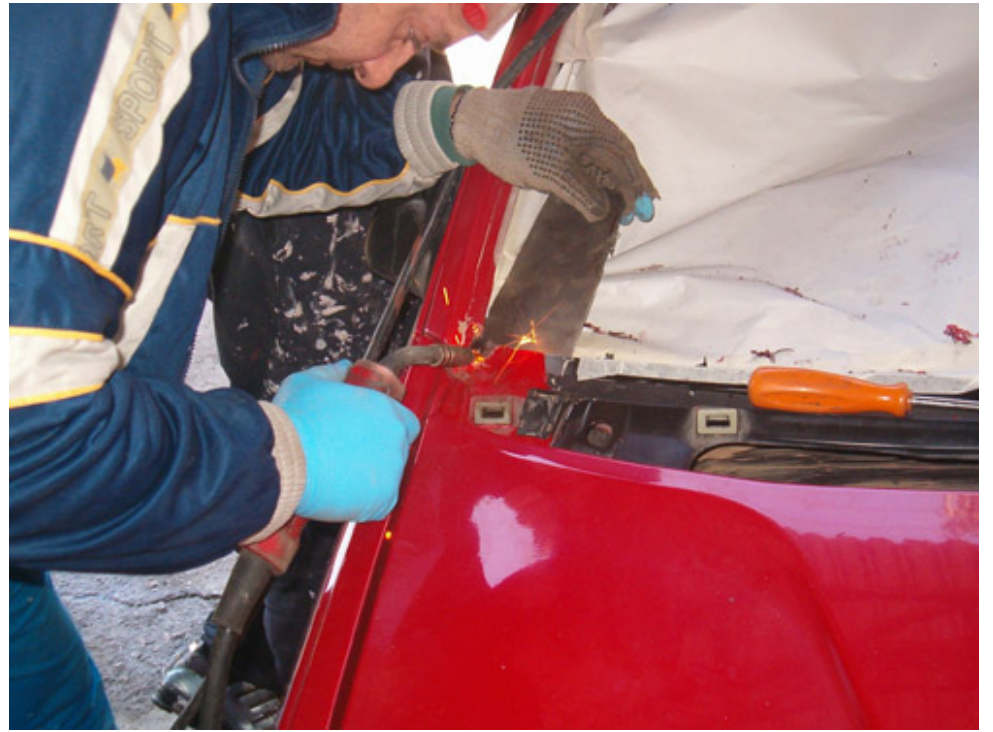
Apostolos decided to cure the rusted part by cutting it away and tack welding the gap...
