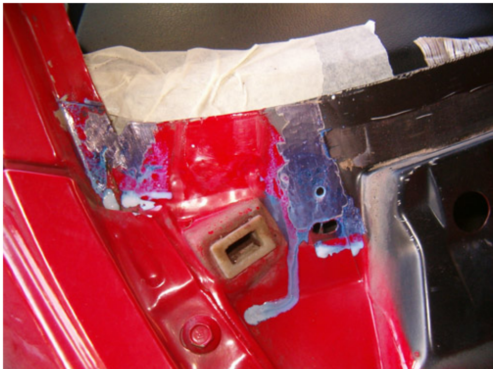
This milky fluid will convert to a black finish once it has bonded to the healthy metal
