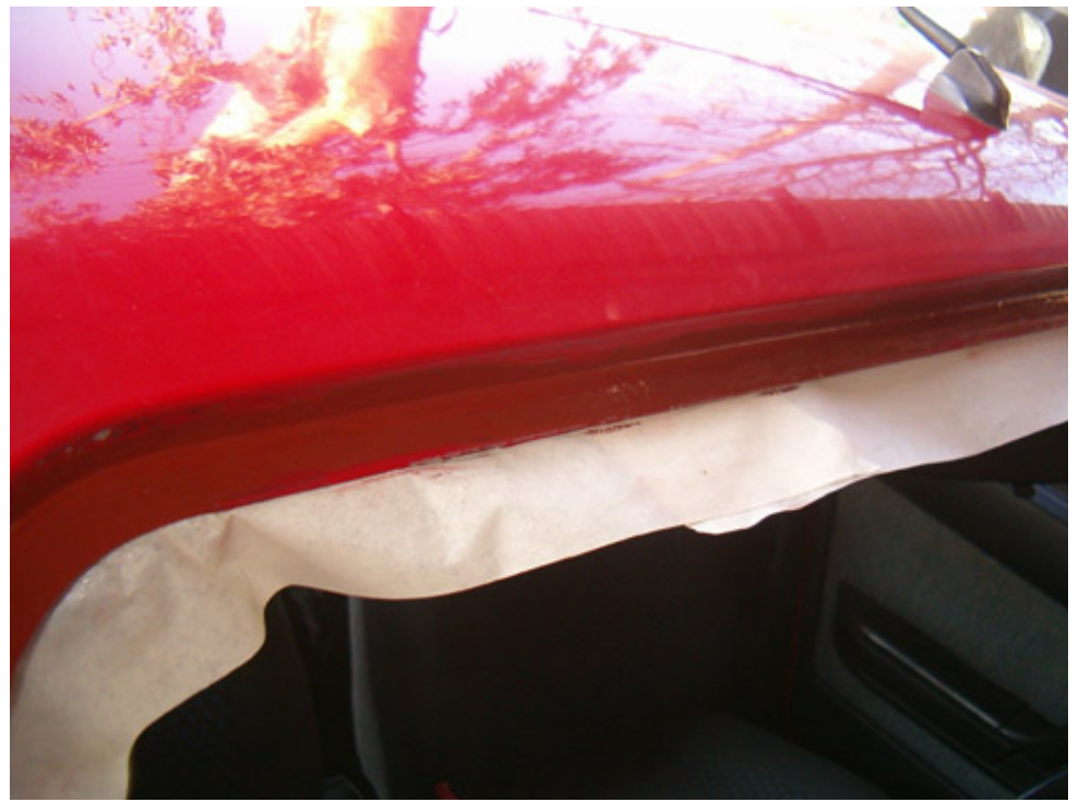
Primer is now applied
