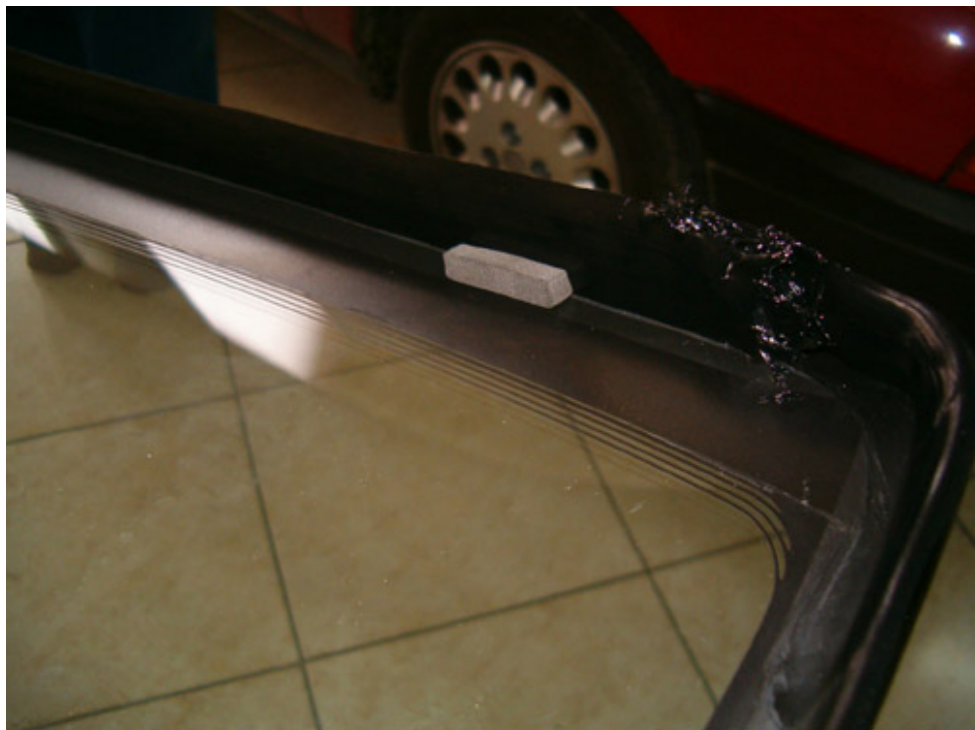
The glue has made a full round around the windscreen reaching the starting point.
