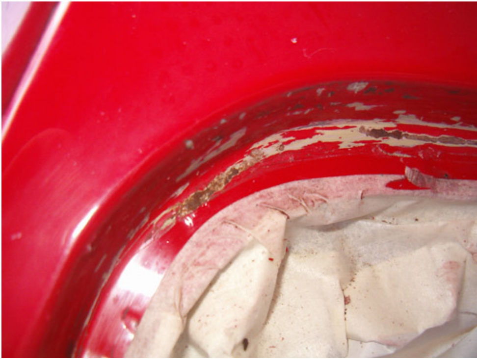
Rust on the upper right corner ...
