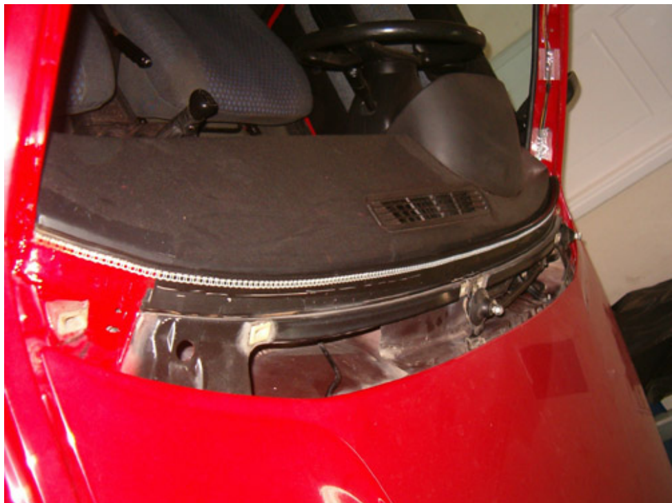
The decorative rubber element is installed...
