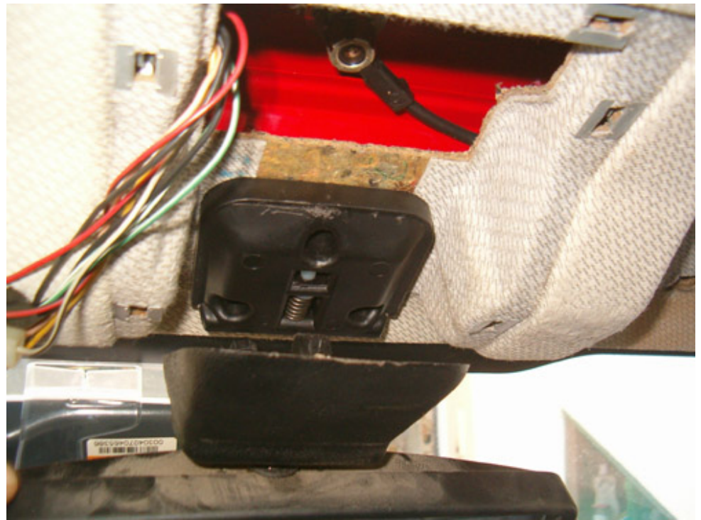
... pull the back view mirror out of its seat
