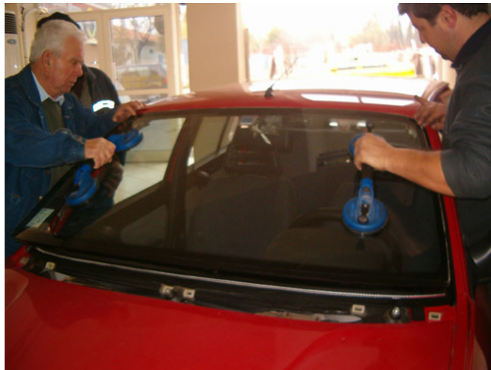
The suckers are now doing a nice job. Michael and his father are merely installing the windscreen.
