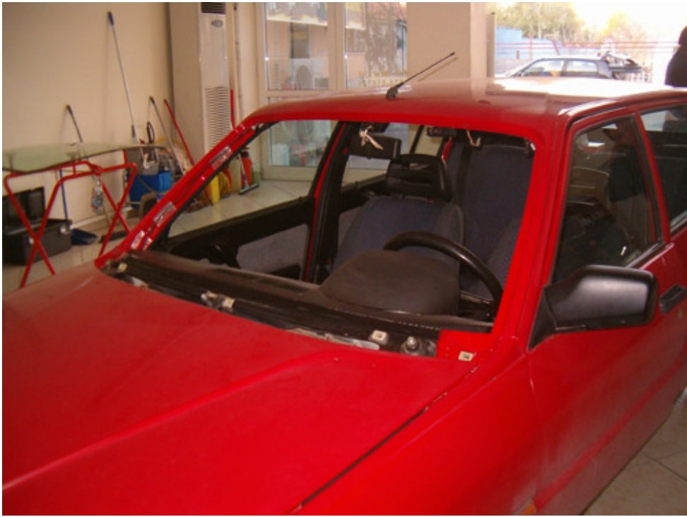
The 33 is now ready to have the windscreen installed. The windscreen expert has prepared the screen by removing traces of old glue.
