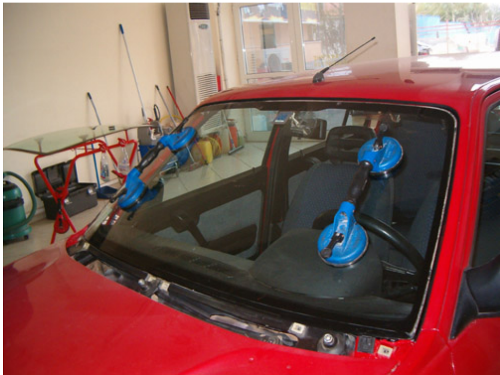
The windscreen gaps around the frame are now adjusted and the plastic stops on the bottom of the frame are locking the final position of the windscreen
