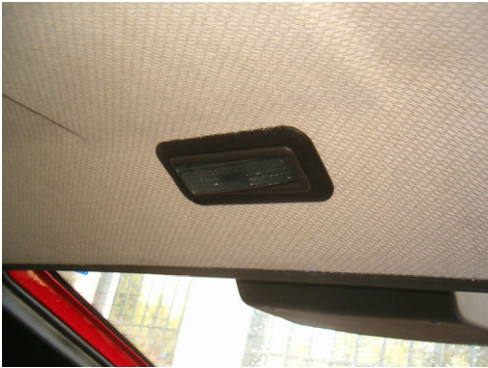
Go to the back and remove the rear interior light.
