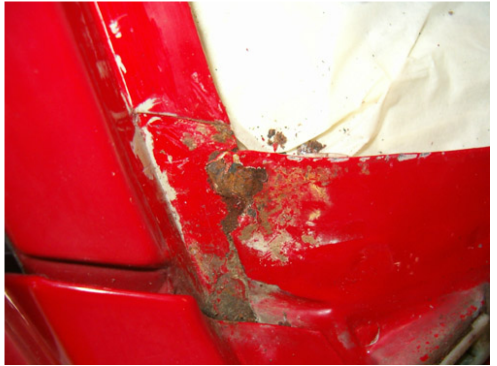
... and worst on the lower corner. Fortunately rust had not eaten away metal and no rust holes were required to fill up
