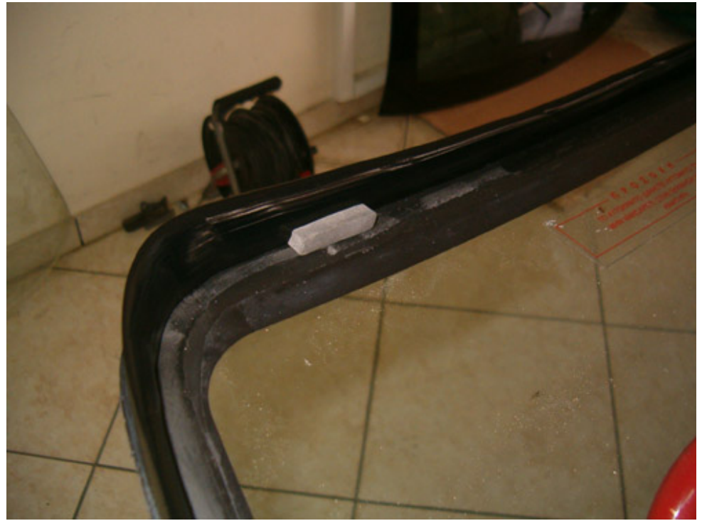
Michael has placed these rectangular pieces of rubber which will guide him regarding the level of the screen compared to the frame of the windscreen. We wouldn't want a windscreen that sits below the level of the frame.
