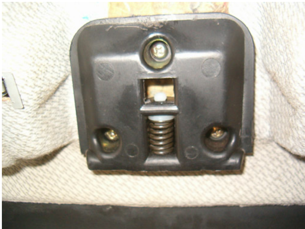
Finally undo the 3 screws attaching support plate to roof.
