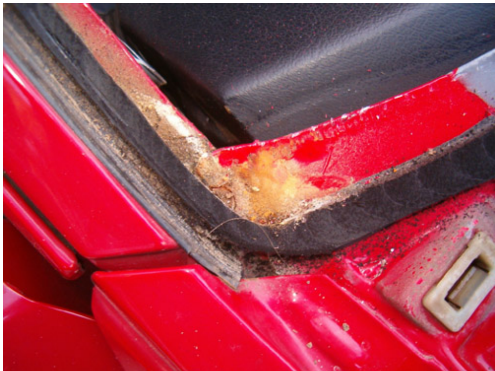
My fears were true ... brown metal in the corner. Looks like water was accumulating in this area causing the corner to develop rust
