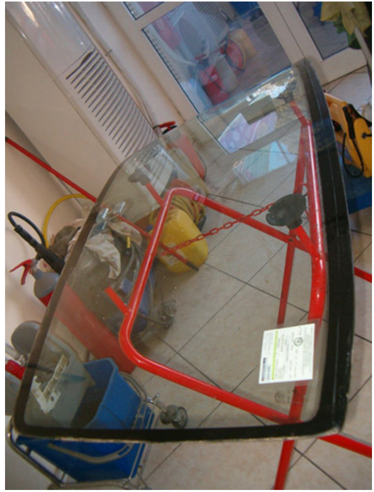
The screen is now out of the frame and sits on the bench waiting to be cleaned
