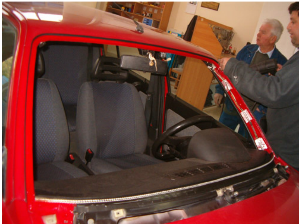
and Michael has almost finished. Notice the heat gun that helps the strip and himself to apply it to the frame
