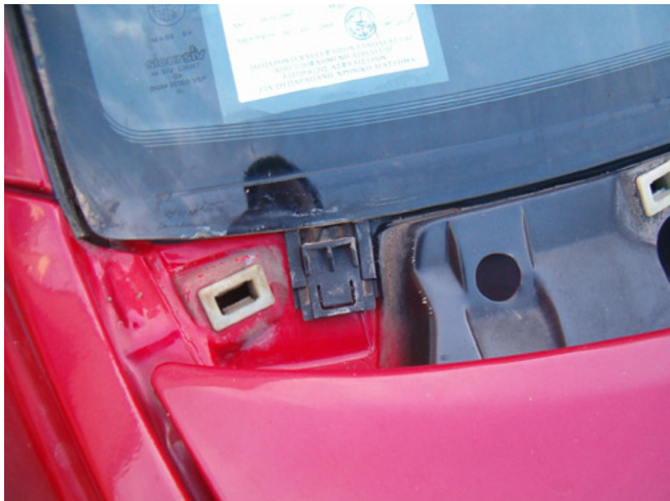
The plastic stops are lowered, so that removal of the windscreen is easier
