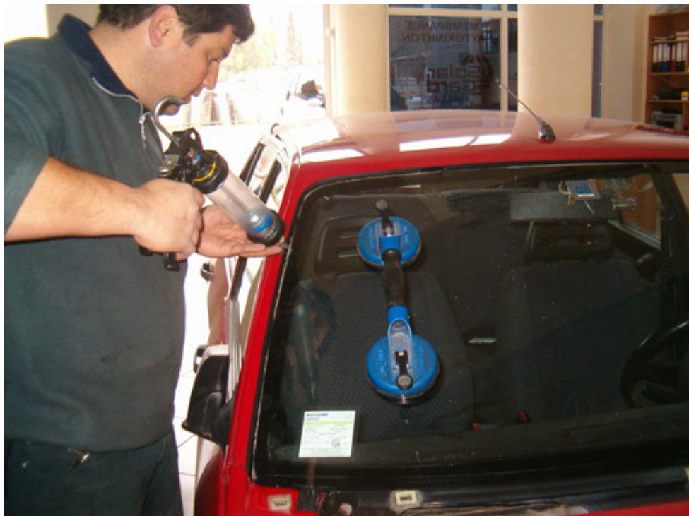
Michael is applying the final finish of windscreen glue to the gap and the decorative rubber strip is finally installed
