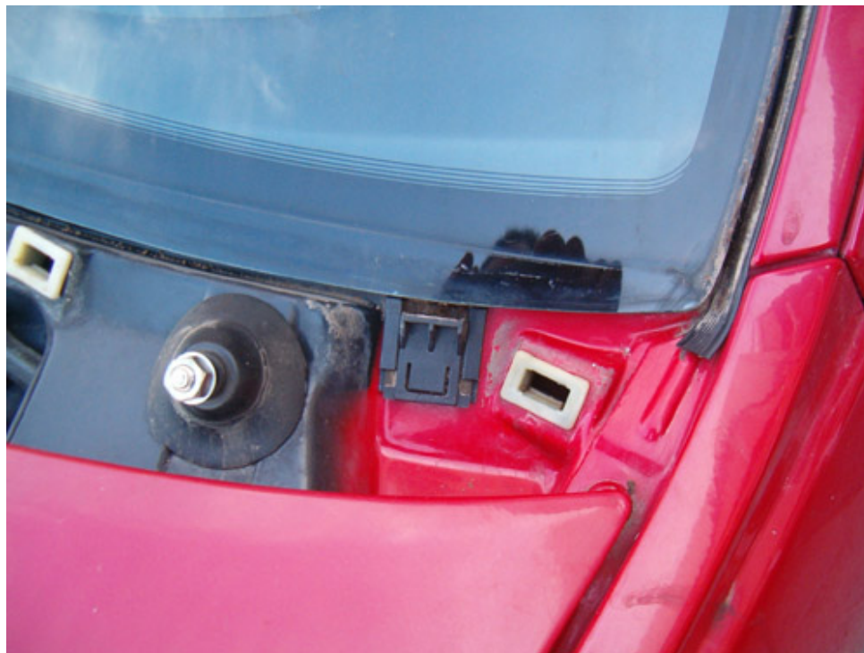
The plastic stops are lowered, so that removal of the windscreen is easier
