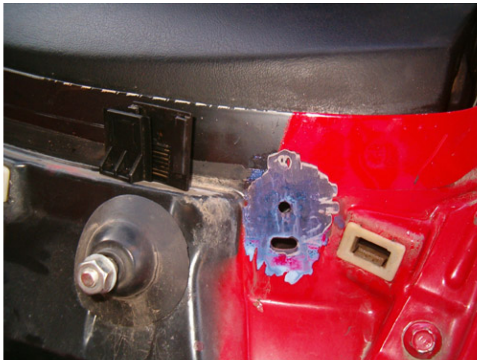
This milky fluid will convert to a black finish once it has bonded to the healthy metal
