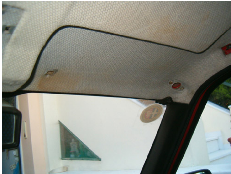
As a first step, remove the sunvisors (left and right side)
