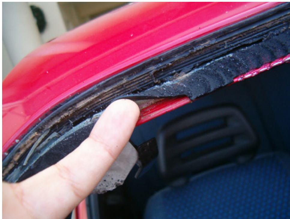
This is the origin of my troubles. The glue has separated from the frame and water found an easy way in
