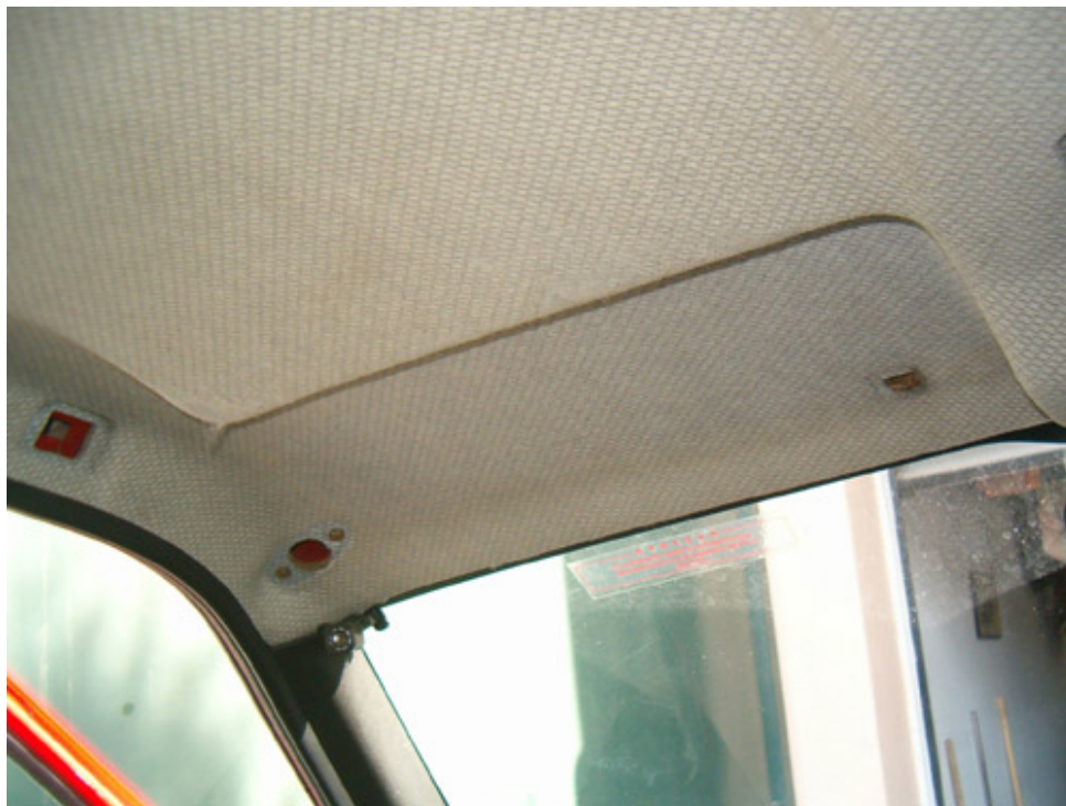
As a first step, remove the sunvisors (left and right side)
