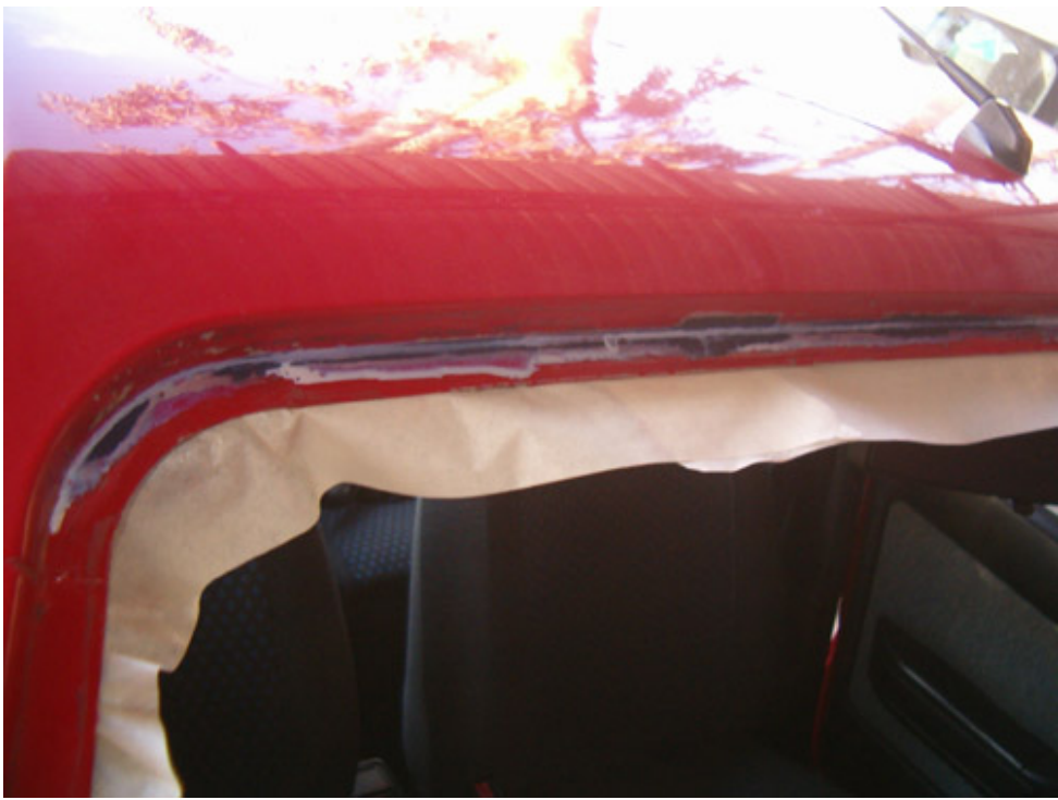
Inhibitor was applied to every area that had caught rust. This way we are confident that rust never forms again.
