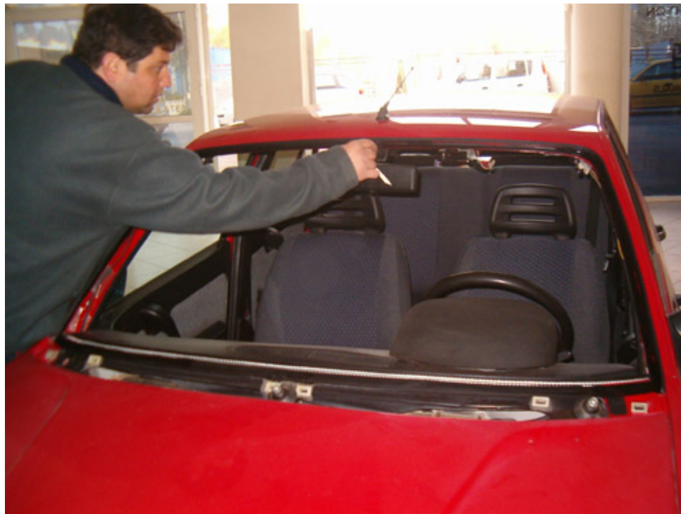
Michael now applies primer which enforces proper bonding between windscreen and metal frame
