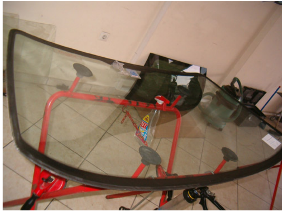
The 33 is now ready to have the windscreen installed. The windscreen expert has prepared the screen by removing traces of old glue.
