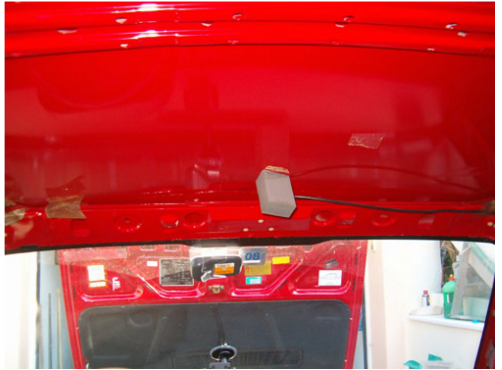
Carefully remove the headliner by pulling it from the trunk
