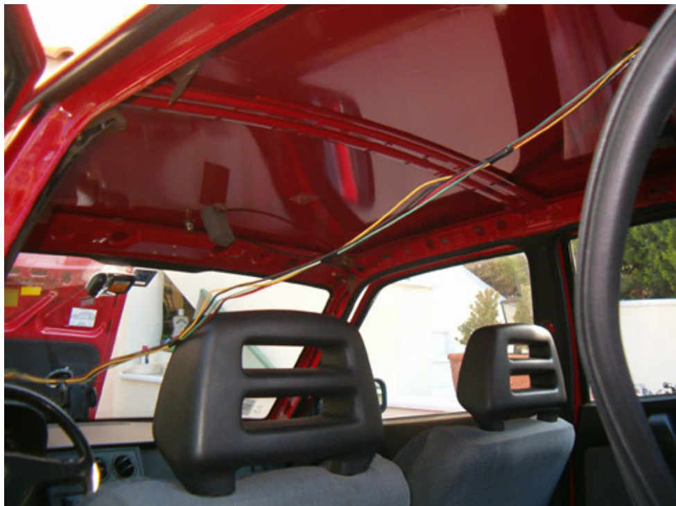
Interior after the headliner is removed
