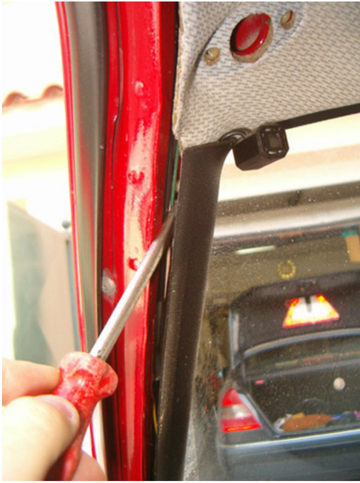
...using a long screwdriver remove the decorative shroud of the A-pillar post
