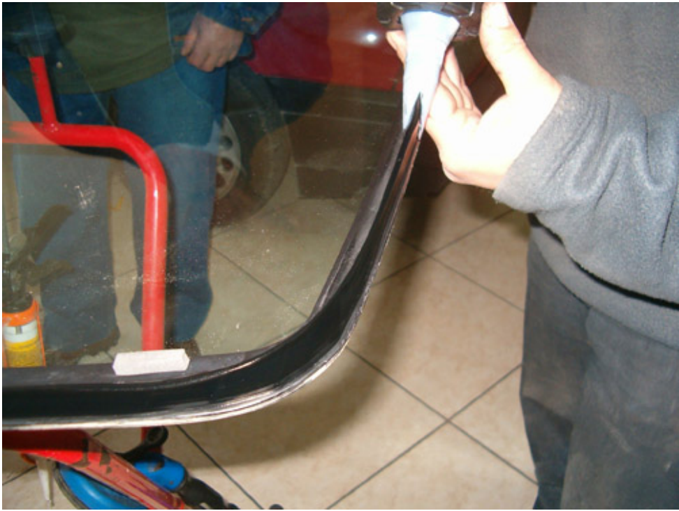
Close up of the glue while it is being applied; notice the height of it along with the quantity.
