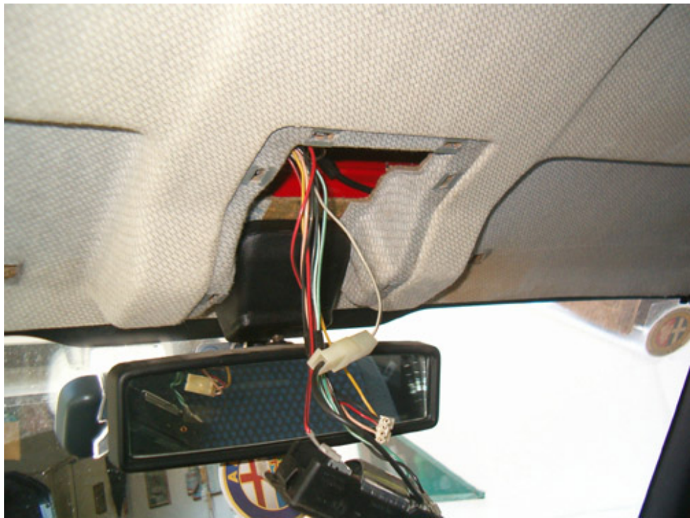
remove interior light and clock...
