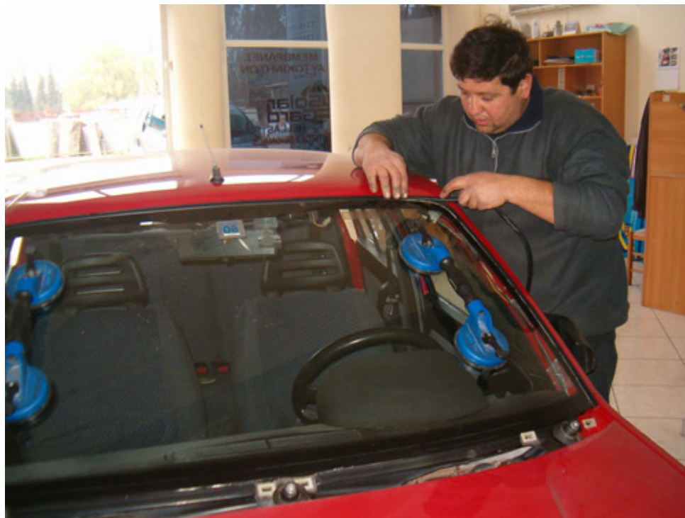
Michael is applying the final finish of windscreen glue to the gap and the decorative rubber strip is finally installed
