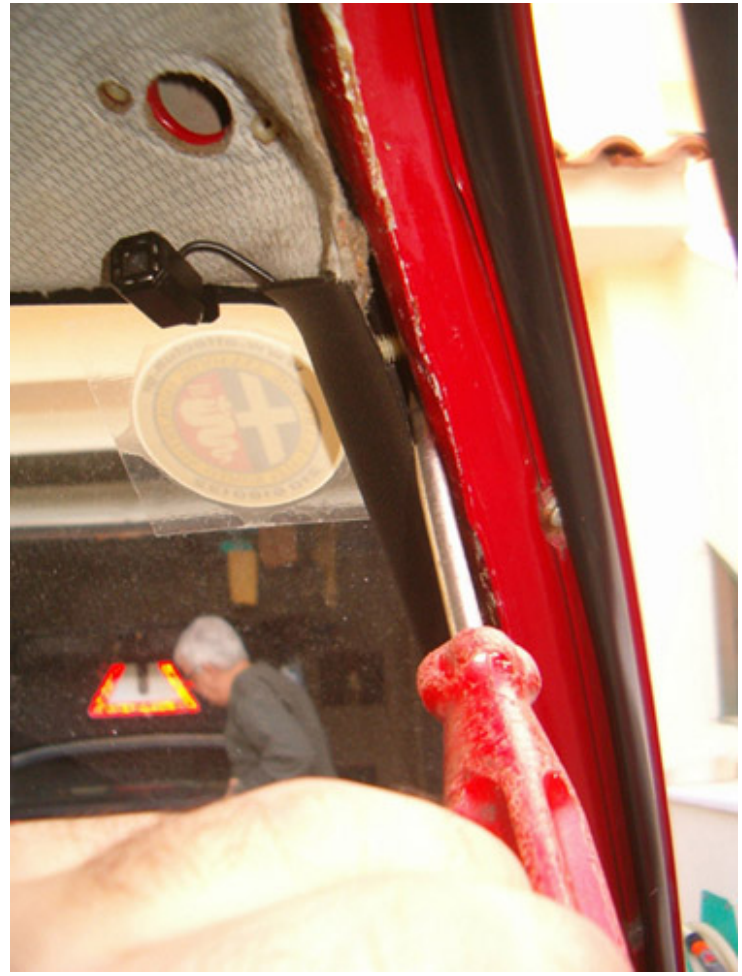
...using a long screwdriver remove the decorative shroud of the A-pillar post
