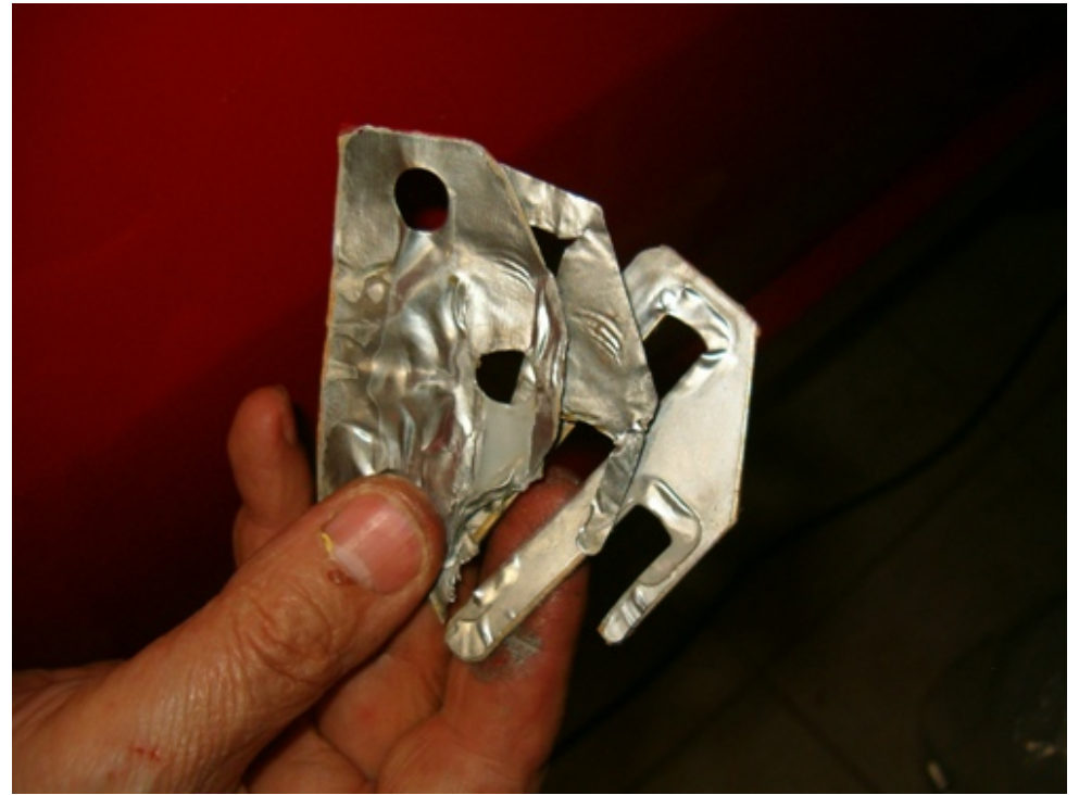
... these are the spacers and their adhesive aluminum foil wrapping them around - this is adhesive foil just for sticking hinge to body part while you are about to torque down the bolts.
