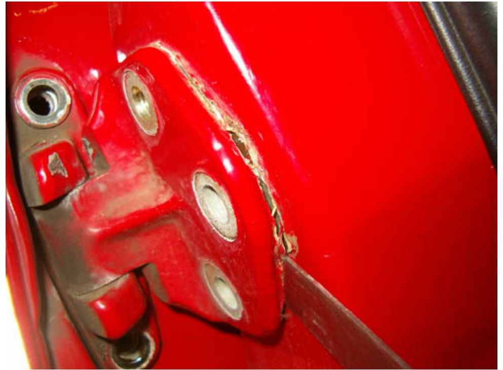
Here you see the hinge taken out using a slim knife
