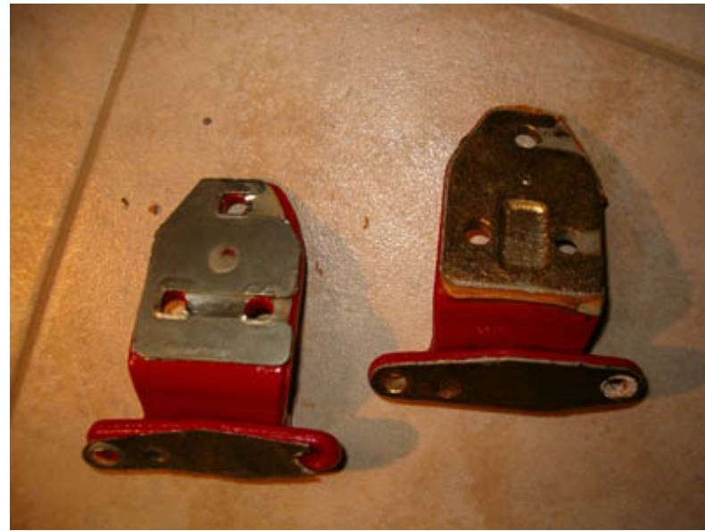
aluminum spacers installed on the new hinge (left)
