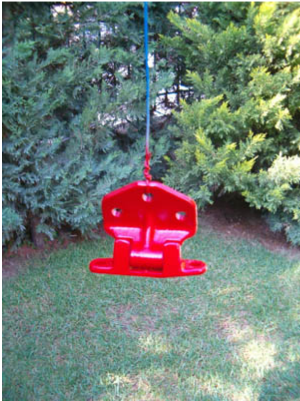
Here you see both of them after the second layer of red paint (Alfa Rosso 130); again let at least 24 hours between layers.
