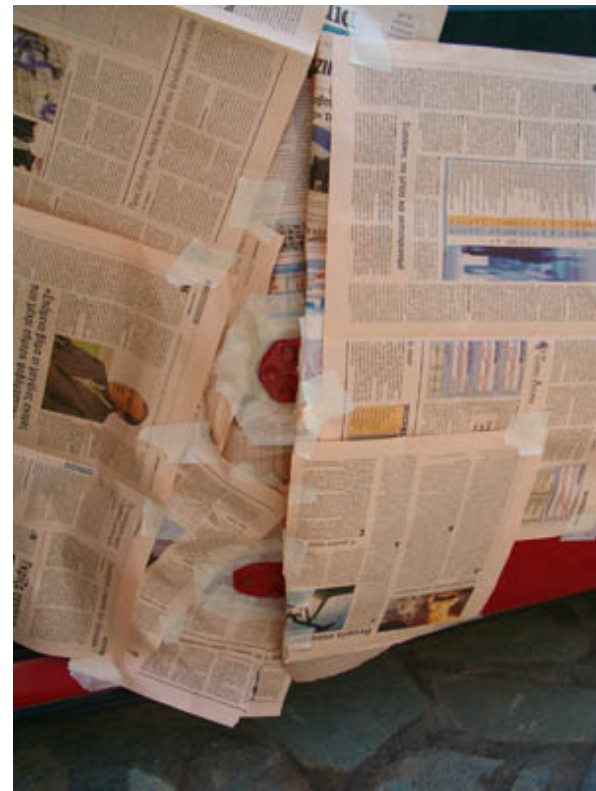
I have used many newspaper sheets and masking tape to cover up every place that paint would stain (plastic covers, rubber seals etc.)
