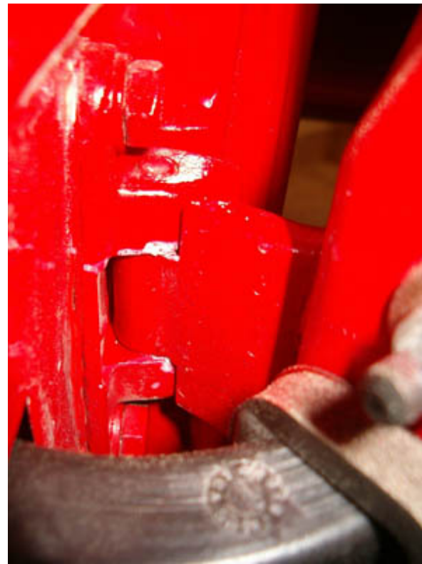
... and from inner side - don't forget to apply white lithium grease to hinges
