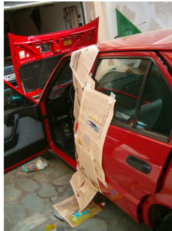
It is now time to paint the gray areas that seam sealer has left not matching to the car's color
