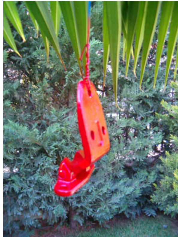
Here you see both of them after the second layer of red paint (Alfa Rosso 130); again let at least 24 hours between layers.
