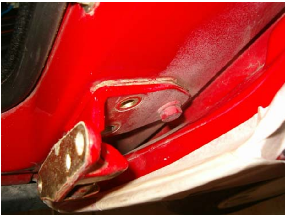
undo upper and lower hinges bolts.
