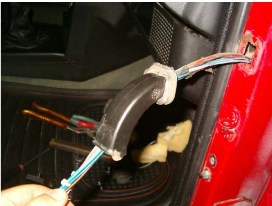
I have decided to replace the wiring snorkel with a new one.
