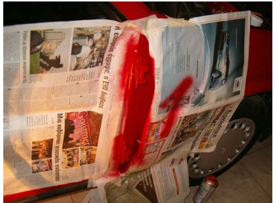
... and paint the freshly sealed areas and the area where factory paint could not reach.
