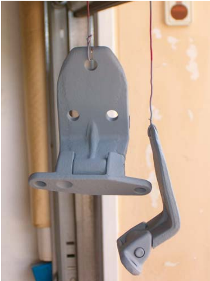
Two layers of primer should be applied.
