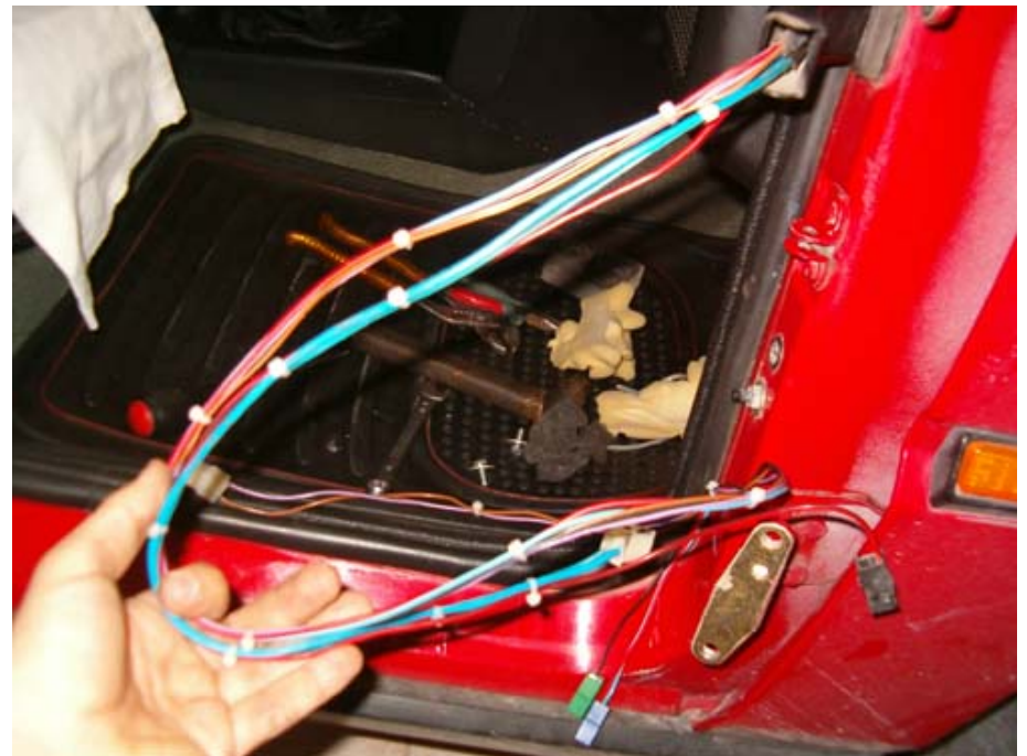
Time to tidy up the wiring harness.
