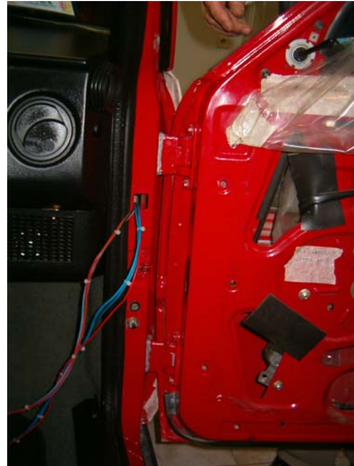
... and tighten the hinges bolts to the door.
