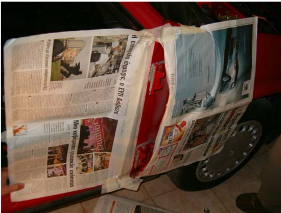
Mask the surrounding area with masking tape and newspaper sheets ...
