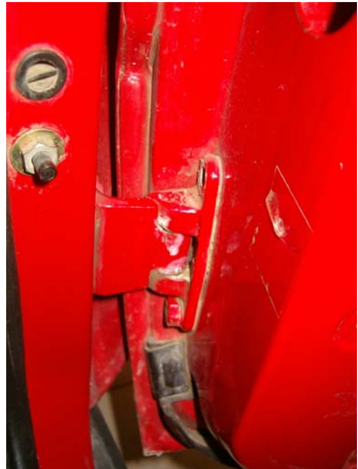
It would be wise to first remove the inner pair and afterwards the outer pair.
