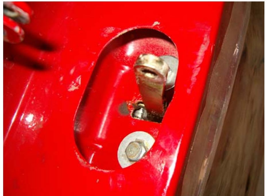
... and the two bolts keeping the tie-rod in place are revealed.
