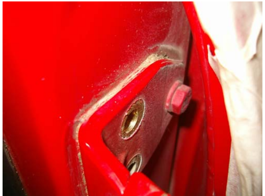
undo upper and lower hinges bolts.
