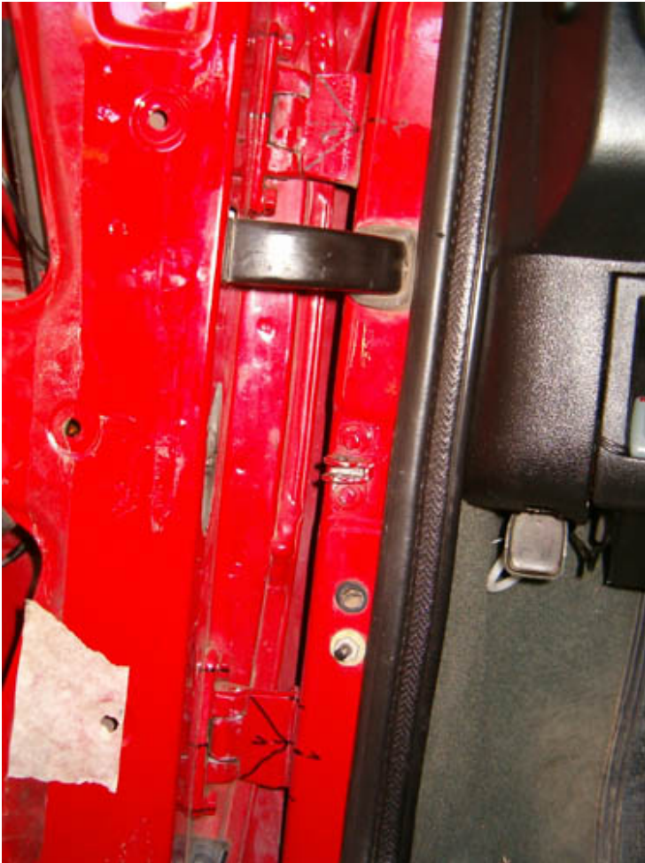
Here is a wider shoot showing the door stripped and left hung by the hinges. The door tie rod has been removed along with the door upholstery cards.
