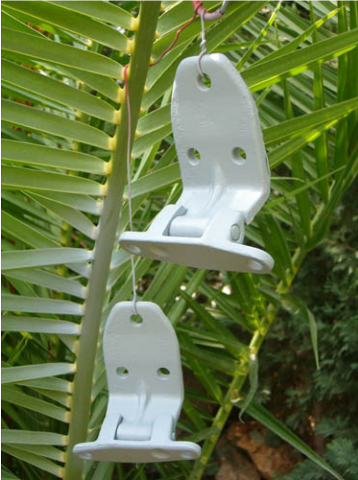
Here are the hinges after the first coat of primer. Another layer will be added after 24 hours...
