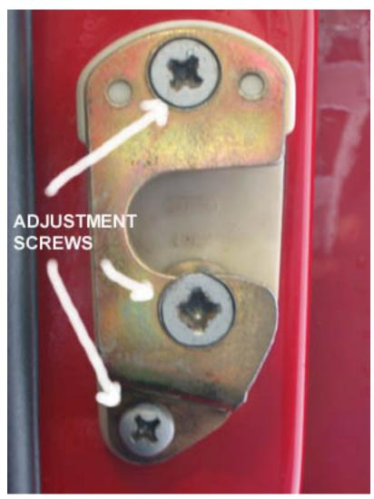
After installing new hinges, it would be necessary to proceed adjusting the door lock clamp. Over ages hinges wear and doors are gradually sagging, resulting in difficult and improper door closing. It may be possible to have adjusted the door lock clamp somewhere in the past in order to make your door function better, but now since the hinges are new, you should adjust the lock clamp from scratch.
