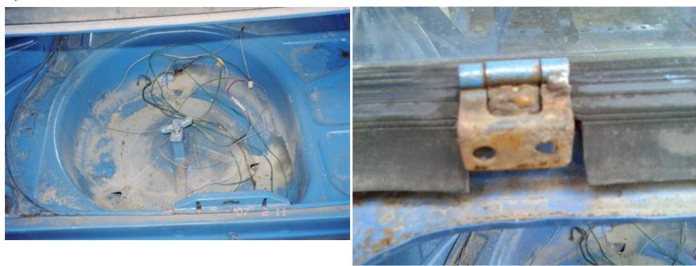
The spare wheel well appears to be in good order. However the wheel arches lips, inner wheel arches, bootlid hinges, lower valances, front chassis rails just to name a few really need attention and new metal welded
