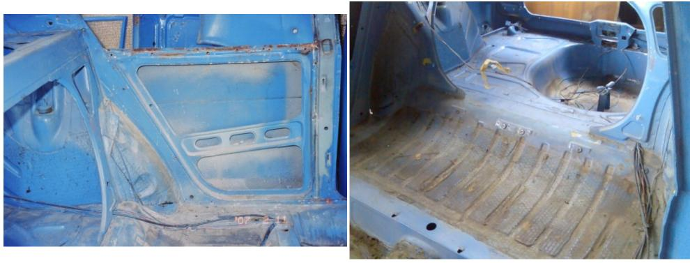
Tar sheets have been removed and the extend of rust is easily seen . Sills have been structurally weakened and for sure new metal will replace the old rusted sections
