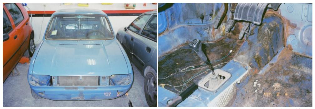
The interior has been completely removed in order to see the extend of rust. There are areas that have not been affected but other areas where structural meaning is essential, rust has eaten sheet metal rendering the car dangerous to drive.
