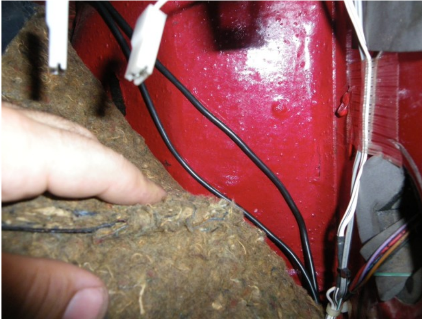
These two thick leads are the ABS wheel sensors going under the carper to the rear of the car.
