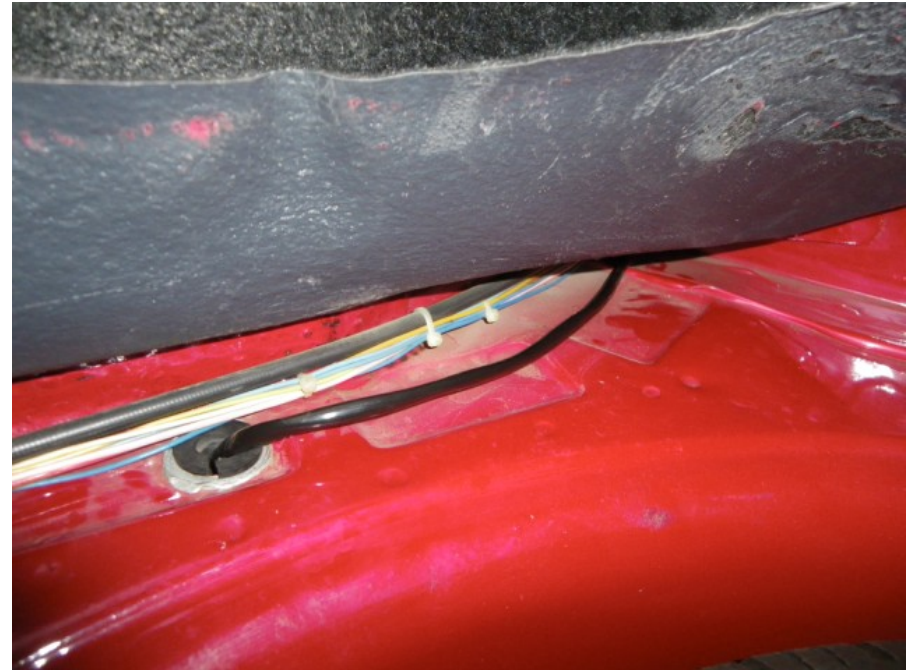
Pass the ABS wheel sensor through the rear chassis rails designated holes ...
