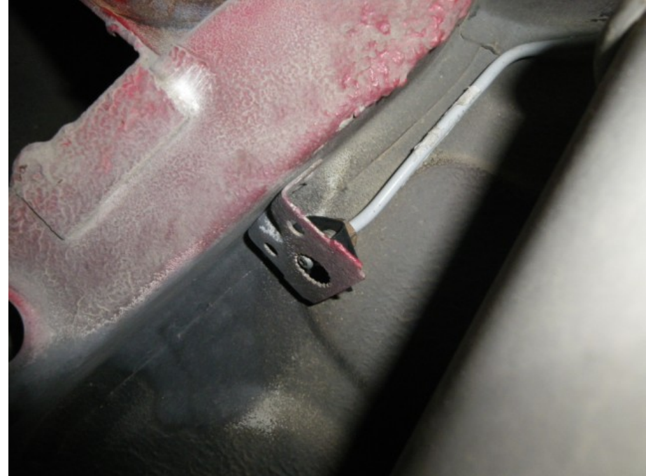
The brake line end meets the preinstalled bracket. Don't forget to use the U shaped spring which is there to keep the brake line and brake hose unions firmly attached.
