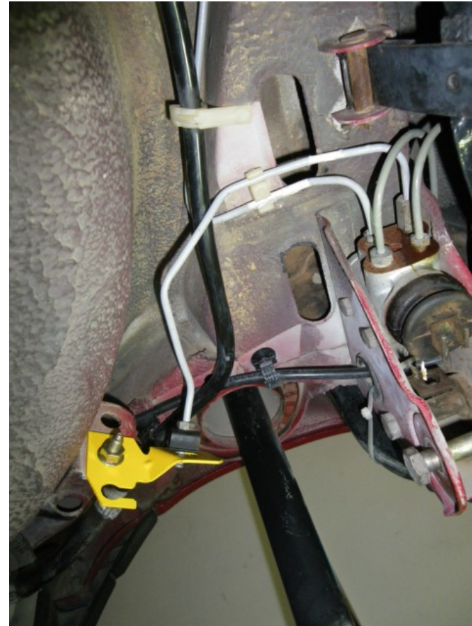
And their final positioning. Notice the extra bracket bolted on the existing bracket.
