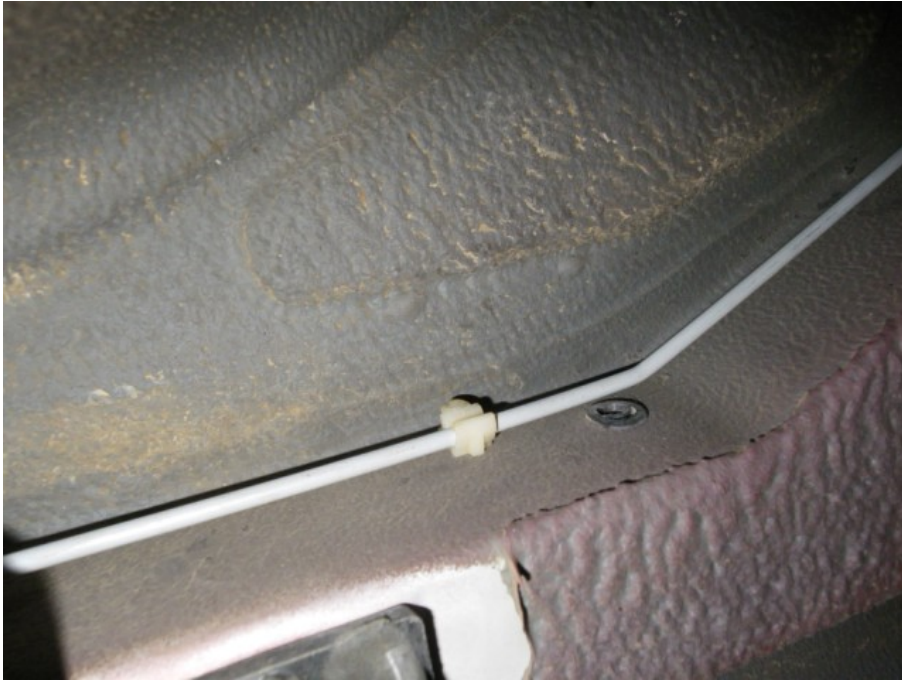
Right side wheel brake line routing. Even the brake pipe clips holes are present to the chassis. Getting hold of a brake lines clip ensure proper positioning.
