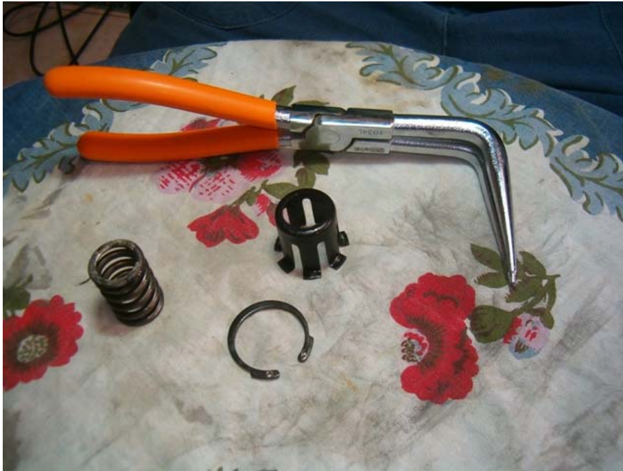
This is the pliers I am talking about. You can see the spring, tower and lock ring – these are from Dennis rear disk conversion project some years ago. Thanks a lot Dennis for lending me this handy tool!
