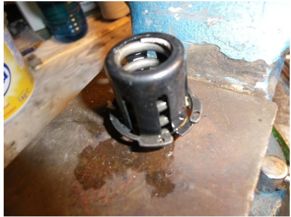
Here is the spring loaded tower along with the lock ring. As you can see there is a slack between the tower legs and the surface below. This space is taken up from the spring tension and it is really difficult to keep the spring down while trying to install the lock ring. All these must performed in a tiny space inside the bore... so you can imagine how important is to have the correct pliers.
