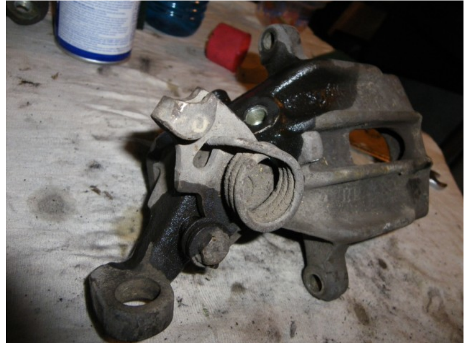
Here is the brake caliper. It is black and dirty holding many years of brake dust and road grim.
