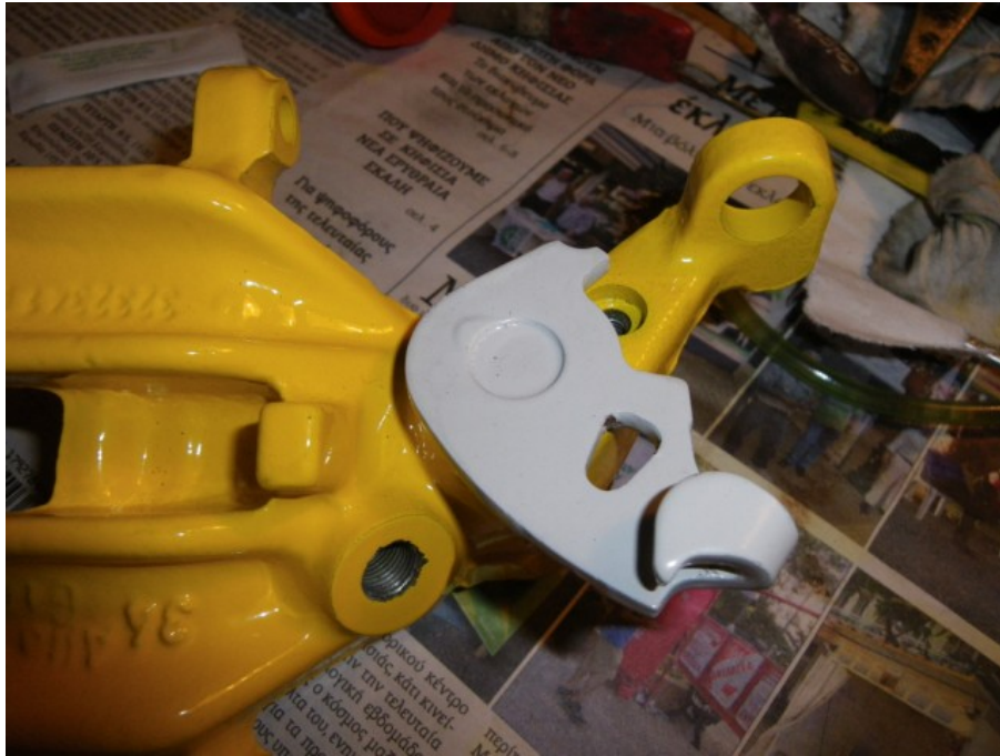
Install the handbrake mechanism lever and push it all the way in.
