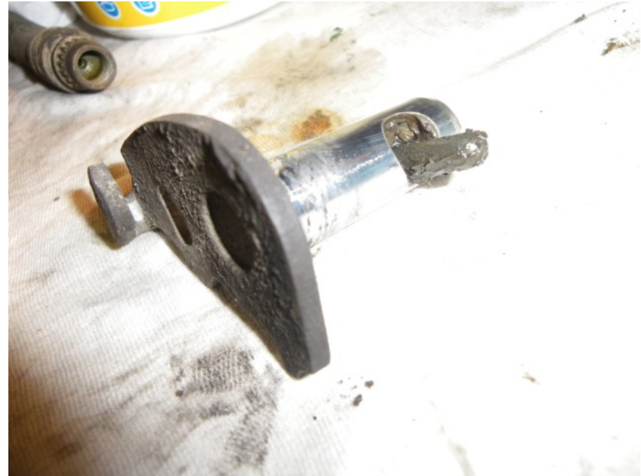
By acting on the handbrake lever this small rod acts on the threaded rod (left photo) and thus the brake pads are acting on the brake disk. This way the rear wheels are locked.
