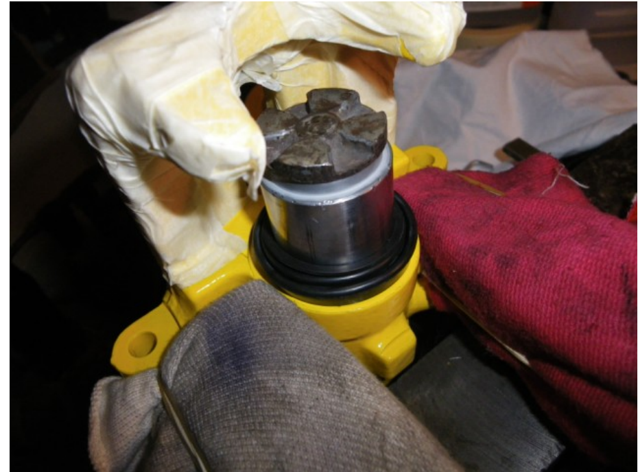
Finally install the piston. Be sure to expand carefully the seal in order to pass over the piston.
