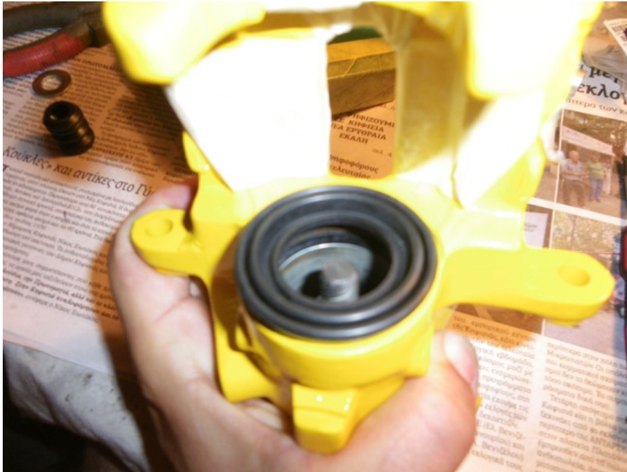
Next install the dust seal – again be sure to correctly install the seal on the respective groove.
