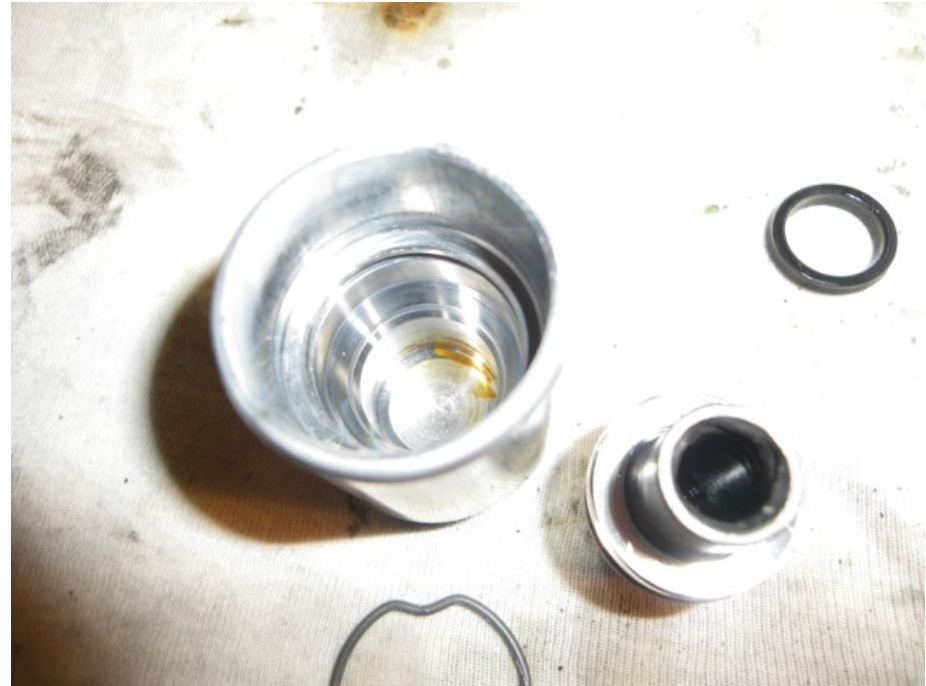
In the mean time, the internals of the brake piston have been taken out. We will deal with the piston later on.
