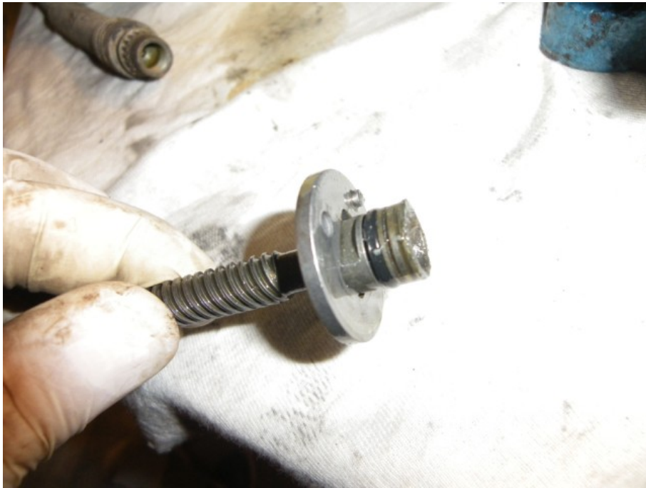
Here is the threaded rod out of the piston bore. On the right there is a recess where the rod which appears on the right side photo is placed.
