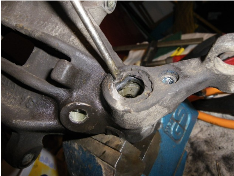
A final step for stripping the caliper bare is to remove the above seal. This is where the handbrake rod enters – this seal keeps away dirt.
