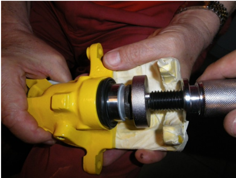
Once it has passed over, use the special tool (this tool is the one for replacing brake pads) to wind in the piston.
