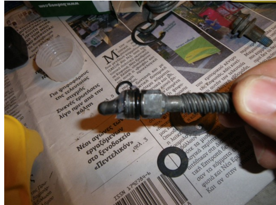
Apply grease on the threaded rod recess and be sure to replace this o-ring. This is the seal which prevents brake fluid from entering this chamber.
