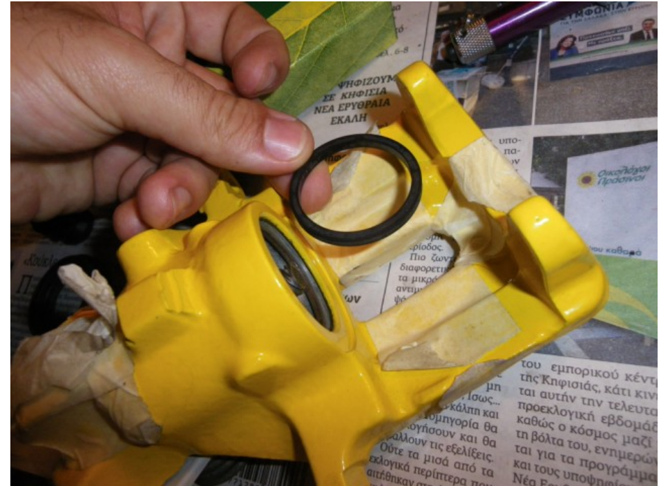
Install piston seal by carefully placing it on the groove. You must also lubricate the piston bore and seal groove with brake fluid.
