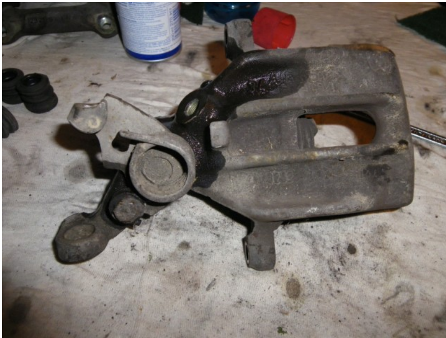
Here is the brake caliper. It is black and dirty holding many years of brake dust and road grim.
