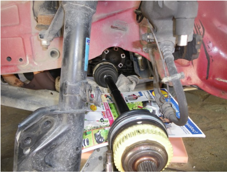
Place the new half-shaft on its relative position.
