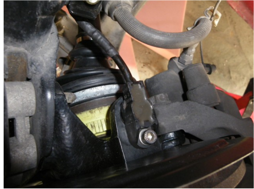
... and brake caliper. Install the ABS sensor on the specified bracket.
