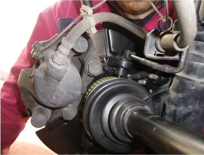
Wheel hub from the inside showing ABS sensor, CV joint induction teeth.
