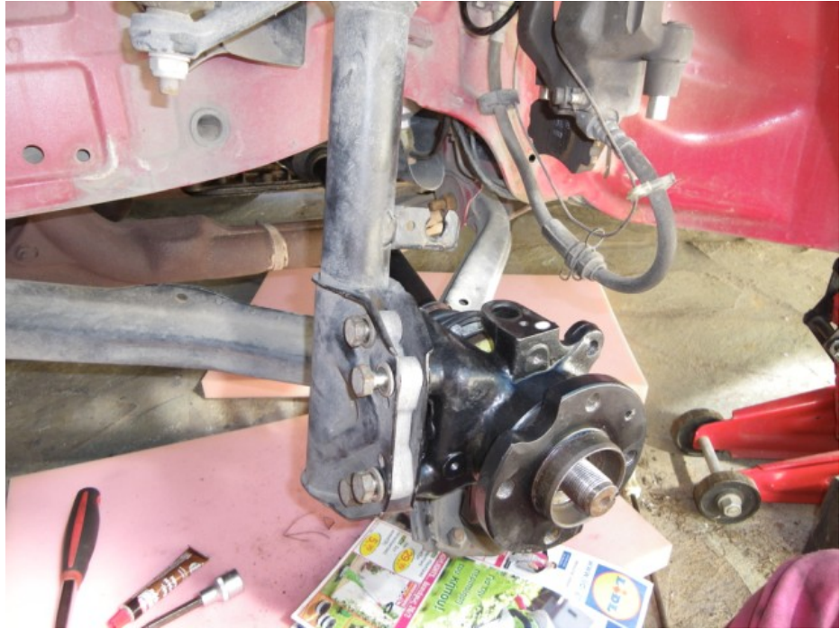
Do the same for the shock absorber and hub bolts.
