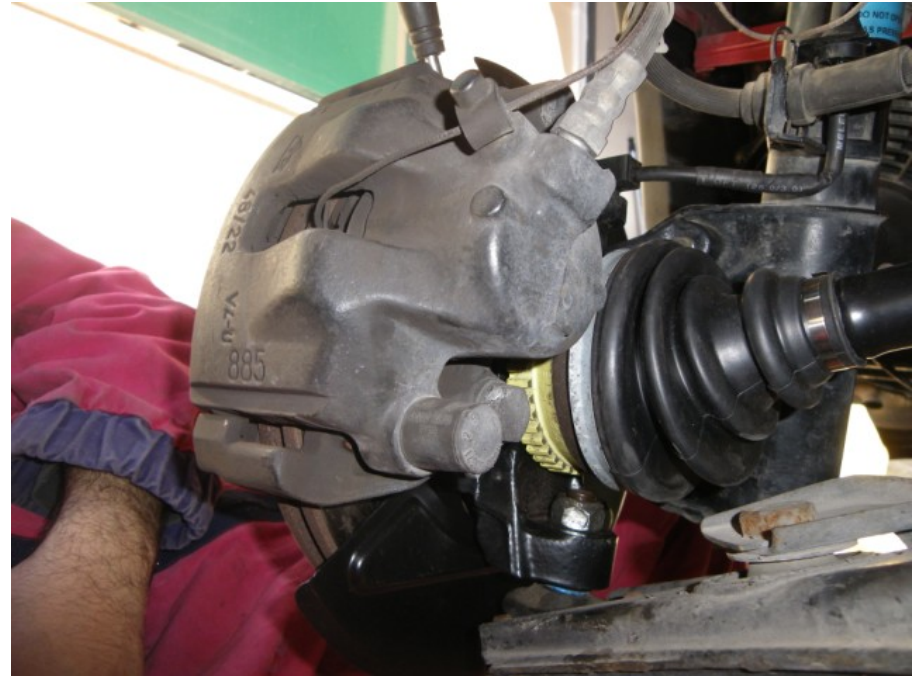
Wheel hub from the inside showing ABS sensor, CV joint induction teeth.
