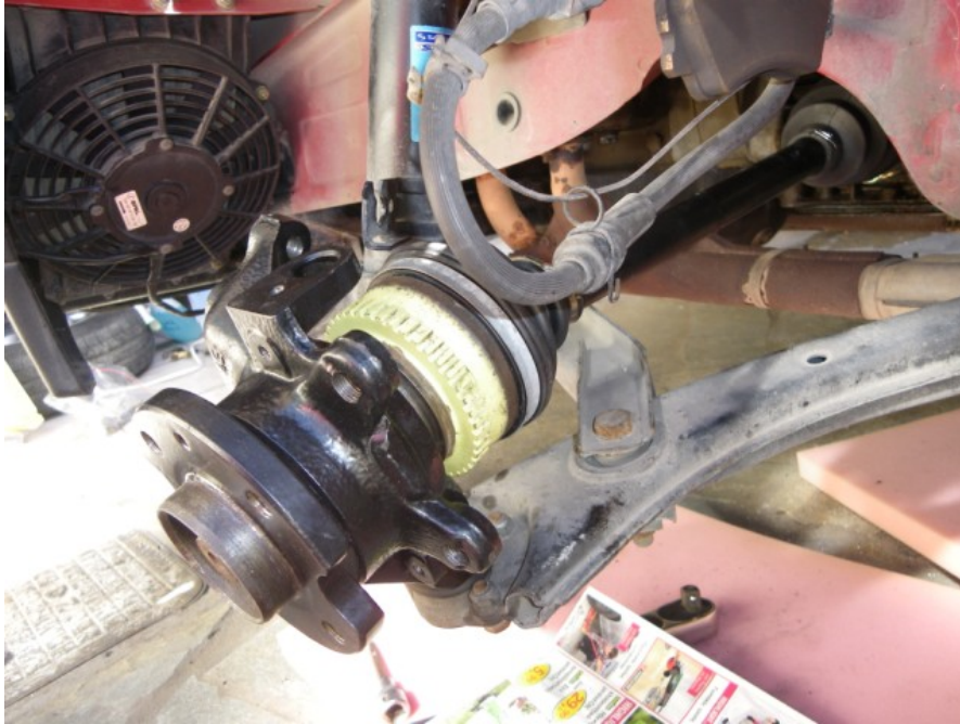
Install a couple of CV bolts so that the half-shaft sits correctly in its position.
