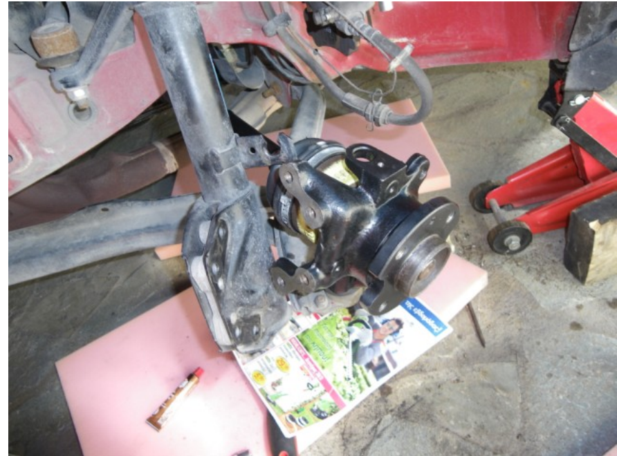
Install the wheel hub and secure it on the lower arm ball joint.
