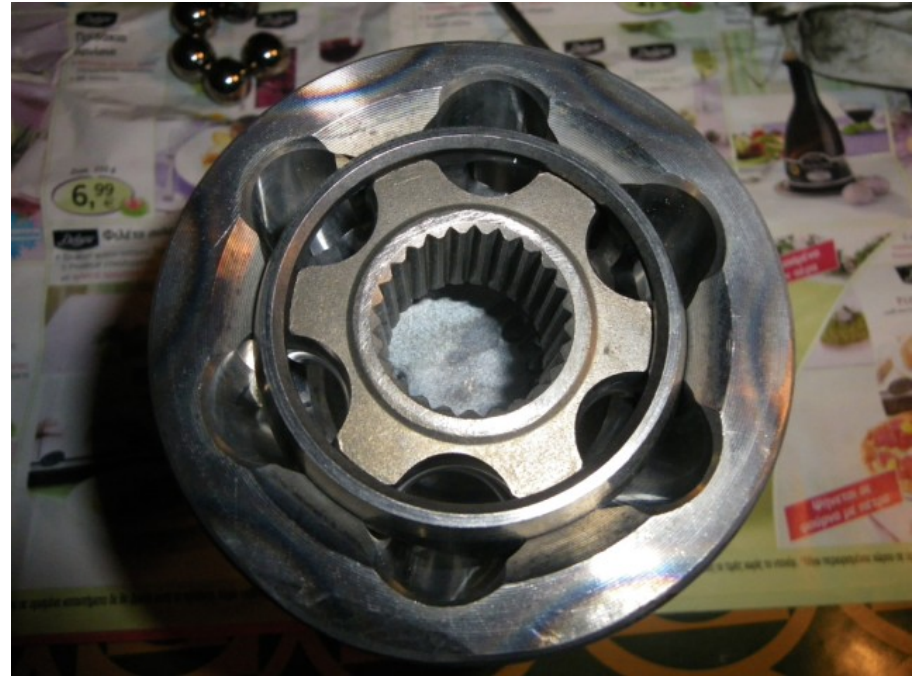
CV joint in the correct setup without the balls. Working one cavity at a time, you may press in the balls. The CV joint appeared to be a little worn out but with the rearrangement of the balls, carrier and splined part, I have rearranged the wear so that the CV now feels firm. This way I have given it more life.
