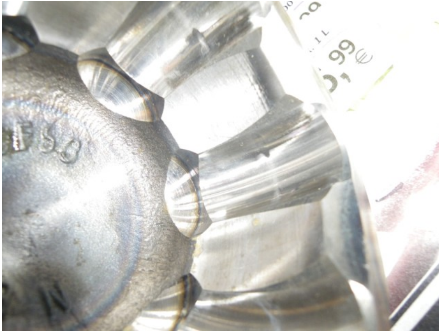
I have demonstrated this close-up of the CV internal cavity in order to show the wear on the recess of the wall.
