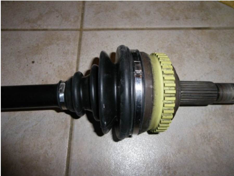
As a last action we will install the CV boots bands for the outer joint ...
