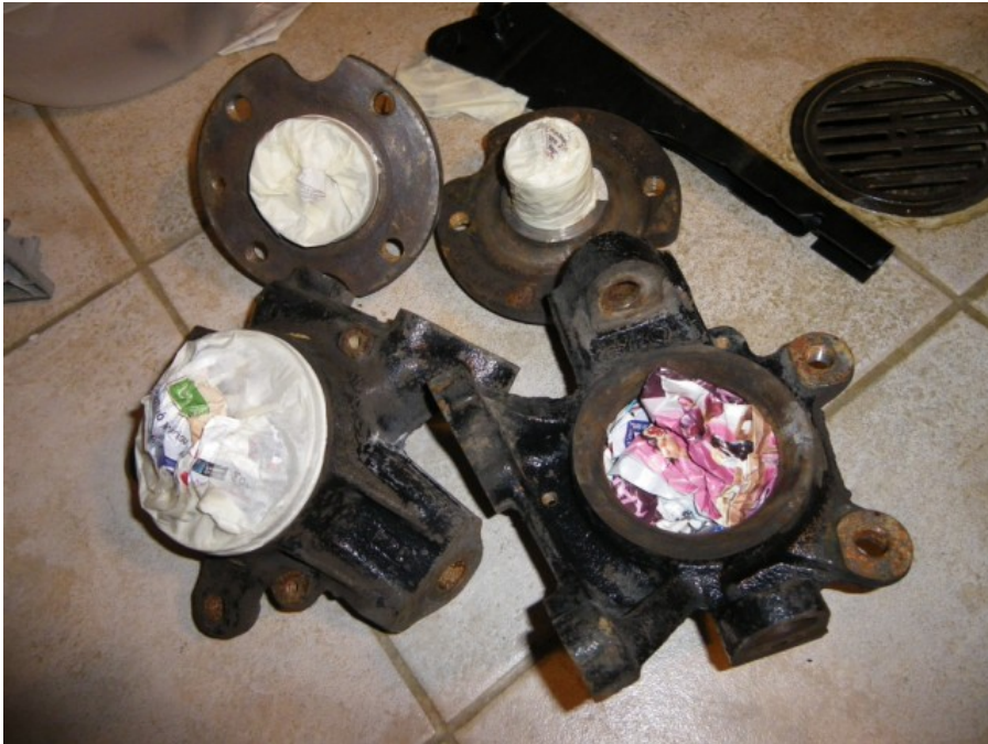
Last but not least are the hubs. Here you can see them as they came off the donor car. They will be taken to the sandblaster – I have masked the places I don't want to be affected like the bearing cavity or the hub carrier.
