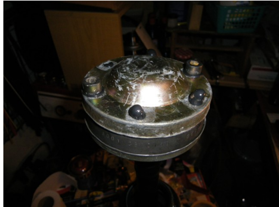
Install the CV cases and keep them aligned to each other relative to the joint by placing two CV bolts. This way the orientation of the two cases and the CV joint body will be straight.
