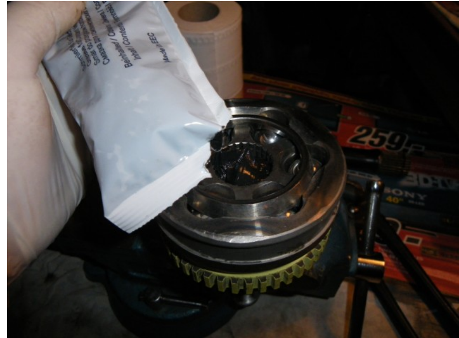
Fill in grease from the splined opening. Be sure to press in grease until you see it coming off the balls. You should now stop ...
