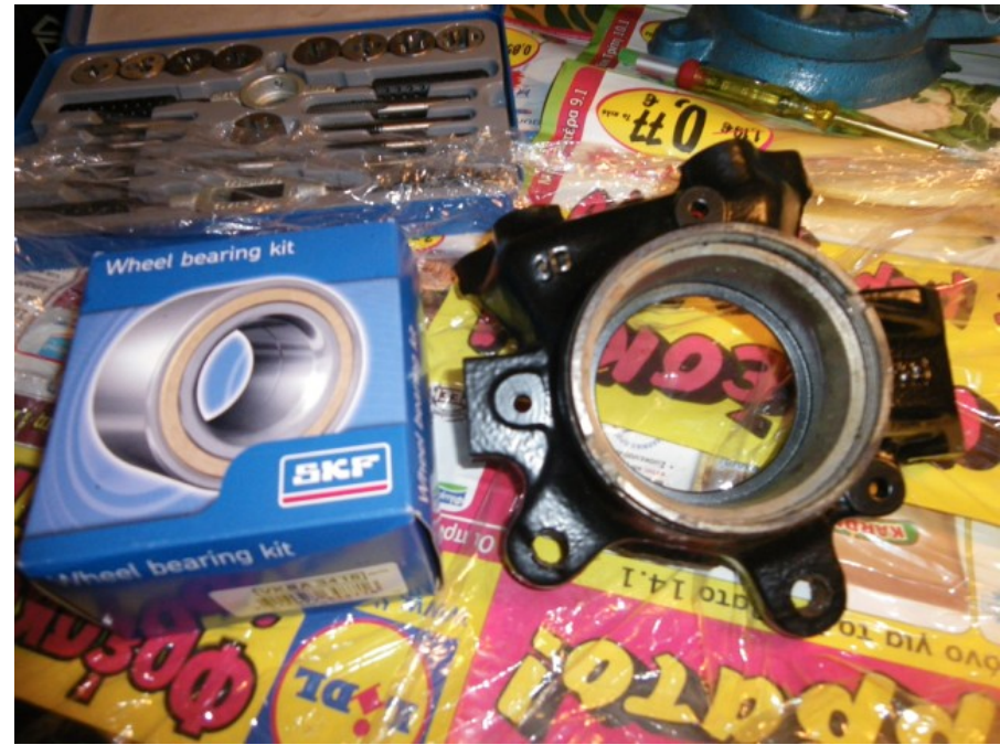
Hubs freshly powder coated along with new bearings. These were pressed in using a hydraulic press.
