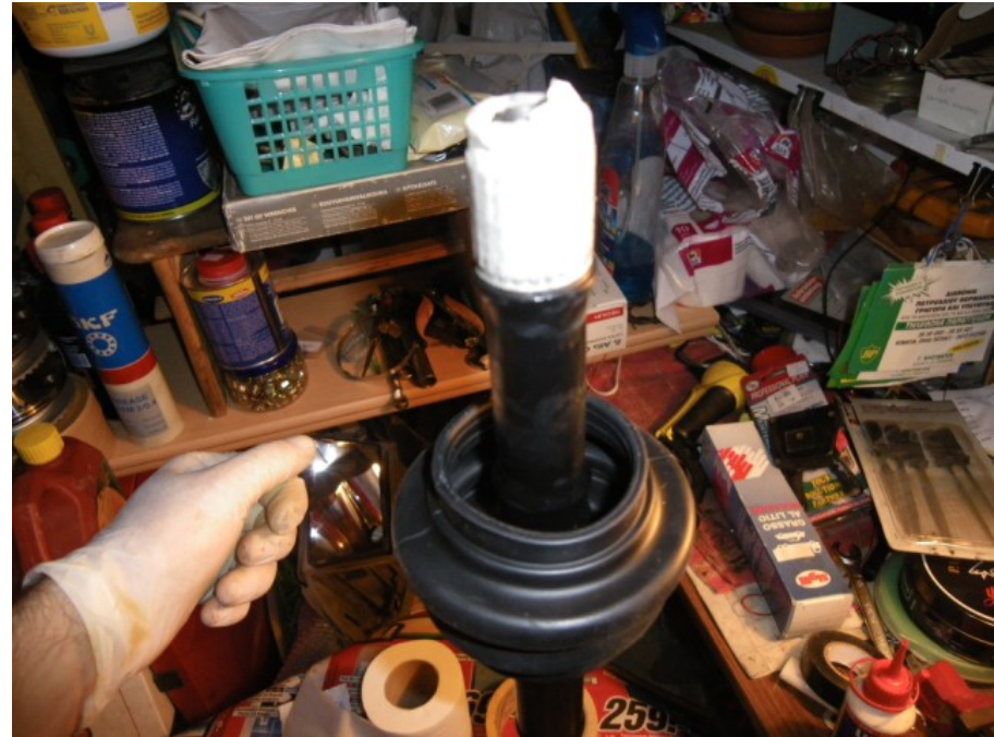
Slide in the inner CV boot. As you notice I have covered the splines with tape in order to avoid damage to the boot.
