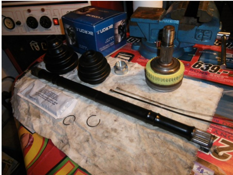
Ready for assembly. New CV boots and freshly powder coated shafts.
