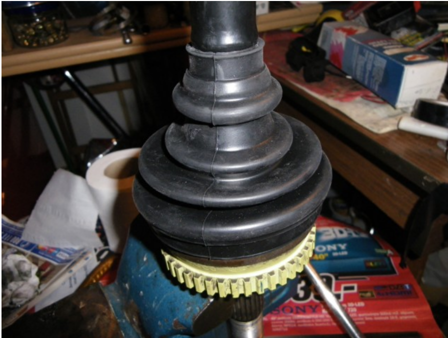
Slide in the outer CV boot and be sure to have it rest on the designated groove on the shaft and CV joint.
