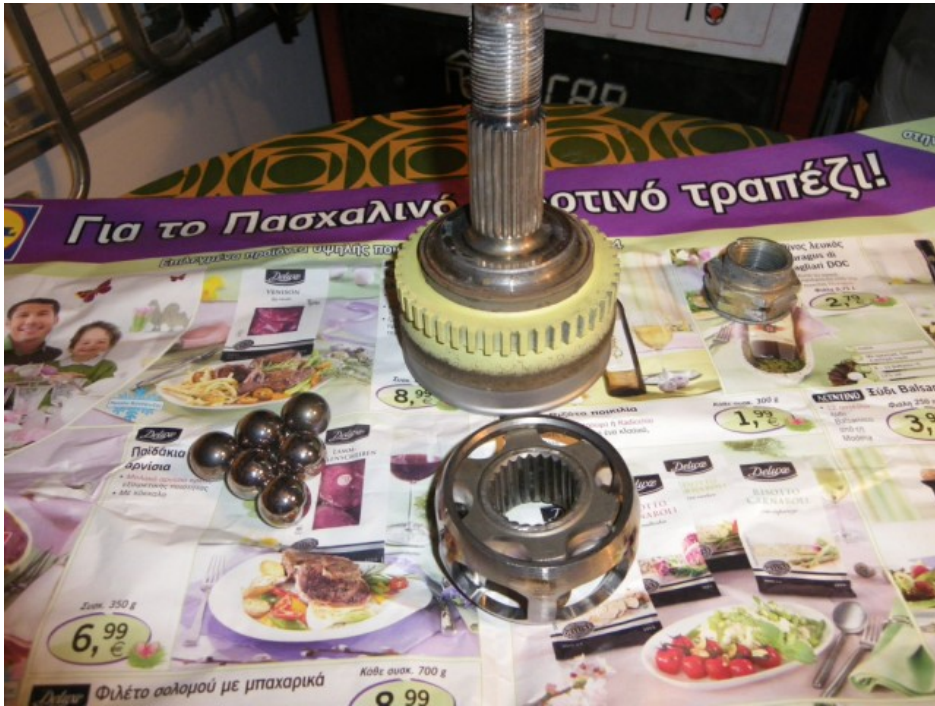
I have done the same for the outer CV joint meaning degreasing and cleaning it thoroughly.
