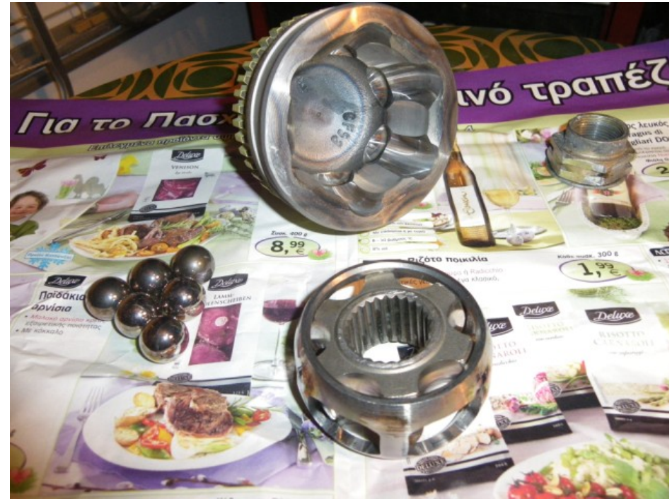
A closer photo of the CV joint.
