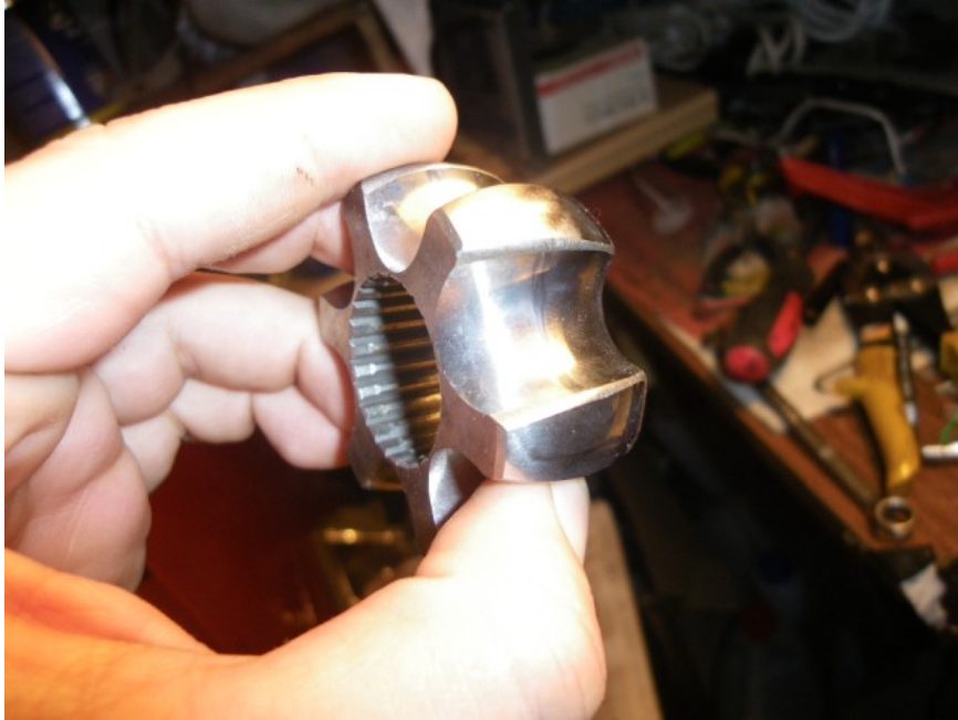
... and here you can see the splined part of the joint where the shaft enters
