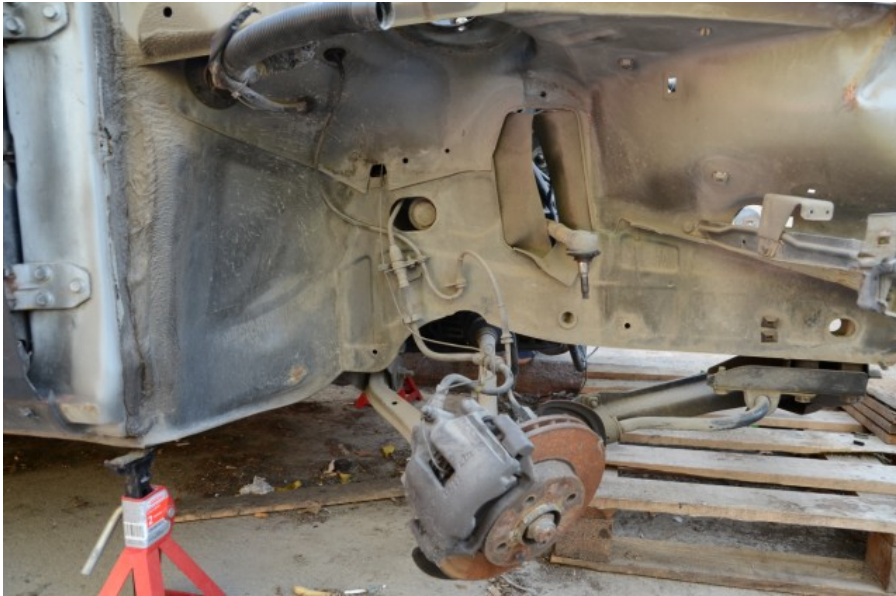
Front hubs showing the ABS wiring. Not seen on the photo is the different CV joint compared to the non ABS versions. The ABS version features a teeth ring which the ABS sensor reads the status of the wheel (rolling or locked)
