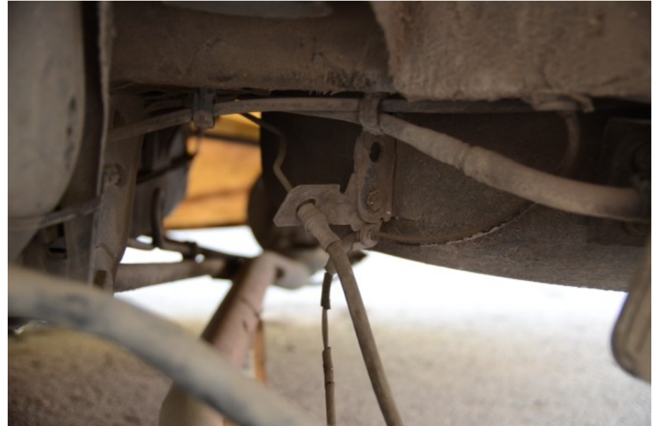
Different bracket setup. A bracket holds the brake hose and the ABS sensor wiring.
