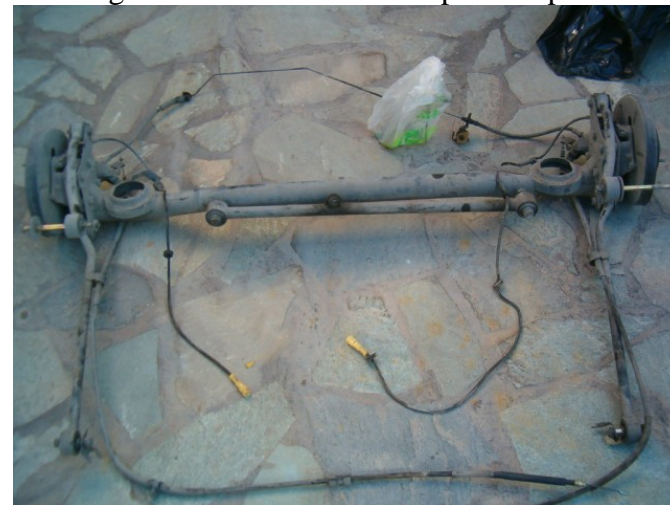
These two wires are connected to the brake light switch. This variation of wiring compared to non-ABS versions feed the ABS unit with input letting it know when the brake pedal is pressed.
