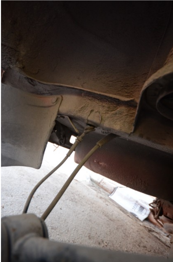
Right side of the rear axle. Brake hose attached to the right wing rail bracket while the ABS sensor wiring runs to the same area.
