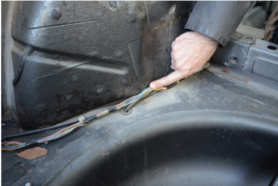
ABS wiring enters boot through the designated openings on each side.
