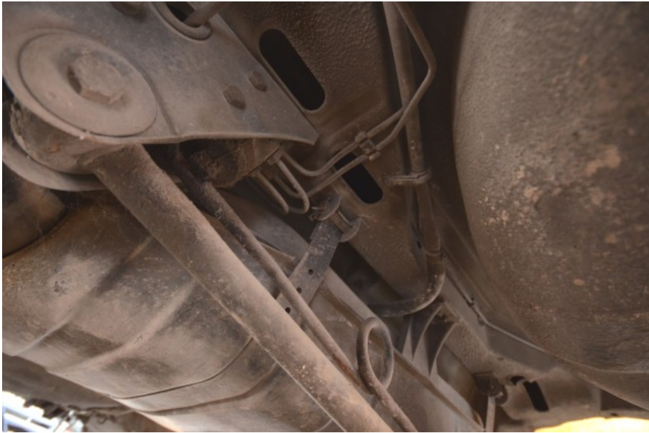
Here is the different brake lines layout. Notice the brake line which runs around the circumference of the spare wheel well.
