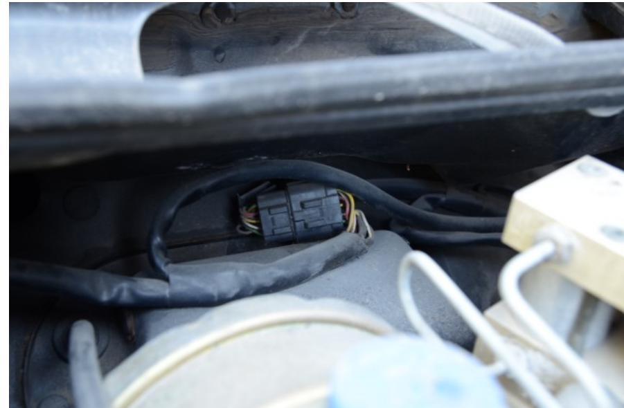
ABS Unit on the left side of the service compartment. Intermediate wiring connector on top of the brake servo container.
