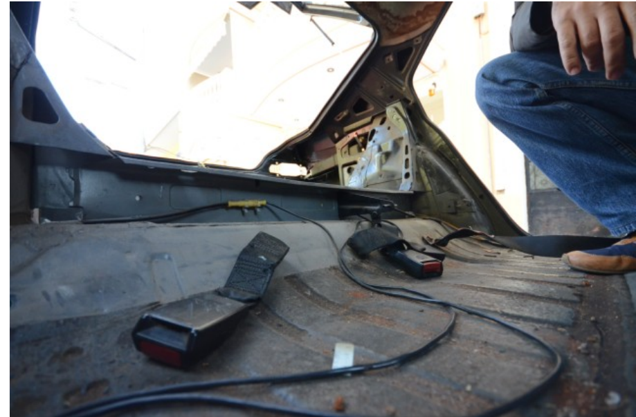
Inside the passenger compartment. ABS sensor wiring runs under the rear seats.
