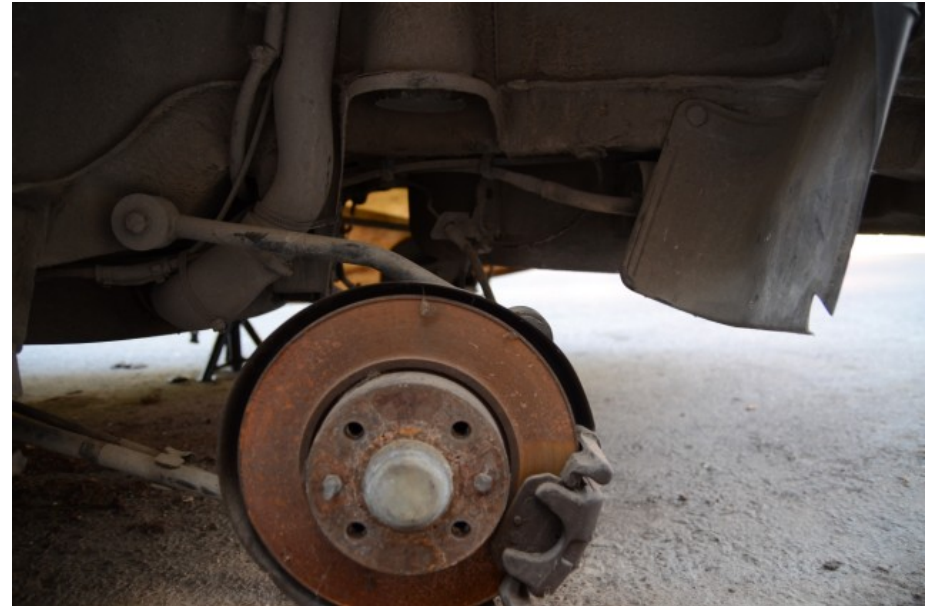
Rear axle. Luckily springs are already out so we will remove the axle easily.
