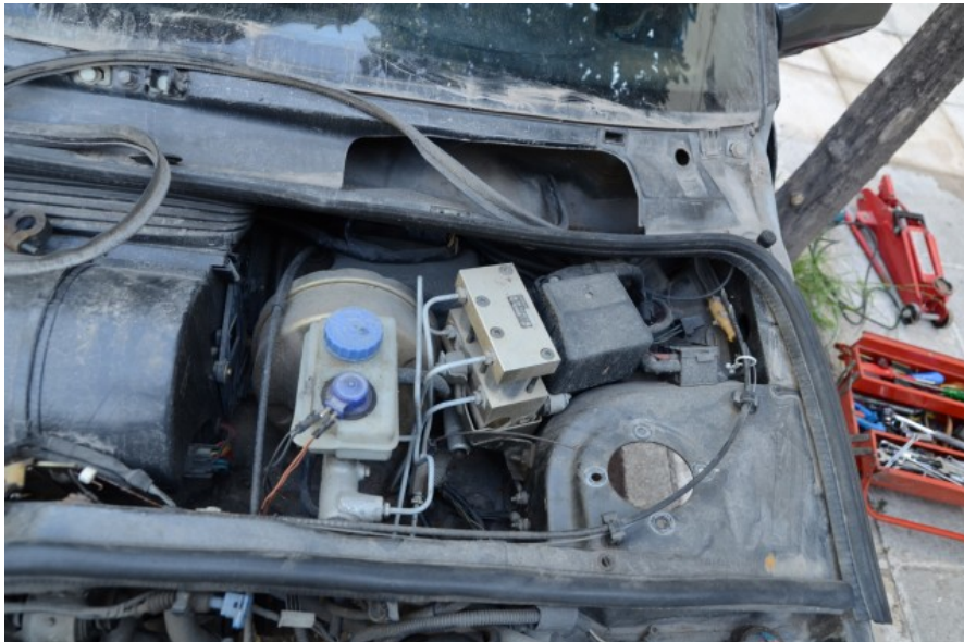
ABS Unit on the left side of the service compartment. Intermediate wiring connector on top of the brake servo container.
