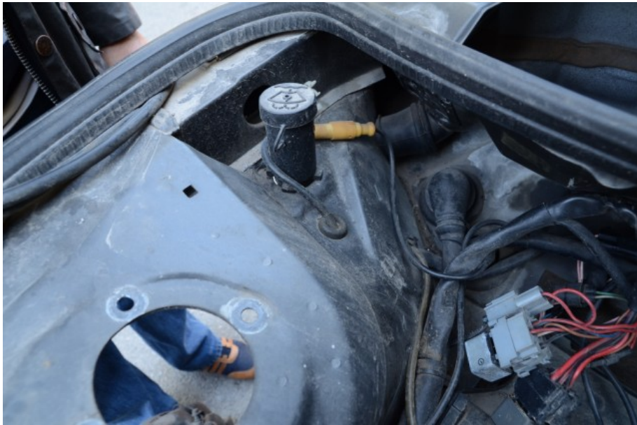
ABS sensor connector (yellow plug) – also found on the left of the service compartment
