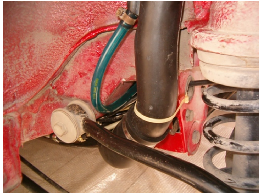
Filler neck is in place with clamps properly tightened, blue relief hose attached to filler tube and properly zip tied.
