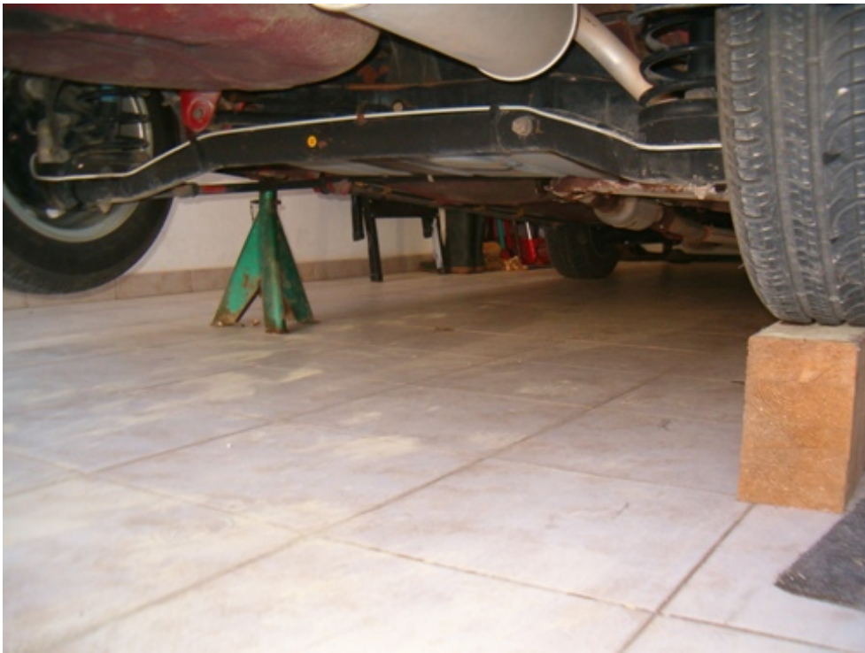
Lift the rear of the car. I have used the good old way of a jacking stand a piece of wood under the wheel.
