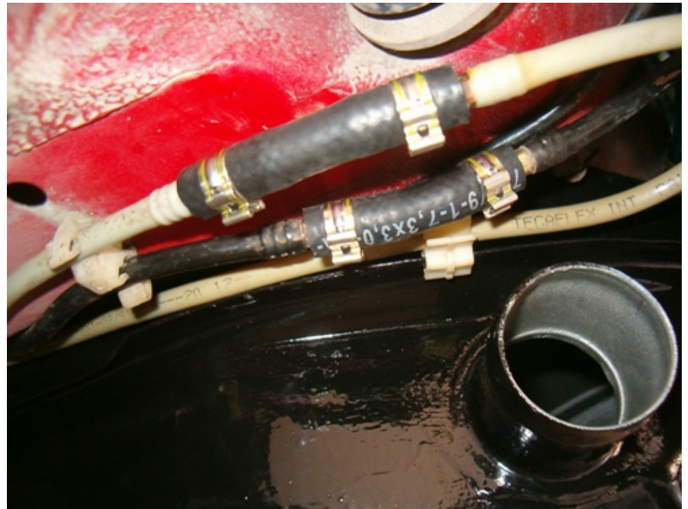
New 8 mm ID rubber lines fitted. Again black is for supply and grey for return.
