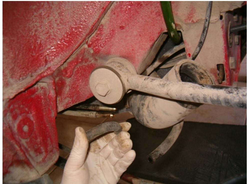
Lets begin by removing the fuel lines along with the plastic fuel filler neck; should it be necessary renew them. Mine showed crack signs so they will be replaced with new ones.
