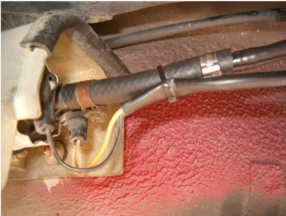
Finally a new hose is also installed to the fuel pump outlet.
