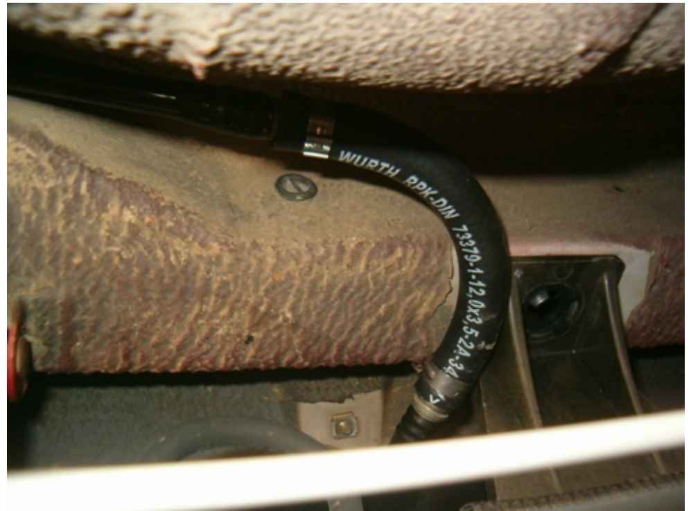
Fuel feed line is attached and properly clamped
