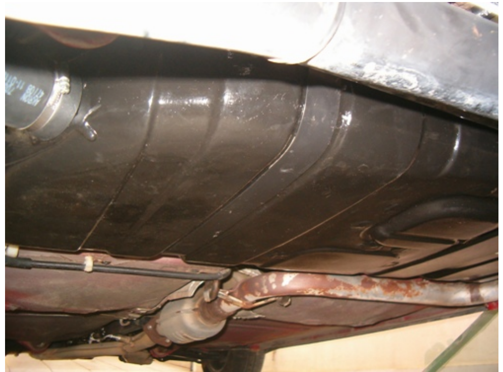
Fuel tank straps are fully tightened.
