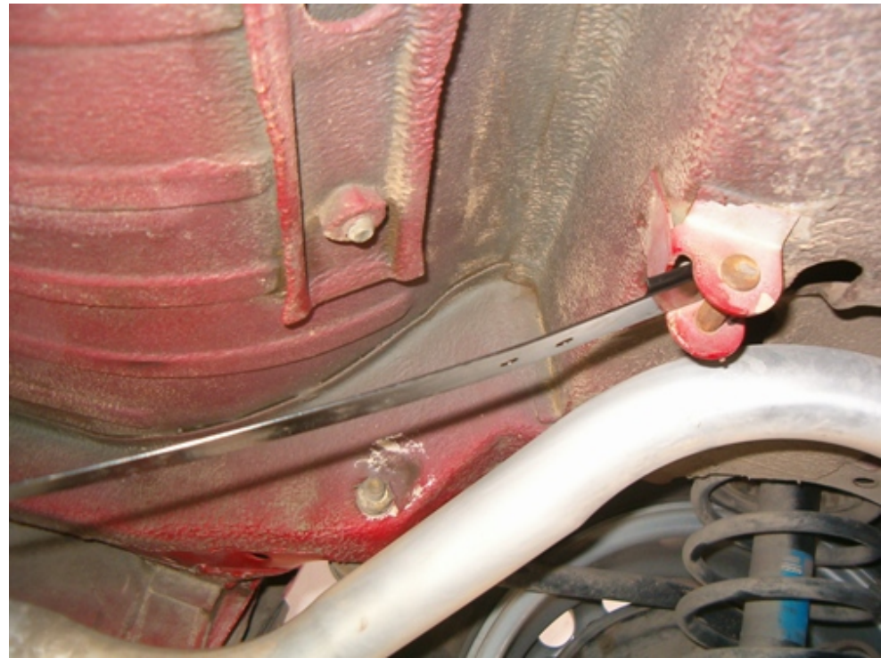
All the underside covered by the tank has been cleaned and new straps are ready to keep the tank in place
